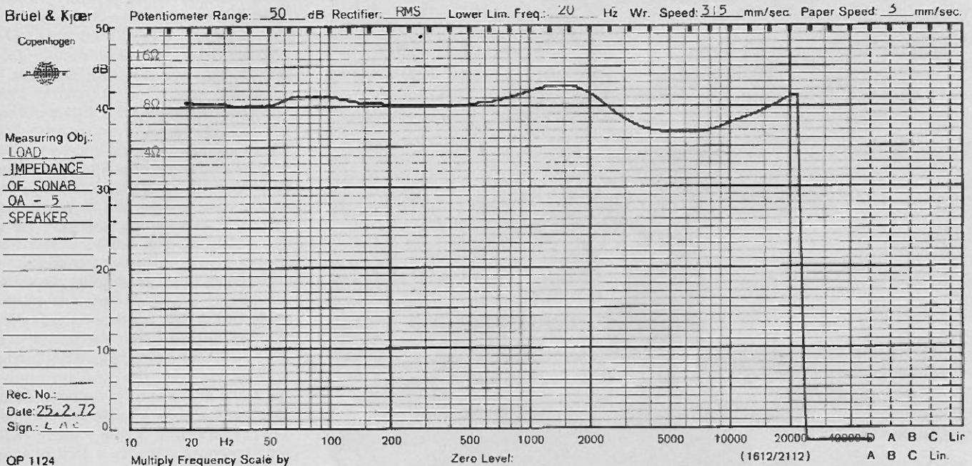
another at 5000Hz. The smoothest frequency response was obtained with the floor covered with 1" thick semi-rigid fibreglass. Under these conditions an unusual characteristic was observed in the form of a high level of sub-harmonic distortion generated at frequencies up to 10 times the speaker's resonance. Rather surprisingly at 500Hz the 50Hz sub-harmonic component was only 30dB down.
