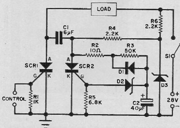
Originally developed by the Unitorde Corporation, this circuit will supply up to four Amps for a period of one second when triggered by an external positive going pulse.
