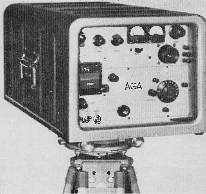
cycles and coarse position is found by determining which coarse cycle is being used. As it is not practical to traverse the whole distance and count cycles, a method of frequency changing is used to decide the coarse distance. This light beam method can measure 20km distances to 10 mm. The latest units, (one is shown in Figure 12), use laser sources to improve the range in daylight.
