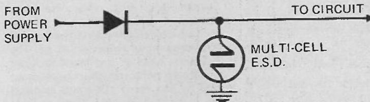
Fig. 1a. Circuit symbol ESD represents dual function of a filter capacitor rated in farads, and as a low capacity storage battery.
