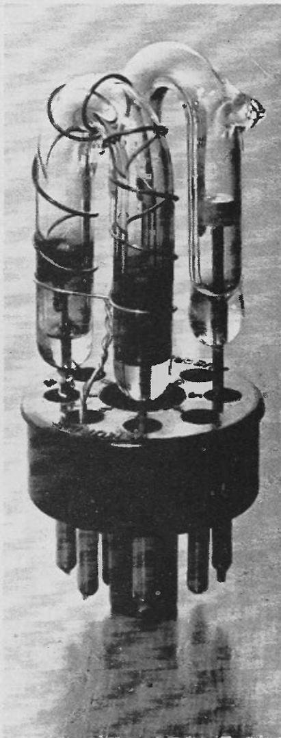
Fig. 4. Two strobe tubes are mounted in one octal holder. A triggering lead has been wrapped around one tube to show technique.
