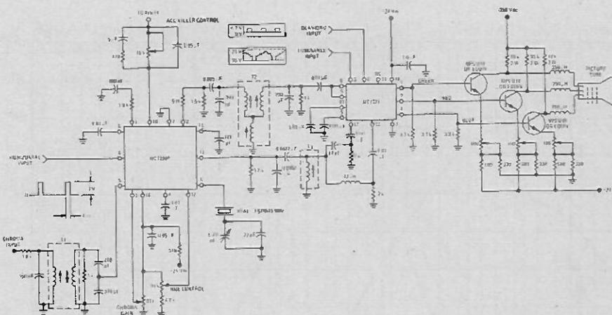
Fig. 3. Typical chroma processing circuit for colour television.
