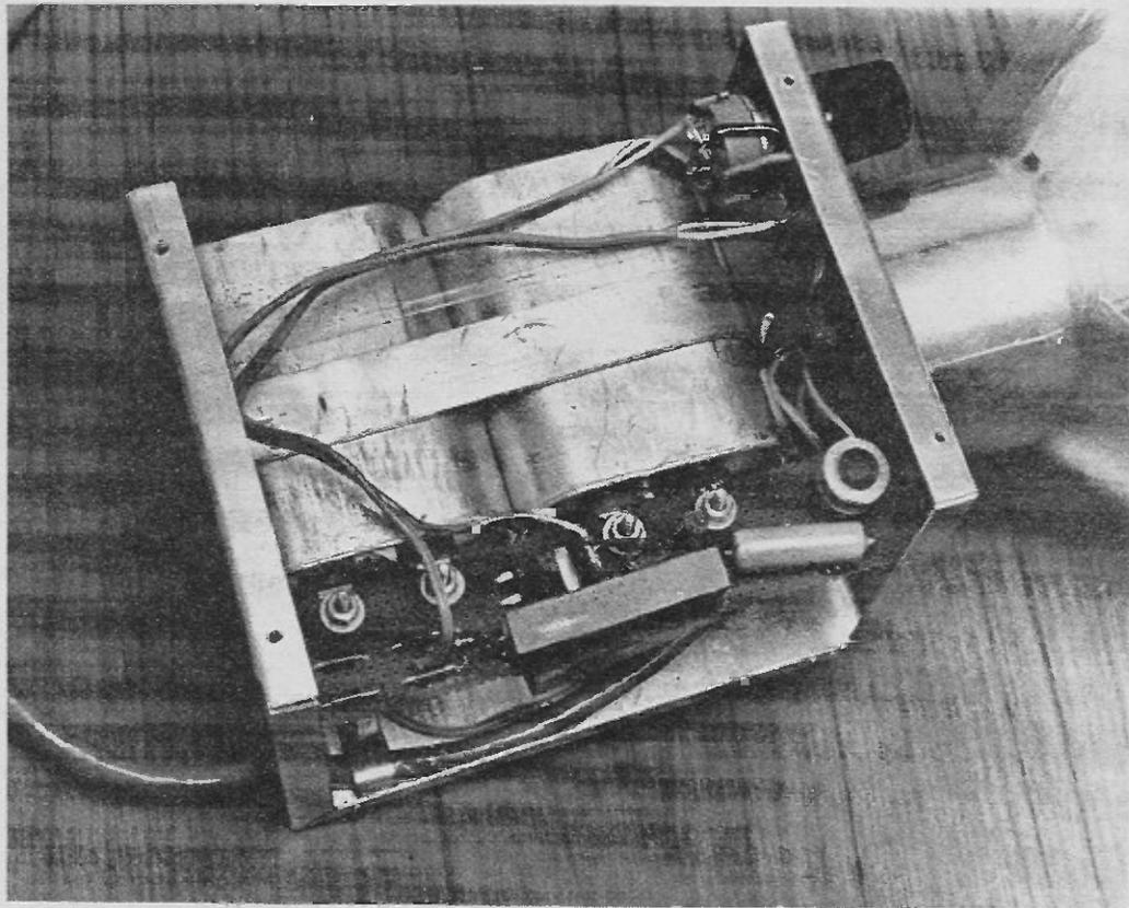
*Fig. 5. Construction of the unit — this particular unit has been constructed to drive two flash-tubes. The additional capacitors and 220 ohm, 10 watt resistor referred to in the text can be clearly seen. The pulse transformer is on the extreme right of the matrix board which in turn is bolted securely to the energy storage capacitors.*
