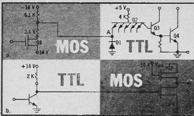
*The best features of differing logic technologies may be utilised in hybrid systems. This article explains how MOS and TTL are interfaced.*
