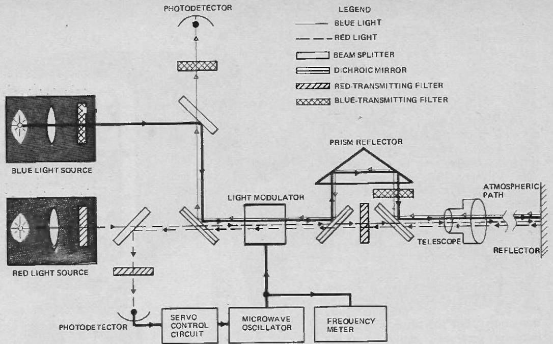
Fig. 13. A schematic of a two-colour distance measuring technique used by ESSA in the United States of America.
