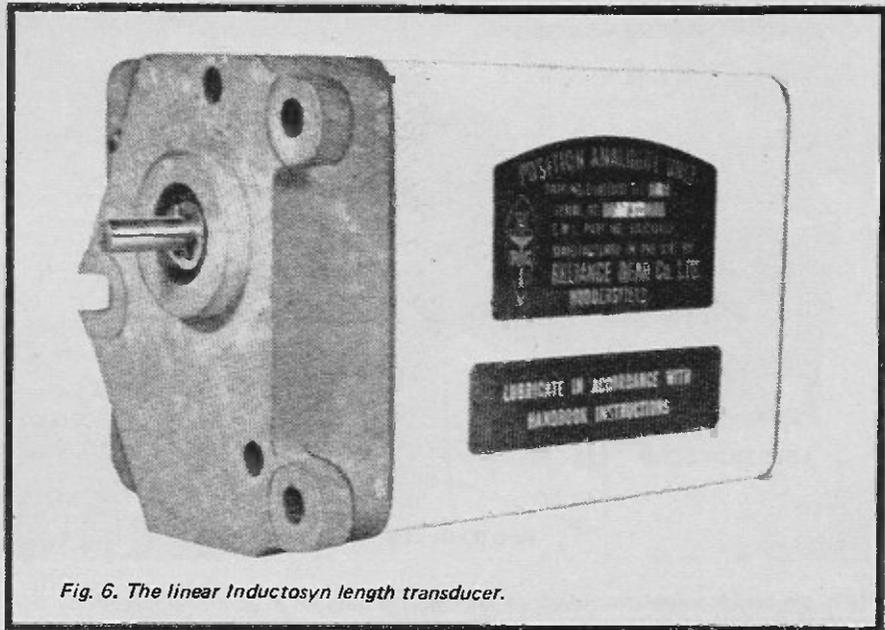
Fig. 6. The linear Inductosyn length transducer.
