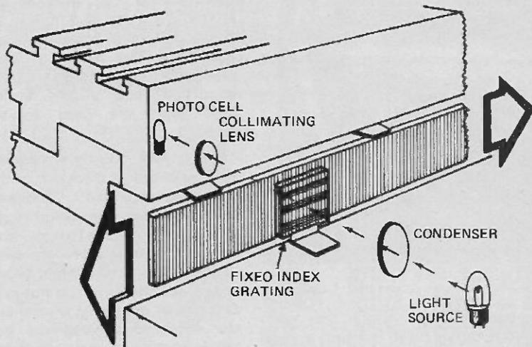
If two diffraction gratings consisting of ruled lines on transparent blanks are superimposed with their rulings not quite parallel to each other, dark bands called moiré fringes are produced across the gratings. The spacing of the fringes is a multiple of the ruling interval and is dependent on the angle of inclination between the two sets of lines.
