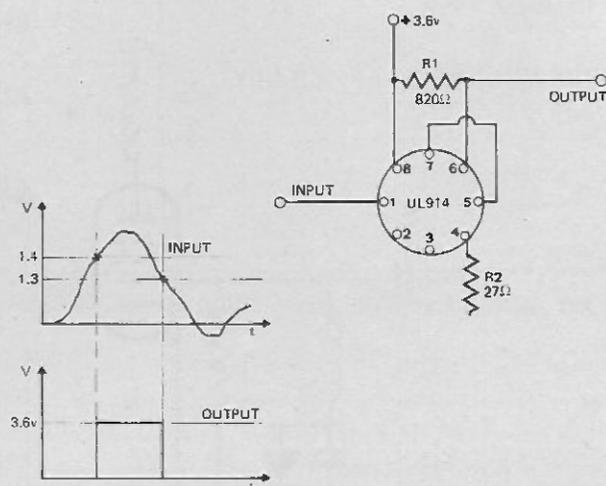
One cheap IC, uL914, can be used as an extremely simple and effective Schmitt trigger suitable for many applications. Hysteresis of the circuit is about 0.1 Volt. This may be varied by altering the values of R1 and R2.
