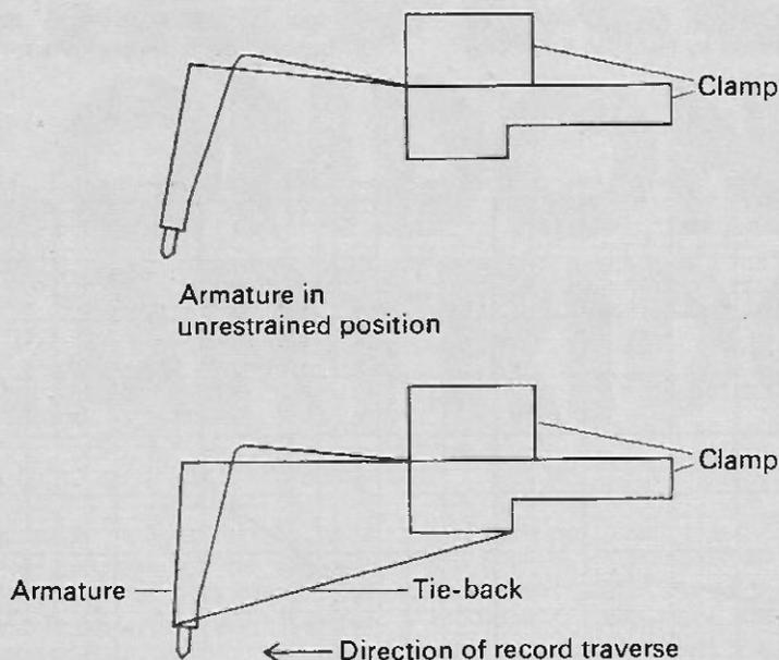
Fig. 2. The stylus and armature are restrained and tensioned by a fine nylon cord.
