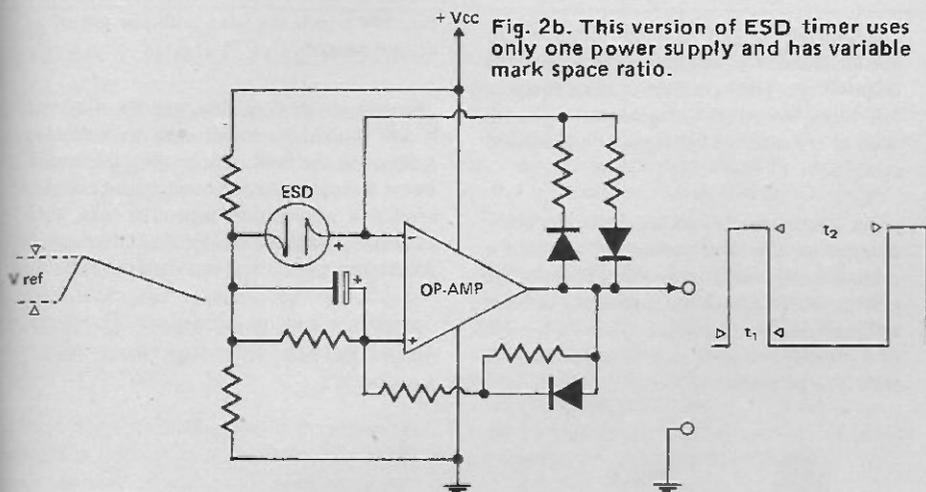
Fig. 2b. This version of ESD timer uses only one power supply and has variable mark space ratio.
