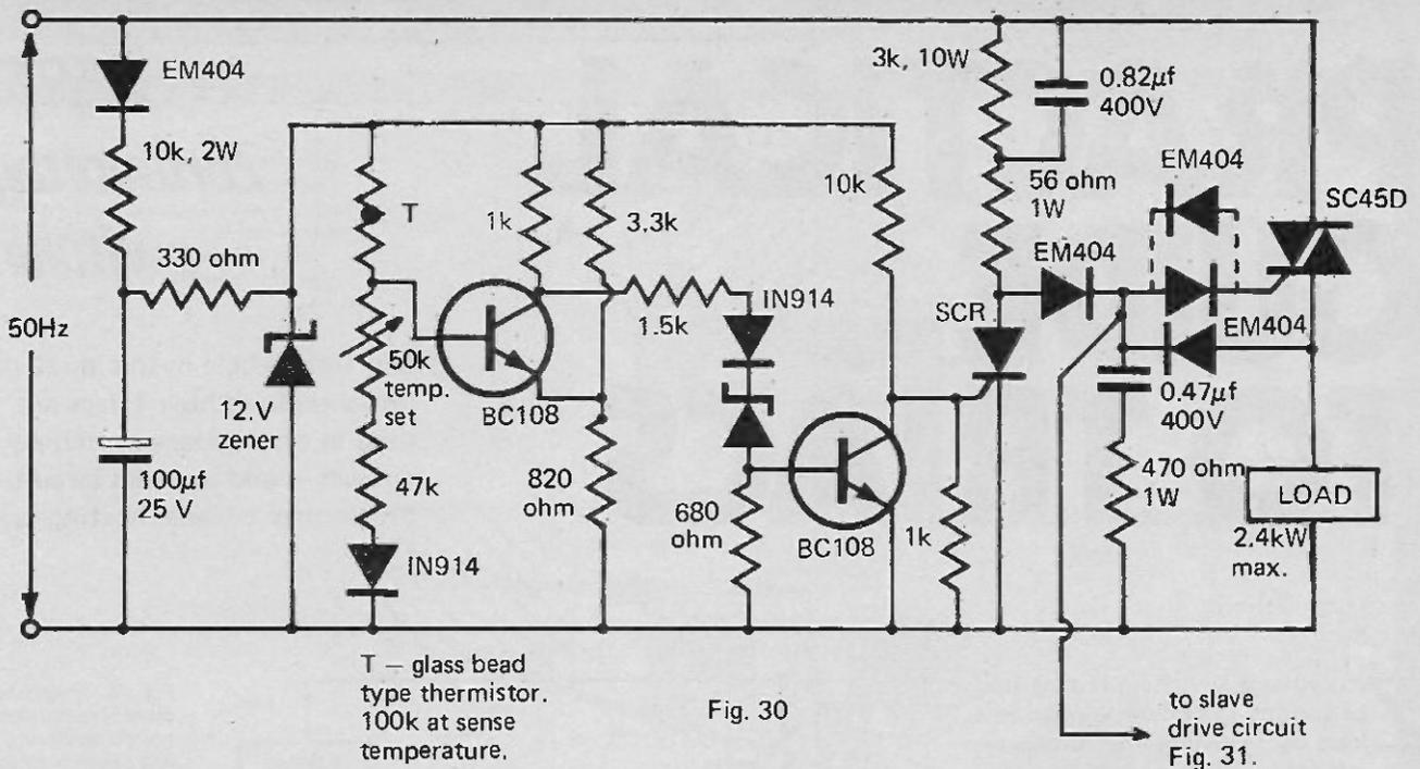
Fig. 30. This circuit can control loads of a size determined only by the rating of the Triac. The slave circuit shown in Fig. 31. can be driven by the output of this circuit if required.
