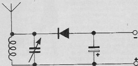
Fig. 8. Simple rf receiver provides 'free' power for implanted bugs.
