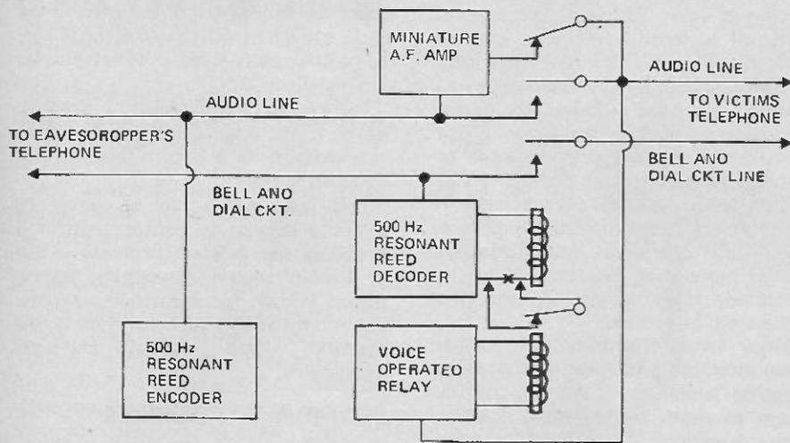
Fig. 5. Block schematic drawing of infinity transmitter. This bug enables an eavesdropper to listen to sounds within a room thousands of miles away.
