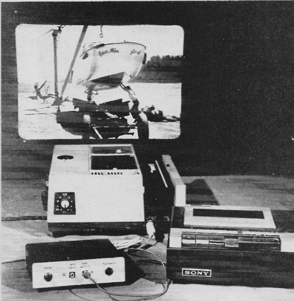
This unit automatically changes slides on an automatic projector. It does this at predetermined times, synchronizing with the commentary prerecorded on a two-channel, cassette or reel-to-reel tape recorder.
