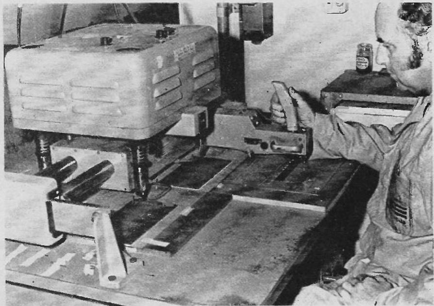
Multiple head machine drills four boards at once.
