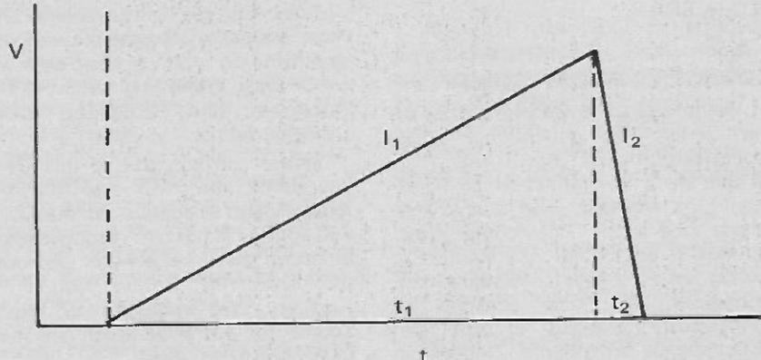
Fig. 1c. ESD timer uses charge and discharge time of device. Short circuit discharge is prevented by current rating of device.
