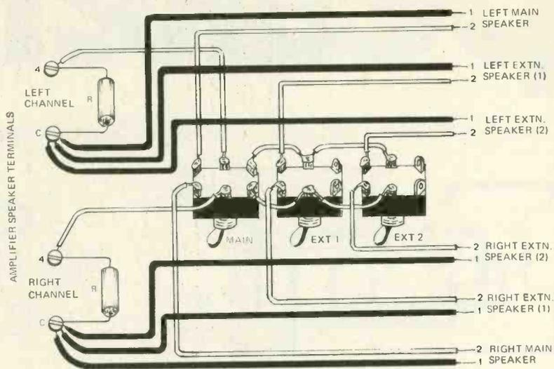
Fig. 4. Four ohm main speakers and two sets of eight ohm extension speakers.
