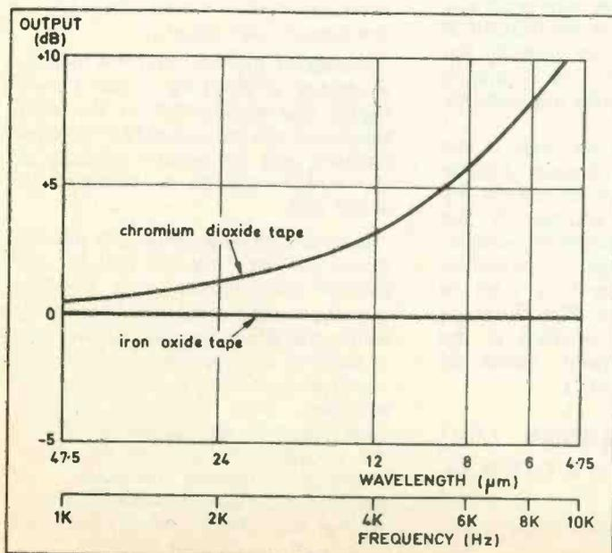
Fig. 3. Comparison of maximum high frequency saturation output of chromium dioxide and iron oxide tape (assumed to be 'flat')
