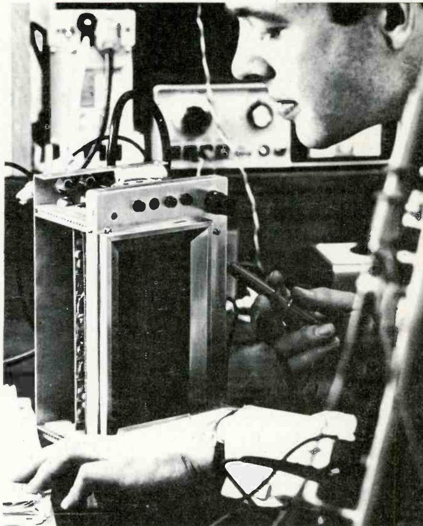
*This new display is based on the use of a matrix of light-emitting diodes and it approaches the very thin, 'picture-on-the-wall', type of display which has always been regarded as the ideal form of display presentation.*
