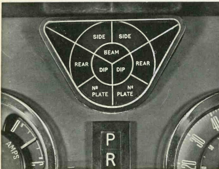
Fig 2 Fibre optic system for monitoring bulb failure by logic group principle (see text)
