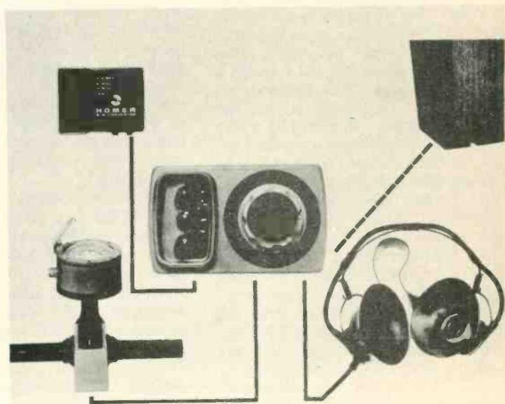
Fig 3 The 'Homer' direction finder equipment from Brookes and Gatehouse Ltd
