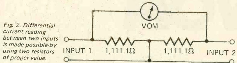
Fig. 2. Differential current reading between two inputs is made possible by using two resistors of proper value.
