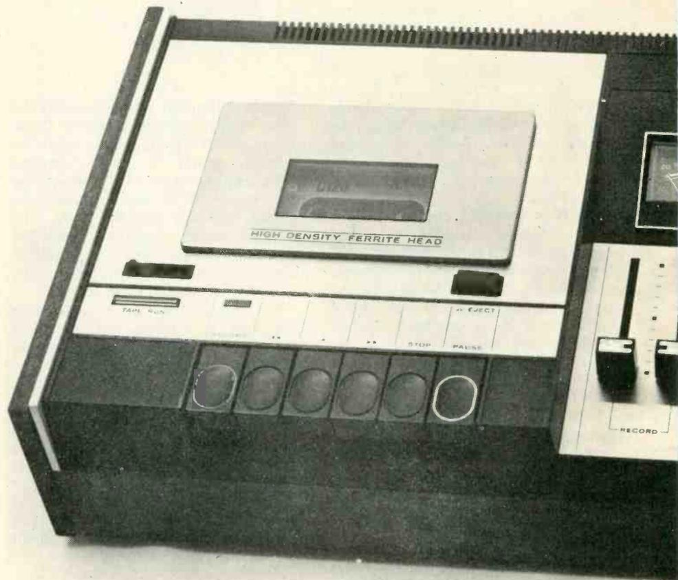
Dolby B) was subsequently developed by Dr. Dolby and this operates on the middle to high frequency part of the audio spectrum, thus removing the tape hiss inherent in the recording process. This system reduces noise by 3 dB at 600 Hz, by 6 dB at 1200 Hz and by 10 dB at 4000 Hz and above — where the ear is most sensitive to hiss.
