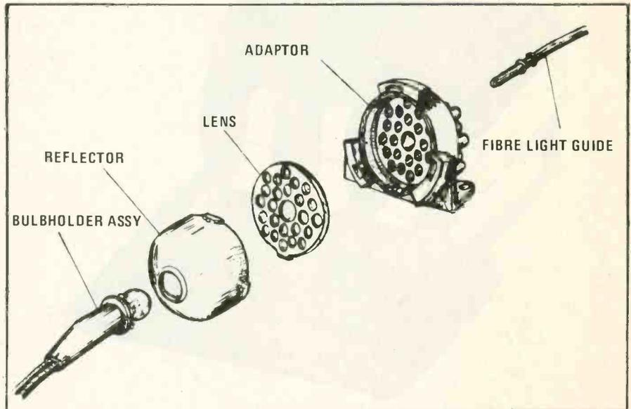
Fig 3 A 27 way central light source divides the illumination from one lamp into 27 fibre light guides which simply plug in to the rear of the adaptor
