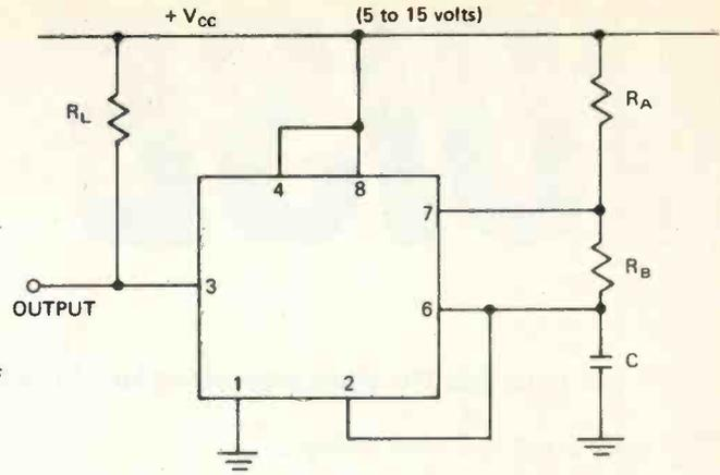
input impedance and consequently has negligible shunting effect across the timing capacitor. Typical component values for a one hour timer are a 10 megohm resistor and a 330µF capacitor.
