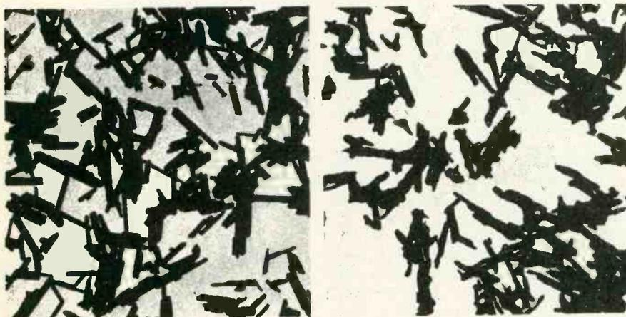
Figs. 1 and 2. Photo-micrographs of chromium dioxide (left) and conventional tape (x20,000)
