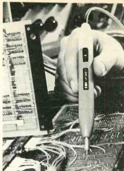
logic 0, open circuit, +ve going pulses, -ve pulses, square waves below 1MHz approx and pulse trains (including square waves) with a pulse recurrence frequency above 1MHz. It can be powered by the equipment under test, from a 4.5V battery or from a standard bench power supply. The device is provided with self-check and is protected against overload from input voltages up to  $\pm 100V$  and supply polarity reversal. (100)
