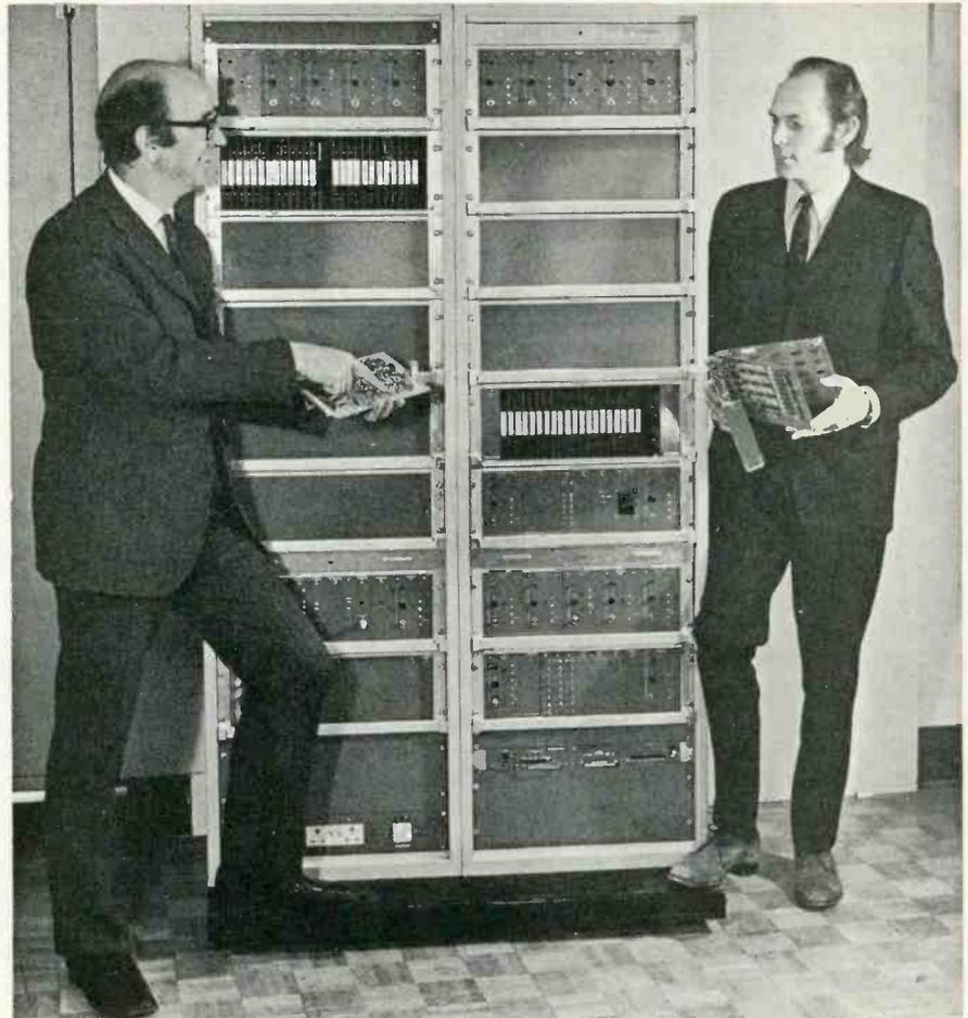
The new IBA Digital Field-rate Television Standards Converter
