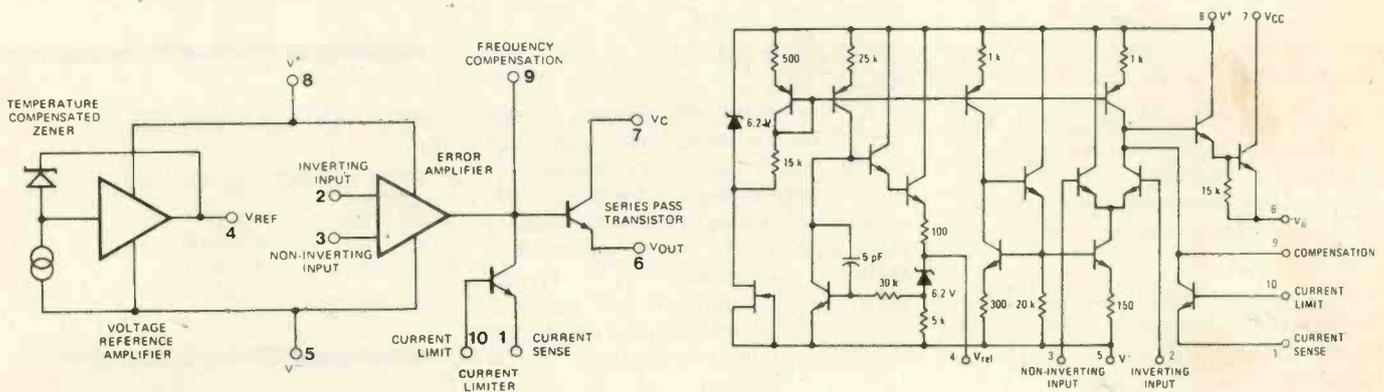
Fig. 2. Simplified schematic of  $\mu A723$ .
