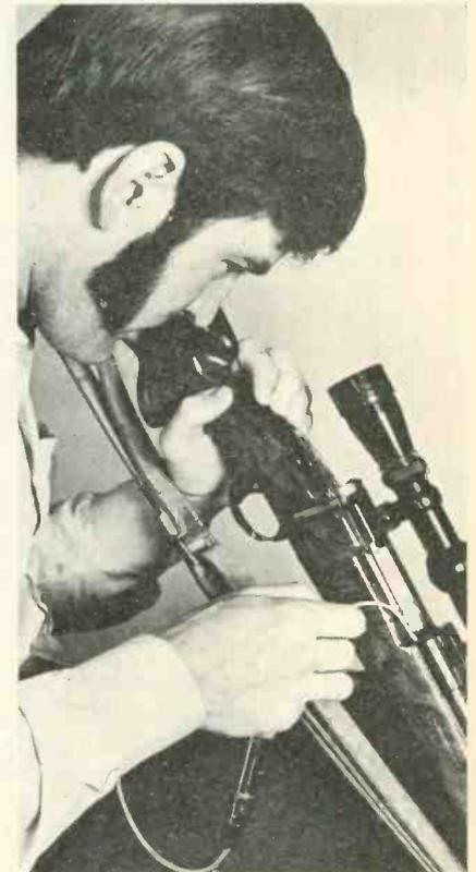
This is neither a scene from "2001" nor a satellite's view of the eye of a hurricane. It's a glimpse down a rifle barrel illuminated at the chamber end by a Corning Flexiflash fibre optic unit. The unit is proving useful for gun enthusiasts in examining rifling, the chamber, the wear in the barrel's throat — all areas that can effect a weapon's accuracy.
