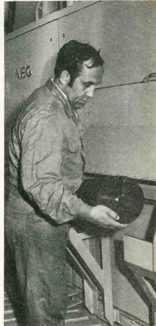
Fig. 2. Removing the fish cylinder from the X-ray treatment plant on-board the ship "Walther Herwig".
