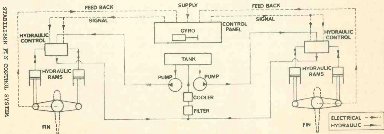
Fig 9 Block diagram of the Vosper Thornycroft stabilizer fin control unit
