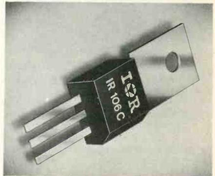
This new miniature low-power Thyristor manufactured using planar techniques, is intended for use in industrial and domestic applications covering heating and lighting controls, automotive appliances, power supplies, meter controls and similar applications.
