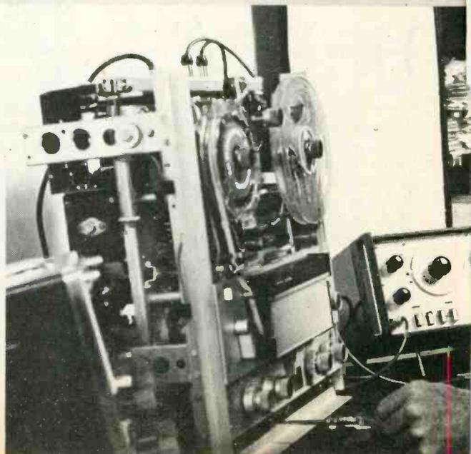
Multi-function test set is specifically intended for tape recorder maintenance and repair
