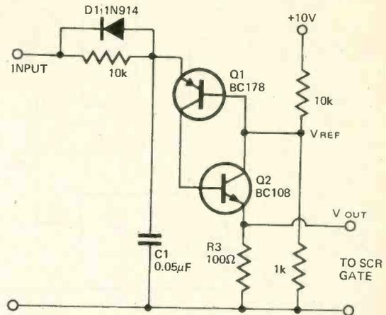
When switching inductive loads, unreliable triggering is sometimes encountered due to feedback of switching transients.
