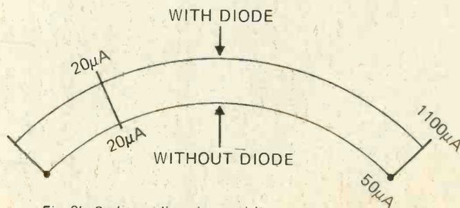
Fig. 3b. Scale non-linearity resulting from circuit of Fig. 3a. Note that low end of scale is linear.
