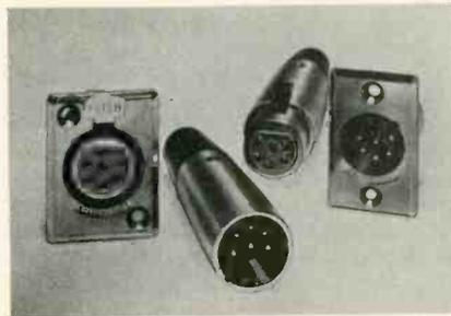
Fully compatible with other leading makes, the Switchcraft audio connector series is said to be particularly suited to critical applications such as microphones, amplifiers, mixers and public address equipment.
