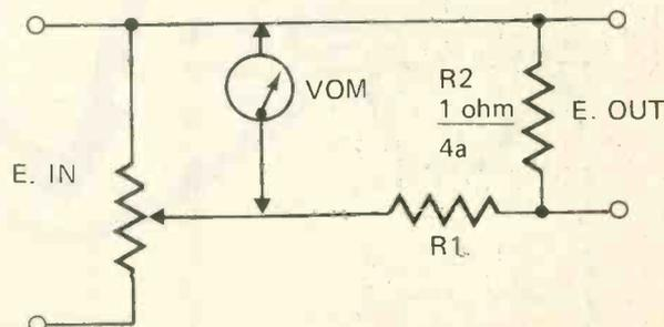
Fig. 6. Microvolt attenuation meter circuit employs voltage divider.
