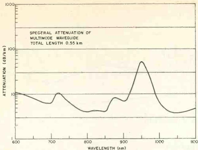
Fig. 1. This graph illustrates the spectral attenuation of a Corning multi-mode waveguide at various frequencies.
