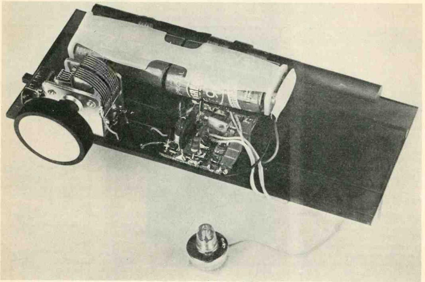
**T**HIS little radio set is an ideal project for the beginner. It draws very little current from the battery, (2 ma) and one set of batteries will drive the radio for months, virtually the normal battery self life.
