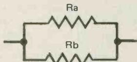
Fig. C. Two resistors in parallel.
