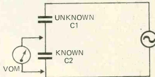
Fig. 4. As a capacitance meter, the VOM measures voltage across known and unknown capacitors.
