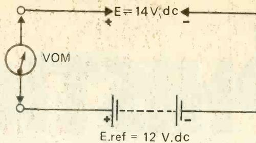
Fig. 1. VOM used as segmental voltmeter. Bucking reference voltage permits accurate reading of small signal variations.
