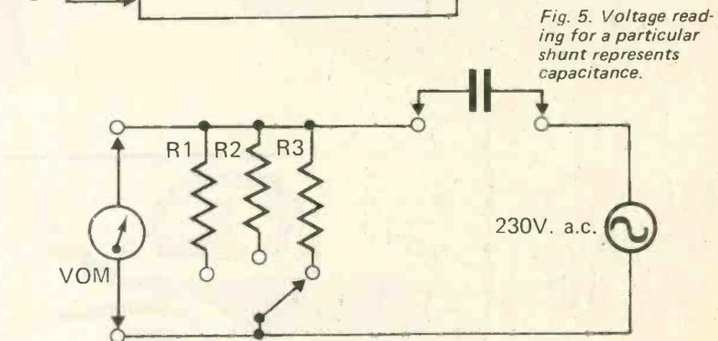
Fig. 5. Voltage reading for a particular shunt represents capacitance.
