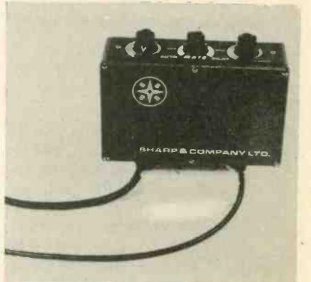
Fig 6 The Sharp and Company autopilot for sail. (a) The wind vane unit (b) This magnetic compass provides a course error voltage (c) The control unit, the motor drive varies according to the boat and is not shown
