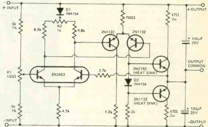
Operational amplifier circuitry requires double-ended power supplies. This simple circuit converts a conventional single ended supply to a double ended operation. Once adjusted, the positive and negative rails will track within a few millivolts without further adjustment.
