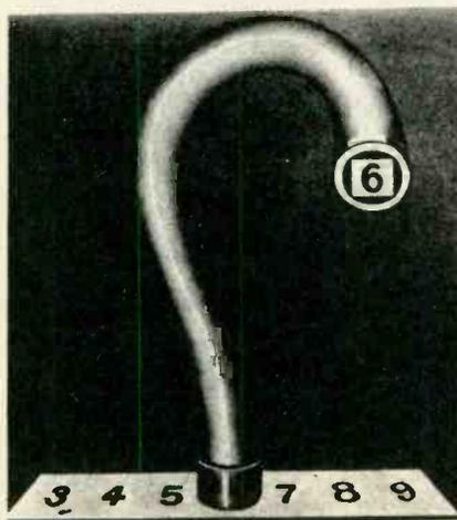
Flexible plastic fibre optics transmits images in full colour. Light loss is 20% per foot plus 10% at each end.
