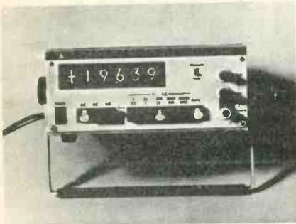
The input arrangement is two terminal floating with guard terminal. Input impedance on the 200mV and 2V dc ranges is said to be greater than 1000Mohm and 10Mohm on the other ranges. A 2Mohm/50pF impedance is offered on the 100mV and 2V ac ranges and 1Mohm/25pF on the higher ranges.
