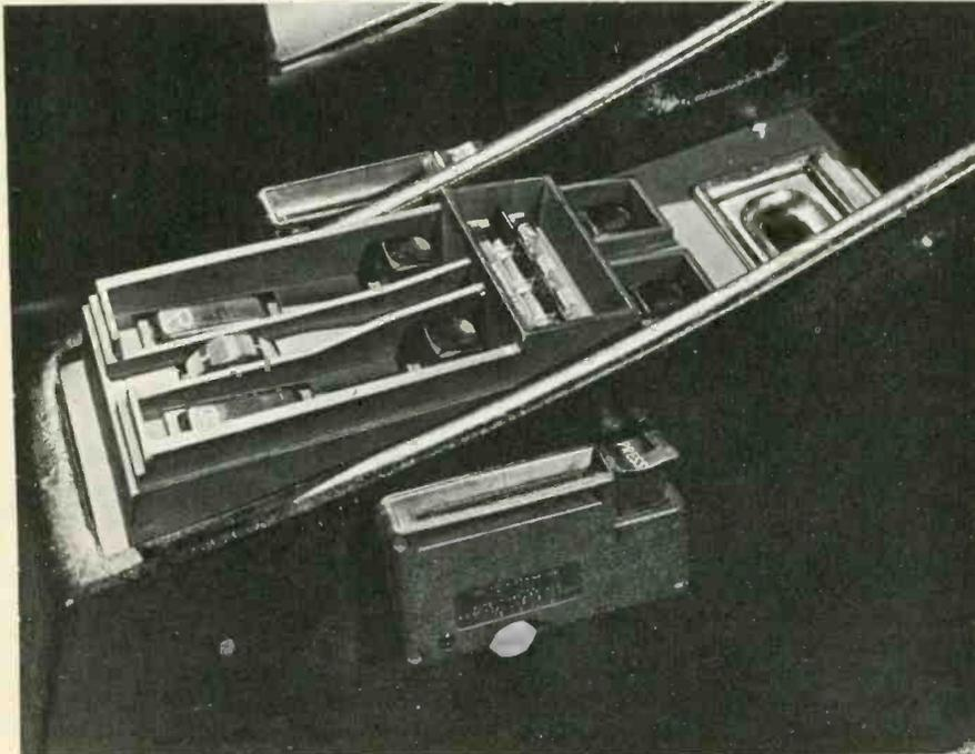
Fig 1 The centre console of the Lucas simulated vehicle which incorporates fibre-optic illuminated controls
