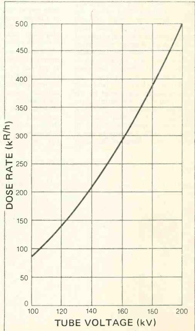
Fig. 6. Dose rate in the centre of the irradiation chamber (with a tube current of 32 mA).
