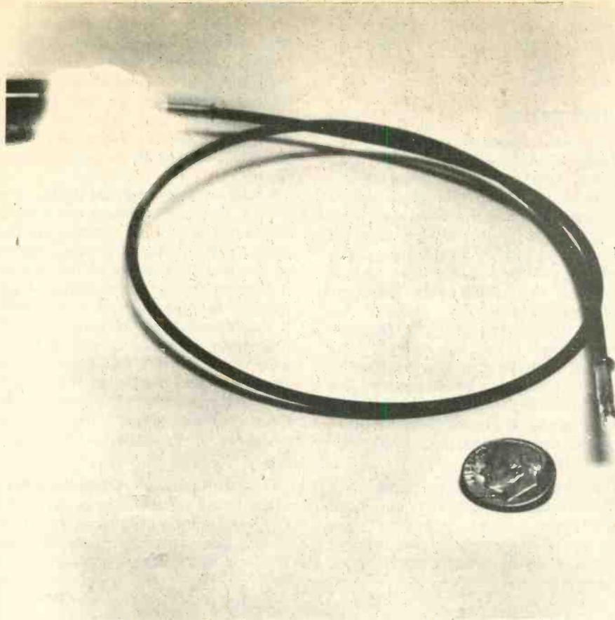
filament. In addition, a SELFOC filament produces no phase differences during transmission. The phase of the exit signal is the same as the entering signal.
