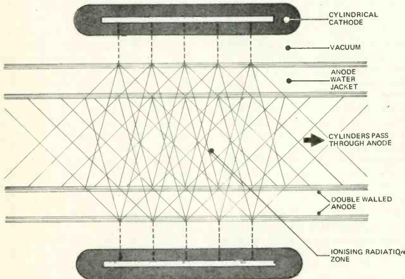
Fig. 3. Diagrammatic layout of the cylindrical X-ray tube.
