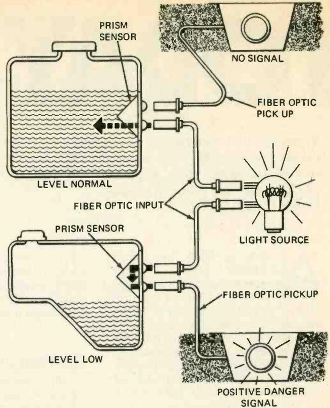
Fig. 3. Fibre-optic system provides isolation between receiver and transmitter.
