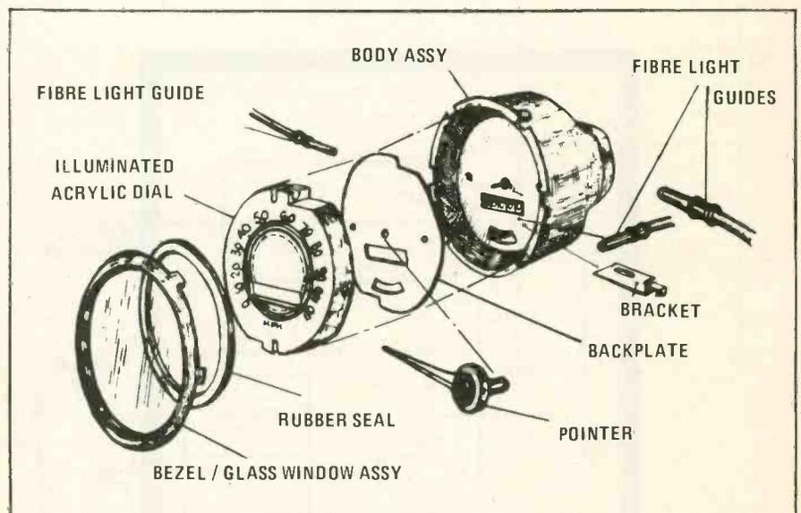
Fig 4 The method of inserting fibre light-guides into a speedometer is typical of all instruments. One guide illuminates the acrylic dial and others are used for the mileage counter etc
