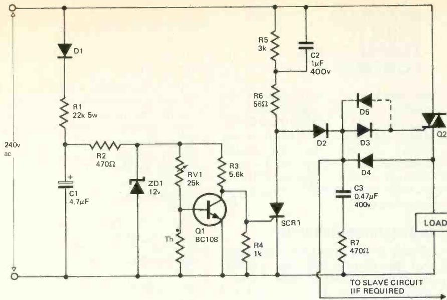
diode ZD1 provide a regulated dc power supply for the sensing circuit consisting of the thermistor (Th), R3, D2 and 'temperature set' potentiometer RV1. Power is also supplied by this circuit to transistor Q1 and Q2.
