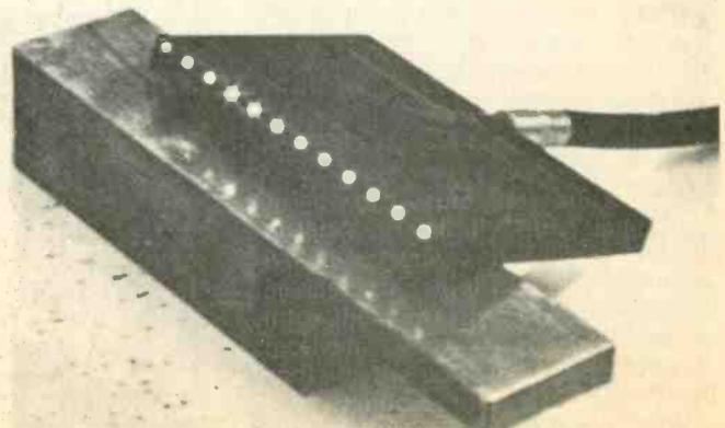
*Single light source is a feature of this punched-card reader. Light shines on far end of 12-branch fibre-optics light guide.*
