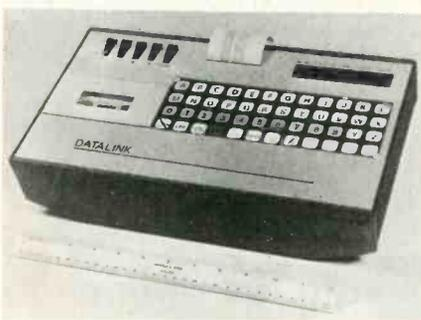
errors has been made extremely remote through self-intelligent electronic circuits which check commands from the internal store, on a write-read principle on tape, before the command to print is given.
