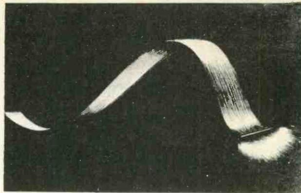
As early as 1870, the British physicist John Tyndall demonstrated that light could be made to follow a curved path. He directed a light into a tank of water, from which a stream flowed through a hole punched in the side of the tank.
