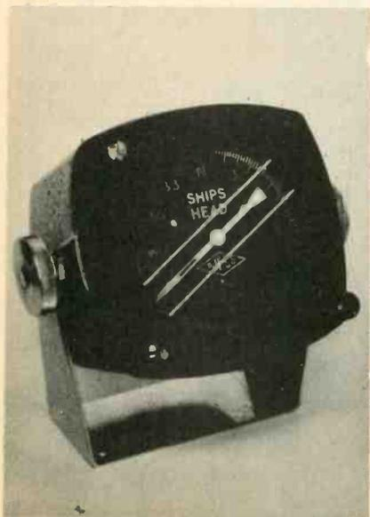
Fig 1b Repeater compass in free standing housing by Neco Pty Ltd
