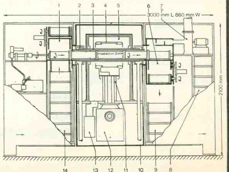
Fig. 4. Cross sectional view of the shipboard installation using the flow-through anode configuration.
