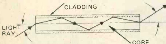
The amount of light transmitted depends upon (a) the intensity of the light source, (b) the loss characteristics of the cladding and core structures, (c) the length of fibre and the number of fibres per bundle.
