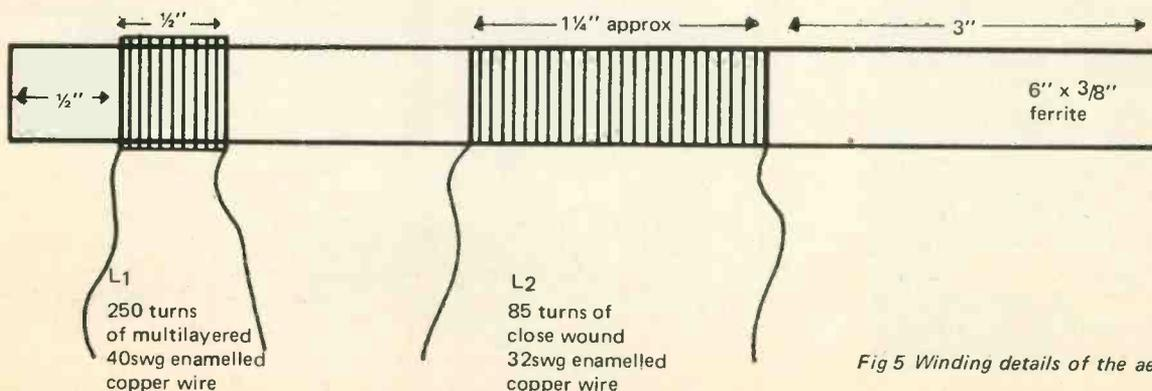
Fig 5 Winding details of the aerial coil
