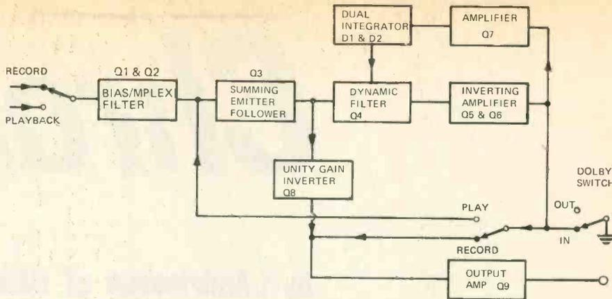
Fig. 3. Block schematic shows the operating principle of the Dolby (B) system.
