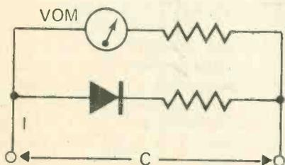
Fig. 3a. Wide range ammeter circuit uses diode to shunt current past VOM at high values of current.
