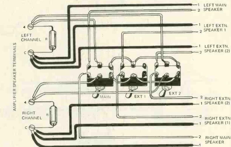
Fig. 5. Eight ohm main speakers and two pairs of eight ohm extension speakers.
