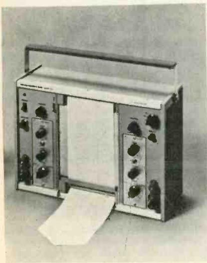
The Mini-writer is suitable for horizontal or vertical use and can be rack mounted.
