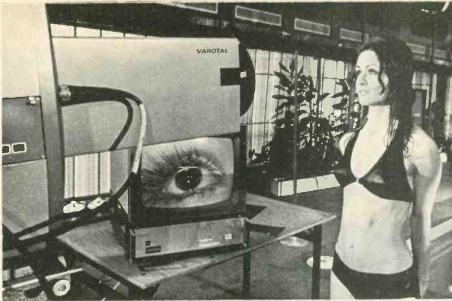
Orders worth £¼ million have been received by Rank Precision Industries for this new Varotal colour TV lens, including £180,000 from USA and Europe. The BBC have just ordered three at a cost of £15,000. It enables a single camera to vary the picture on the screen from a panoramic view of a swimming pool to a magnified close-up of an eye. The eye on this monitor screen belongs to model Sandra Brown of Leicester.
