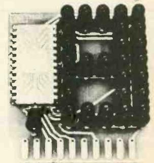
Using discrete solid-state light emitting diodes, this new display from Hewlett Packard is readable up to 60ft away.
