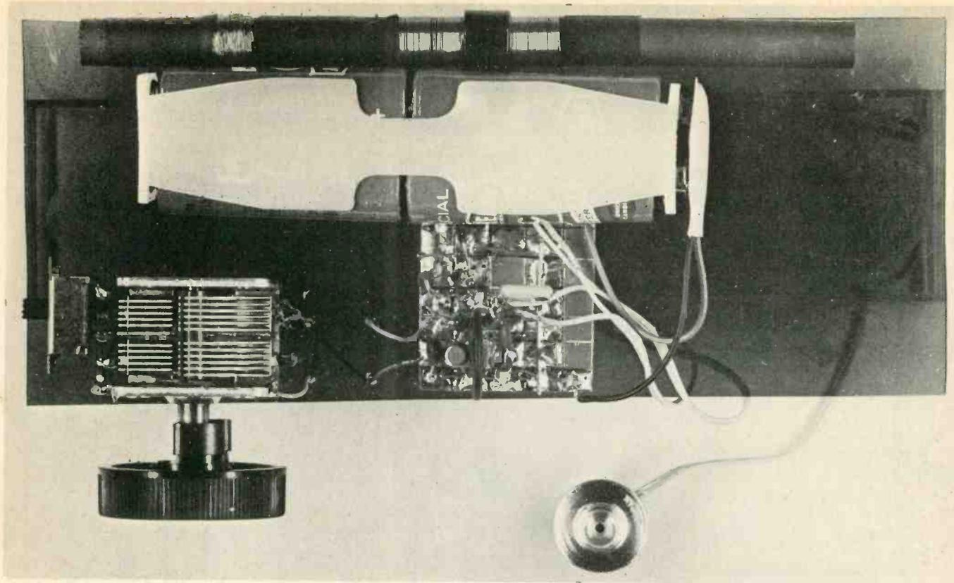
Fig 4 Layout of our prototype receiver. Note position of wave change switch to left of tuning gang
