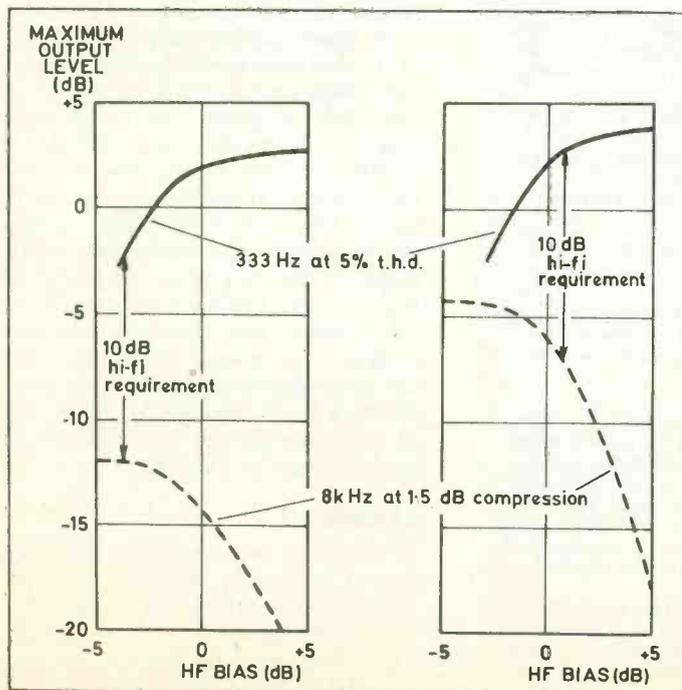
Figs 5 and 6. Comparison of MOL curves at 333 Hz and 8,000 Hz as a function of bias for conventional tape (left) and chromium dioxide (right).
