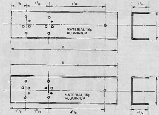
Drilling details of ITT box lid and associated heat sinks
