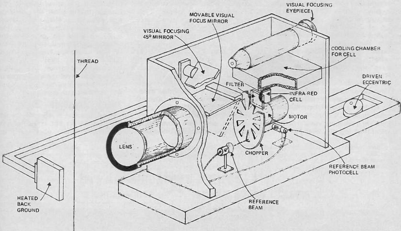
Fig. 3. Schematic of the I.C.I. nylon thread non-contact thermometer.
