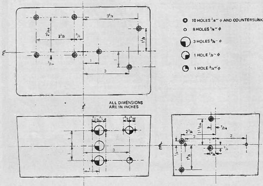
Countersunk screws and spacers are used to ensure that the printed circuit board stands well clear of inner face of the lid. These should be installed at this stage — but do not yet attach the board itself.
