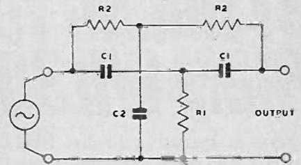
$$f = \frac{1}{2\pi C_1 R_2} \quad R_2 = 2R_1 \quad C_2 = 2C_1$$
