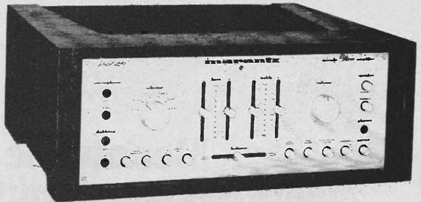
Latest amplifier from Marantz has 120 watts output per channel.
