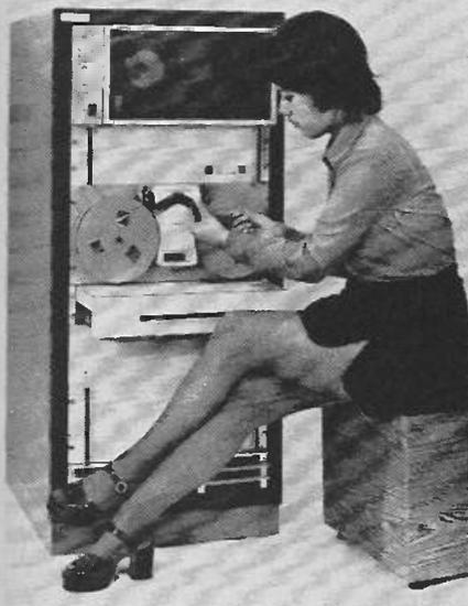
The System 2001 uses a Tally high speed paper tape reader to input data to the Kennedy Magnetic Tape unit at a speed of 500 characters/second.
