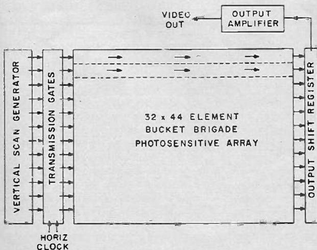
Fig 3 - Block diagram of a BBD charge-transfer sensor
