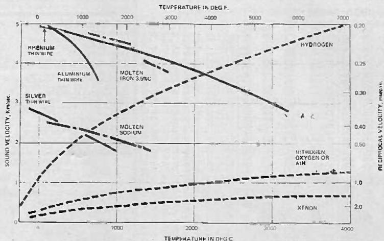
Fig. 9. Propagation velocities of sound in various selected media.
