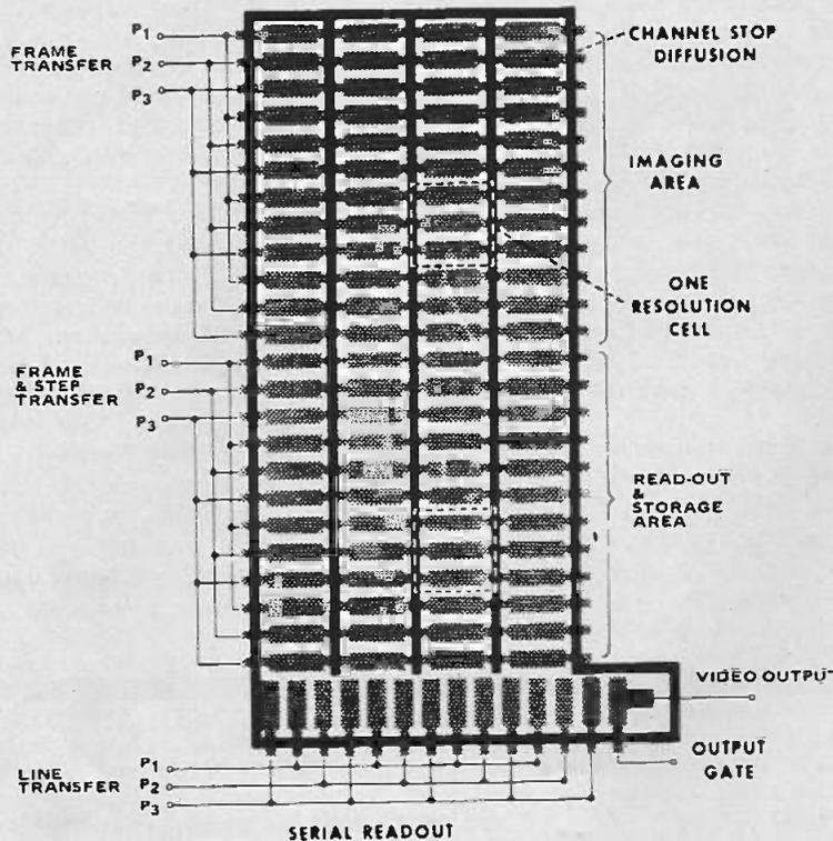
Fig 5 - Frame transfer principle in Bell's CCD sensor
