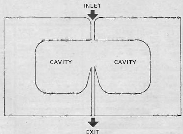
Fig. 10. Cross-section through a resonant fluidic temperature sensing cavity.
