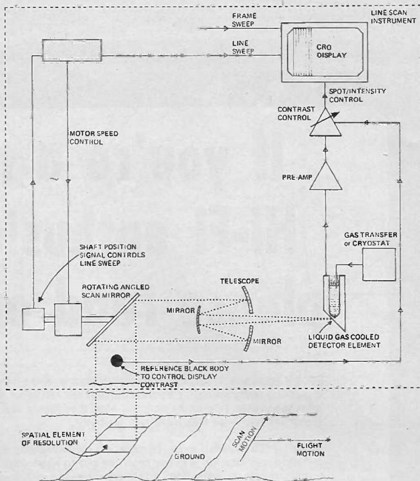
Fig. 6. Schematic of airborne thermal scanning apparatus used in remote sensing for civil and military purposes.
