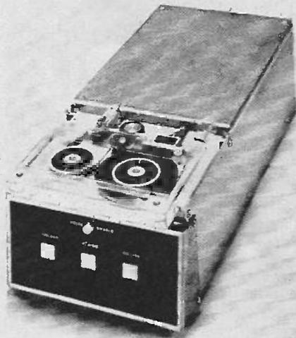
The tape drive on Model 330 is fully bi-directional at 25 ips normal speed, resulting in a data transfer rate of 40,000 bits/second at 1600 cpi recording density it is claimed. Forward and reverse search modes, as well as rewind speed, are 90 ips. With 300 feet of high grade 0.25" one mil tape, total data capacity (gapless) is  $23 \times 10^6$  bits for 4-track operation. Model 330 meets the proposed ANSI standard it is claimed.
