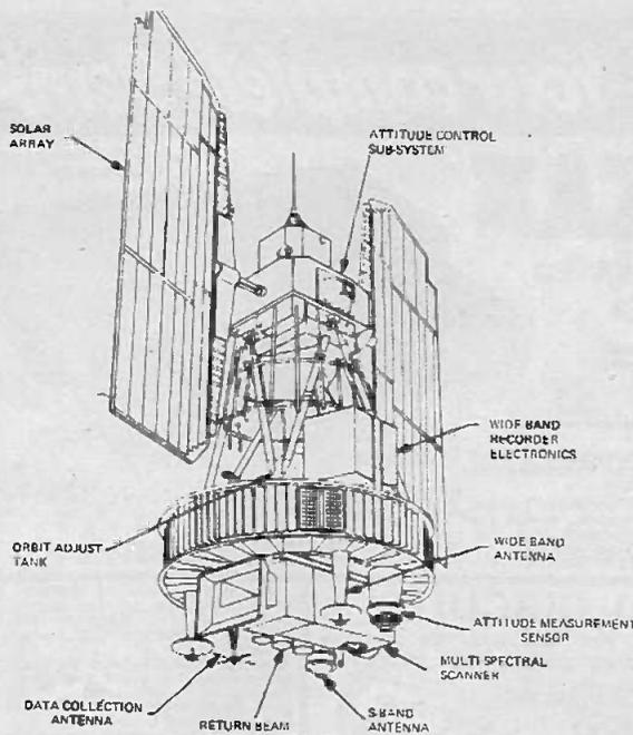
Fig. 8. The ERTS satellite currently orbiting the Earth to provide thermal emission data over long periods.
