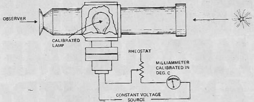
Fig. 2. The basic disappearing-filament optical pyrometer — the rheostat is adjusted until the light filament just disappears. Temperature is read from the dial.
