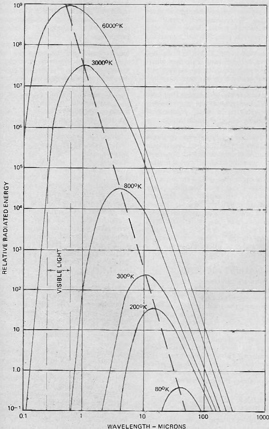
Fig. 1. Distribution of black body radiation as temperature varies. The total energy radiated at a particular temperature is represented as the area under the curve for each.
