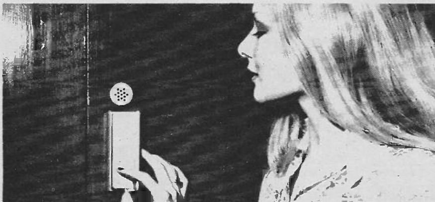
float-charged from the mains so that should the main supply at any time be cut off the battery will take over the operation of the whole system. Also, as an additional security, if anybody tampers with the finger-plate by trying to cut the wire an alarm will sound. A special high security electric lock completes the system. Manufacturers are J. Donne Holdings Ltd., Canberra House, 312-319 Regent Street, London W1R 57B.
