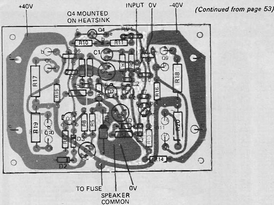
Fig. 3. How the components are mounted on the printed circuit board.
