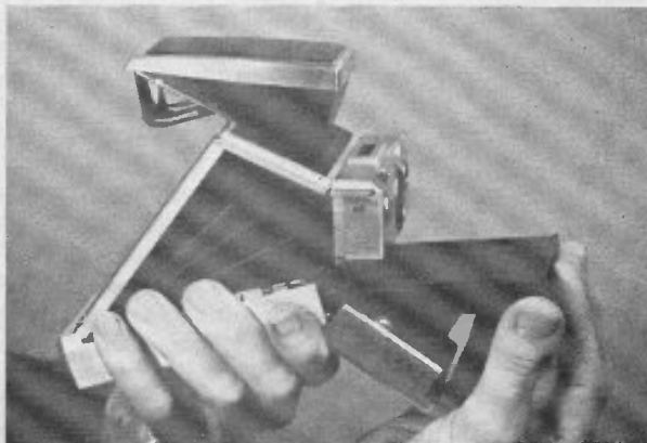
Fig. 15. The solid state module and the printed circuit card shown in the relative positions they occupy in the camera.
