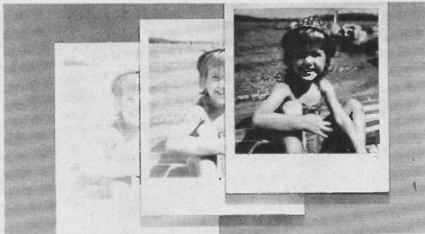
Fig. 17. A print from the SX 70 as it appears during the development phase which takes 10 minutes.
