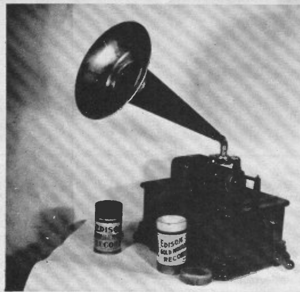
Edison "Standard" Phonograph, one of the most popular record players of early times. This 1909 model featured a turnover stylus for playing either normal two minute or the finer grooved "Amberol" 4 minute cylinders.
