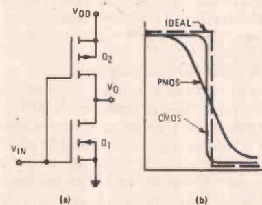
Fig. 9. Typical inverter circuit with P and N-channel MOSFETs connected in complementary symmetry. (a) Characteristic curves. (b) CMOS curve closely approaches ideal switch.
