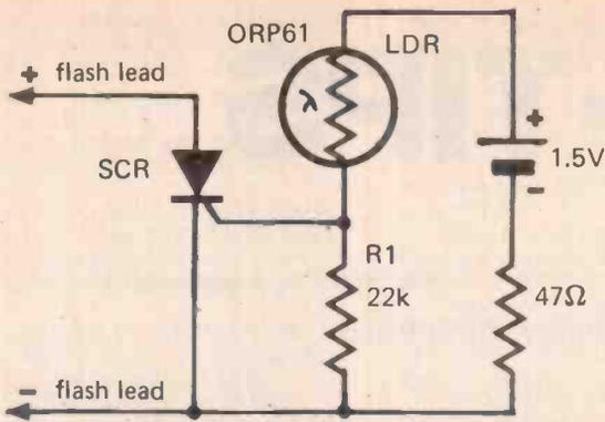
In photography, a separate flash, triggered by the light of a master flash light, is often required to provide more light, fill-in shadows etc.
