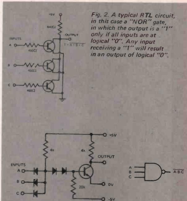
*Fig. 2. A typical RTL circuit, in this case a "NOR" gate, in which the output is a "1" only if all inputs are at logical "0". Any input receiving a "1" will result in an output of logical "0".*
