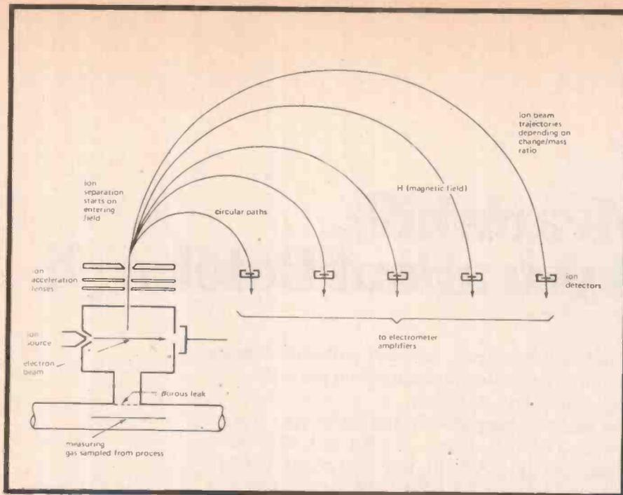
Fig. 5. In the mass spectrometer, ionised gas atoms and molecules are separated into groups depending on their electron-charge/mass ratio.
