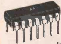
From Motorola, a monolithic dual stereo preamplifier for low noise preamplification of stereo audio signals. Just look at some of these features:
