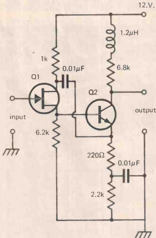
This circuit has a typical gain of 10dB and bandwidth of 90 MHz.
