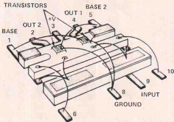
*Fig. 1. The first integrated circuit developed by Texas Instruments in 1959 used the "mesa" process. The device is a flip-flop and was the forerunner of the Resistor-Transistor Logic family.*
