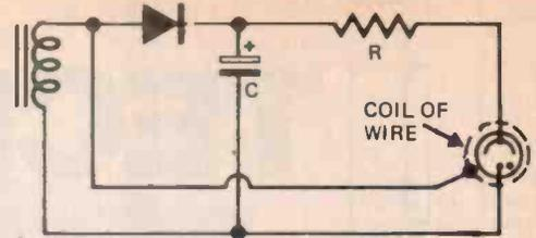
In some applications, VR tubes prove reluctant starters. This can often be overcome by wrapping a coil of insulated wire around the tube and then connecting it to the high voltage ac side of the supply.
