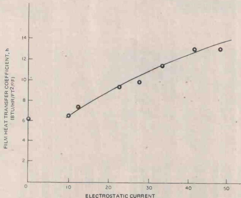
Fig. 3. Electrostatic cooling depends strongly on the current flow. Here, cooling of an Irttran-2 element with a needle probe begins at 10  $\mu$ A.
