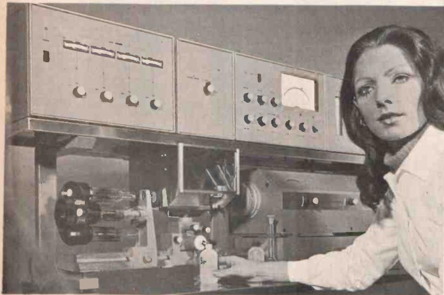
Fig. 8. An atomic-absorption flame spectrophotometer.
