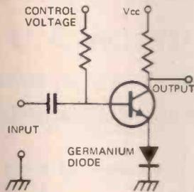
In this circuit a germanium diode is used to effect gain control of a common-emitter amplifier.
