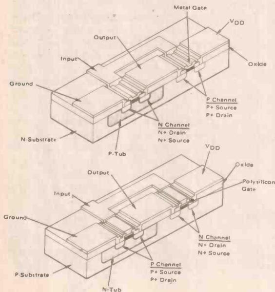
Fig. 7. Two basic processes of CMOS fabrication
