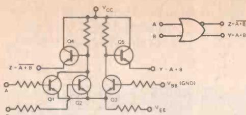
Fig. 5. The basic ECL gate configuration. High-speed performance results from the non-saturation operation of high  $f_T$  transistor current switches.
