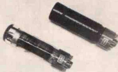
Illustrated are just two examples of EMI's 50mm diameter fast photomultiplier tubes. On the left, is shown a tube prior to receiving its conductive coating which forms an electrostatic screen. The tube on the right is shown after it has been coated and covered
