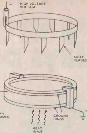
Fig. 2. Best electrostatic cooling of the Irttran window was obtained as shown above.
