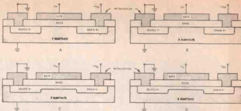
Fig. 6. (A) N-channel MOSFET in the "OFF" condition. (B) P-channel MOSFET in the "OFF" condition. (C) N-channel MOSFET in the "ON" condition. (D) P-channel MOSFET in the "ON" condition.
