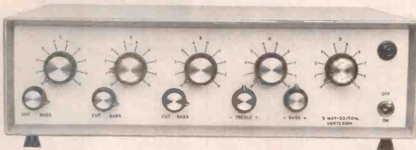
THIS is a high fidelity amplifier with bass cut controls on each of the three low impedance balanced line microphone stages and a high impedance (1.5 meg.) gram stage with bass and treble controls, plus the usual line or tape input. All the input stages are protected against overload by back to back low self capacity diodes and all use F.E.T.s for low noise, low intermodulation distortion and freedom from radio breakthrough.
