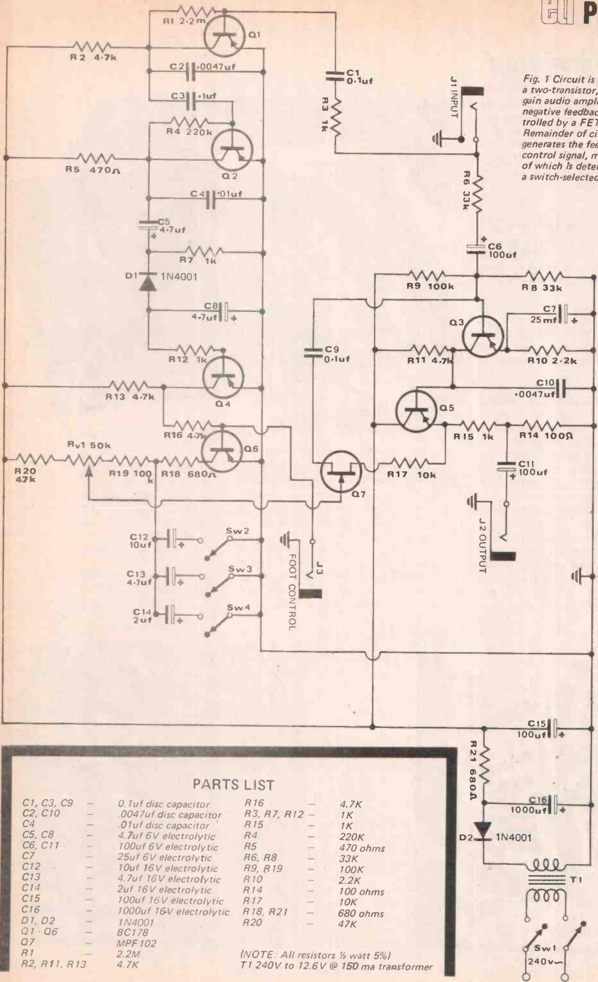
Fig. 1 Circuit is essentially a two-transistor, high gain audio amplifier with negative feedback controlled by a FET. Remainder of circuit generates the feedback control signal, magnitude of which is determined by a switch-selected capacitor.
