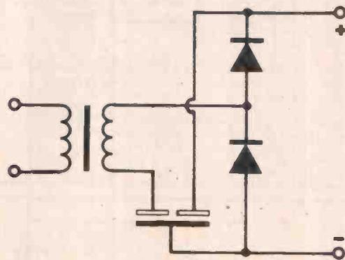
Twin electrolytic capacitors take up less space than two separate units but cannot normally be used in voltage doubler circuits.
