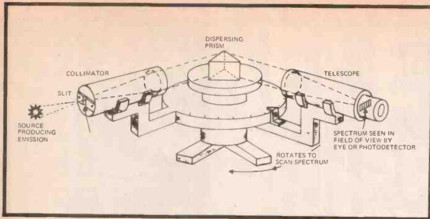
Fig. 6. In the optical spectrometer radiation from a gaseous source is dispersed to form a spectrum of lines and bands unique to each element.
