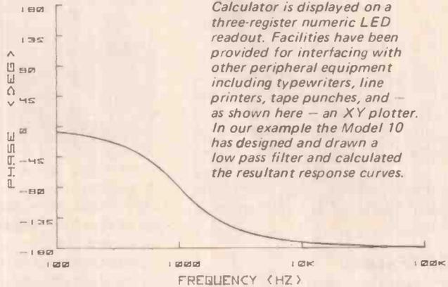
*Data from the Model 10 Calculator is displayed on a three-register numeric LED readout. Facilities have been provided for interfacing with other peripheral equipment including typewriters, line printers, tape punches, and — as shown here — an XY plotter. In our example the Model 10 has designed and drawn a low pass filter and calculated the resultant response curves.*
