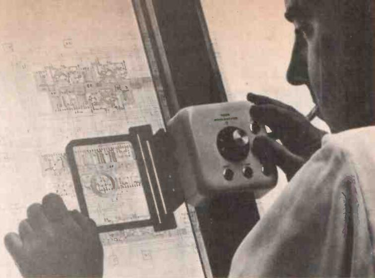
Layout of CMOS process masks is considerably enhanced by this coordinate digitizer machine. It is a convenient, efficient method for converting the designer's signal routing plan into data that a computer can understand and follow.
