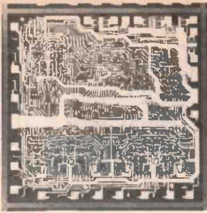
An example of emitter-coupled logic (ECL) large-scale integration (LSI) from Motorola. The device is the MC 10181, a 4 bit Arithmetic Logic Unit/function generator housed in a 24 pin DIL package.
