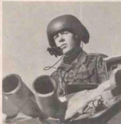
personal communications centres. It has its own built-in facility using either a throat or boom mike as well as having a patented 'acoustic valve' which allows the wearer to hear airborne sounds without the need to remove the helmet and yet still provides a substantial acoustic protection against unexpected explosive sounds.
