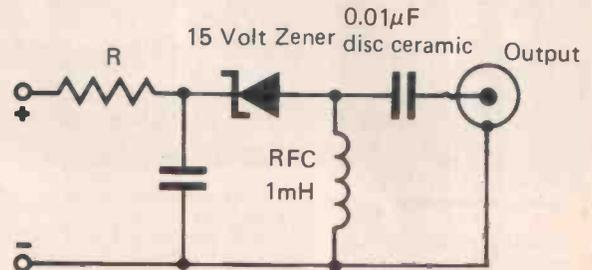
Zener diodes generate substantial amounts of internal noise. The level of this is typically 30 dB above thermal noise at frequencies up to 150 MHz.
