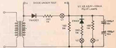
A simple unit for checking diode condition is shown above.
