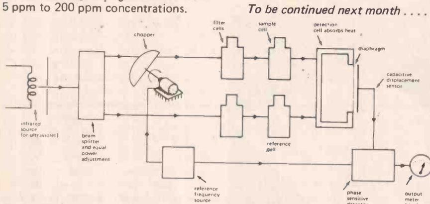
Fig. 10. The principle of the non-dispersive absorption analyser. The source is either in the infrared (the NDIR instrument) or in the ultraviolet region.
