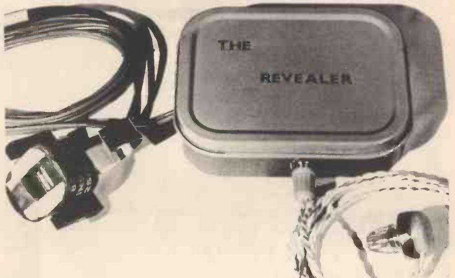
Fig 1. The completed unit together with earpiece and search coil.
