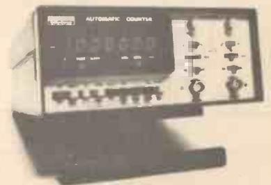
The new 2600 series of frequency counter timers are built on a basic unit with one 50MHz module allowing direct frequency and multiple period measurements with 30mV sensitivity. With the addition of a further 50MHz module time interval measurements can be taken with 100ns resolution. The third variation uses a 50MHz module plus a 520MHz module to give high frequency measurement with 50mV sensitivity.
