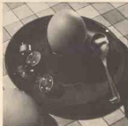
The microminiature motor measures only 13mm x 19mm (approx), has good low noise characteristics and will give long and reliable service even in ambient temperatures as high as 85°C. It is designed to operate at 375 r.p.m. at 50Hz, delivering 0.8g cm at spindle speed with a power consumption of 200 mW.
