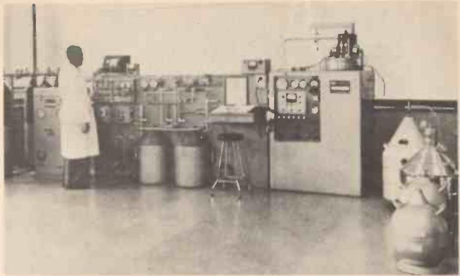
Fig. 6. Helium liquefier plant. Helium is recovered from experiments. Note the dewars on the right.
