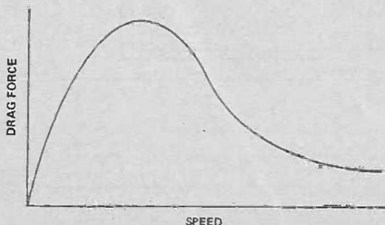
Fig. 12: Speed-drag curve of a superconducting levitating magnet.
