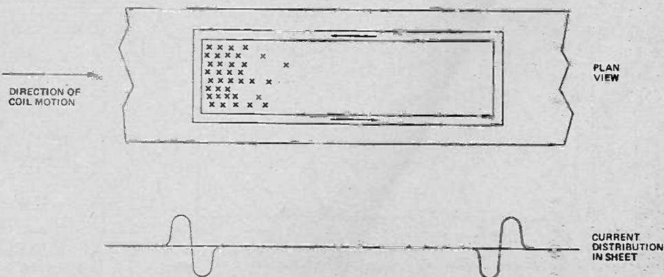
Fig. 10: Flux distribution from an induced electromotive force due to a large rectangular coil moving over a conducting sheet.
