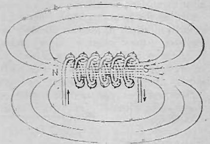
Fig. 7a. The basic inductor is merely a wire with current flowing through it.
