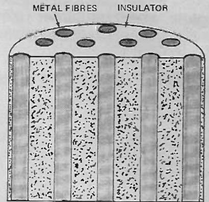
OXIDE-METAL COMPOSITE MATERIAL FOR FIELD EFFECT TRANSMISSION
