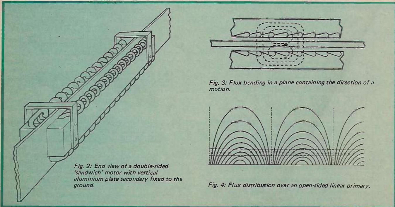
Fig. 2: End view of a double-sided 'sandwich' motor with vertical aluminium plate secondary fixed to the ground.
