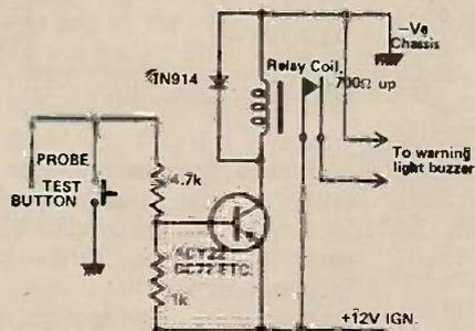
A simple circuit is shown for indicating a drop in radiator coolant level. A variety of transistors and relays can be used and the probe can be made quite easily. The coolant and anti-freeze resistance to earth is about  $100\Omega$  and with the level below the probe, infinity.
