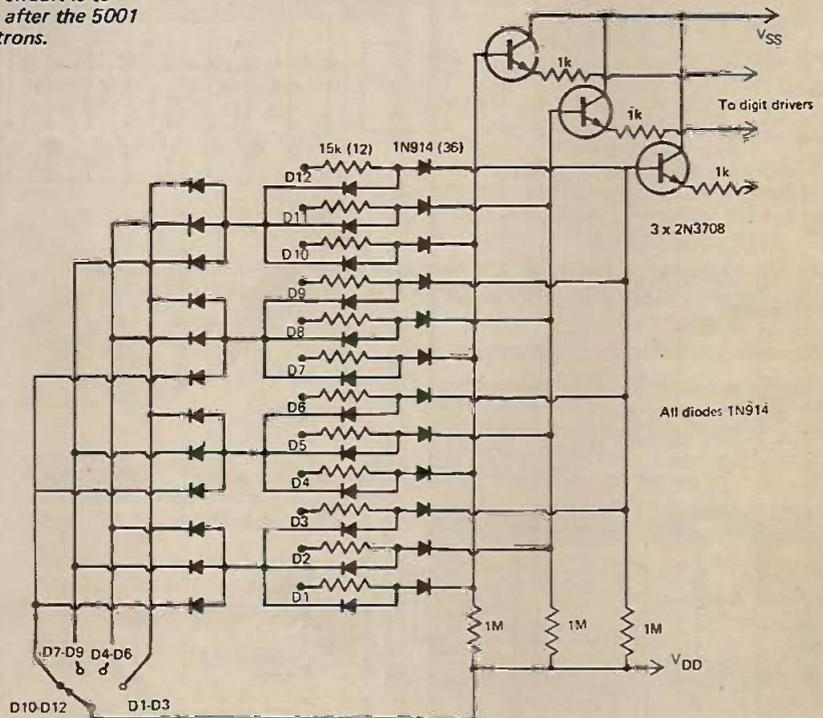
Fig. 6. Digit switching circuit. If wired up as shown, the display is similar to that of the Sharp calculator: only three digits are used and the 12 digit number is viewed three at a time. Variations are 4 at a time or 6 at a time. This applies to both LEDs and Minitrons.
