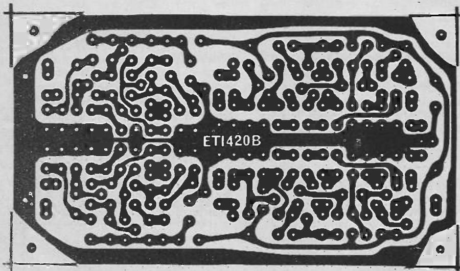
Fig. 2. Printed circuit board pattern for the preamplifier.
