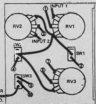
Fig. 4. Wiring to potentiometers and switches — external input module.
