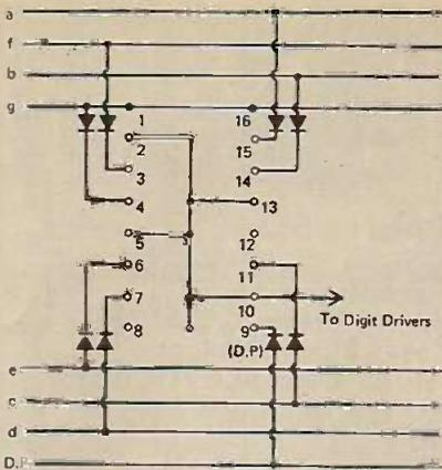
Fig. 5. Connections for Minitrons. All diodes are 1N914 or similar. Connections to LEDs are the same but the diodes are not required.
