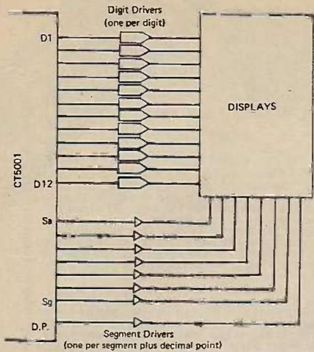
Fig. 3. Basic arrangement for the display.
