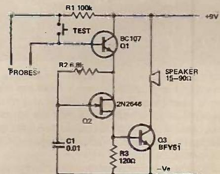
The disadvantage with battery operated alarm circuits is the quiescent current that they draw. The circuit shown above draws so little current that the shelf-life of the battery is the limiting factor - the only current drawn is the leakage of the transistors.
