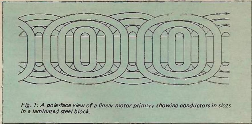
Fig. 1: A pole-face view of a linear motor primary showing conductors in slots in a laminated steel block.
