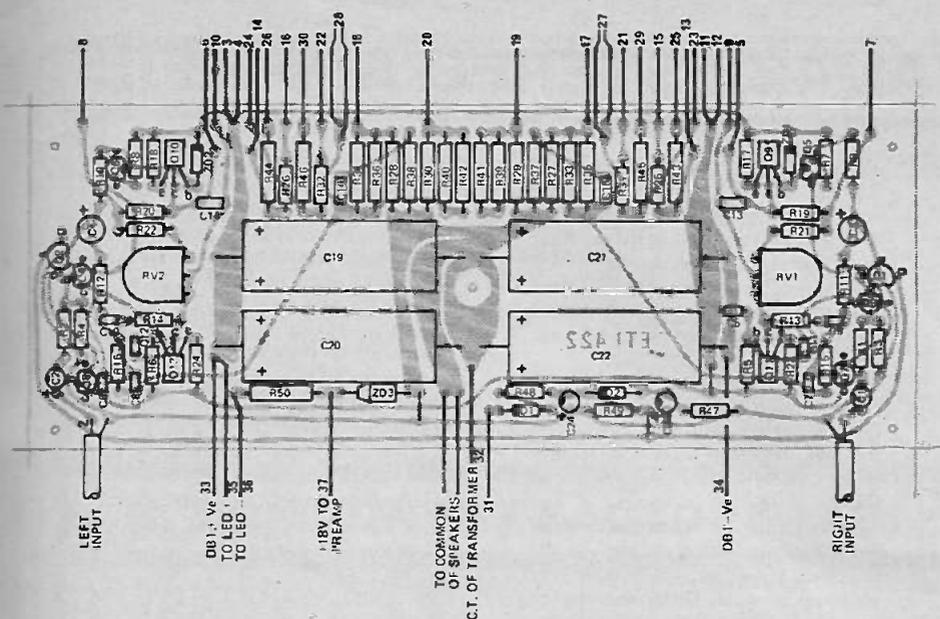
Fig. 6. Component overlay for the main amplifiers and power supply.
