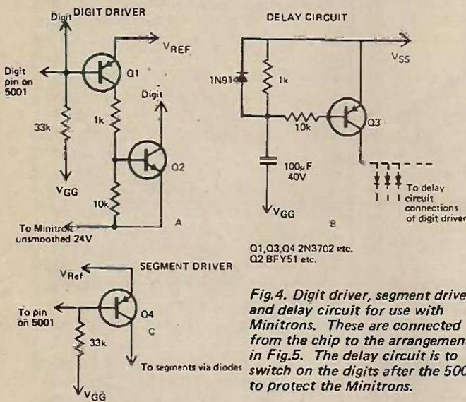
Fig. 4. Digit driver, segment driver and delay circuit for use with Minitrons. These are connected from the chip to the arrangement in Fig. 5. The delay circuit is to switch on the digits after the 5001 to protect the Minitrons.
