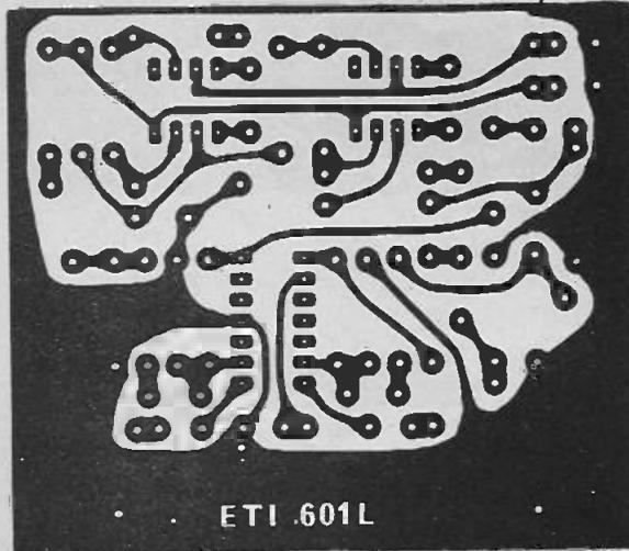
Fig. 2. Printed circuit pattern for the external input module.
