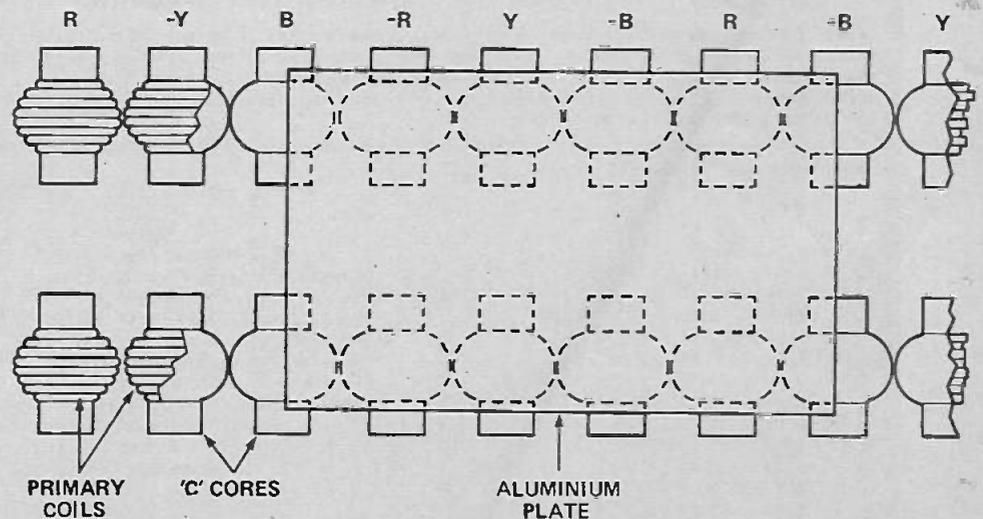
Fig. 15: The magnetic river seen (pole-face view) as simply a pair of parallel linear motors.
