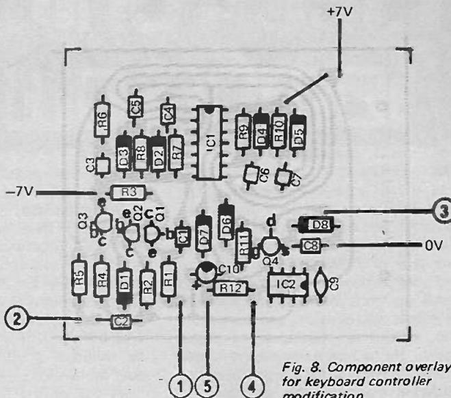
Fig. 8. Component overlay for keyboard controller modification.
