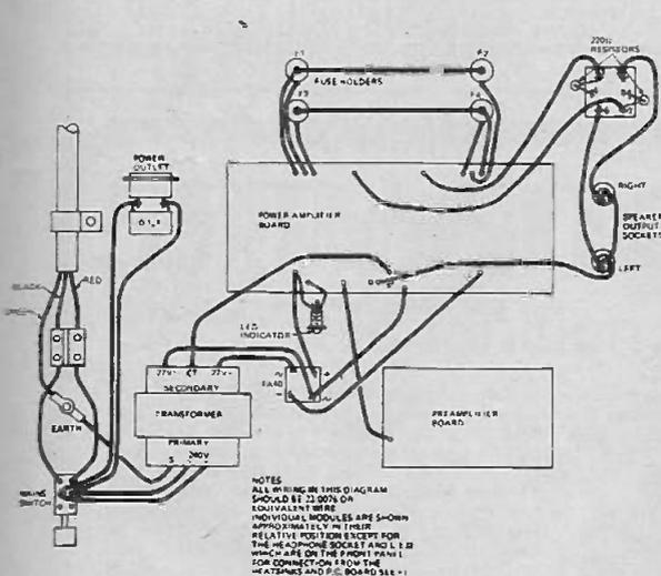
Fig. 9. Power wiring diagram of the complete amplifier.
