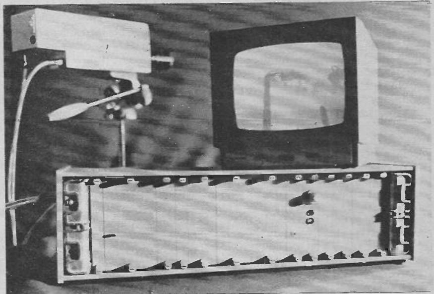
constantly compared with the image which is transmitted live. If sudden changes occur in a stationary television image a visual or audible alarm is given immediately.
