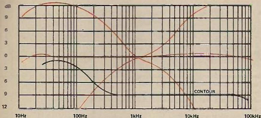
Frequency response with controls flat and at maximum settings. The response of the 'contour' control is shown in black.
