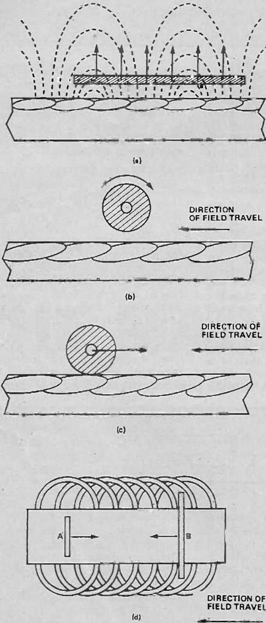
Fig. 5: Phenomena associated with the flux pattern from an open-sided motor:—
