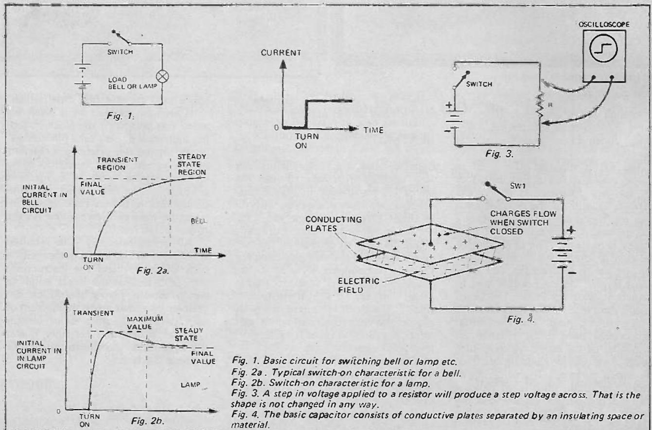
two curves is the transient region. Once the signal has *stabilized* to a constant value it is said to be in the steady state condition.
