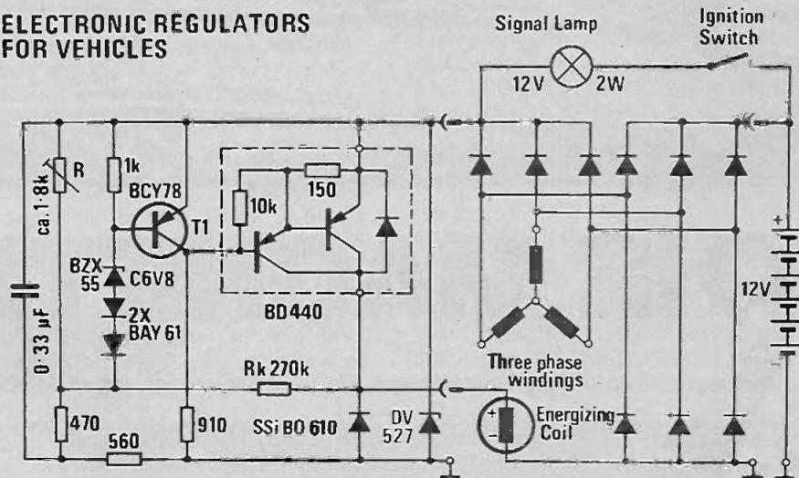
Most vehicles manufactured today are fitted with three phase alternators rather than dc generators but the method of control relies on electro-mechanical regulators, which are unreliable and inaccurate. In order to gain the full benefits of high regulation accuracy and long life from an alternator it is desirable to use a fully electronic control system. Siemens have developed a circuit for this which can be constructed from discrete components.
