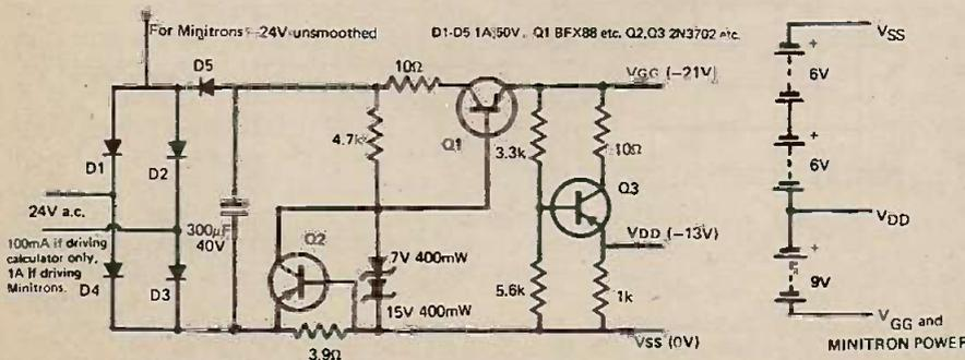
Fig.2. Power supply circuits. On the left is the one for mains, on the right for batteries.
