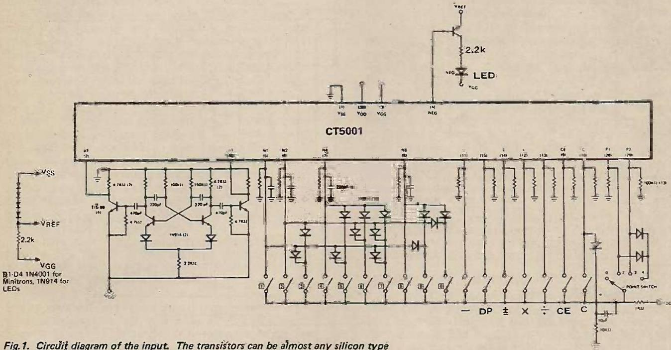
Fig.1. Circuit diagram of the input. The transistors can be almost any silicon type such as 2N3708, 2N706. All diodes are 1N914 or similar. Capacitors can be any type except ceramic.
