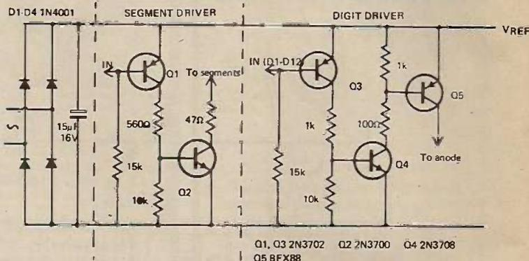
Fig. 7. Segment and digit driver circuits for 0.33" LED displays.
