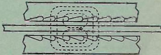
Fig. 3: Flux bending in a plane containing the direction of a motion.
