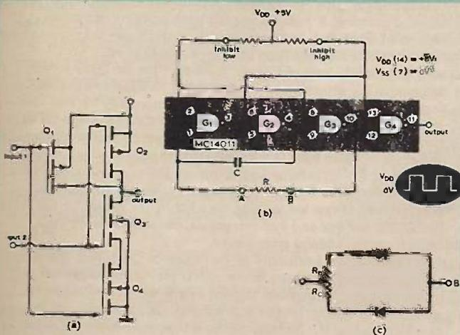
Fig. 1a. The basic circuit of the CMOS NAND gate on which the Astable is based. Fig. 1b. The ultra low frequency astable. Fig. 1c. Insert this network at points AB in place of R to obtain variable mark/space ratio up to 5000:1.
