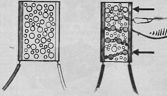
**LEFT:** A cross sectional diagram of Spherax in its relaxed state with the shaded area showing the live feed. **RIGHT:** Spherax in its compressed state. When pressure is applied the metallic particles, represented by the spheres, form a chain creating a circuit through which current (the shaded area) flows.
