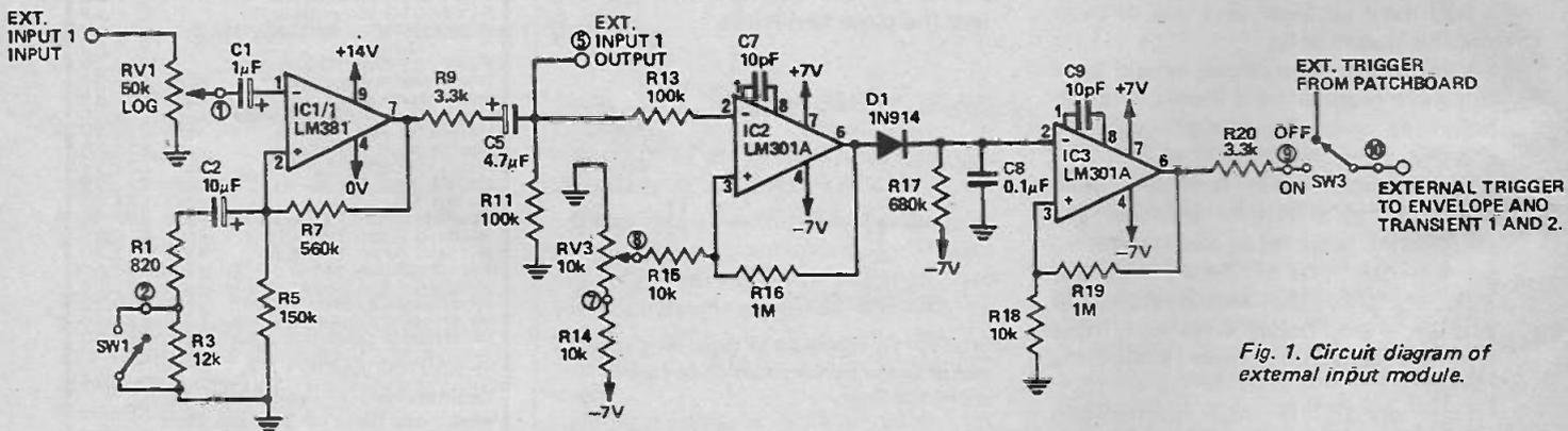
Fig. 1. Circuit diagram of external input module.
