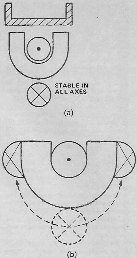
Fig. 14. Single 'C-core' magnetic river apparatus in cross-section: (a) Return current beneath the core. (b) Return currents led back up each side of poles.
