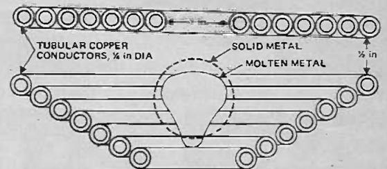
Fig. 7: Cross-section through a liquidmetal levitator using water-cooled tubes as primary windings.
