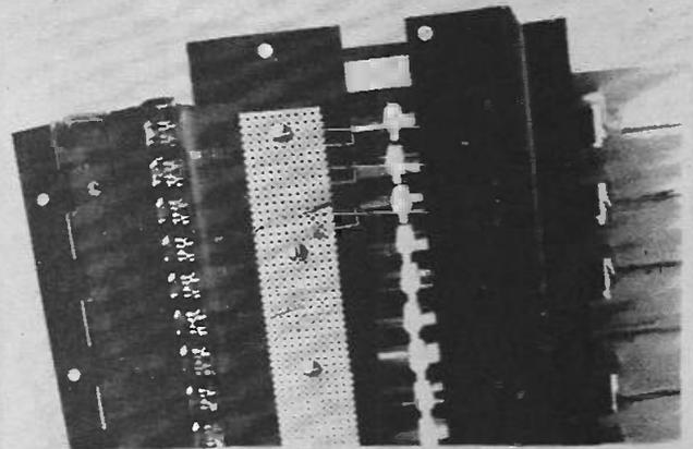
Underneath view of the keyboard showing how the wire fits to the SRBP.
