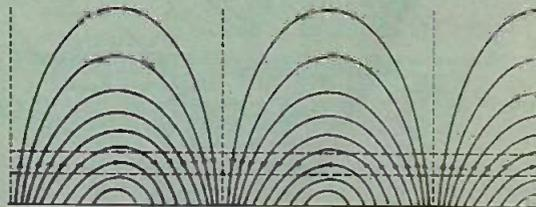
Fig. 4: Flux distribution over an open-sided linear primary.
