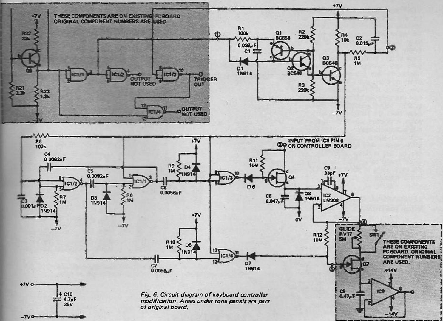
Fig. 6. Circuit diagram of keyboard controller modification. Areas under tone panels are part of original board.
