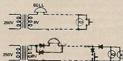
Many houses have a door-bell push lit up by a small bulb as in Fig. 1. A second bulb was required to light up the house number - but the two bulbs together used so much current that the bell trembler was continually buzzing. Running a separate feed from the transformer to the front door was inconvenient.
