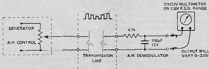
Fig. 10. AM demodulator circuit.
