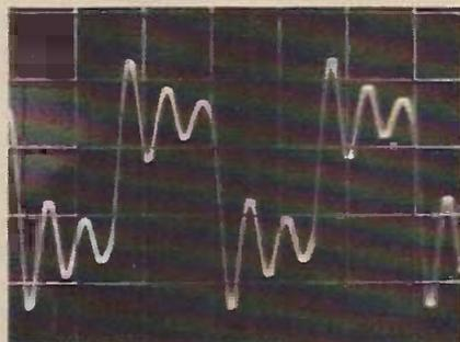
Severe ringing at 10kHz into 8 ohms plus 2  $\mu$ F to simulate an electrostatic speaker.
