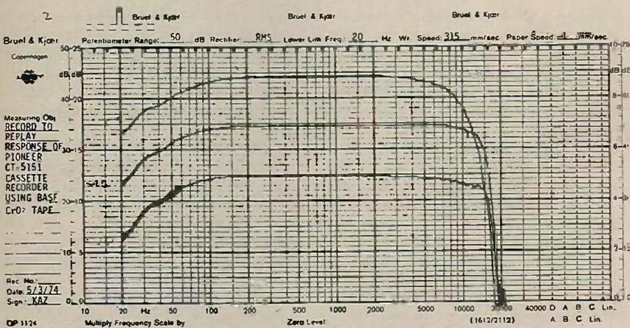
The drop out shown on the top graph (OVU) was due to a characteristic of the test tape used — not the recorder.
