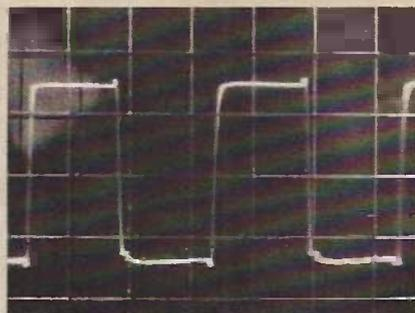
Square-wave response: 10kHz into 8 ohms.
