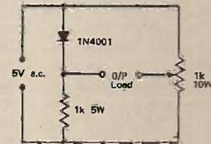
This simple circuit can be used as a full-wave rectifier. If you put a load at the output and adjust the potentiometer, you will see on the oscilloscope the two half cycles have equal amplitudes and they are touching each other, so its a full-wave rectifier with one diode only. This is only suitable for low currents.
