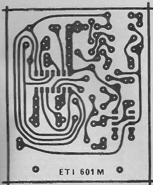
Fig. 7. Printed circuit pattern for keyboard-controller modification.
