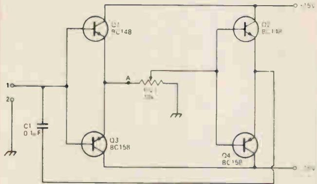
The value of capacitance existing between points 1 and 2 may be varied over a 1000 to 1 range by RV1. The lower value of capacitance is due to C1, the transistor stages effectively multiply this capacitance, thus the total capacitance available from the circuit, as given, is 100μF. It is possible to replace RV1 by a NTC or PTC resistor and thus the value of capacitance will depend on ambient temperature.
