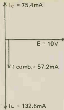
same across each component, and again a vector diagram of reactive and resistive currents will provide us with the magnitude and phase of the input current.
