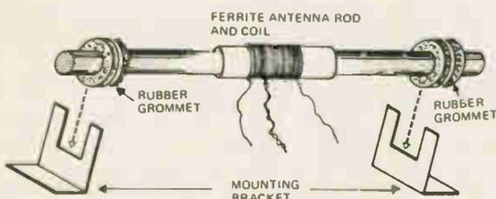
*The ferrite antenna rod and coil can be supported by two grommets and small metal brackets.*
