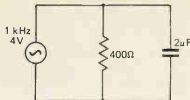
Fig. 3a. Parallel combination of capacitance and resistance.
