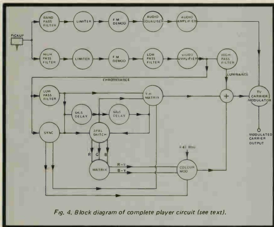
Fig. 4. Block diagram of complete player circuit (see text).
