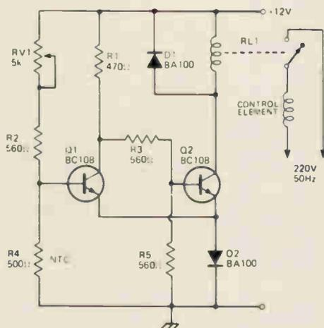
A negative temperature coefficient (NTC) resistor is used to sense temperature. Transistors Q1 and Q2 form a Schmitt trigger which switches when the voltage at the base of Q1 increases above 1.4 volts. Thus when the temperature falls below that set by RV1 the Schmitt changes state and the relay opens switching the heater 'ON'. Regulation accuracy is 1° to 2°C.
