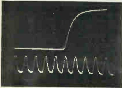
(Upper trace). Step waveform at approximately  $0.3\mu\text{s}$ . (Lower trace). Waveform at 10MHz.
