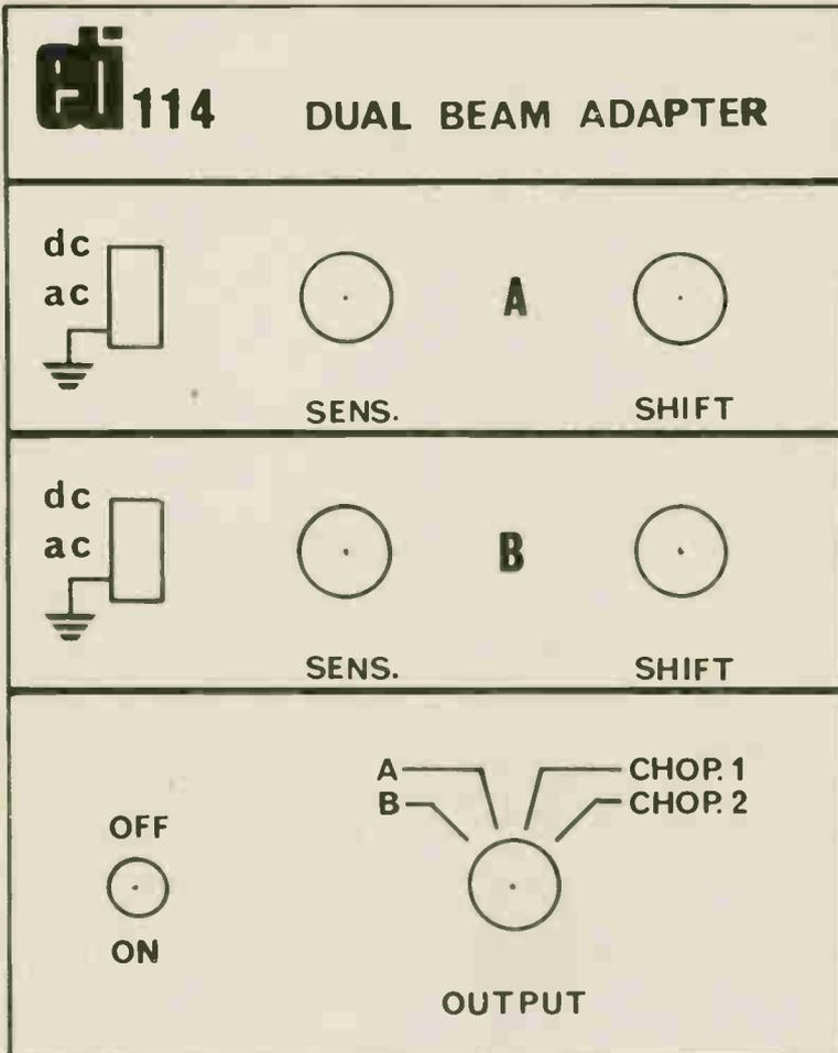
Fig.5. Artwork for front panel of the adaptor.
