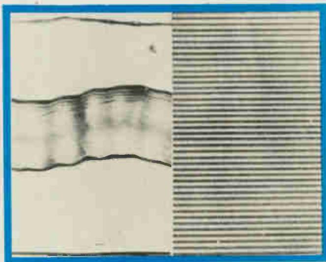
Fig. 1. Photomicrograph compares grooves of (left) standard long-play audio record, and, (right) Teldec video disc.
