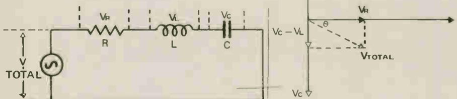
Fig. 6a. Series combination of L, C and R.
