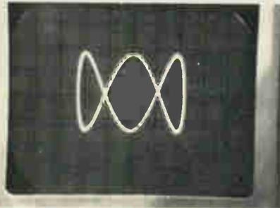
Three to one Lissajous pattern using the X-Y mode inputs and display. The  $0.8\text{cm}$ /division graticule can be seen in this photo.
