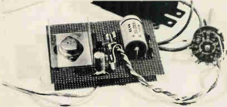
The power supply shown unmounted. Note the aluminium heat sink for the power transistor.
