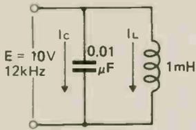
Fig. 5a. A parallel combination of L and C.
