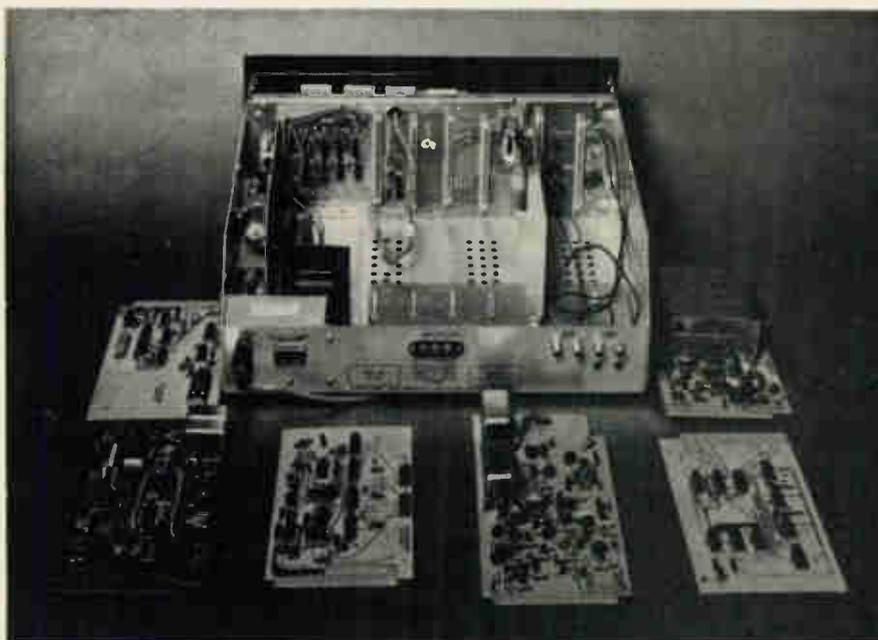
Rear view of the tuner with six of the circuit boards removed.
