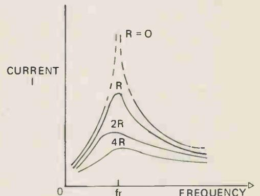
Fig. 11a. The dynamic resistance of a series tuned circuit affects the sharpness of the resonant effect as shown.
