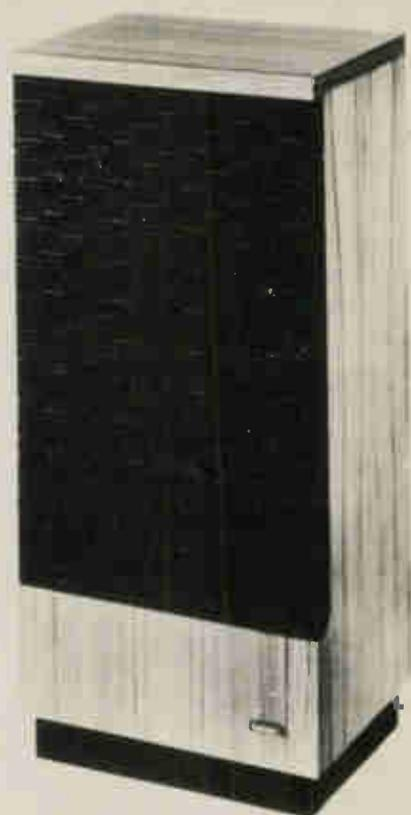
All three speakers are sealed into the enclosure with urethane foam strips, and internal damping is achieved by large blocks of 8 cm thick urethane foam. The speaker connections are unusual terminals at the bottom of the enclosure. These consist of a pair of screw terminals which flank a DIN type speaker socket, and the unit comes equipped with a seven metre long colour coded lead with a DIN plug at one end and a pair of spade lugs at the other.
