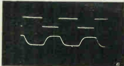
(Upper trace) 10,000Hz square-wave from generator. (Lower trace). Output from amplifier under test.
