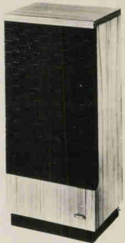
All three speakers are sealed into the enclosure with urethane foam strips, and internal damping is achieved by large blocks of 8 cm thick urethane foam. The speaker connections are unusual terminals at the bottom of the enclosure. These consist of a pair of screw terminals which flank a DIN type speaker socket, and the unit comes equipped with a seven metre long colour coded lead with a DIN plug at one end and a pair of spade lugs at the other.
