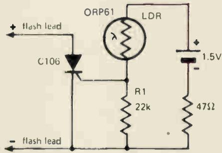
In photography, a separate flash, triggered by the light of a master flash light, is often required to provide more light, fill-in shadows etc. The sensitivity of this circuit depends on the proximity of the master flash and the value of R1. Increasing R1 gives increased sensitivity.
