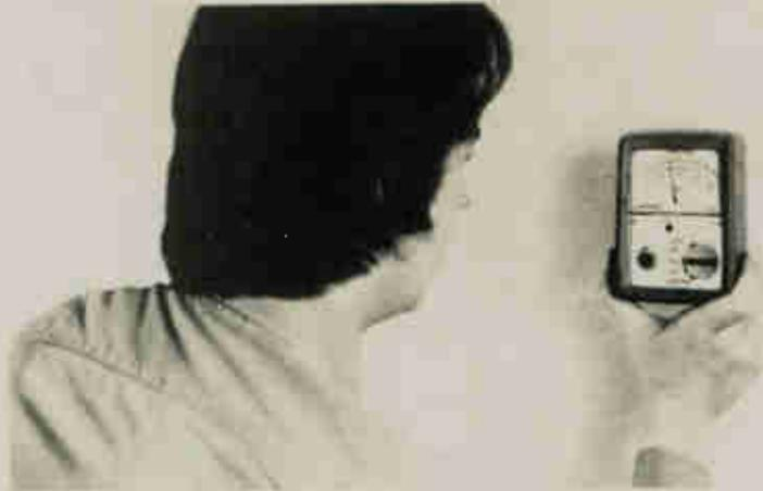
Metrawatt (U.K.) Ltd. has introduced a battery-operated cable tracer designed to aid electrical engineers and D.I.Y. enthusiasts in the location of cables concealed under plastered walls and similar coverings and in troubleshooting for cable breaks and short circuits. The LS2 - which is priced at £27.50 - can also be used as a voltmeter for measuring a.c. voltages up to 400V.
