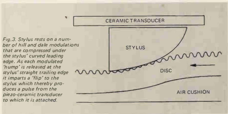
Fig. 3. Stylus rests on a number of hill and dale modulations that are compressed under the stylus' curved leading edge. As each modulated 'hump' is released at the stylus' straight trailing edge it imparts a 'flip' to the stylus which thereby produces a pulse from the piezo-ceramic transducer to which it is attached.
