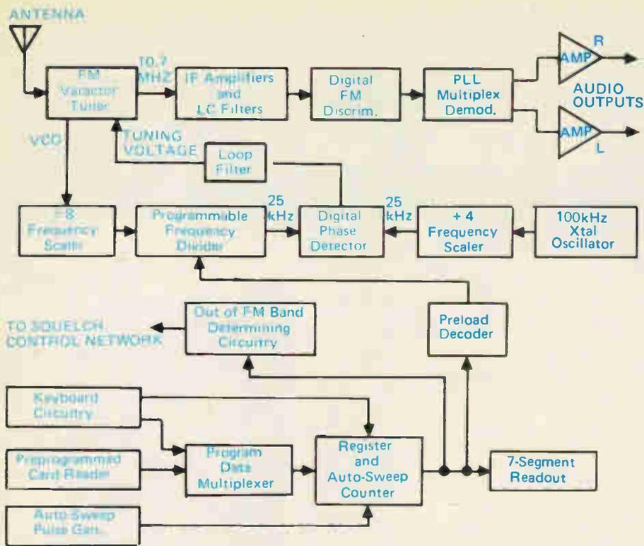
Block diagram (greatly simplified) of the circuit.
