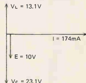
$$X_L = 2\pi FL = 6.28 \times 12 \times 10^3 \times 1 \times 10^{-3} = 75.4 \text{ ohms}$$
