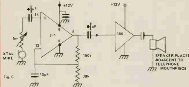
The LM381N dual op-amp has appeared several times in its usual guise as a low noise stereo audio preamplifier device. Indeed, it requires the very barest minimum of external components, since the function of the feedback resistors and capacitors is simply to determine the audio frequency response and gain.
