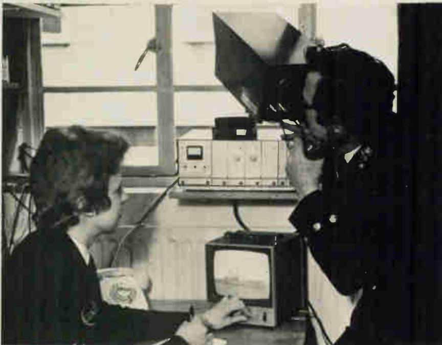
The picture shows the setting up of an audio-video linkage between buildings at HMS Mercury, the navy's signal school near Petersfield. This new opto-electronic linkage transmits across obstacles such as roads, railways and waterways using modulated infra-red radiation (900 nanometers). It
