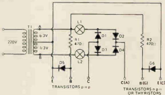
The 6.3-0-6.3V winding of T1 is bridge rectified by D1-D4, the two ac arms of the bridge being connected through L1 and L2 (75 mA maximum). The rectified waveform is applied to the collector of the transistor (or anode of SCR) under test.
