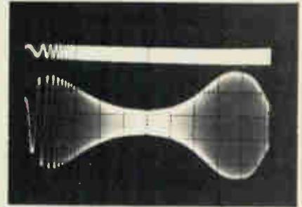
(Upper trace). Output from an audio frequency sweep generator L to R, 10 to 100Hz  $\pm 0.1\text{dB}$ . (Lower trace) Output from amplifier under test with bass and treble controls at maximum.
