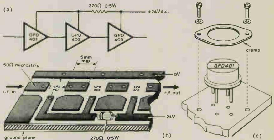
This wideband r.f. amplifier will provide a gain (within 2dB) of 35dB from 5 to 400MHz. The noise figure will be about 4.7dB and the power output (into 50Ω) will be +14dBm.
