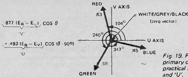
Fig. 19. Phases and amplitudes of primary colour vectors using practical modulation signals 'V' and 'U'.
