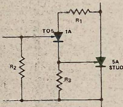
A typical stud thyristor of 5A rating will need 10mA or more for triggering into conduction. This can be reduced to 1mA or less by using an additional 1A thyristor of TO5 construction.
