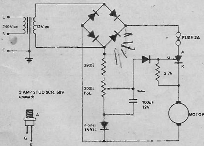
The following is a low voltage adaptation of the type of speed control popularly used to regulate power drills. It gives very good starting
