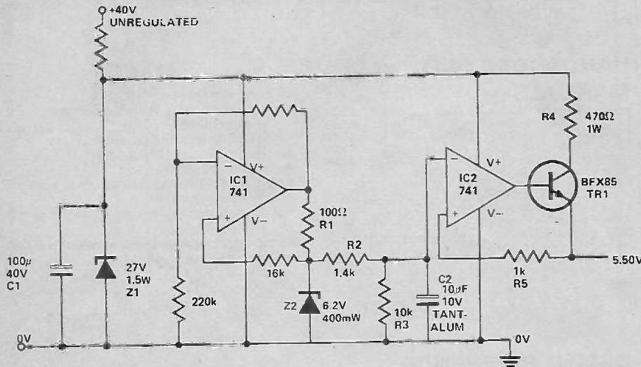
This circuit was evolved to provide a highly stable and ripple-free voltage to act as the reference for the stabilised power-supplies of an electronic music synthesiser; the stability of its voltage-controlled oscillators depended directly on the constancy of supply-rail voltages.
