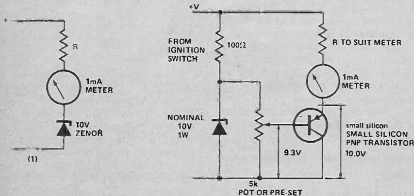
To make a meter cover the range 10 to 15V or 10 to 20V over its whole scale, then circuit (1) is often used.
