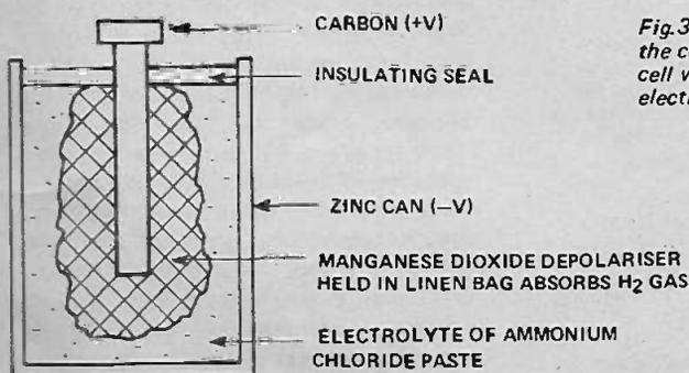
Fig. 3. Cross section of the common tubular dry-cell which uses a paste electrolyte.
