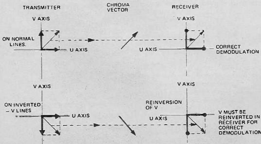
Fig. 21. Inversion of V signal on alternate lines in the PAL system.
