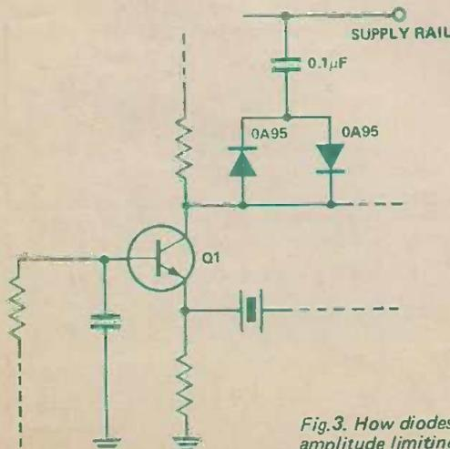
Fig. 3. How diodes are used for amplitude limiting.
