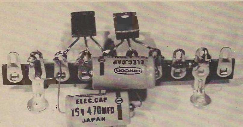
Fig. 8. Actual tag strip for negative earth version. Note the wire joining the two tags above the mounting feet, and also the use made of the lower holes in the tags.
