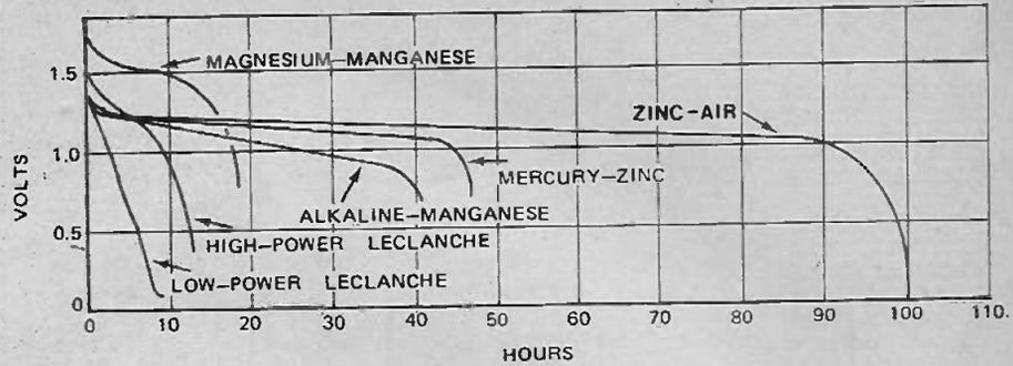
Fig.6. Comparative chart showing voltage characteristics of similar size units of various types of dry cell battery.
