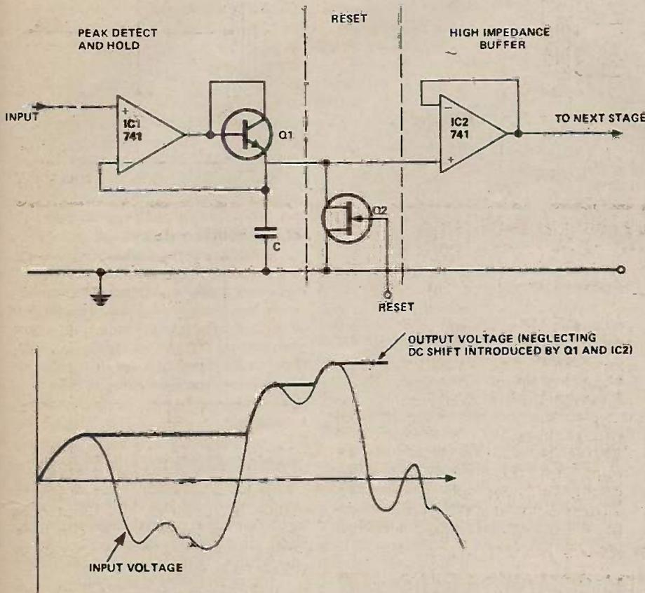
If the voltage at the input becomes bigger than the voltage on the capacitor, then the output of the 741 goes positive, the diode conducts, and the capacitor is charged up to the input voltage-forward voltage drop of diode. When the voltage at the input is less than that on the capacitor, the
