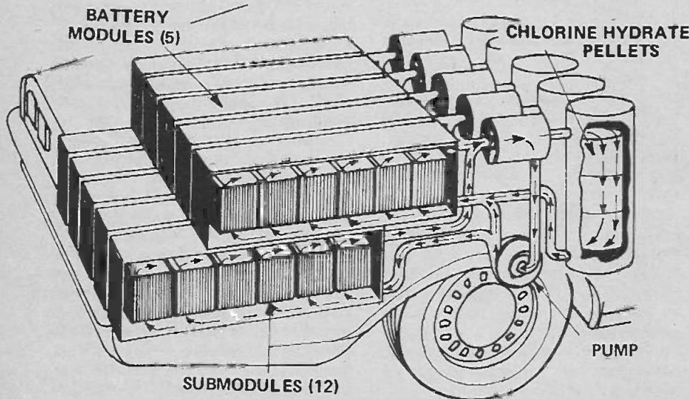
Fig.9. Layout of chlorine-zinc battery installation in a vehicle.
