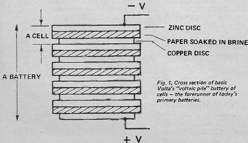
Fig. 1. Cross section of basic Volta's "voltaic pile" battery of cells — the forerunner of today's primary batteries.
