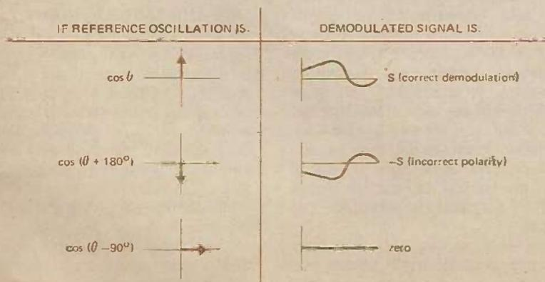
Fig. 15. Principle of synchronous modulation and demodulation. Correct demodulation is only obtained if the receiver's reference oscillator is synchronised in frequency and phase to the transmitter's carrier oscillator.
