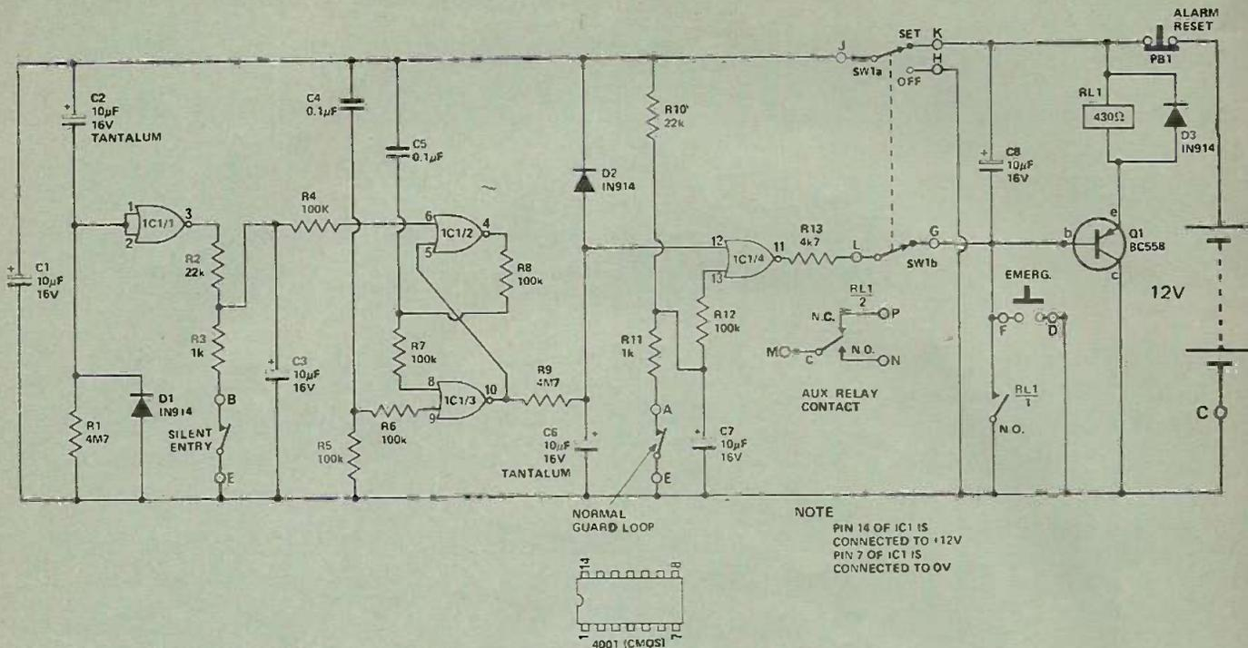
Fig. 1. Circuit diagram of the ETI Burglar alarm.
