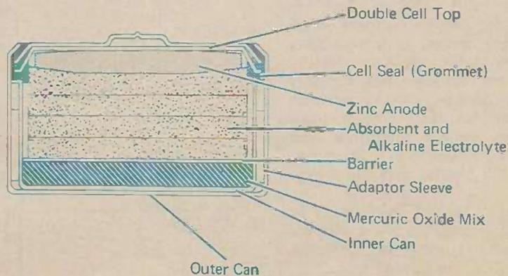
Fig.4. Cross sections of a typical mercury cell.
