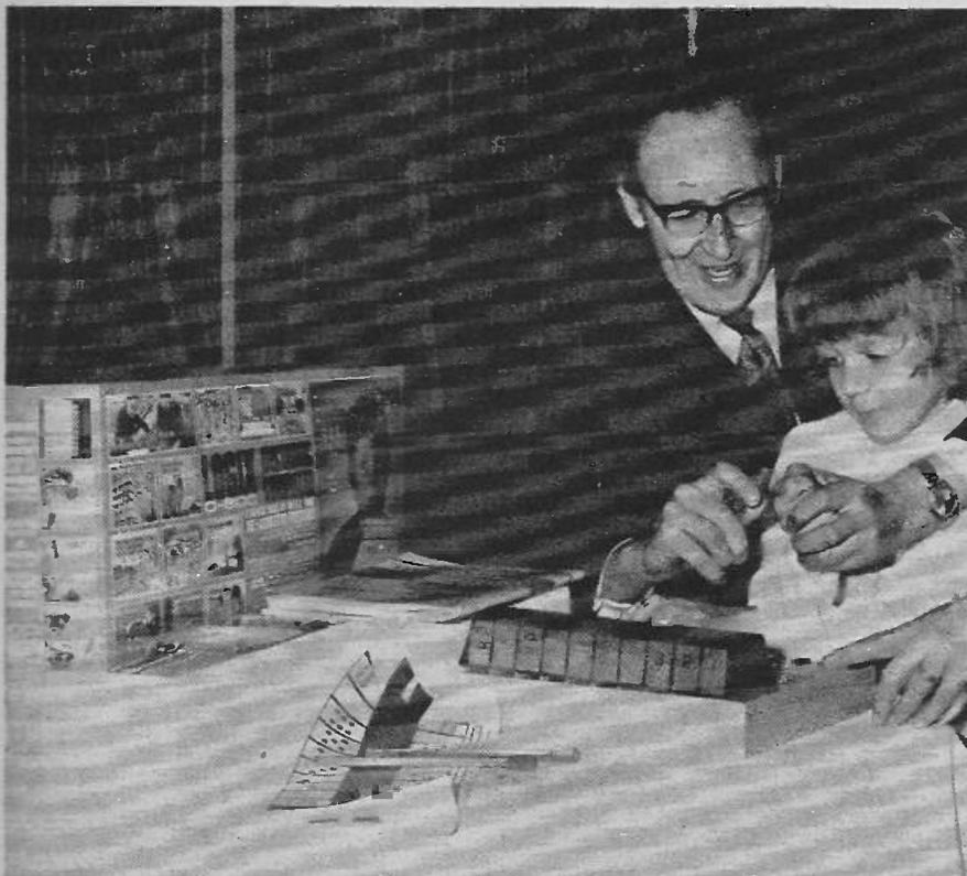
*A new range of scientific construction kits for young people is being introduced to the UK from Canada by Patterson Edwards Ltd. The toy in the picture is a miniature computer. The computer, which works on the same principle as a real one, comes complete with 112-page manual containing fifty programs. It is also possible for youngsters to make up their own programs. The computer comes in the form of a kit which retails for approximately £18.*
