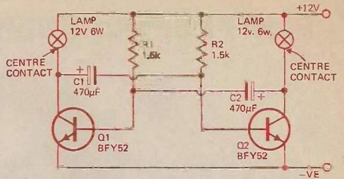
Fig.4 Circuit of the POSITIVE earth version
