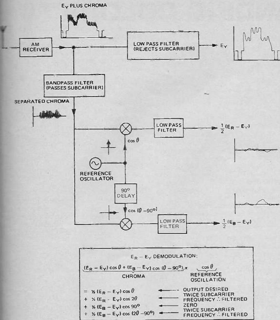
Fig. 17. A suitable receiver for the signal produced by Fig. 16. For correct colour demodulation the reference oscillator must be precisely phase-locked to the transmitter. The insert shows a full description of the  $(E_R - E_V)$  demodulator; the  $(E_B - E_V)$  demodulator works similarly.
