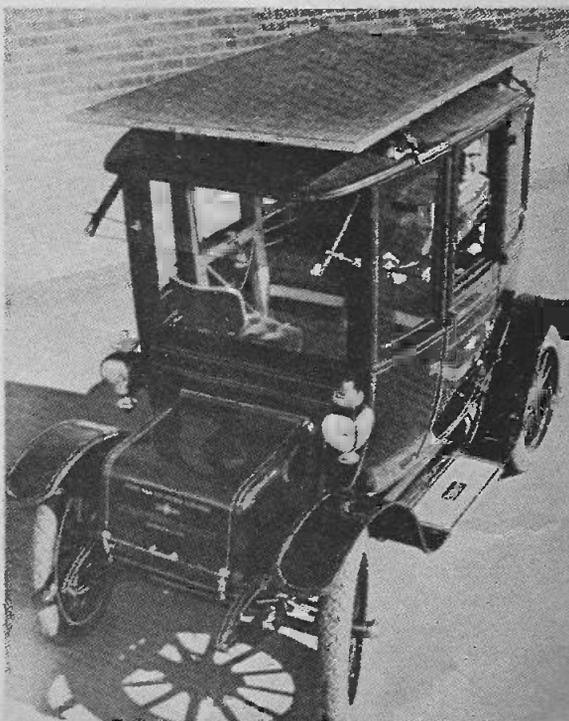
*This 1912 Baker Electric is now driven by solar energy! An array of 10 640 silicon solar cells mounted on the vehicle's roof charge intermediate storage batteries. Final drive is via the Baker's original dc electric motor*
