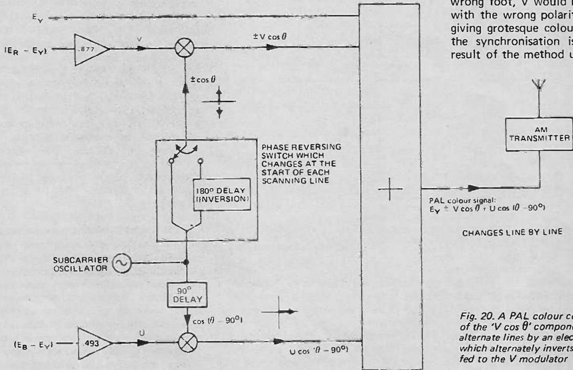
Fig. 20. A PAL colour coder. The polarity of the 'V cos  $\theta$ ' component is reversed on alternate lines by an electronic switch which alternately inverts the subcarrier fed to the V modulator
