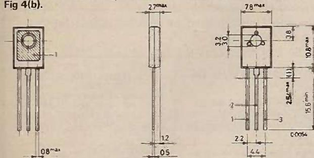
Pin 3 connected to metal part of mounting surface.
