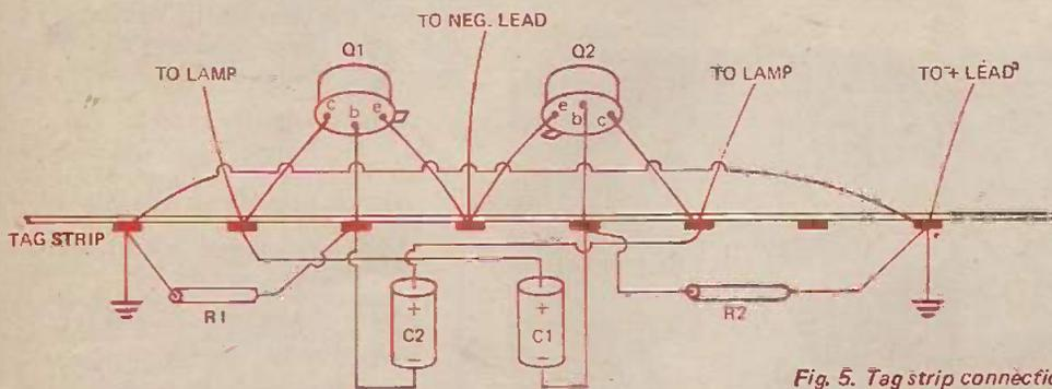
Fig. 5. Tag strip connections of positive earth version.
