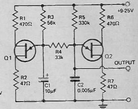
This circuit will produce a continuous sequence of increasing frequencies (in steps) until the highest is reached. The system then resets itself and starts again.
