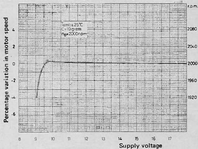
The speed of a small cassette recorder can vary with the supply voltage, with the ambient temperature and with the torque applied by the tape to the motor spindle. Such variations of speed can produce a considerable effect on the sound reproduction.
