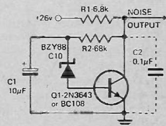
A basic noise generator can be built using one transistor and a Zener diode.
