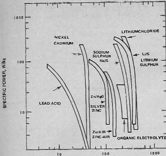
Fig. 5. Comparative chart of the main forms of high-temperature battery designs.
