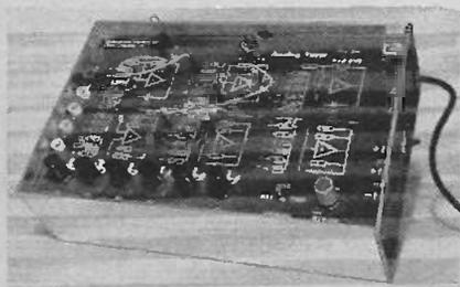
An analogue computer which can be used in schools for teaching the basic principles of analogue and hybrid computation has been developed by Limrose Electronics.
