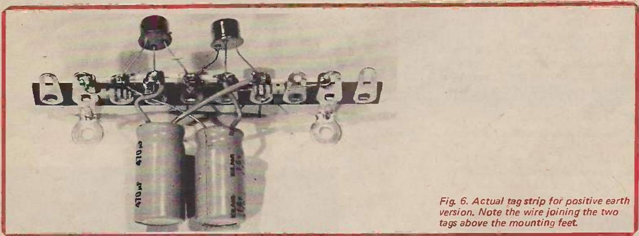
Fig. 6. Actual tag strip for positive earth version. Note the wire joining the two tags above the mounting feet.
