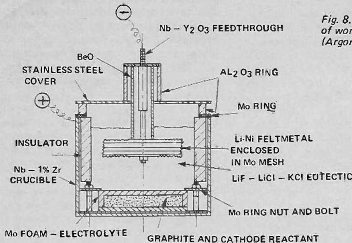
Fig. 8. An advanced form of workable Li-S cell (Argonne Laboratory).
