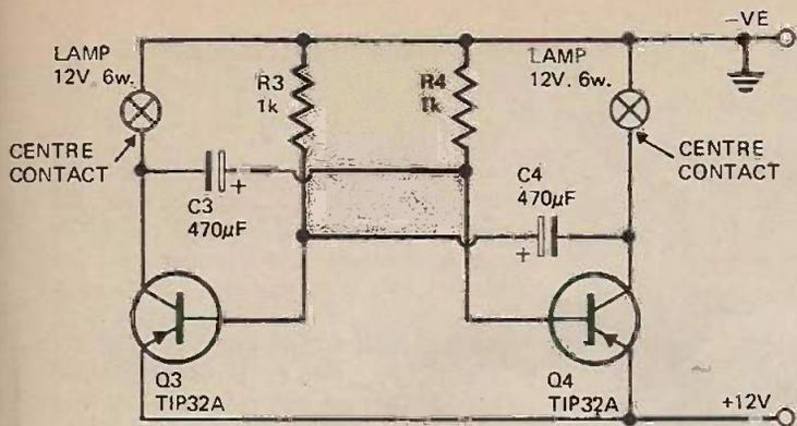
Fig.3 Circuit of the NEGATIVE earth version
