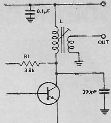
Fig. 8b. Adding a coil to the circuit shown in Fig. 8.
