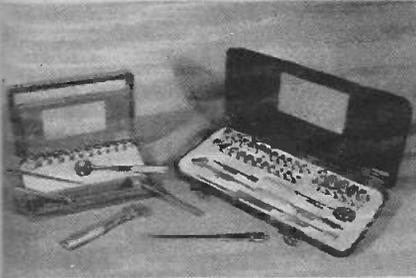
The first set is a 17-piece, 1/4" drive Socket Set covering BA sizes and includes 11 sockets, from 0BA to 10BA, two extension bars and one each ratchet handle, flexible handle, cross bar, and sliding bar. The carrying case of plastic has an integral carrying handle.
