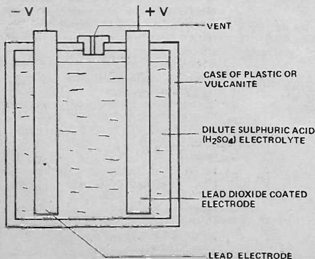
Fig.4. Schematic of the common lead-acid storage cell. They are made in flat parallel plate and tubular forms depending on the application.
