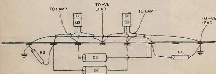
Fig. 7. Tag strip connections of negative earth version.
