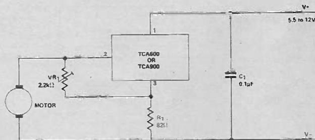
Fig 2: Typical Speed Control circuit of a cassette player running from batteries or mains.
