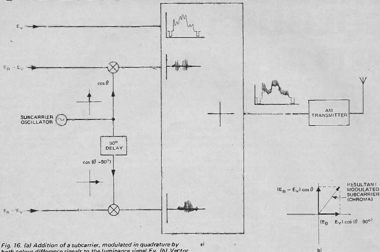
Fig. 16. (a) Addition of a subcarrier, modulated in quadrature by both colour difference signals to the luminance signal  $E_Y$ . (b) Vector representation of subcarrier.
