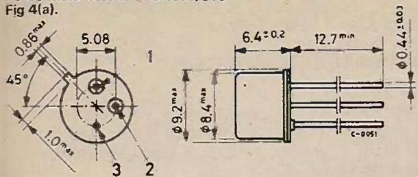
Pin 3 connected to case.
