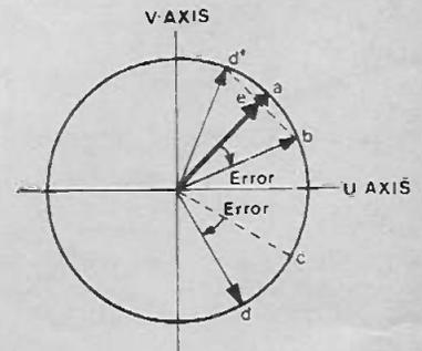
Fig. 22. Effect on two successive lines of the same colour of a demodulation phase error in the receiver. For explanation see text.
