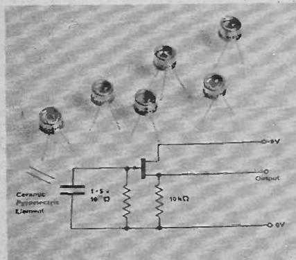
The new Plessey PPC 522 low-cost broadband ceramic pyroelectric infra-red detector which comprises a detector element and J.F.E.T. preamplifier encapsulated in a TO5 transistor can, with a suitable cell window according to the required application. These devices are specifically designed for intruder detection, fire alarm and pollution monitoring applications.
