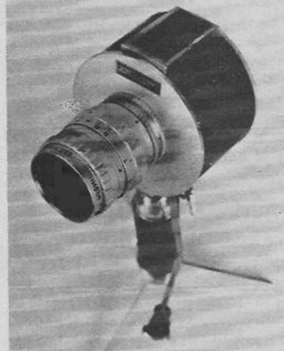
The camera can operate at a distance of up to 100 feet from the monitor. An optional battery pack is available when complete portability is required. The standard lens of the MV101 is a 25mm f/1.4 C-mount type. Information from Fairchild Camera and Instrument Corporation, 464 Ellis Street, Mountain View, California 94042 USA.
