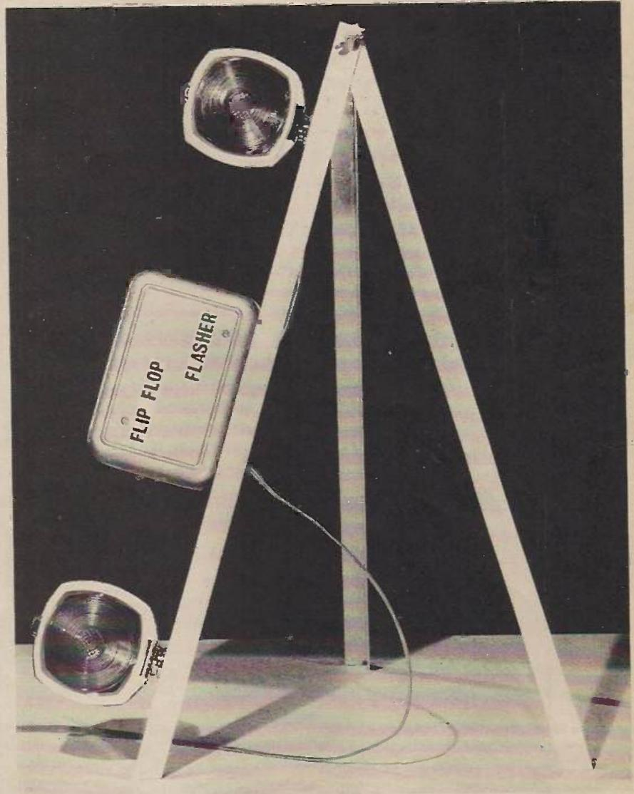
legs can separate by an angle of only about 32 degrees. The third leg is attached to a small bracket made from the same aluminium angle, and shown in Fig 10. The bracket is attached to the front legs by the bolt and wing nut which holds them together. The rear view arrangement is shown in Fig 11,
