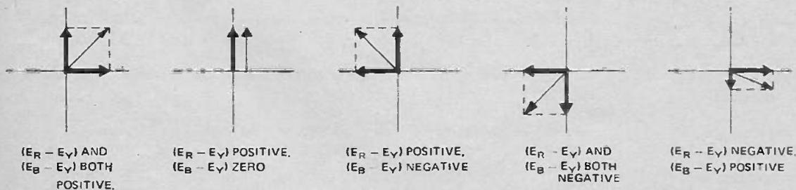
Fig. 18. Typical chroma vectors (thin arrow) produced by various values of  $(E_R - E_V)$  and  $(E_B - E_V)$  modulated as in Fig. 16.
