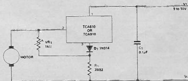
Fig 3: A circuit for use in a car or where the supply voltage is 9 to 18V.
