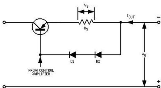
Fig.14. Automatic current limiting is obtained with a series sensing resistor. This method of control is often used in series-pass voltage regulators.
