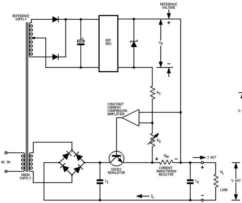
Fig. 13. Constant-current control is easily obtained as an extension of the constant-voltage supply. A series sensing resistor produces a voltage which, in conjunction with an error amplifier, controls the series pass transistor to maintain constant current.
