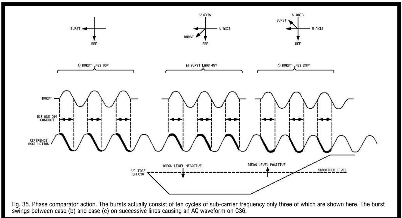
Fig. 35. Phase comparator action. The bursts actually consist of ten cycles of sub-carrier frequency only three of which are shown here. The burst swings between case (b) and case (c) on successive lines causing an AC waveform on C36.
