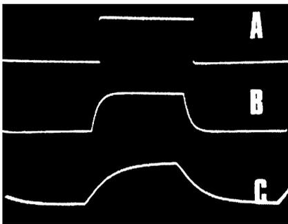
Fig. 16. Amplifier tests-with square-waves. (A) 1000 Hz square-wave input signal. (B) Indicates fairly good high frequency response falling away about about 20kHz. (C) indicates poor high frequency response falling away badly at probably less than 10kHz.
