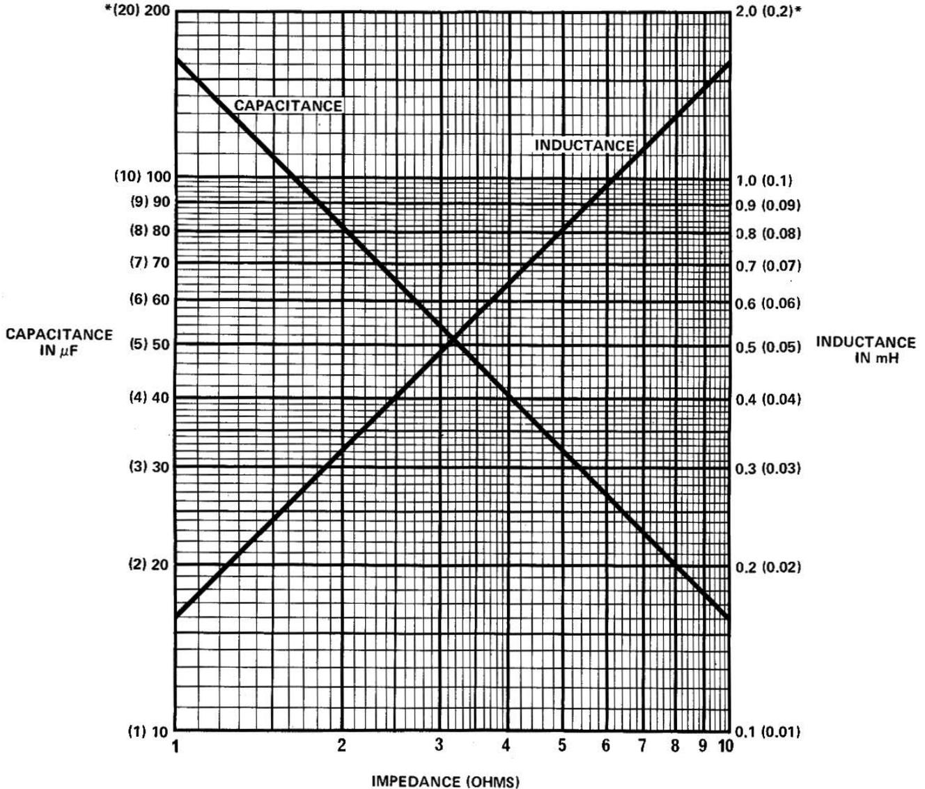
FOR IMPEDANCES GREATER THAN 100 OHMS DIVIDE CAPACITANCE SCALE BY THE SCALING FACTOR AND MULTIPLY THE INDUCTANCE SCALES BY THIS FACTOR.
