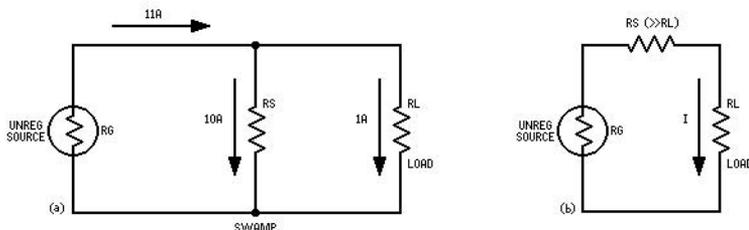
Fig. 1. Regulation can be slightly improved by: (a). Voltage regulation - an additional shunt load. (b). Current regulation - an additional series load.
