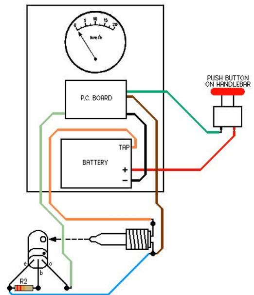
Fig.3. This schematic drawing shows how the various parts are interconnected. The direction of light should be perpendicular to plane of transistor body.
