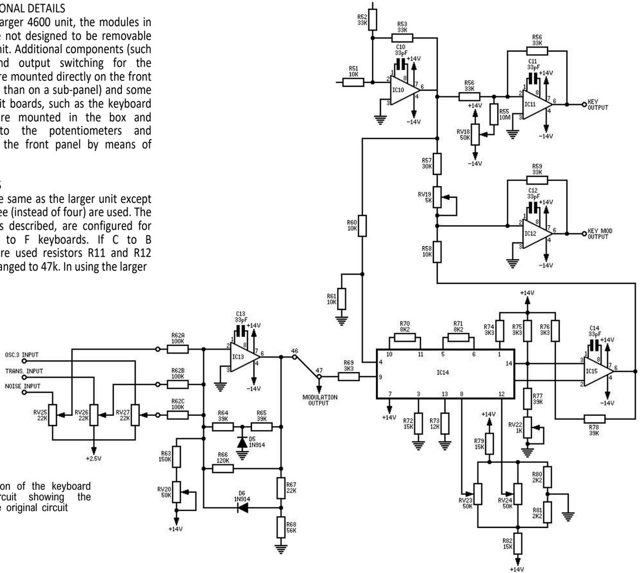
Fig. 1. Portion of the keyboard controller circuit showing the changes to the original circuit
