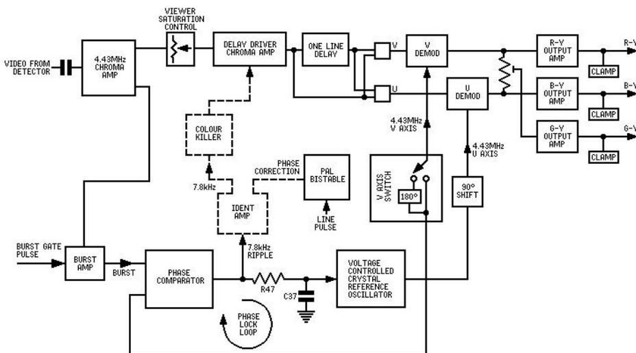
Fig. 34b This is a block schematic of Fig. 34a. The dotted stages are not essential for decoding.
