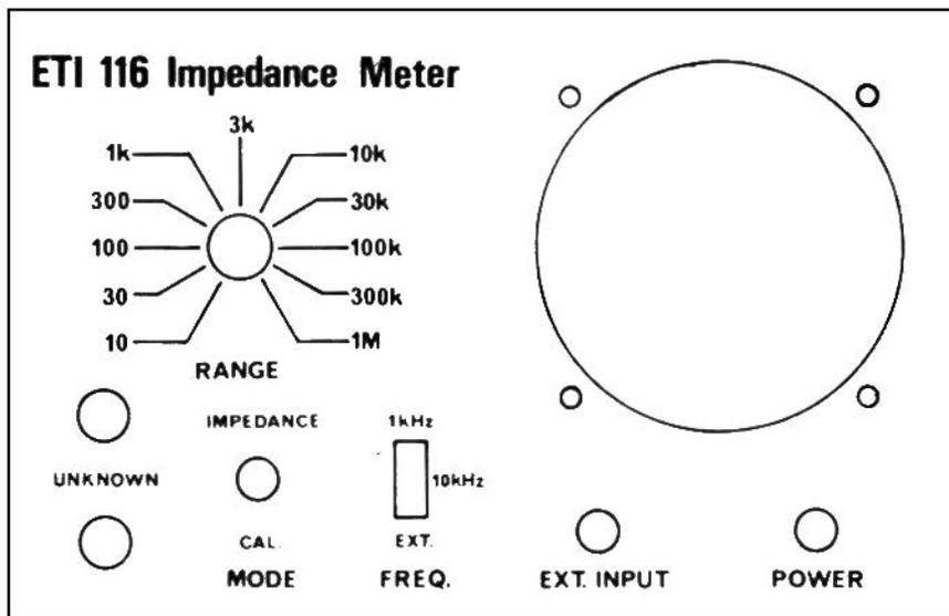
Fig.6. Layout of the front panel. Full size is 152mm x 98mm.
