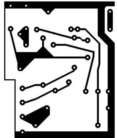
Fig.2. The PCB pattern.
