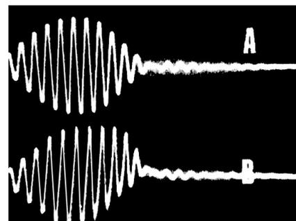
Fig. 25. Pickup cartridge track-ability testing. (A) Good track-ability. (B) Poor track-ability. See text for explanation.
