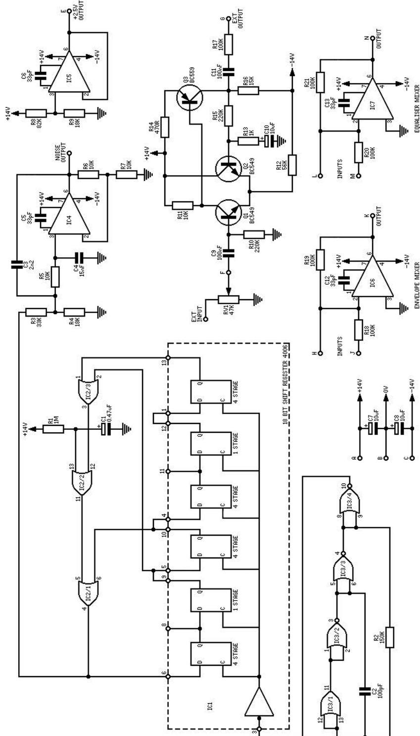
Fig. 2. The auxiliary board circuit diagram.
