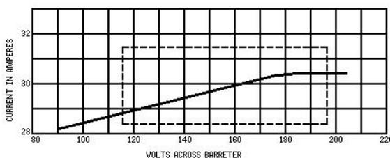
Fig. 2 (a). The barretter tube regulates by the increase in resistance with temperature (and hence current) of an iron wire filament. (b). The gaseous-tube voltage regulator operates by virtue of the constant voltage which appears across a gas discharger over a wide range of current.
