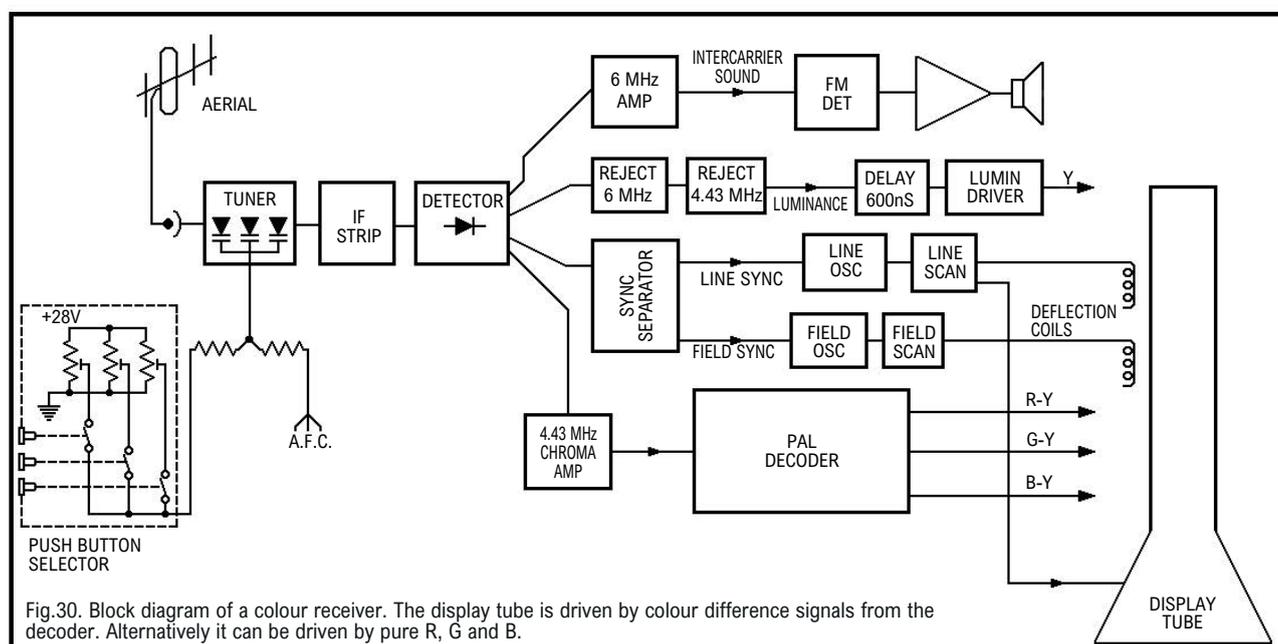
Fig.30. Block diagram of a colour receiver. The display tube is driven by colour difference signals from the decoder. Alternatively it can be driven by pure R, G and B.
