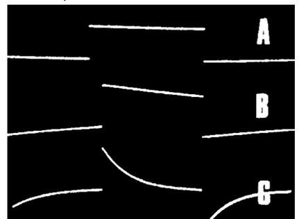
Fig.16. Amplifier tests with square-wave (A) 100 0 Hz square-wave Input signal. (B) only slight slope at top Indicates good response at low frequencies. (C) Curved and steep slope indicates severe loss of low frequency response.
