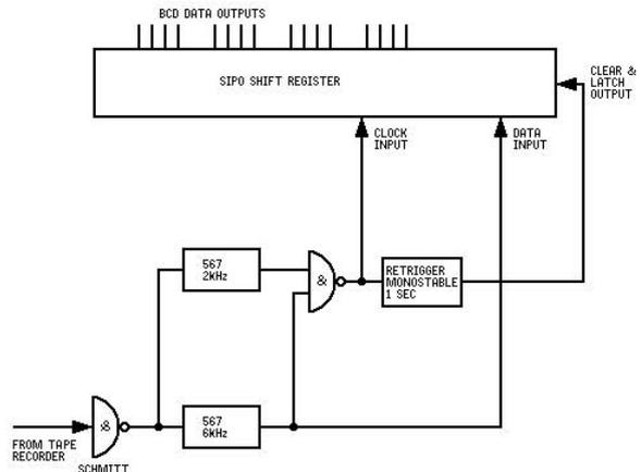
Fig.4. Decoder Block Diagram.
