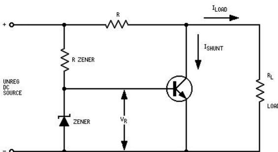
Fig. 10. Basic shunt regulator uses transistor to maintain constant load current on the unregulated DC source.
