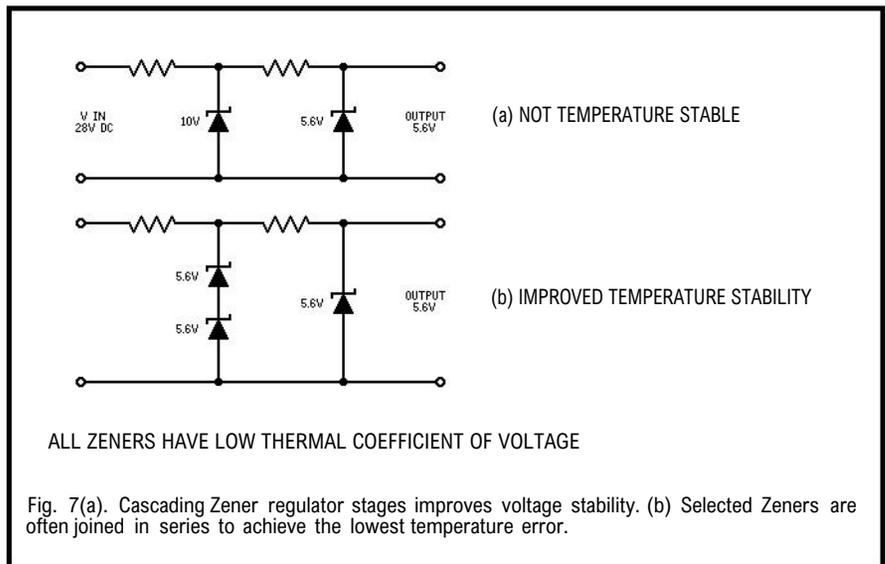
Fig. 7(a). Cascading Zener regulator stages improves voltage stability. (b) Selected Zeners are often joined in series to achieve the lowest temperature error.
