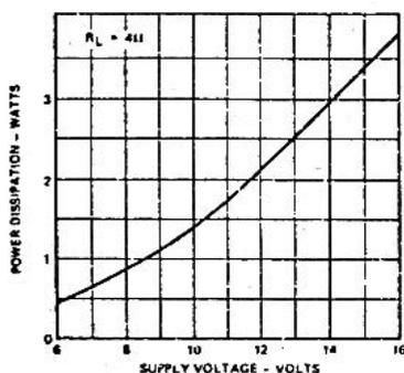
Fig.5. The maximum power dissipated in the device plotted against the supply voltage.
