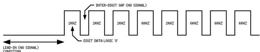
Fig.2. How a BCD number "17" goes onto cassette.
