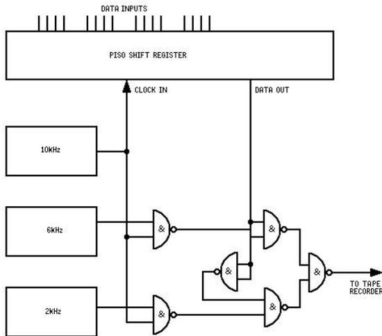
Fig.3. Encoder Block Diagram.
