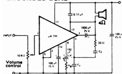
Fig.7. A circuit in which one side of the of the loudspeaker is earthed.
