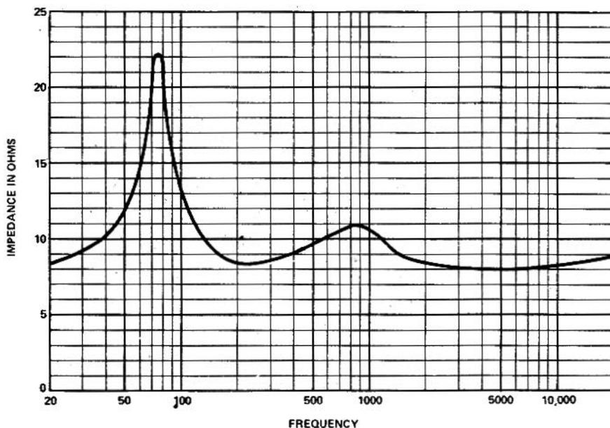
Fig.7. Impedance-versus-frequency plot for a two-way speaker box. Note the combined speaker/box resonance is 75Hz. The crossover frequency was 2kHz. A plot such as this would be extremely difficult to generate using a conventional LCR bridge, but is very simply done using the ET/116 impedance meter.
