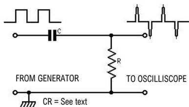
Fig.5. Simple RC network to obtain marker pips from a square-wave signal and which lend themselves for time scale calibration. A diode may be connected across R to eliminate positive and/or negative going pulses as desired.
