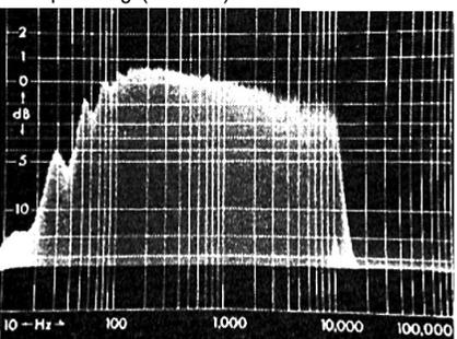
Fig.30. Record-to-replay frequency response of a cassette tape recorder by frequency sweep test.
