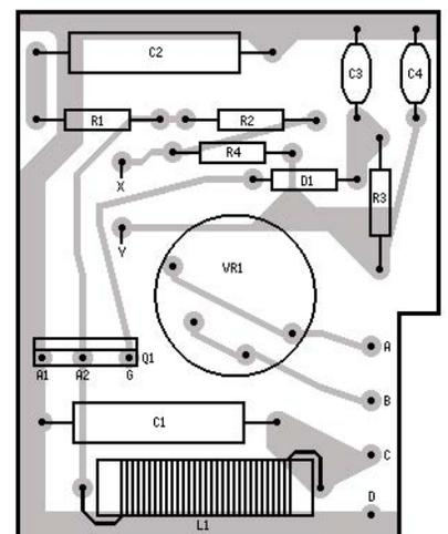
Fig. 3. Components layout, seen from the front of the PCB. The PCB has been flipped from left to right.
