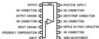
Fig. 1. Connections of the 14-pin dual-in-line  $\mu$ A706
