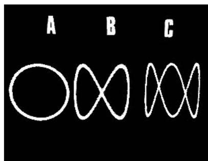
Fig.12. Typical Lissajous patterns of 1:1. 2:1 and 3:1. See text for interpretation.
