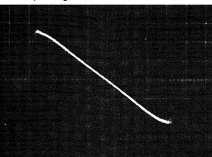
Fig.28. Sweep response. FM detector characteristic with good linearity over about 400kHz.
