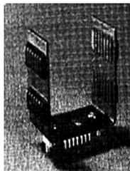
Photo 2. A large heat sink for the efficient cooling of the uA706.
