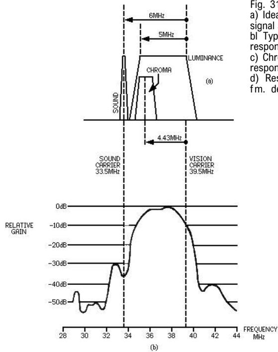
Fig. 31. a) Idealised spectrum of colour TV signal at i.f. b) Typical frequency response of a receiver i.f. strip c) Chroma amplifier response d) Response of inter-carrier sound fm. detector.
