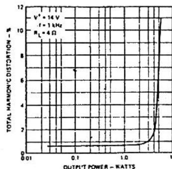
Fig. 4. This graph shows that the distortion is almost independent of output power at low levels, but increases extremely rapidly at the onset of clipping.
