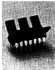
Photo 3. A small heat sink attached to a uA706A.
