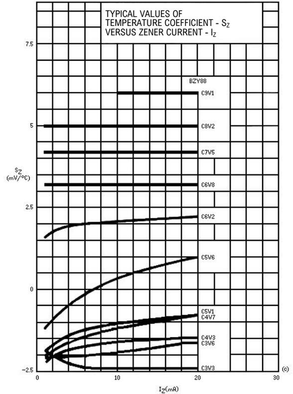
Fig.6a. Typical Zener diode regulator. (b) Dynamic resistance of BZY88 series Zeners. (c) Temperature coefficients of BZY88 series diodes.
