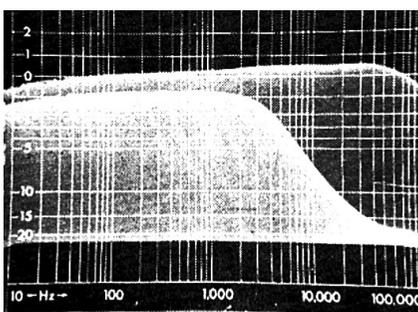
Fig.29. Audio amplifier responses by frequency sweep testing (see text).
