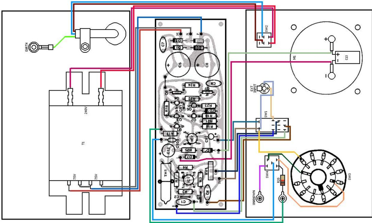
Fig. 4. Component overlay and wiring diagram for the impedance meter.
