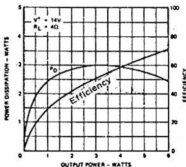
Fig.6. The power dissipated in the device at various output power levels.
