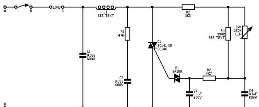
Fig.1. The circuit of the dimmer.
