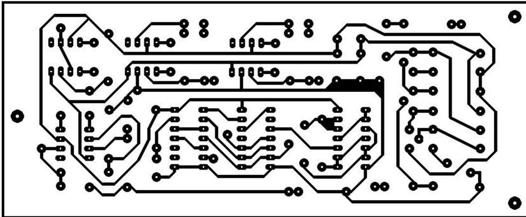
Fig. 3. Printed circuit board layout for the auxiliary board. Full size 142 x 57 mm.
