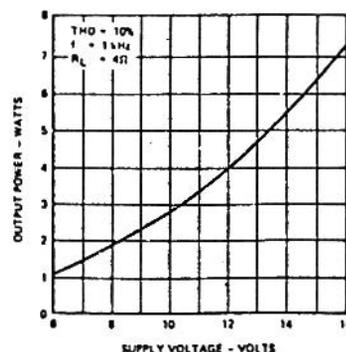
Fig. 3. Maximum power output plotted against the supply voltage.
