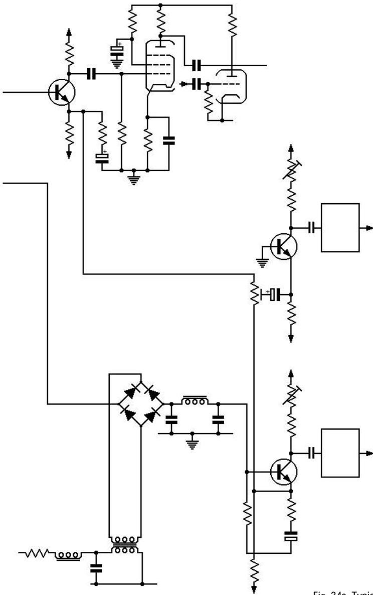
Fig. 34a. Typical PAL decoder.
