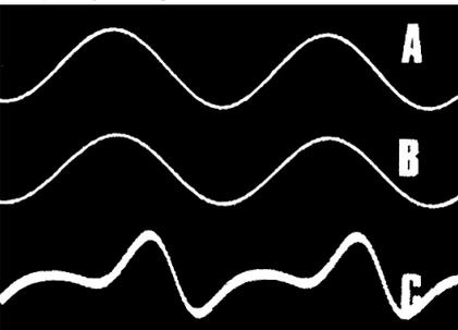
Fig. 18. Deceptive sine-waves (A) and (B) both 'look' good but (A) has less than 0.2% distortion whereas (B) has more than 0.3% and its harmonic content is shown at (C) greatly amplified.
