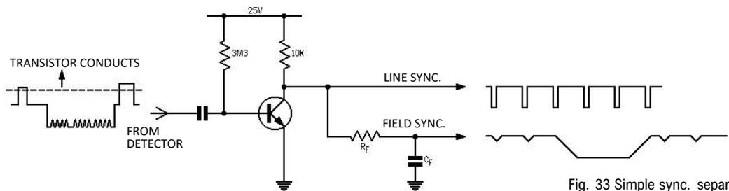
Fig. 33 Simple sync. separator
