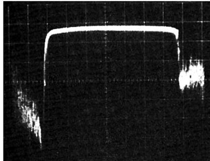
Fig.27. As Fig.26 but with input signal at 60 dB into amplitude limiting, showing even further widening of the characteristic at this level, corresponding to about 530kHz.
