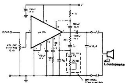
Fig. 2. A  $\mu$ A706 circuit using a minimum number of components.
