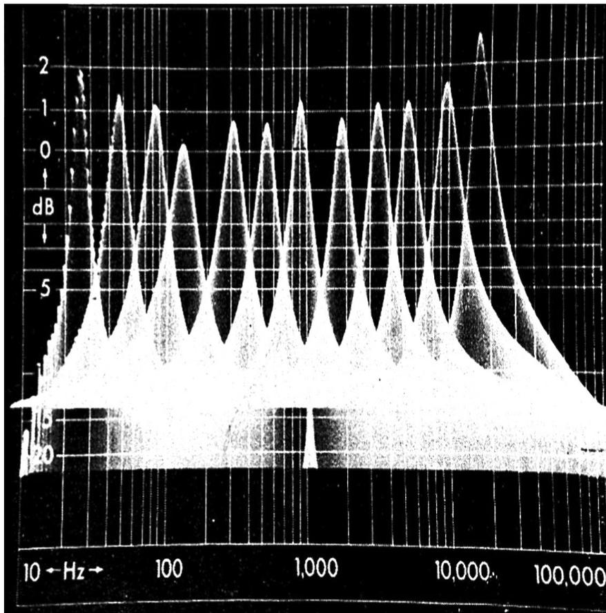
Fig.31. The individual responses of twelve filter controls on a graphic equaliser taken by frequency sweep testing and superimposed photographs.
