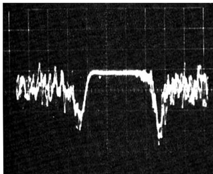
Fig.26. Overall FM selectivity with input signal 6 dB into amplitude limiting, Horizontal calibration 8 0kHz/div showing effective bandwidth of 240kHz. The requirement for good stereo based on a phase linear characteristic.
