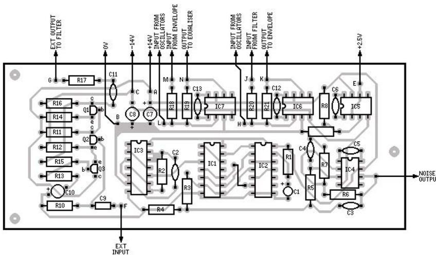
Fig. 4. Component overlay for the auxiliary board. The PCB is flipped from left to right.
