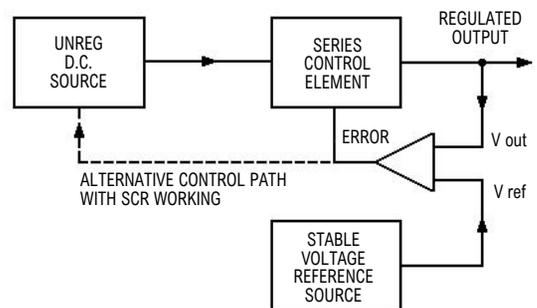
Fig. 9. Generalised diagram of active feedback type regulator.
