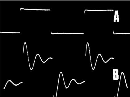
Fig. 11. Square-wave test for ringing, (A) Input signal (B) Output from amplifier showing severe ringing due to inductive circuitry. Frequency of ring is about 5kHz.
