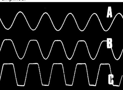
Fig. 19. Examples of clipping. (A) Clean sine-wave form generator. (B) and (C) Asymmetrical and symmetrical clipping due to overload, or malfunction of the amplifier under test.
