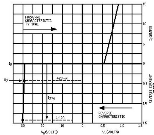
Fig. 4. In a zener diode the reverse breakdown region is used to provide a constant voltage as current demand varies.
