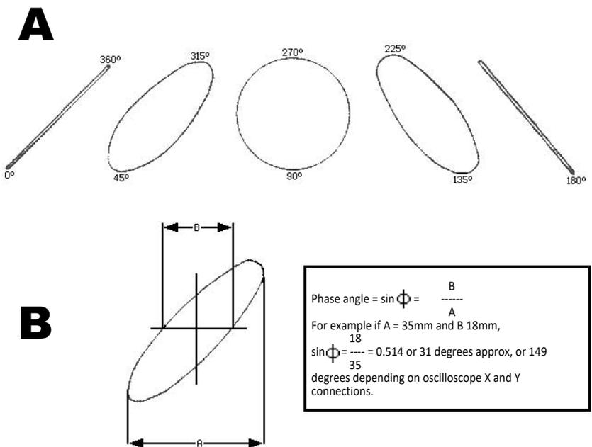
Fig.9 (A). Phase angles. See text for explanation. (B) Determination of phase angle from an oscilloscope.
