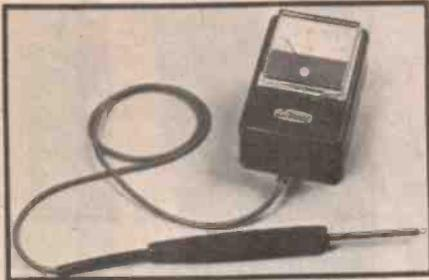
specially calibrated high quality moving coil meter which incorporates automatic cold junction compensation. The range of the pyrometer is from zero to 500 degrees Celcius with a scale marked every twenty degrees.
