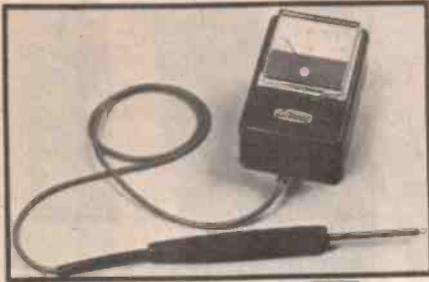
specially calibrated high quality moving coil meter which incorporates automatic cold junction compensation. The range of the pyrometer is from zero to 500 degrees Celcius with a scale marked every twenty degrees.
