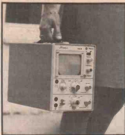
is a 'beam-locate' button — extremely useful for laboratory or experimental work. The circuit includes a really excellent trigger control — this is not a Scopex claim but showed up when ETI had a chance to play with one briefly.
