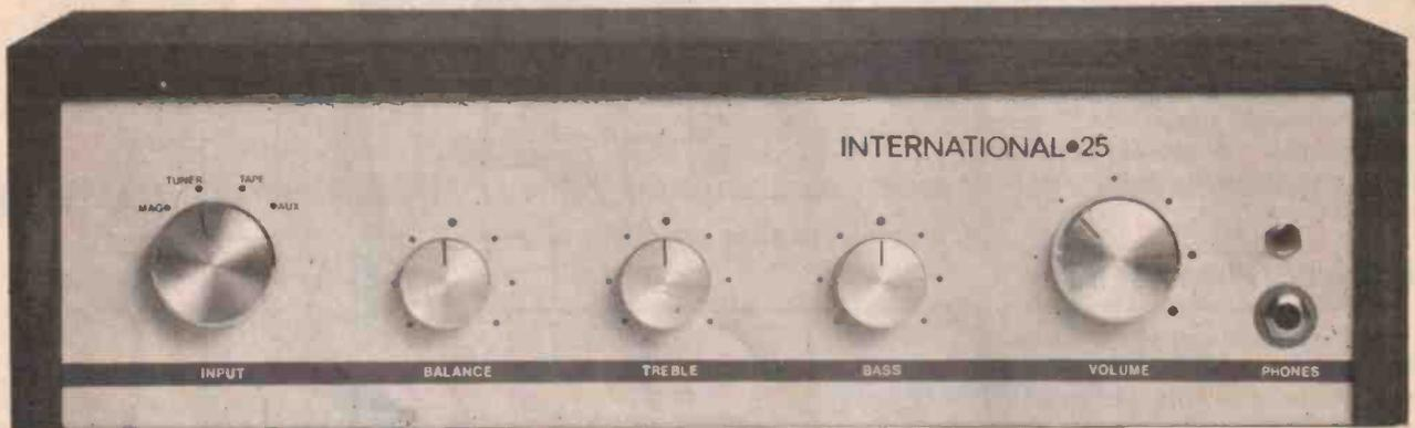
This second part completes the details for building the INTERNATIONAL-25 amplifier. This high fidelity 25W per channel amp matches the INTERNATIONAL-FM tuner in our September and October issues. This project is built on one pcb and does not require any advanced knowledge of electronics.
