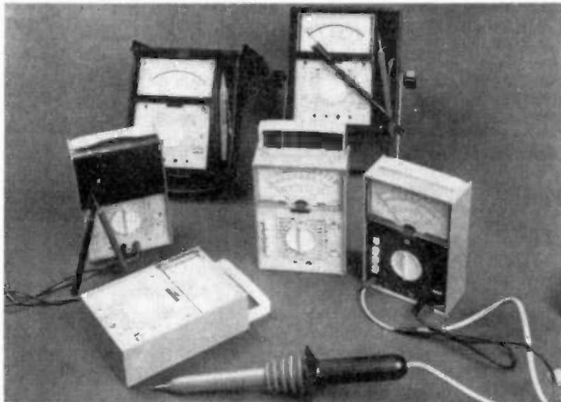
Western Instruments have released a new VOM series, one major feature of which is their 'invulnerability'. All five models in the 660 series are drop-proof and feature a custom rugged self-shielded taut-band mechanism, diode-protected meter movement, temperature compensation, pluggable circuit board assemblies,
