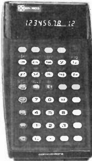
rechargeable cassette. The machine uses algebraic logic and is fully guaranteed for 1 year. A 12-digit green display gives 8-digit mantissa and 2-digit exponent plus signs. The functions of the calculator are:
