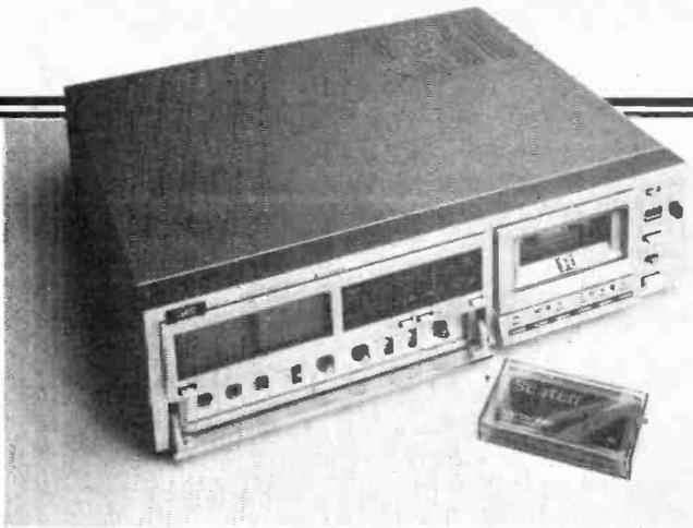
Left: JVC's KDA8 computerised cassette deck. It fixes up its own own bias and equalisation levels, and can cope with metal tape.
