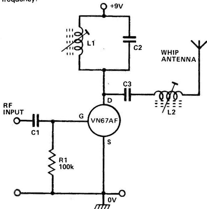
**Fig 21. 60mW R/C or CW transmitter L1-C2 is tank circuit, C3-L2 is the antenna circuit.**
