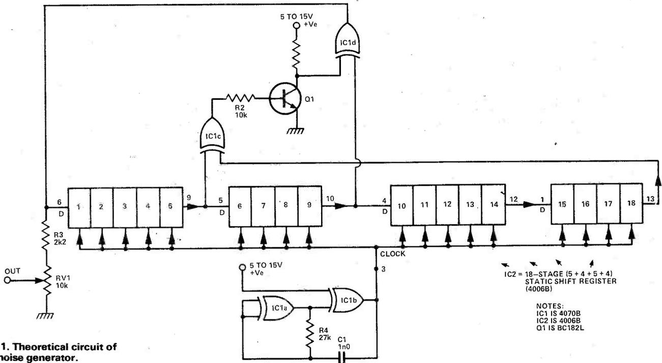
Fig. 1. Theoretical circuit of the noise generator.
