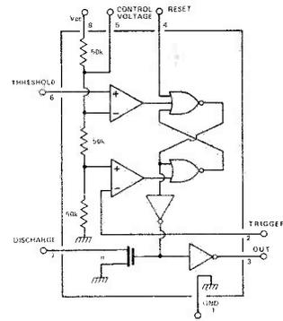
Fig. 9. The internal circuitry of the CMOS 555.
