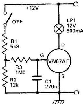
Fig. 17 the lamp turns on slowly when the switch is closed as C1 charges up via R3, and turns off slowly when the switch is opened as C1 discharges via R3.
