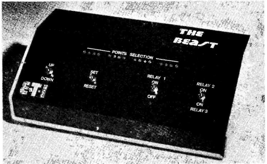
The points controller (above) can control up to sixteen sets of points or relays. It can activate several times per second. The set of points chosen is shown on the row of LEDs on the front panel. Think about your own particular points control needs before you start to build this unit. The data distribution unit is shown on page 91.
