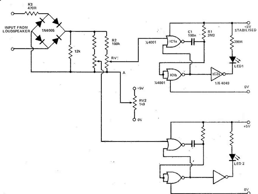
threshold limit is largely overcome by using RV2 to bias point A to just below the threshold voltage. In practice, the circuit operates on an input frequency of from less than 5 Hz to more than 50 kHz sine wave and at an input voltage of from approximately 1V4 RMS (0.25 W into 8R) to more than 90 V RMS (1 kW into 8R). A single positive or negative 4 μS wide pulse will also operate the circuit.
