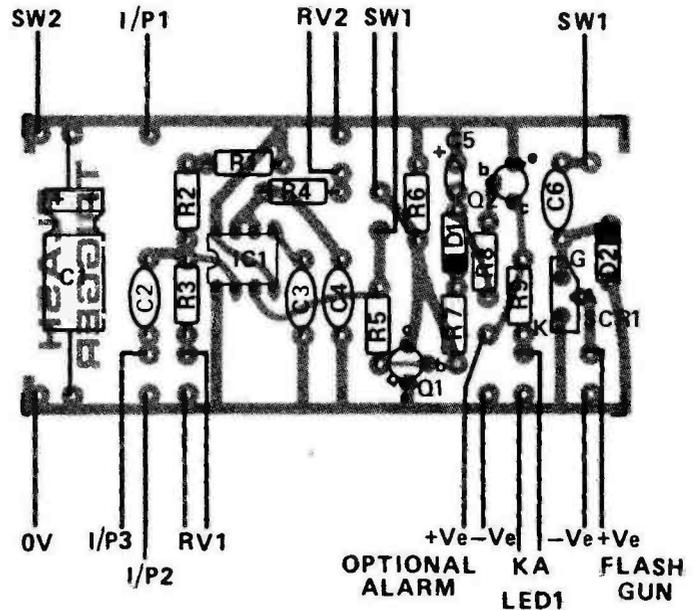
Fig. 3. Component overlay.
