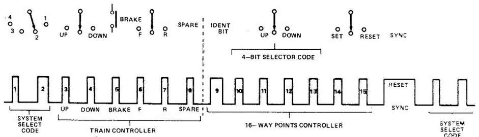
Fig. 1. The 15-bit 'simultaneous' code used by the remote control system.
