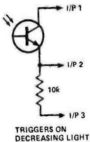
Photo transistor is TIL78
