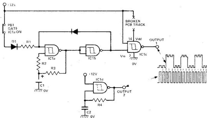
**Fig. 5. A broken track caused problems in this 4093B dual oscillator, but proved difficult to find.**
