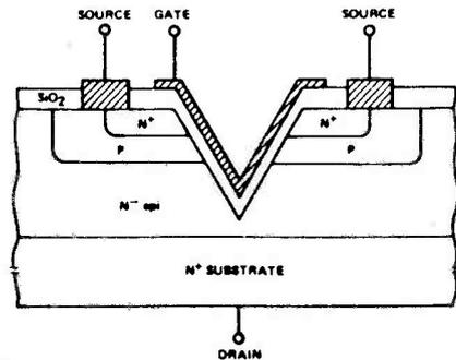
Fig 2. Cross Section of a VMOS power FET.
