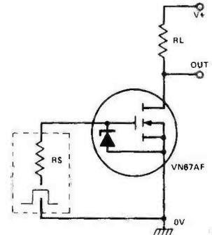
The rise and fall times of the output of the circuit are determined by the source impedance of the input signal, the input capacitance and forward transconductance of the VMOS device and the value of R<sub>L</sub>. If R<sub>L</sub> is large compared to R<sub>S</sub> the VN67AF gives rise and fall times of roughly 0.11 nS per ohm of R<sub>S</sub> resistance. Thus, a 100R source impedance gives an 11 nS rise or fall time.
