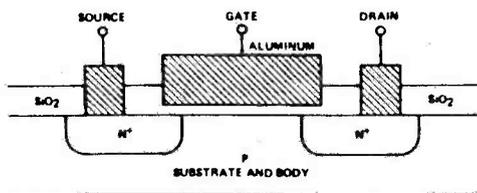
Fig 1. Cross Section of a conventional FET.
