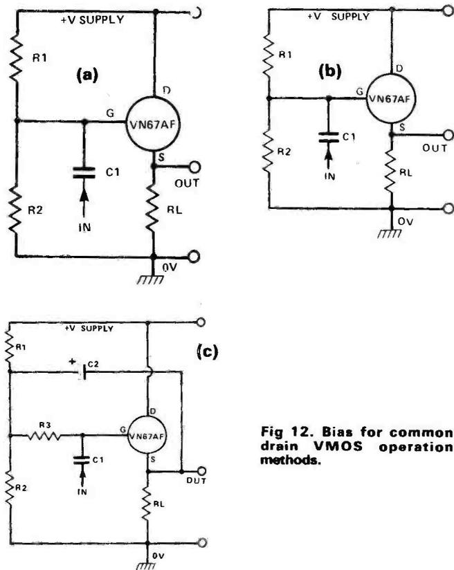
**Fig 12. Bias for common drain VMOS operation methods.**
