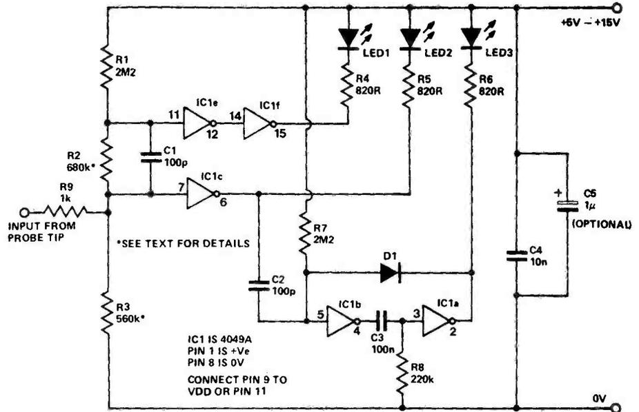
Fig.1. Circuit diagram. Note the polarity of LEDs 1, 2 and 3.
