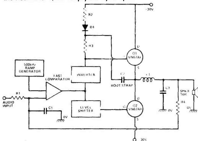
**Fig 22. Basic circuit of a 20W class-D switched-mode audio power amplifier. An ideal application for VMOS.**
