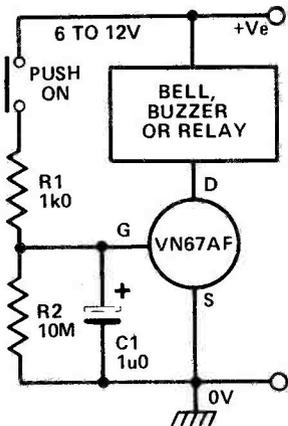
**Fig 15. Delay turn off switch.**
