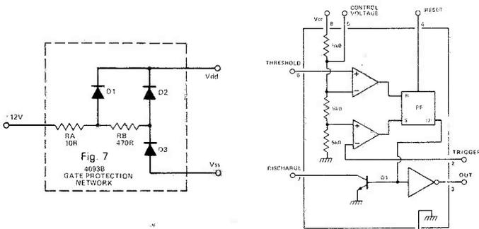
Fig. 7 (left) the internal gate protection network of the 4093B. Fig. 8 (right) The internal circuitry of the familiar bipolar 5555.
