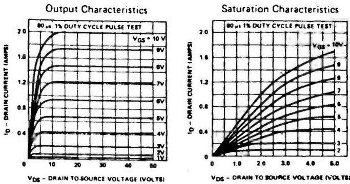
Fig 3. Output and saturation characteristics of the VN67AF VMOS power FET.
