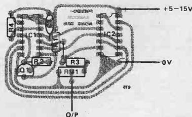
Fig. 3. Component overlay.
