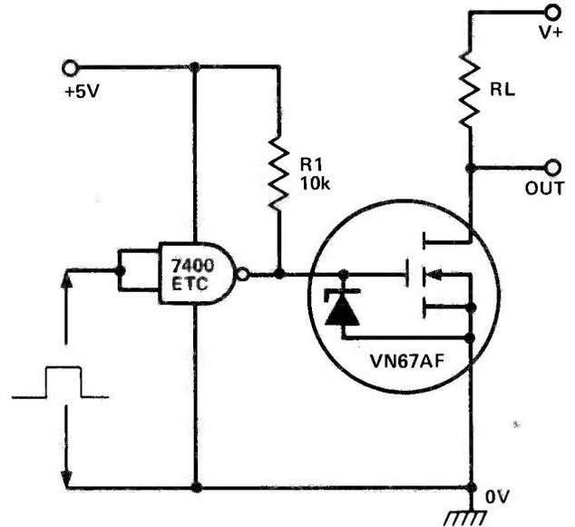
Fig 9. VMOS can be driven from the output of TTL if a pull-up resistor (R1) is used.
