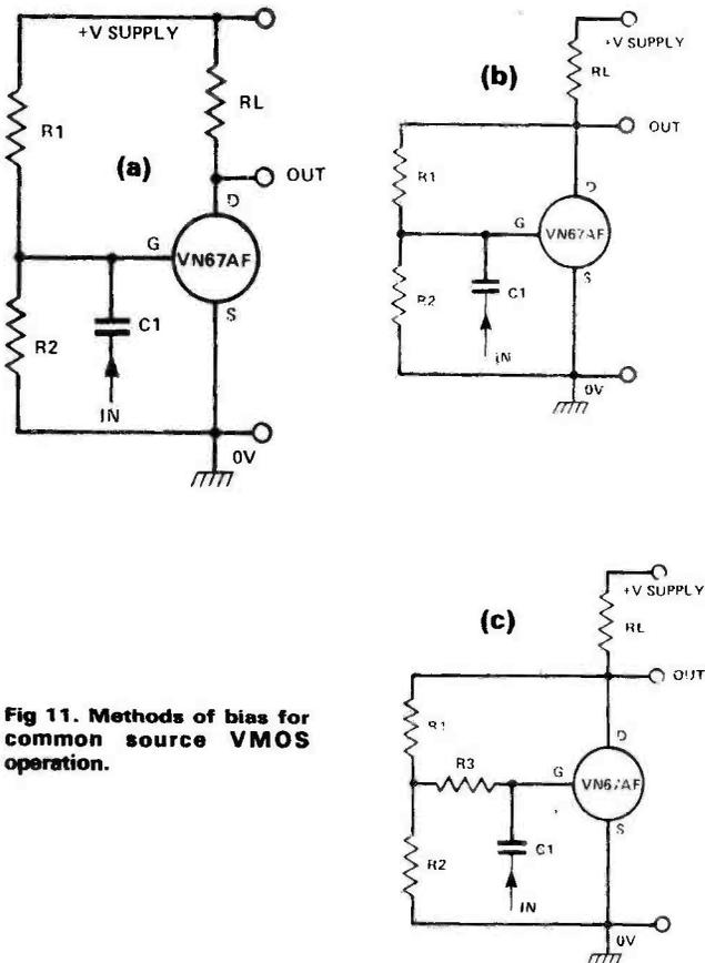
**Fig 11. Methods of bias for common source VMOS operation.**
