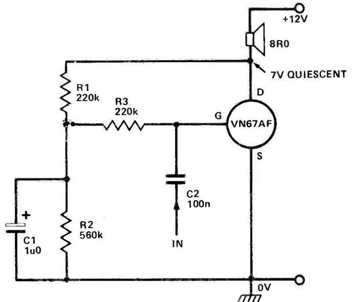
**Fig 20. Super simple class-A amplifier.**
