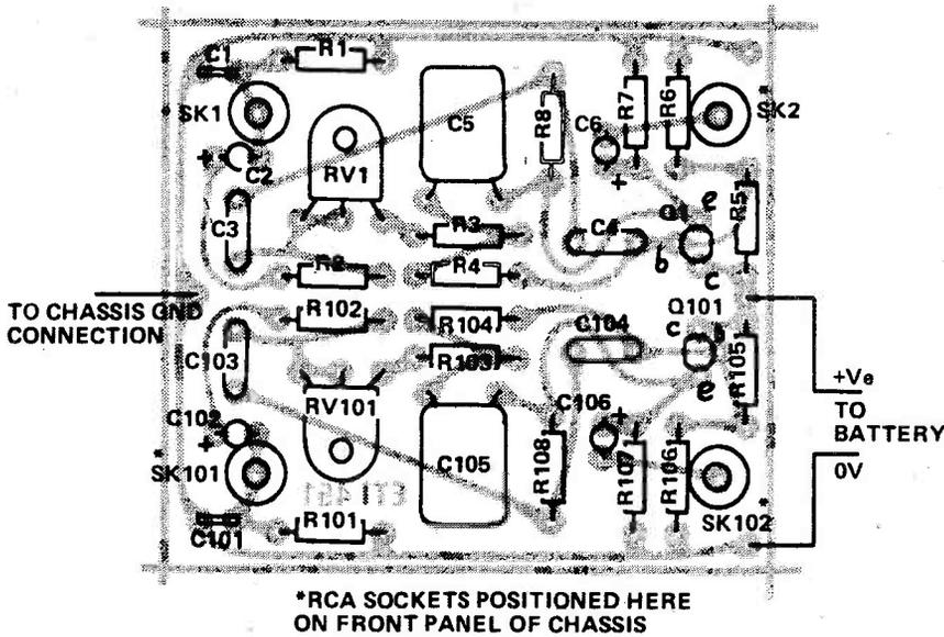
Fig.2. Component overlay.
