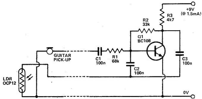
shining on the LDR, the higher the frequency-range boosted by the circuit.
