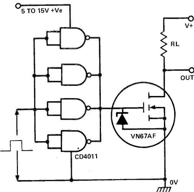
Fig 8. VMOS switching times can be reduced by driving with a number of gates in parallel. Typical  $R_T = 25 \text{ nS}$ .
