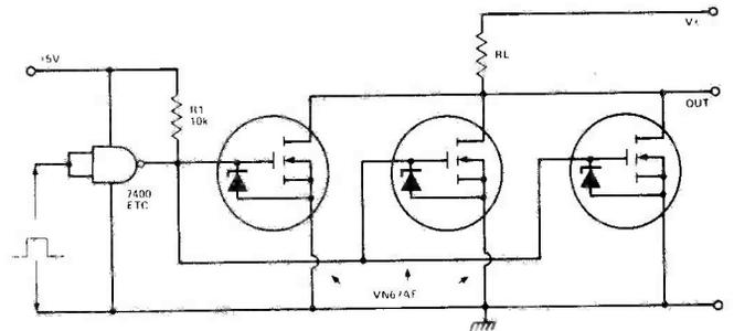
Fig 10. Boosting the output of Fig 9 by driving three VN67AF in parallel.
