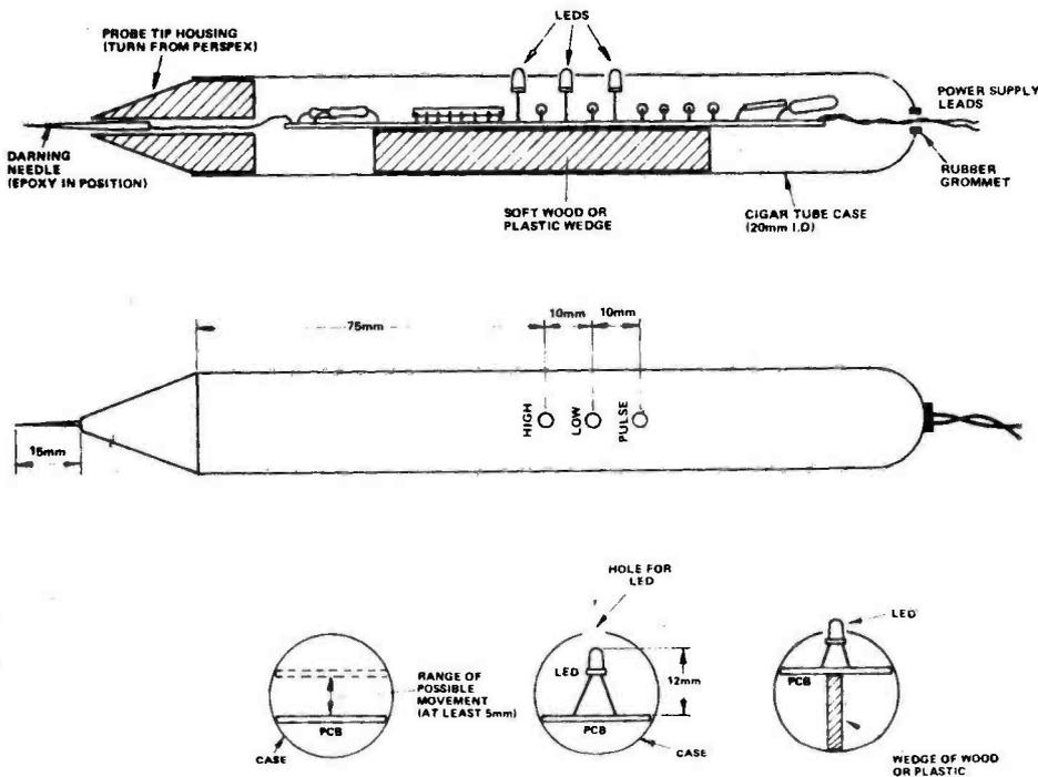
Fig.3. The PCB slides into the cigar tube and rests on a piece of wood or plastic.
