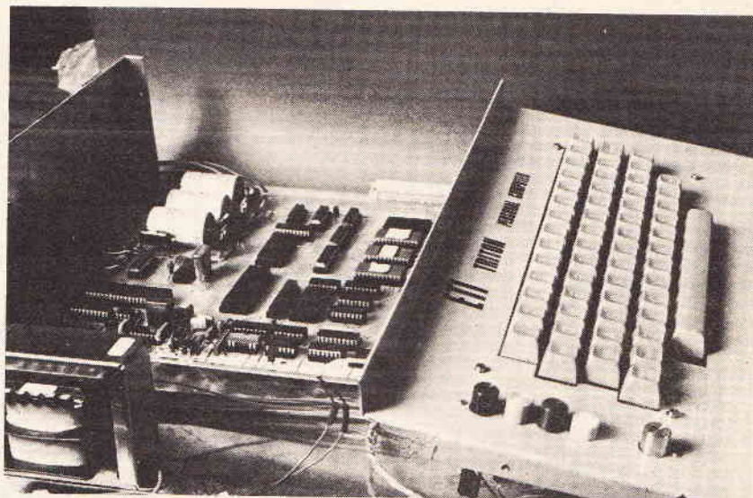
The Triton's board mounted in its case. Note that the extender socket is available on the right hand side of the case and that the output of the modulator is brought out to a UHF socket on the back panel. The back panel also carries the DIN sockets and the mains fuse.
