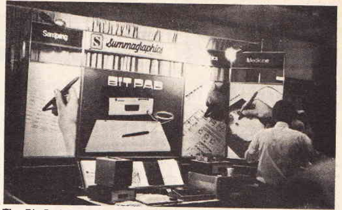
The Bit Pad is a rather nice (but expensive) device for turning freehand into computer input.
