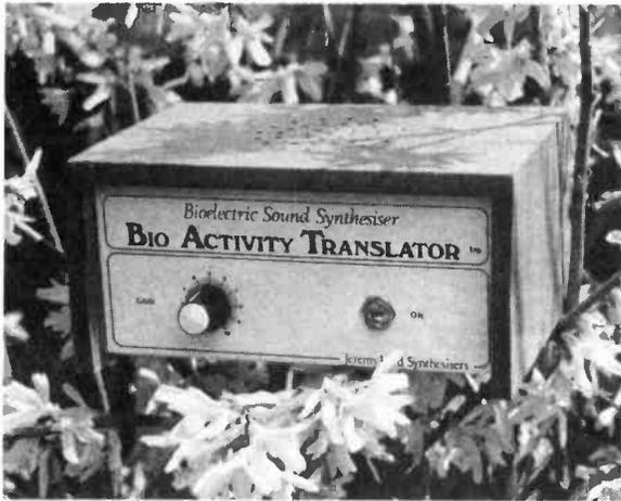
Natural Bio Electric signals are monitored by an electrode attached to the leaf. When amplified and filtered, a VCO, VCA and other exclusive synthesiser circuits are controlled by the potential to produce tracking sequences of notes. These follow in pitch, rhythm and volume the ever changing signal.
