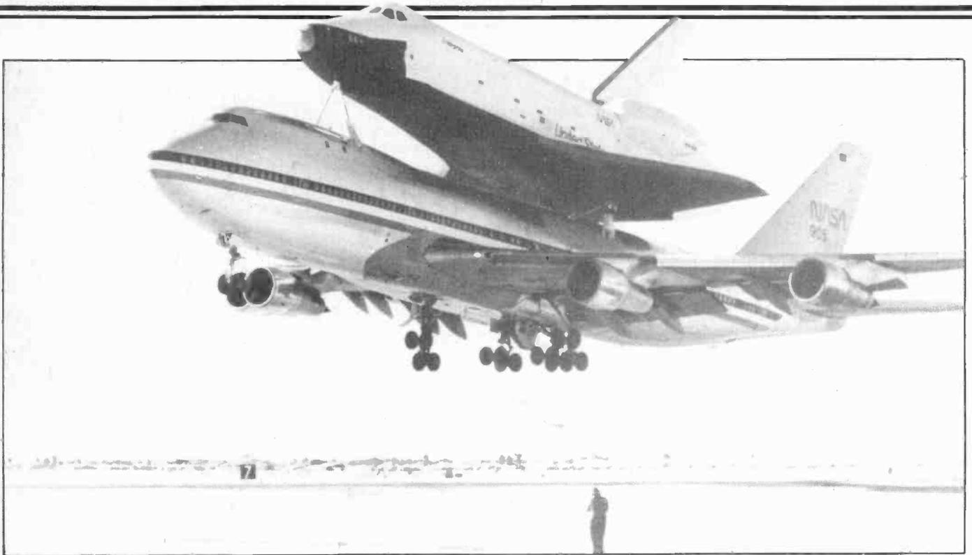
The first captive flight of America's Space Shuttle on the back of a NASA 747.
