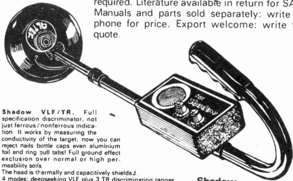
**Shadow VLF/TR.** Full specification discriminator, not just ferrous/nonferrous indication. It works by measuring the conductivity of the target, now you can reject nails bottle caps even aluminium foil and ring pull tabs! Full ground effect exclusion over normal or high permeability soils.
