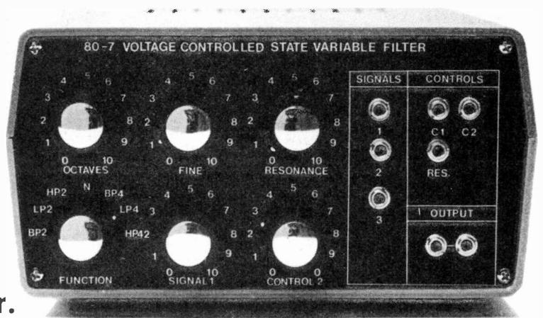
The Voltage Controlled State Variable Filter has low pass, high pass, band pass and notch filtering capabilities. The first three responses are available as both two pole (12 dB/octave) and four pole (24 dB/octave) filters. Manual and external control of resonance is included.
