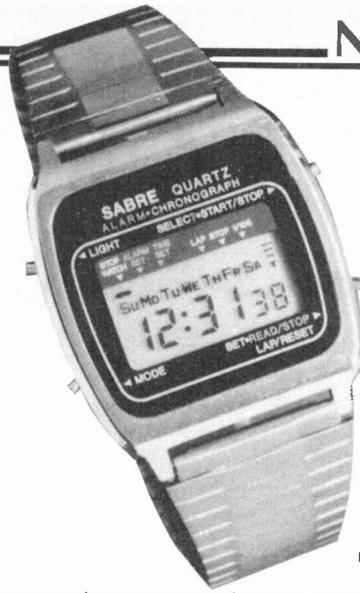
New generation of quartz LCD Watches. Sabre Alarm Chronograph uses standard watch cells and measures only 3.9 mm thickness.
