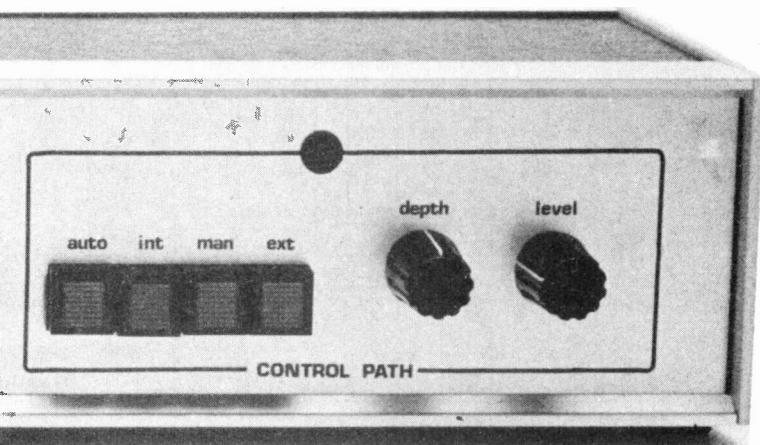
This box of tricks gives you the opportunity to try out what has up to now been an effect used predominantly in the studio. The stereo sound image can be controlled automatically or manually. You can position the image in one place and keep it there or continually sweep the image between channels ..... and more.
