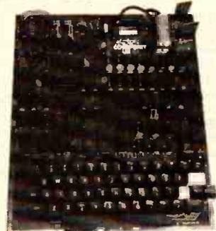
★ 6502 based system — best value for money on the market. ★ Powerful 8K Basic — Fastest around ★ Full Qwerty Keyboard ★ 4K RAM Expandable to 8K on board. ★ Power supply and RF Modulator on board. ★ No Extras needed — Plug-in and go. ★ Kansas City Tape Interface on board. ★ Free Sampler Tape including powerful Disassembler and Monitor with each Kit. ★ If you want to learn about Micros, but didn't know which machine to buy then **this is the machine for you.**
