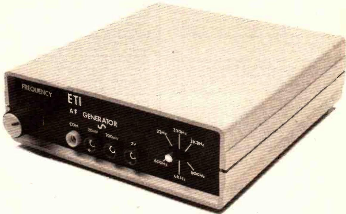
Good quality sine/square generators, giving very low sine/wave distortion, are invaluable pieces of test gear but tend to be rather expensive. For the vast majority of practical applications, such as gain and frequency response testing, function checking and sound generation, etc, the expensive 'very low distortion' sine wave characteristic is, however, superfluous, since distortion factors up to several percent are quite acceptable in such applications.
