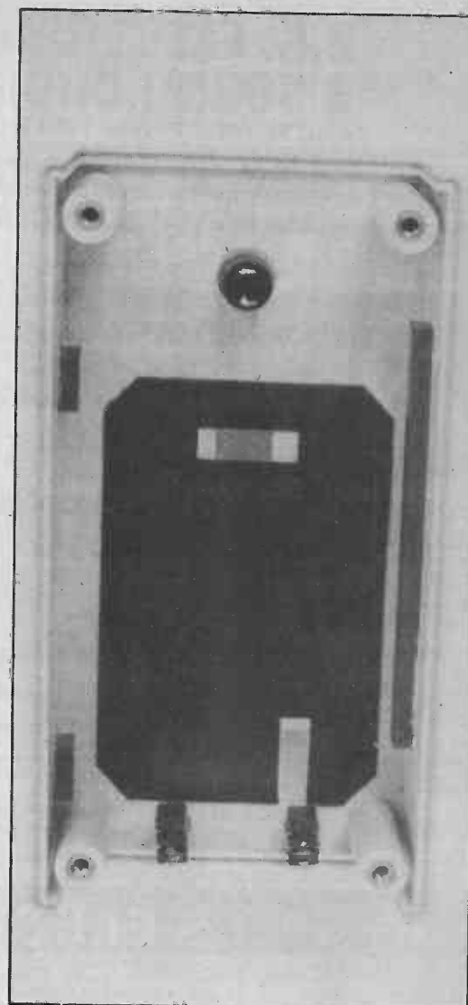
This photograph shows the red filter and plastic mounting strips glued into the top of the case.
