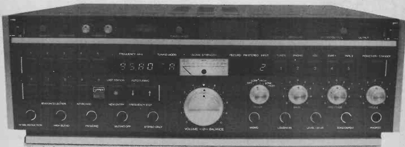
Above: the Revox with its hair down, revealing the little used and hence well-disguised controls for tuner threshold determination, speaker output selection and record output on/off.
