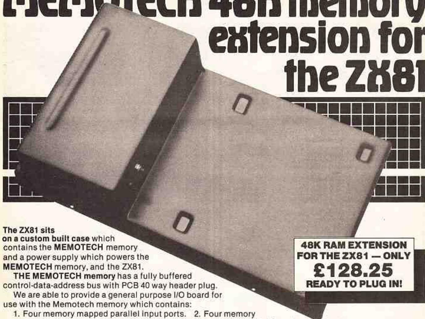
The ZX81 sits on a custom built case which contains the MEMOTECH memory and a power supply which powers the MEMOTECH memory, and the ZX81.
