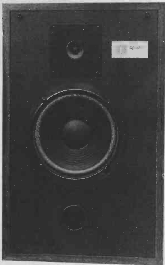
A de-grilled Radiance R82 — the acceptable face of hi-fi. On the backside, so to speak, you'll find the three-position treble control and some unusual rotary-locking speaker terminals.
