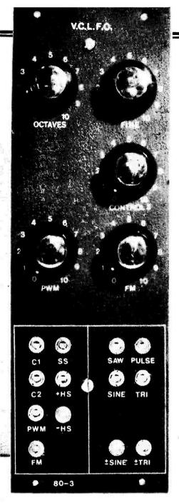
Above: both versions of the VCO, panel mounted for rack fixing. Note that all inputs/outputs are at the bottom of the panel to prevent wiring fouling the con-
