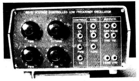
Above and below: the inside and outsides of a low frequency VCO. The PCB is panel mounted just to show we did both ways! This method of construction is best suited to professional (or *very* serious amateur) use.
