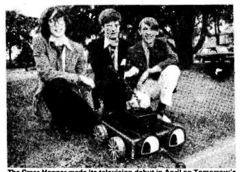
The Grass Hopper made its television debut in April on Tomorrow's World. Designed by Frank Carver, it's an admirably practical robot for armchair gardeners — it cuts grass. The design team, from Faraborough 6th form college have since produced a Mk 2 CMOS version.
