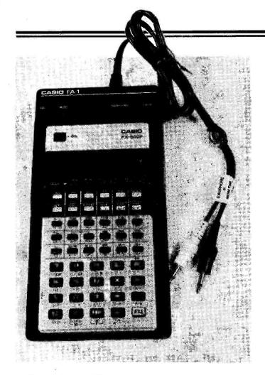
Left: the calculator nicely settled into its FA1 tape adaptor. Two slots in the holder engage the black lugs along the calculator sides to ensure a good alignment between the (gold plated) plug and socket.
