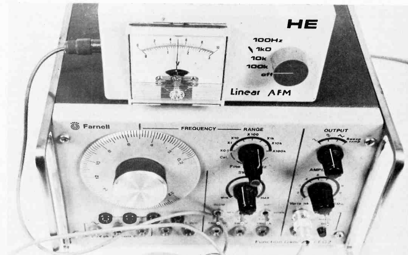
Calibrating the Audio Analogue Frequency Meter against the workshop signal generator. For those without any test equipment an alternative method is outlined in the text.
