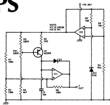
voltage supplied by the 741.Comparator IC1 is used as a Schmitt trigger, the output of which is used to discharge C1 via D1. To calibrate the circuit Q1 is immersed in boiling distilled water and PR1 adjusted to give 1 kHz output.
