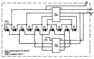
Fig.4. (left) Circuit diagram of the Power Amplifier. Fig.5. (above) Circuit diagram of the Bargraph Monitor.
