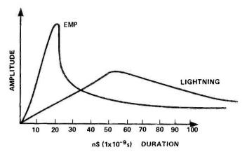
Fig. 4. Comparative rise-times of an EMP from a 1 Mt. bomb and an average lightning flash. Note that the EMP is many times faster.
