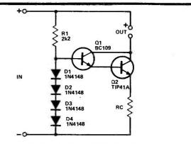
The value of RC is equal to 1,500 divided by the required output current in milliamps and would, for example, be 10 R for rapid charge Ni-Cads requiring a charge current of 150 mA (1,500 divided by 150 = 10 R).
