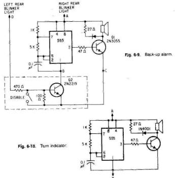
oscillator as normal and point D supplies power to the base of transistor Q2. This turns the transistor on and effectively shorts it to ground, causing the oscillator to work.
