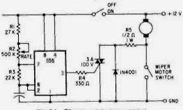
Fig. 6-4, Thyristor-switched wiper control.
