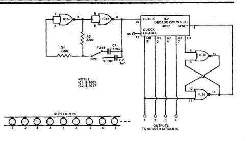
be simply power transistors for low voltage lamps or triacs for seriesconnected mains operated lamps. The outputs of the driver circuits are connected to the lamps in groups as shown.
