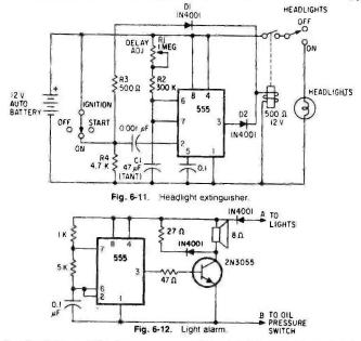
circuits, this one (Fig. 6-12) is composed chiefly of an amplified astable multivibrator. In addition, there is a diode in the positive power lead to protect the circuit from reverse voltages. Operation is very simple. When the ignition is on and the headlights are on, both point A and point B have +12 V applied to them, and the circuit has zero voltage drop across it so it does not operate.
