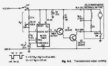
A transistor and a couple of resistors can be added to the circuit for better cold-weather starting. During starting, the transistor holds the timer in its off state lightening the load on the car's cranking motor. (And to prevent radio interference, a  $10-\mu F$  capacitor can be connected from the Darlington emitter to ground.)
