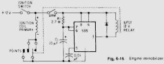
the output of the timer will go low again and the relay will turn onshorting out the points and cutting off the ignition circuit.
