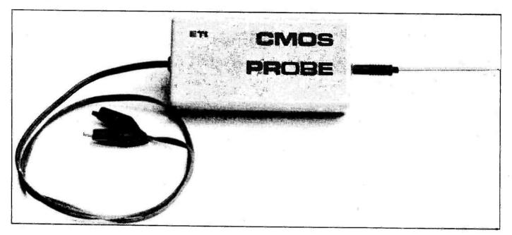
his unit, powered from the equipment under test, enables the voltage levels of CMOS circuitry to be checked to determine if they are within the valid logic range. Two LEDs are used to indicate high and low logic levels, invalid levels and open circuit conditions.
