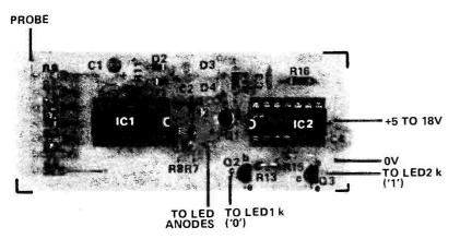
Fig.2. (above) Component overlay. Note the orientation of IC1 and IC2. Board construction is straightforward.
