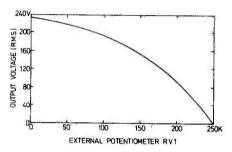
Fig. 2 Variation of output voltage with RV1. (input voltage = 240 RMS)
