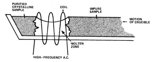
Fig.2. The heating effect of high frequencey AC can be put to good use in semiconductor material manufacture.
