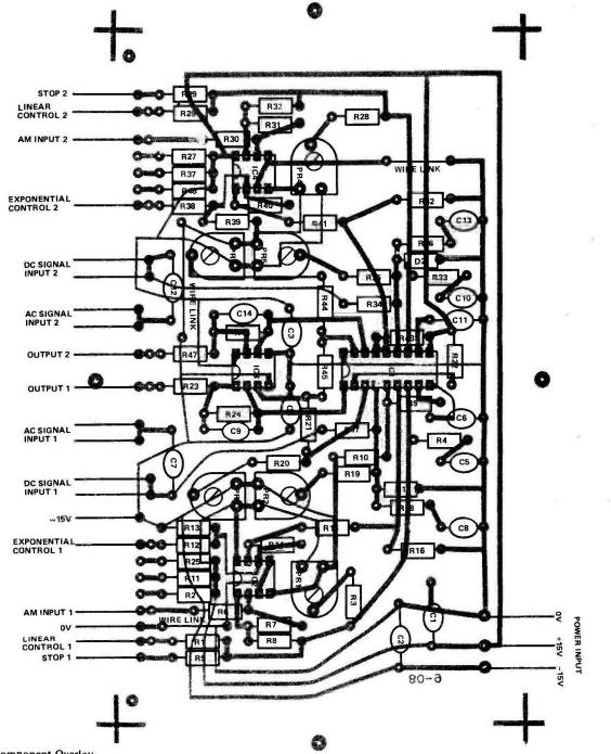
Fig.2. Component Overlay.
