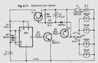
is produced by a 555 astable, but the most important part of the circuit is the circuitry that adapts the one-pole, three-position switch normally found in cars for operation with this circuit, which would ordinarily need a two-pole, three-position switch.
