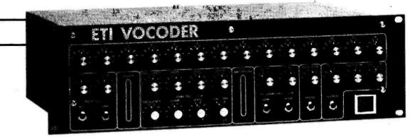
Now you can make your own synthesiser or guitar or even your cat speak or sing to you. This design uses 14 channels and has all the goodies like LED PPM meters, slew rate control, voiced/unvoiced detector and very versatile internal excitation! What more could you ask for? The ETI Vocoder's got the lot.
