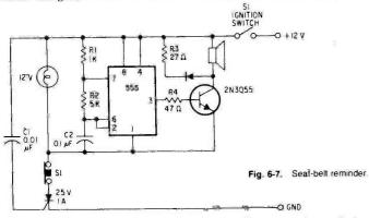
of an SCR via pushbutton S1. As long as the SCR is not triggered, the oscillator will not operate.
