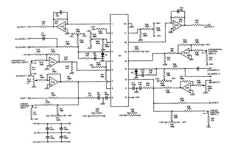
Fig.1. Circuit diagram of the Project 80 Dual VCA.
