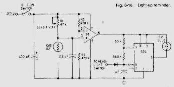
switch on your headlights. And, if you replace the astable circuit with a monostable and a relay, you can even have it turn the lights on for you automatically.
