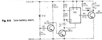
However, if the voltage at the input to the circuit drops below 10 V, the zener diode will stop conducting and Q1 will turn off. This will cause Q2 to turn on, and will supply a ground return for the 555 oscillator, resulting in a tone being generated.
