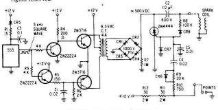
Fig. 6-1. Electronic ignition system
