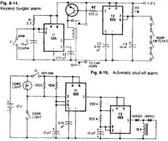
capacitor starts to charge up. This will take about 11 sec with the components shown. After 11 sec, the output voltage on pin 3 of T2 drops, and causes the transistor to turn on.
