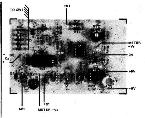
Fig.3. Component overlay. Note the orientation of the ICs. Insert them the wrong way at your peril.
