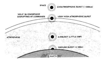
Fig. 1. The different methods of detonation of a nuclear device. Note that an airburst will maximise damage to surrounding environments physically but minimize EMP.
