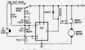
Fig. 6-5. Relay-switched wiper control
