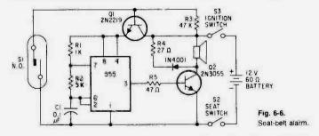
taped to the seat-belt buckle in such a way that when the seat belt is properly secured, they are in close proximity to one another.
