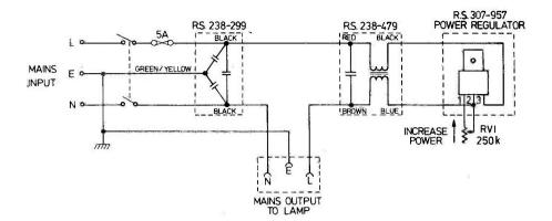
which corresponds to a maximum power transfer of approximately 98% for a resistive load. The graph shows how the output voltage varies with various values of R V 1. When used at full load current, the device should be mounted on a heat sink having a thermal rating of 4°C/watt (eg RS 401-497). Alternatively, as the tab is electrically isolated, it may be fixed directly to the chassis for heat dissipation.
