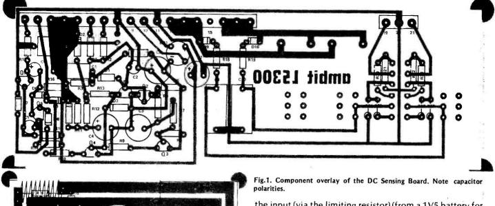
the input (via the limiting resistor) (from a 1V5 battery for example) causes the relay to drop out and the LED to start flashing again.
