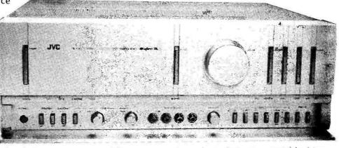
amplifier range and employs their new variable bias circuit, which is claimed to allow class A operation at much higher powers than has hitherto been possible by increasing the efficiency of power transfer.
