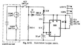
The output of the oscillator drives a relay. Diode D2 is used to prevent the timer from latching on due to the back emf generated by the relay coil. If a double-pole relay is used, the circuit can turn both the horn and the headlights on and off. The horn blowing will surely scare away any potential thief, and the flashing headlights will indicate to passersby which car is being tampered with.
