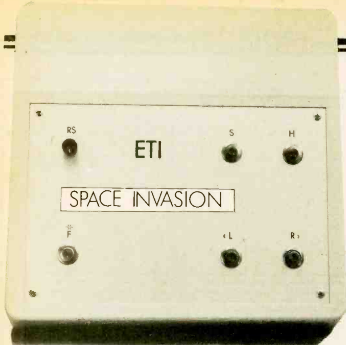
The face of the Space Invasion. The simple controls are reset, start (play), hold, fire, left and right.
