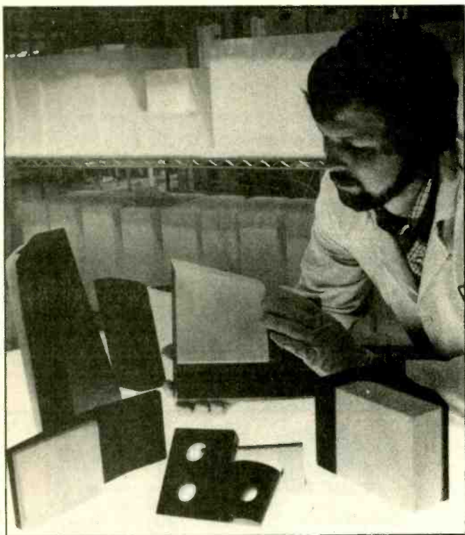
At the Lockheed plant in Sunnyvale, California, a technician examines some of the silica tiles manufactured for the Space Shuttle. As each tile is shaped to fit only one spot on the spacecraft, no two tiles are the same.
