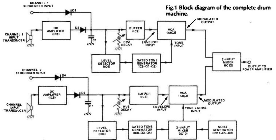
Fig.1 Block diagram of the complete drum machine.
