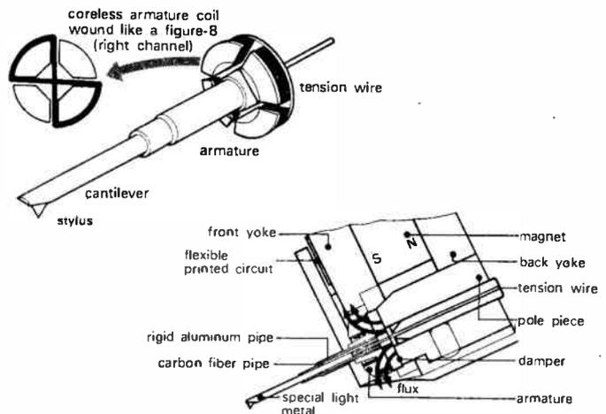
**Fig. 6** A cross-section of a Sony moving coil pickup, showing how the coils are miniaturised to decrease the mass of the moving element, thus improving transient behaviour.
