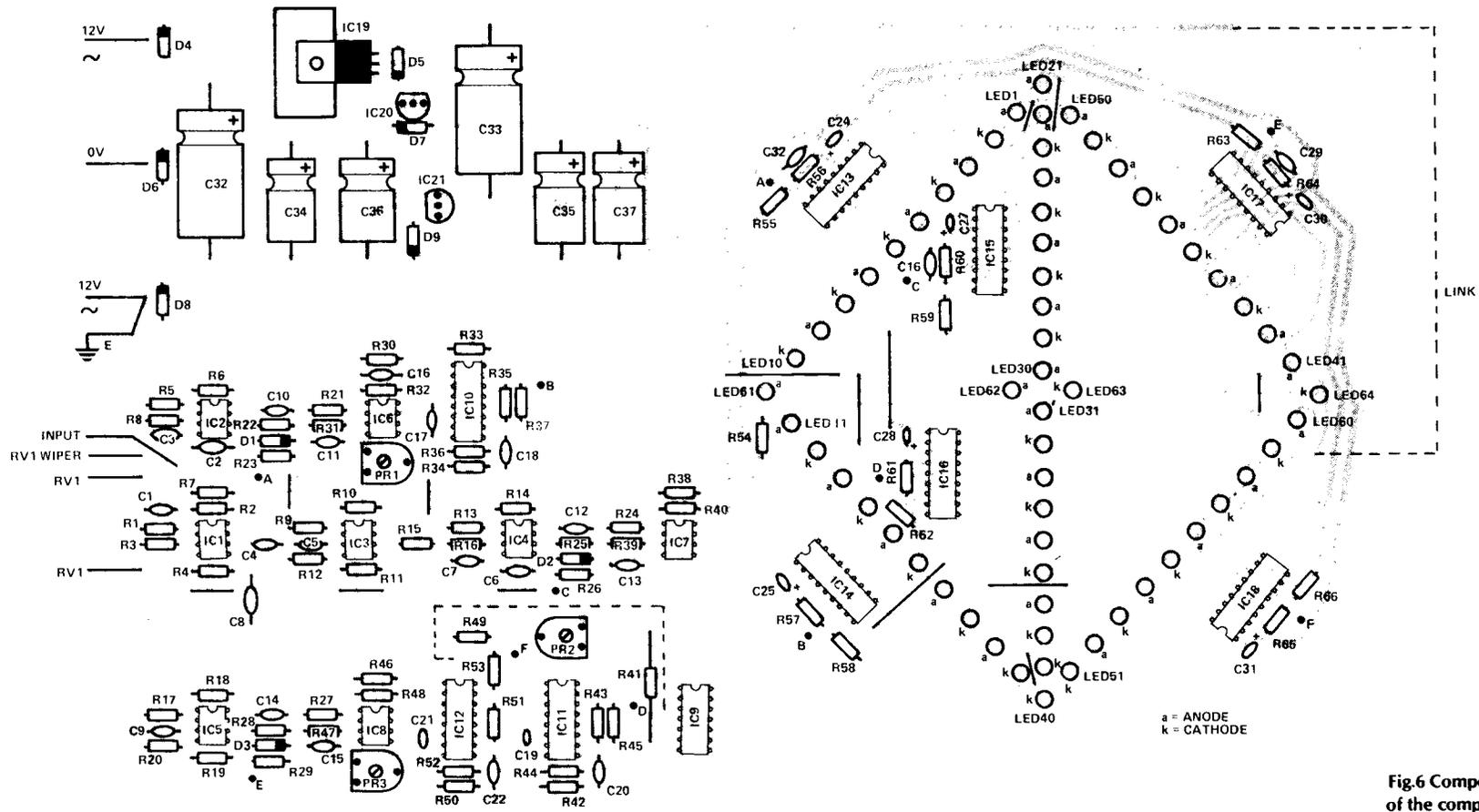
Fig.6 Component overlay of the complete VCSA.
