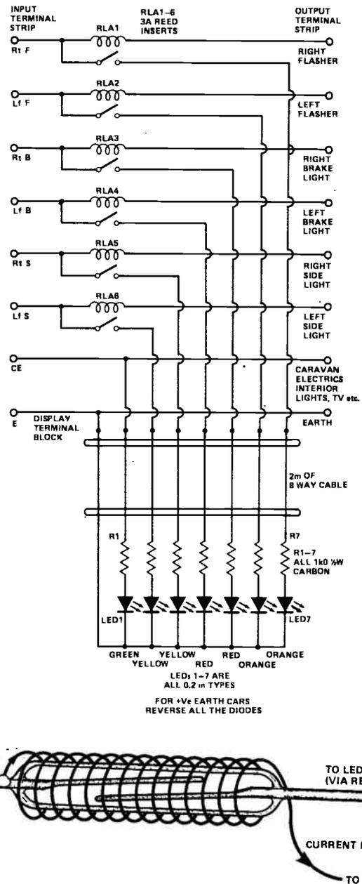
Fig. 2 Circuit diagram with relay assembly/wiring details.
