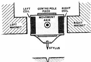
Fig. 2 Moving coil cartridge basics. As the stylus moves the coils, a current is generated within them by the magnetic field from the fixed magnets.
