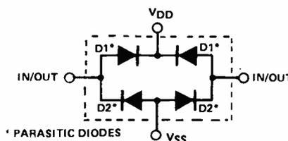
Fig. 3 The 4066B quad bilateral switch has standard B-series protection on its gate control input terminals, but has this simplified form of protection on its 'switch' elements.
