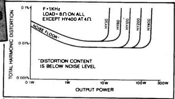
Load impedance all models 4Ω-∞ Input impedance all models 100KΩ
