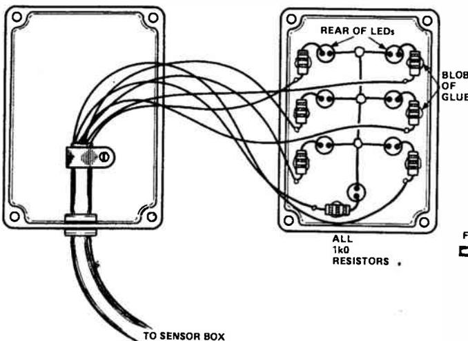
Fig. 1 Construction details of the display box.
