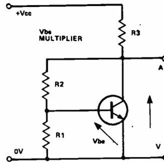
R3 limits the current through the parallel combination of the transistor and R1/R2. Suppose as an example that  $V_{cc}$  tries to rise. The potential divider formed by the three resistors will try to raise the voltage across R1. This will tend to increase the collector current and thus increase the potential drop across R3, leading to a stabilising effect at point A. This is a case of voltage-derived series feedback.
