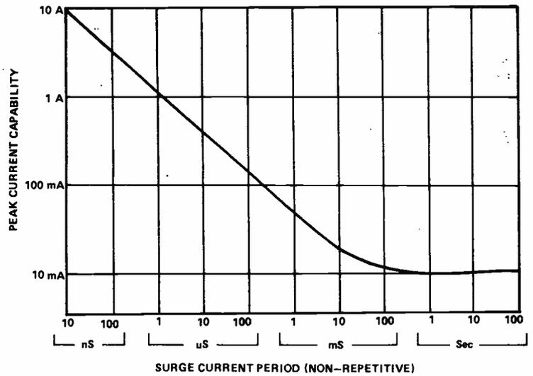
Fig. 6 Typical surge-current capabilities of CMOS protection diodes.
