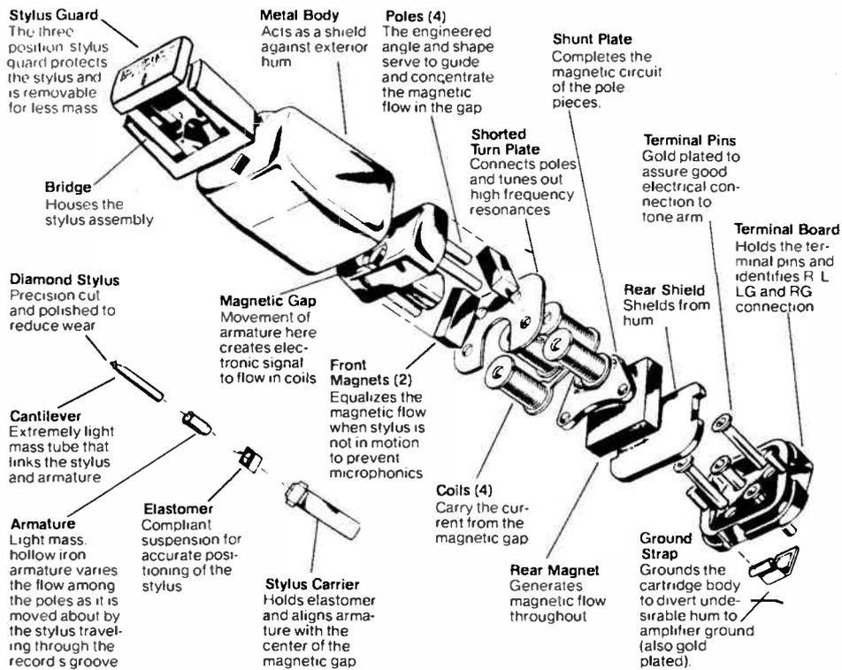
**Fig. 5** This exploded view of an Empire induced magnet design gives an indication of the lengths that top manufacturers will go to in order to beat resonances and colourations.
