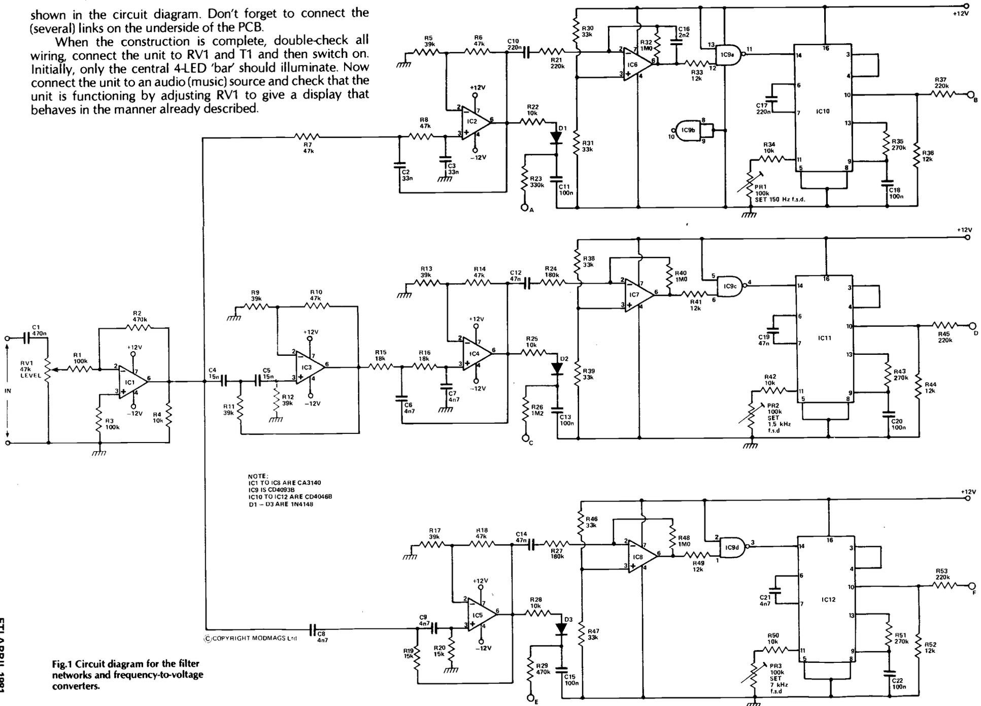
Fig.1 Circuit diagram for the filter networks and frequency-to-voltage converters.
