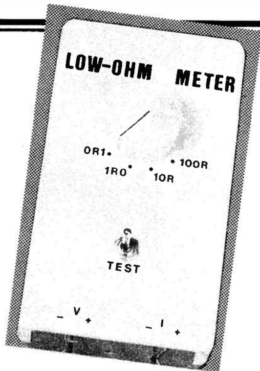
Ever wanted to measure the resistance of a transformer winding or a suspect solder joint, but found that your trusty multimeter wasn't sensitive enough to do the job? If so, our Low-Ohm Meter will solve your problems. It accurately measures resistances from a hundred ohms down to a few milliohms, in four decade ranges, using a precision four-terminal measuring technique that eliminates the effect of connecting leads, etc. from the readings.
