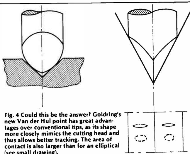
Fig. 4 Could this be the answer? Goldring's new Van der Hul point has great advantages over conventional tips, as its shape more closely mimics the cutting head and thus allows better tracking. The area of contact is also larger than for an elliptical (see small drawing).
