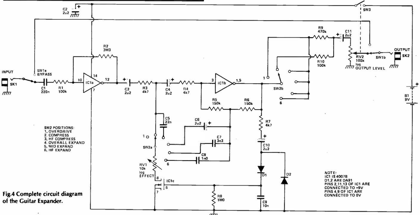
Fig.4 Complete circuit diagram of the Guitar Expander.
