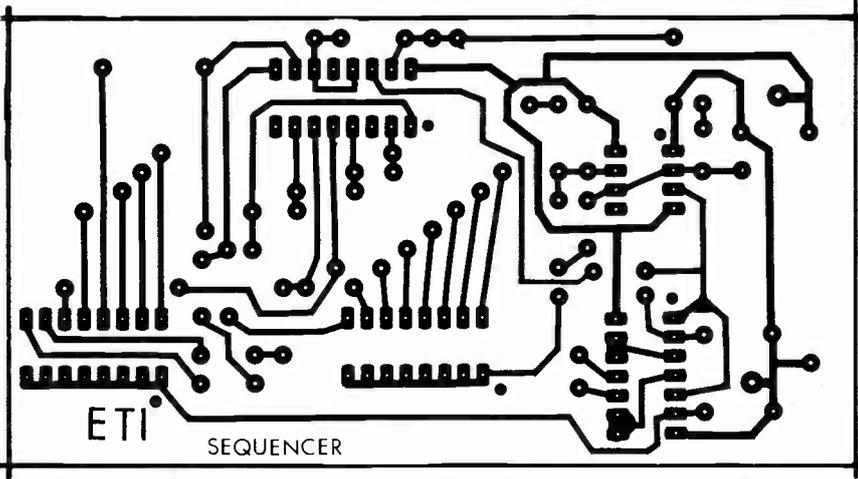
Above and below: The two foil patterns for the ETI Drum Machine.
