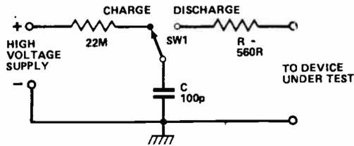
Fig. 4 Manufacturers use this equivalent-body discharge network when evaluating the capabilities of their CMOS protection networks.
