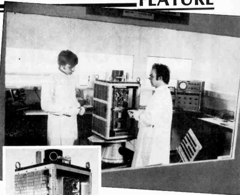
Left: the aluminium alloy frame of the spacecraft contains 16 boxes machined from solid aluminium. Each box holds two PCBs. In all UOSAT will use about 400 ICs. Below: UOSAT in position, mounted on the Delta 2310 launch vehicle during a trial mating in December 1980.
