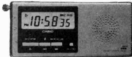
Large LC Display of full digital time. Symphonic alarm (Mozart, No. 40), or buzzer, with snooze facility. Hourly time signal option. Integral speaker and amplifier. Rapid setting. Accuracy +/- 15 secs./month. One lithium battery lasts approx. 12 months. Dims.: 9.3 x 108 x 48mm (3/8 x 4 1/4 x 1 7/8"). 53g (1.9oz.).
