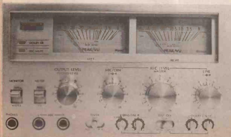
The unfamiliar controls in the bottom right-hand corner operate the built-in test oscillator for those of you who like to squeeze the last drop of perfection out of your system.
