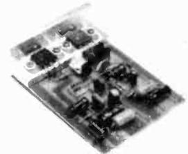
PFA100 120W into 8Ω (V<sub>s</sub> = ± 60V)
