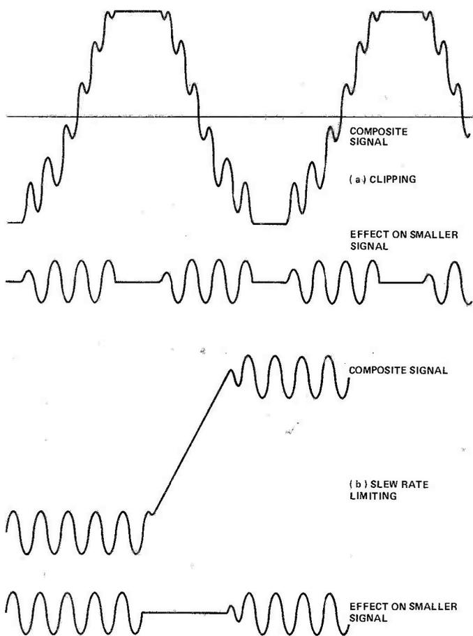
Fig. 5 Intermodulation distortion types due to (a) clipping and (b) slew rate limiting.
