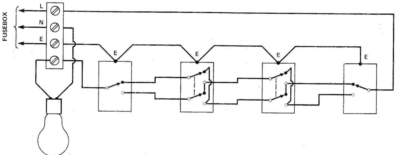
Fig. 1a Ah, in the good old days this was the circuit you'd have to use to switch a light from more than a couple of switches; it was a good circuit — it kept many a plasterer in gainful employment, not to mention the copper mills . . .
