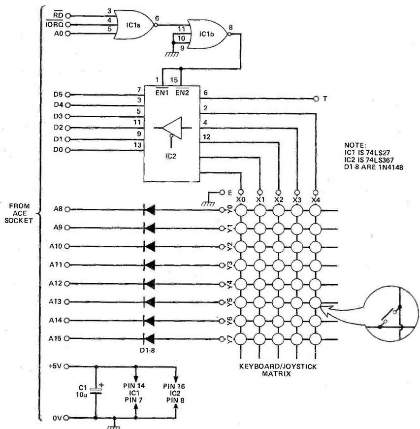
Fig. 1 Circuit diagram of the interface.
