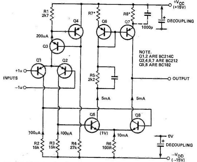
**Fig. 8(b) High gain, low distortion gain block. R7 and R8 (marked with \*) are optional 100R resistors which lessen the need to match the characteristics of Q6 and Q7 — they could be replaced with links.**
