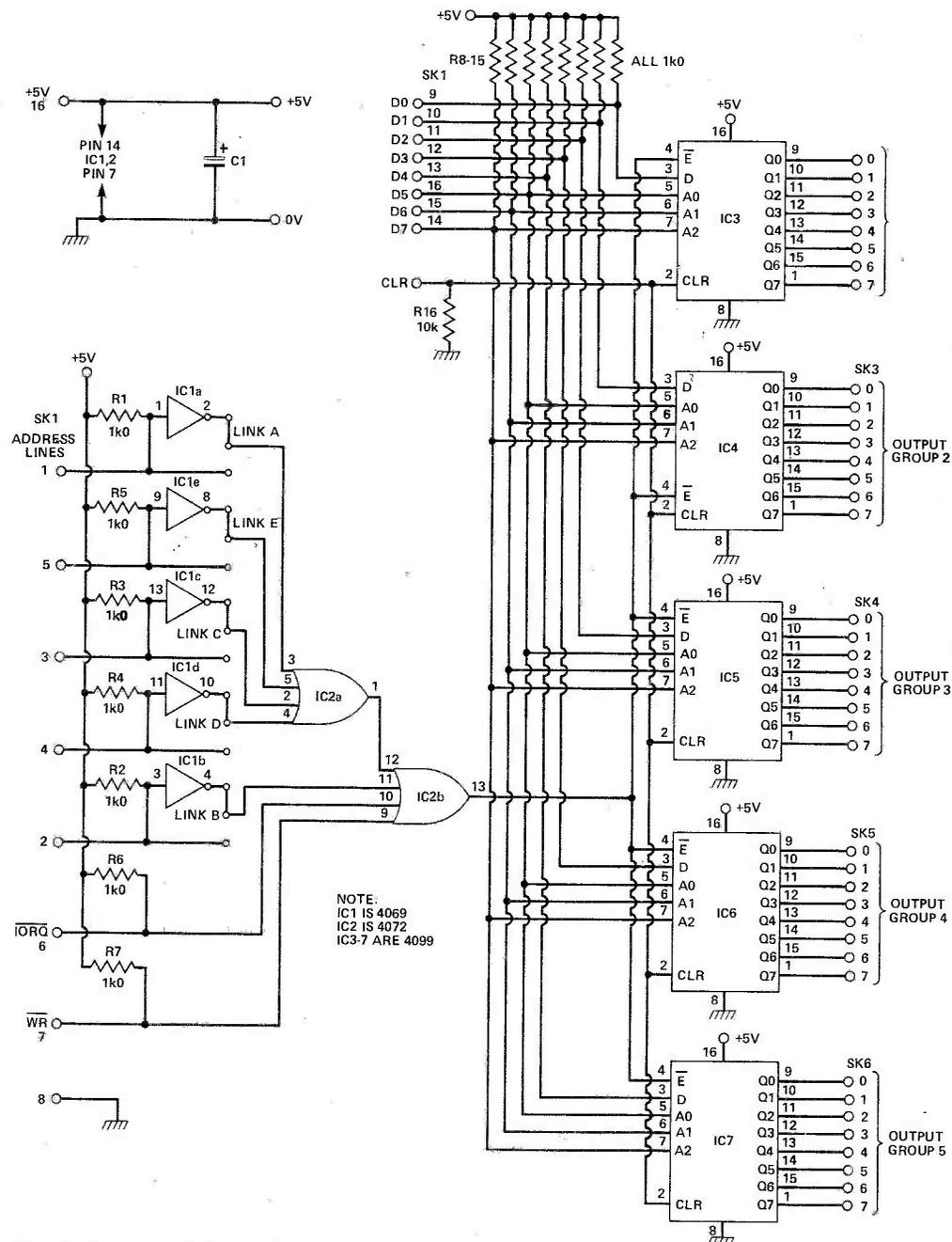
Circuit diagram of the multiple output port.
