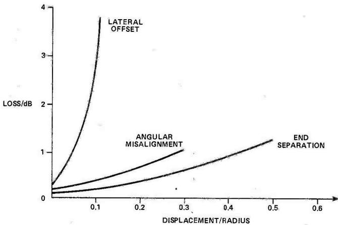
Fig. 9 Characteristics of transmission loss sensors.
