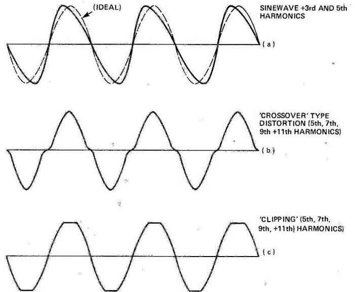
Fig. 4 Waveforms containing odd harmonic distortion.
