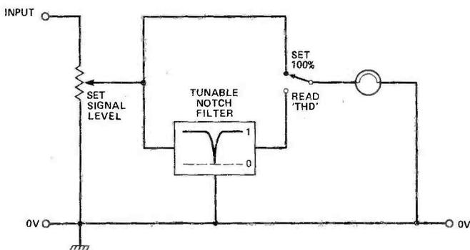
Fig. 1 Total harmonic distortion measuring instrument.
