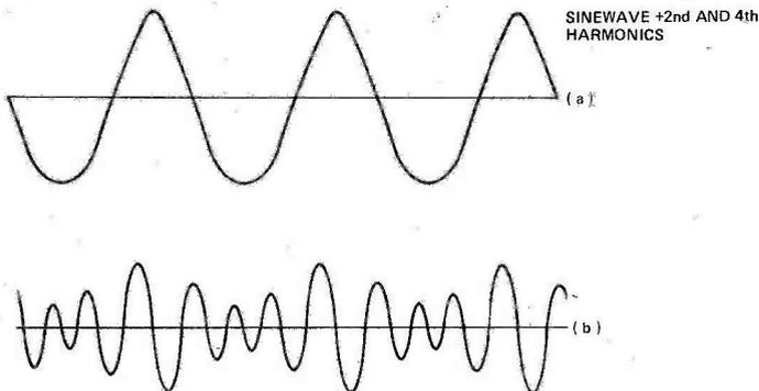
Fig. 3 Harmonic (a) and intermodulation (b) distortion.
