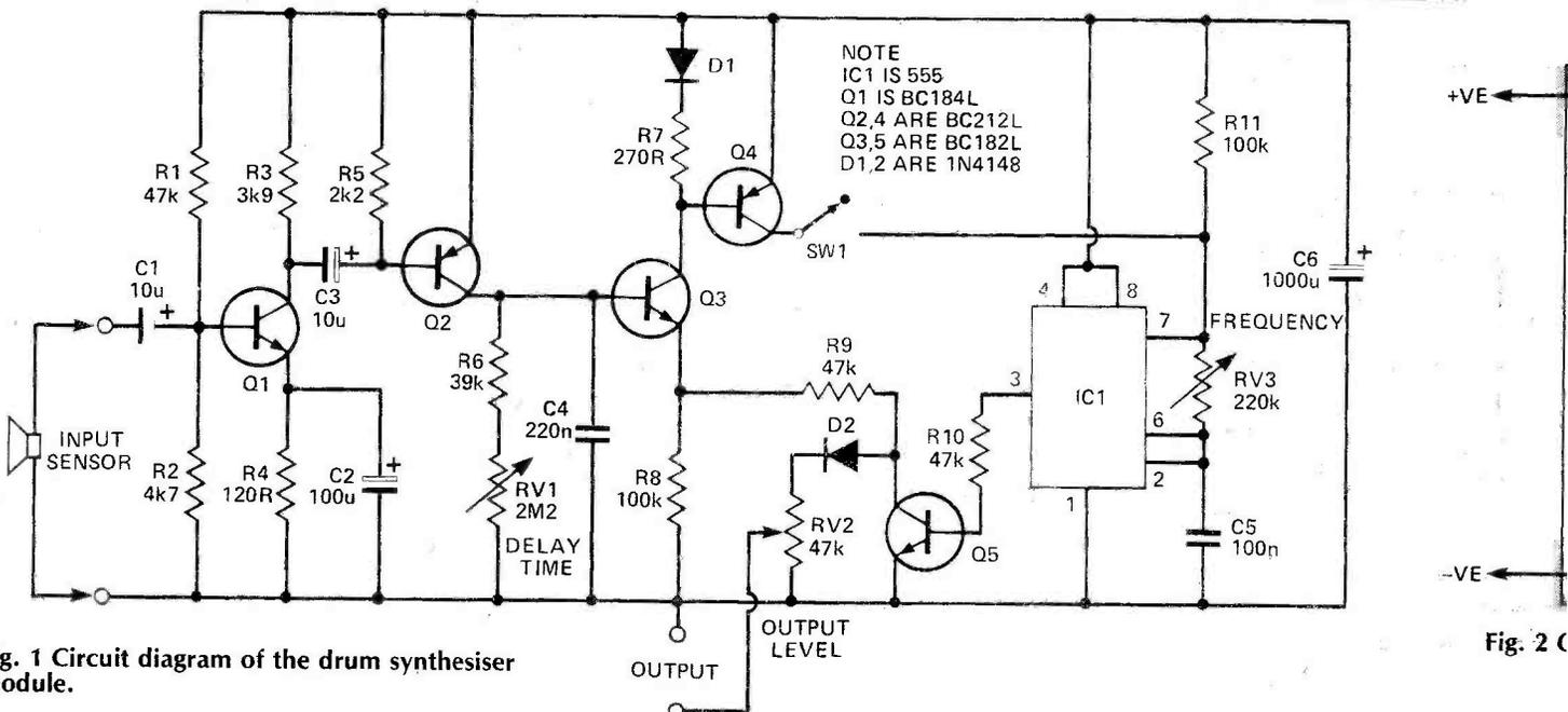
Fig. 1 Circuit diagram of the drum synthesiser module.
