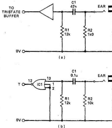
Fig. 7a. Standard Ace tape input port circuit; b. alternative tape port using spare gate on interface.
