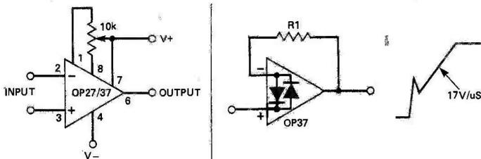
capacitance with a series resistor of 50R or more load capacitances larger than 2000pF can be accommodated. Input offset voltage can be externally trimmed without affecting input offset voltage drift with temperature or time.
