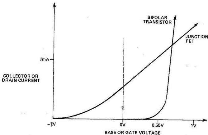
**Fig. 7 Input characteristics of bipolar and field-effect transistors.**
