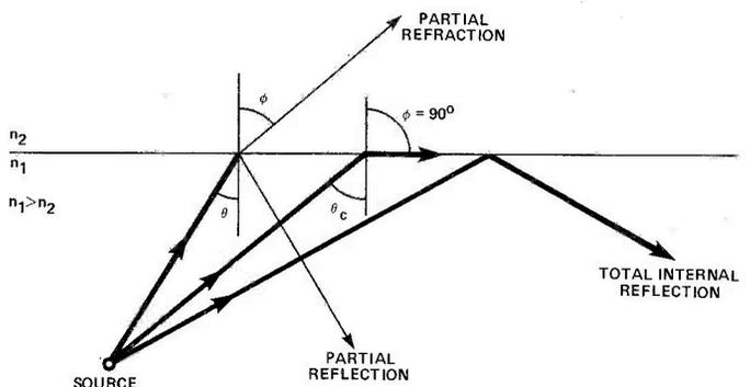
Fig. 2 Illustration of Total Internal Reflection.
