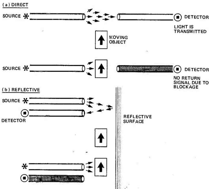
Fig. 4 Position detection using optical fibres.
