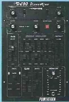
**DJ90 Stereo Mixer** — this is a really versatile new mixer that enables the constructor DJ to produce a professional performance every time. There are two stereo inputs for magnetic cartridges, a stereo auxiliary input and mike input. Other 'plus' features are auto-panning for fast or slow slider controls, multi-mixing, ducking, interrupt, input modulation, in short everything... the whole works — AND — under £100 complete! Complete kit **£97.50 + VAT**
