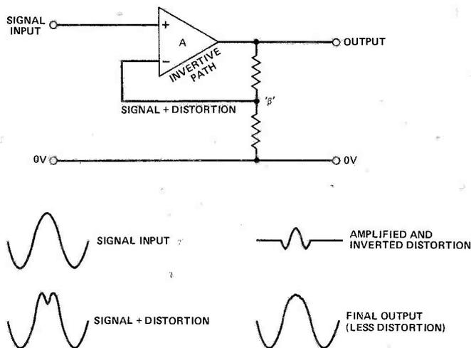
Fig. 6 Negative feedback arrangement and results.
