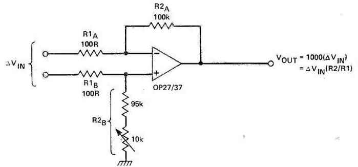
Fig. 4 Single op-amp difference circuit.
