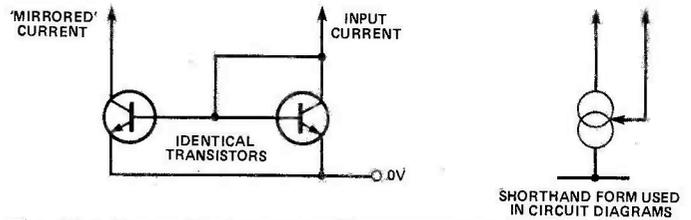
**Fig. 8(a) Current mirror circuit arrangement.**
