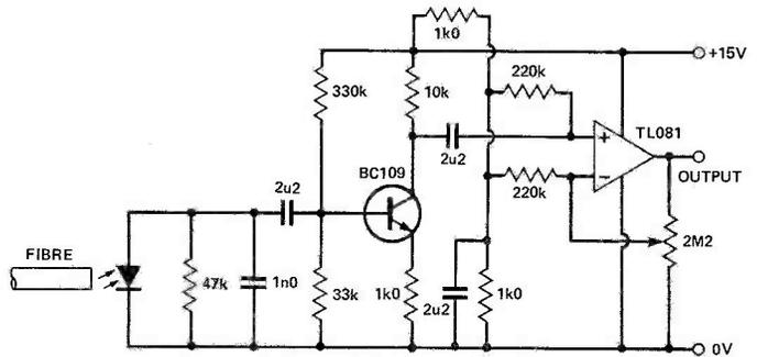
Fig. 16 Audio frequency receiver.
