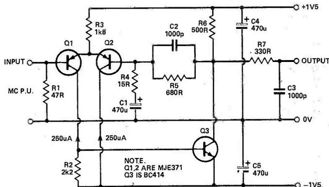
Fig. 12 Moving coil cartridge head amplifier.
