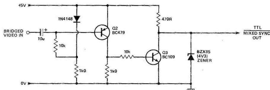
Fig. 3 Circuit to recover the MIXED SYNC pulse from the composite video.
