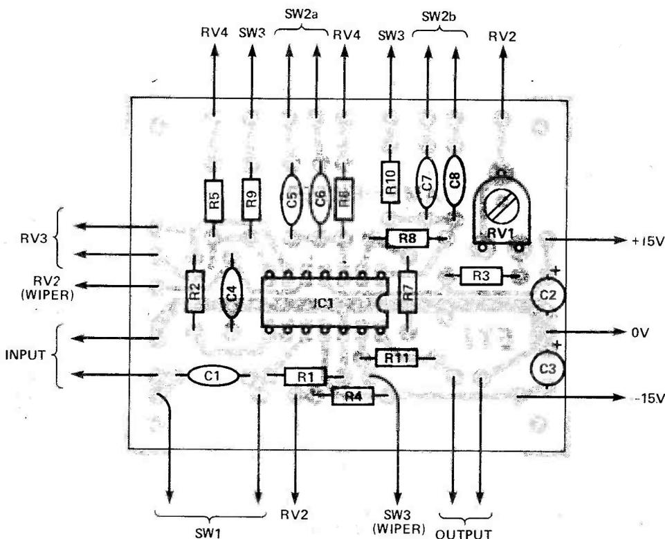
Fig. 1 (left) Component overlay for the PCB
