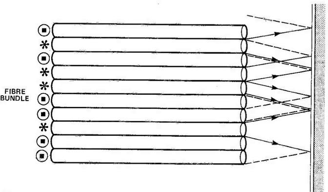
Fig. 7 Principle of the optical level.
