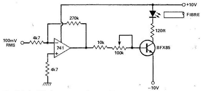
Fig. 14 Audio frequency transmitter.
