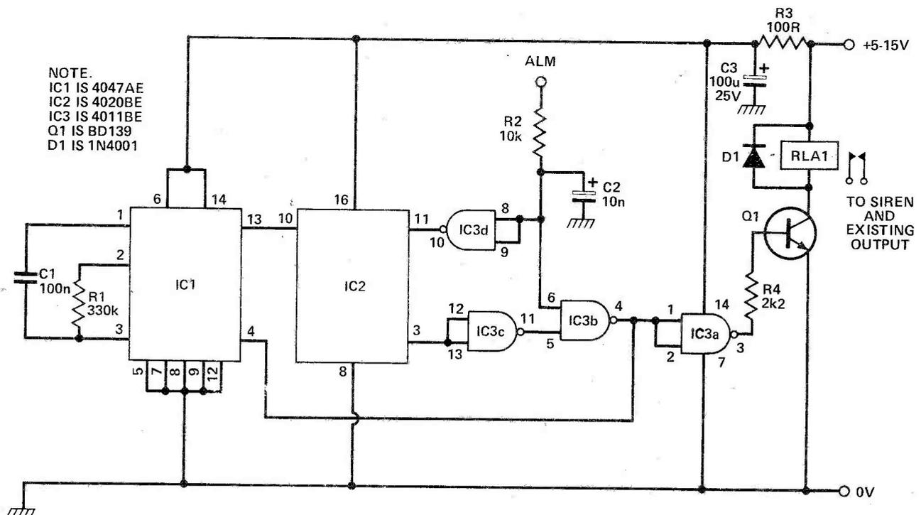
Fig. 1 Circuit diagram of the alarm extender
