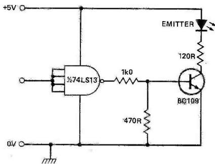
Fig. 11 (above) TTL compatible link.
