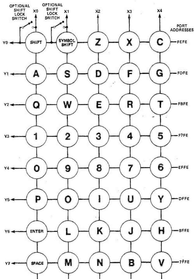
Fig. 3 The coding of the keyboard matrix.
