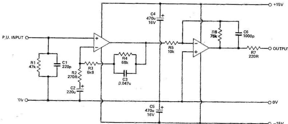
Fig. 10 (left) High quality RIAA equalisation stage, based on the gain block of Fig. 8(b) or a high-quality op-amp.
