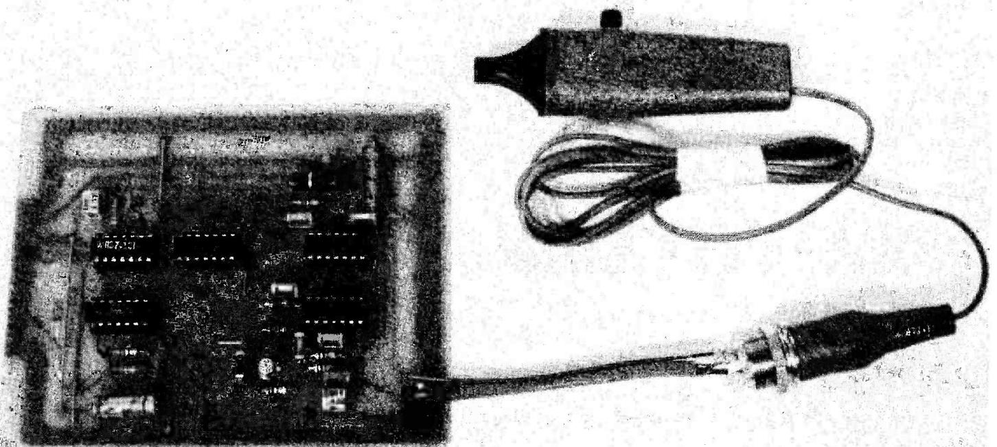
The ETI version of the light pen — unlike the author, we used the body of a highlight pen so that we could fit in the optional switch.
