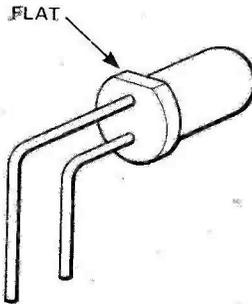
Fig. 4(a) The layout of the indicator LEDs. (b) Mounting details of the two-colour LEDs.
