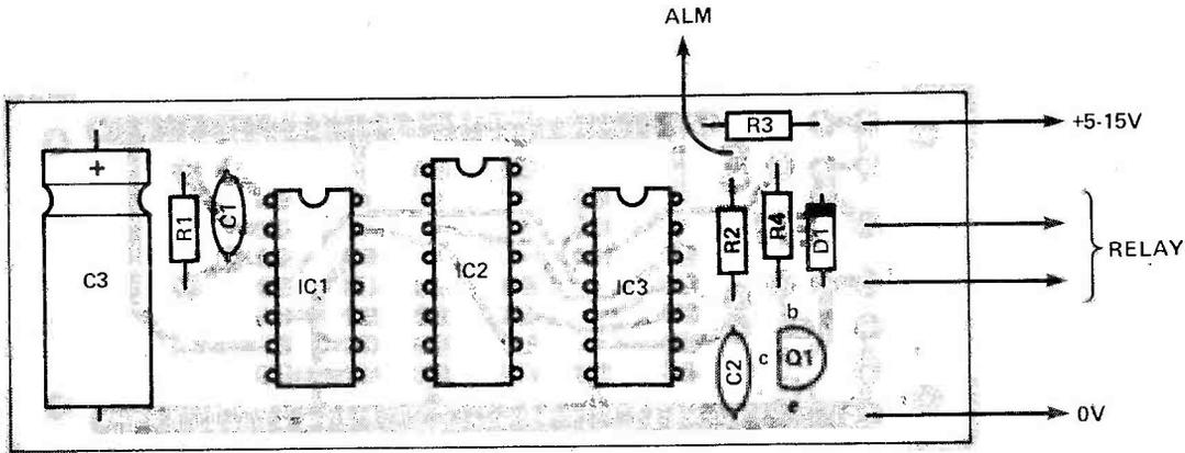
Fig. 2 Component overlay for the PCB
