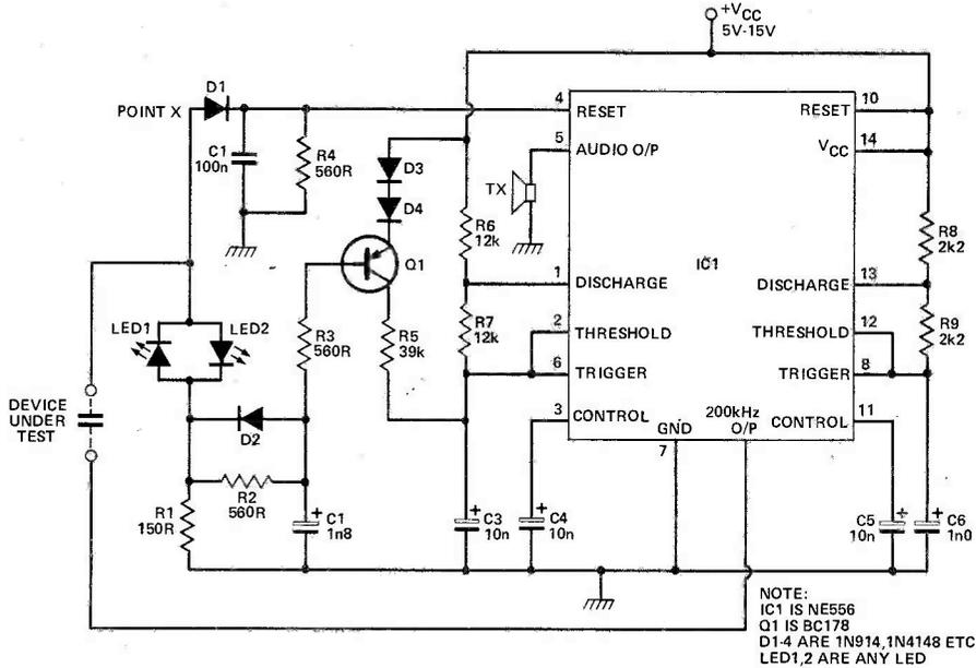
provide a train of positive pulses. These pulses are passed through the device under test to the two LEDs and an audio oscillator formed by the other half of the NE556.
