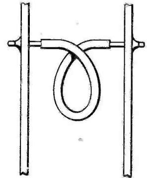
Fig. 5 How we suggest looping the connecting wires between the two boards.
