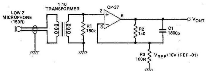
proximately 7000R. Fortunately the noise performance does not degrade appreciably until the source impedance is four or five times this optimum value. The source impedance at the output of this transformer of 15k still provides near optimum noise performance. C1 rolls off the high frequency response at 90 kHz giving a noise power bandwidth of 140 kHz.
