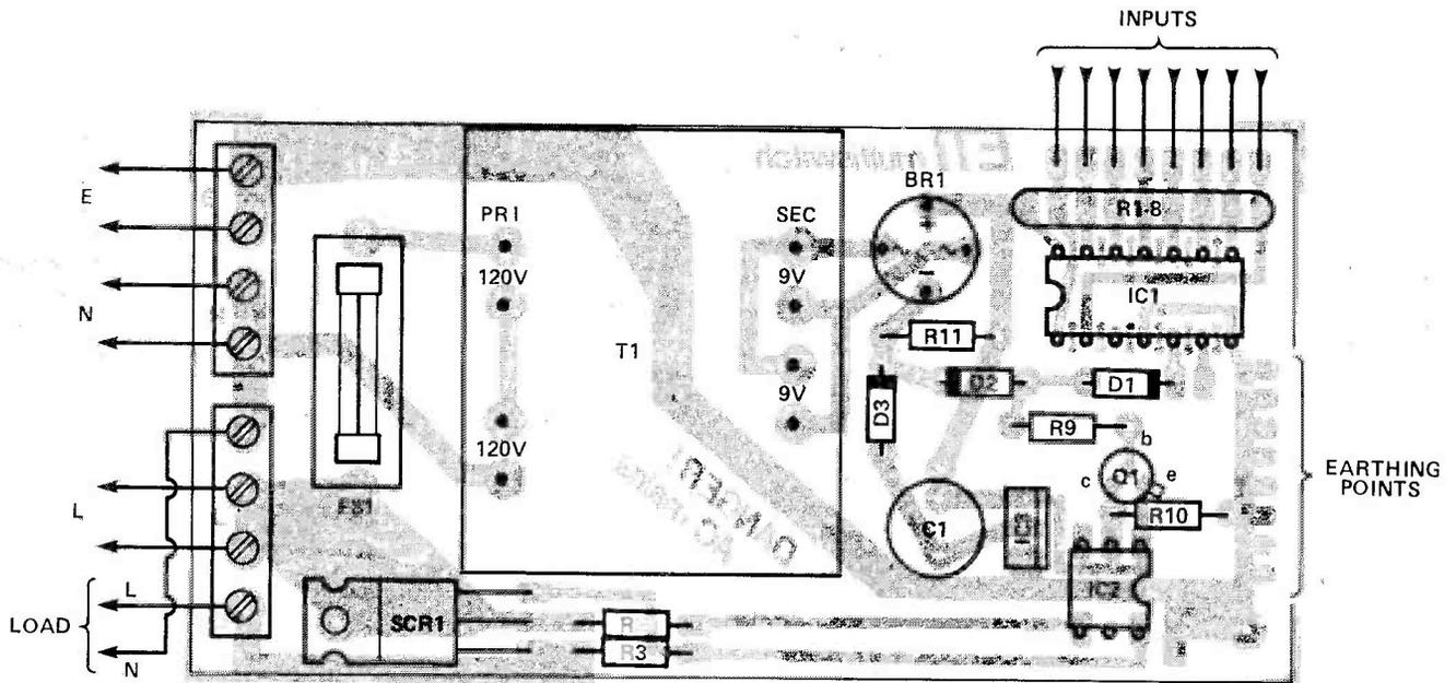
Fig. 3 Overlay diagram of the thingummy. Note that R11 gets a little warm and should be mounted standing slightly proud of the board.
