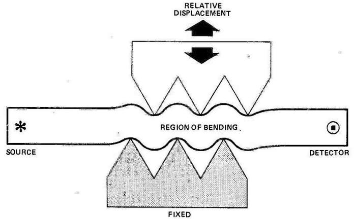
Fig. 10 Fixed/floating microbending transducer.
