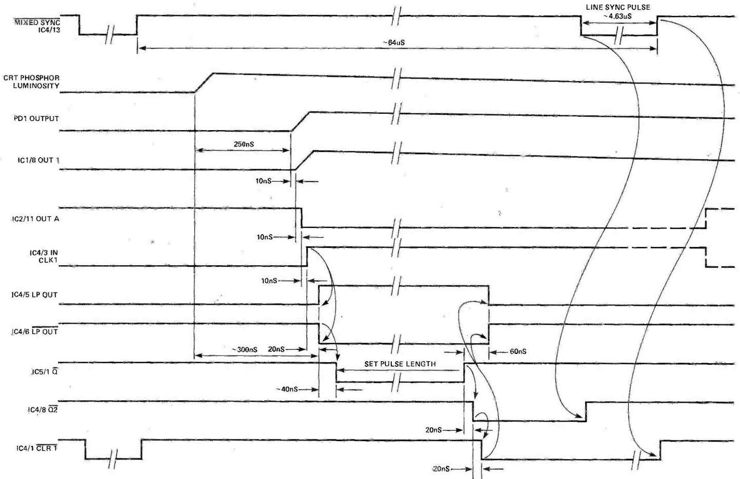
Fig. 2 Timing diagram of the light pen.
