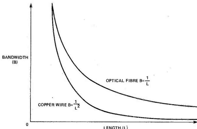
Fig. 1 Comparison of bandwidth over distance for copper wire and optical fibre.
