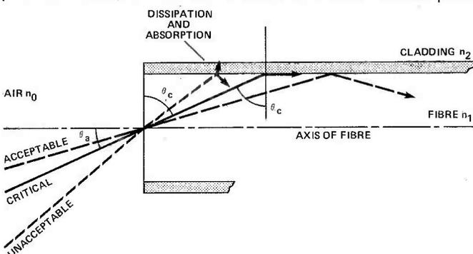
Fig. 3 Acceptable Angle needed to achieve TIR.
