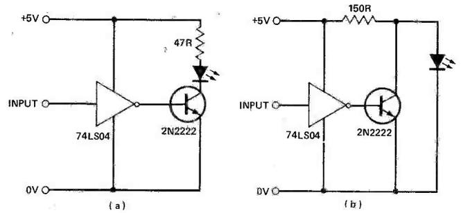
Fig. 15 Series and shunt driven transmitters.
