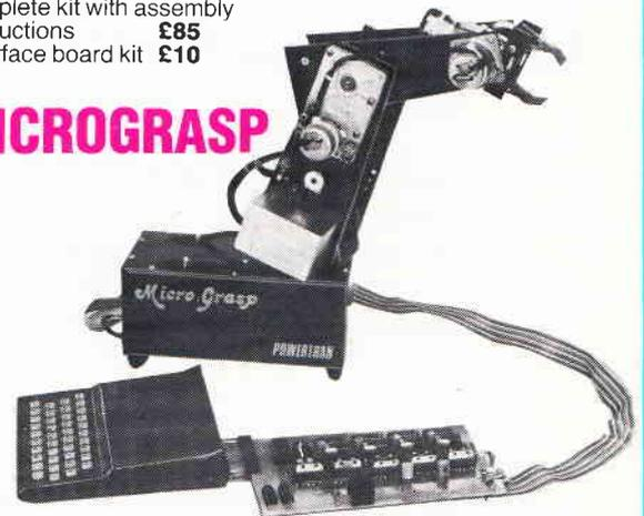
A real, programmable robot for under £200! Micrograsp has an articulated arm jointed at shoulder, elbow and wrist positions. The entire arm rotates about its base and there is a motor driven gripper. All five axes are motor driven and servo controlled, giving positive positioning. The robot can be controlled by any microcomputer with an expansion bus – the Sinclair ZX81 being particularly suitable.
