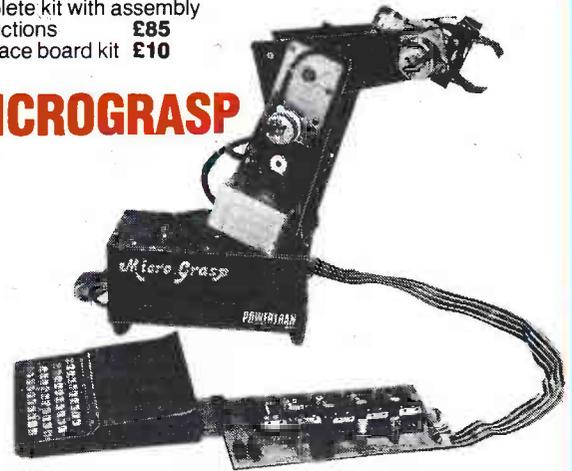
A real, programmable robot for under £200! Micrograsp has an articulated arm jointed at shoulder, elbow and wrist positions. The entire arm rotates about its base and there is a motor driven gripper. All five axes are motor driven and four of these are servo controlled giving positive positioning. The robot can be controlled by any microcomputer with an expansion bus – the Sinclair ZX81 being particularly suitable.
