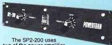
The SP2-200 uses two of the power amplifier sections of the MPA 200 (above), each with its own power supply. A custom designed toroidal transformer enables both channels to simultaneously deliver over 100W rms into 8 ohms. Each channel has its own volume control, and a sensitivity of 0.775mV (OdBm) makes this amplifier suitable for virtually all pre-amps or mixers.
