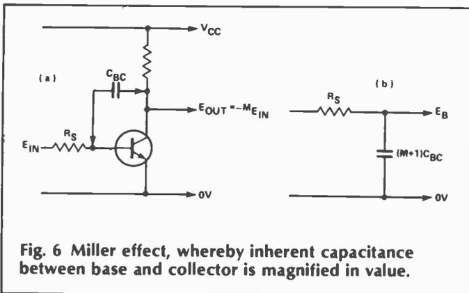
Fig. 6 Miller effect, whereby inherent capacitance between base and collector is magnified in value.
