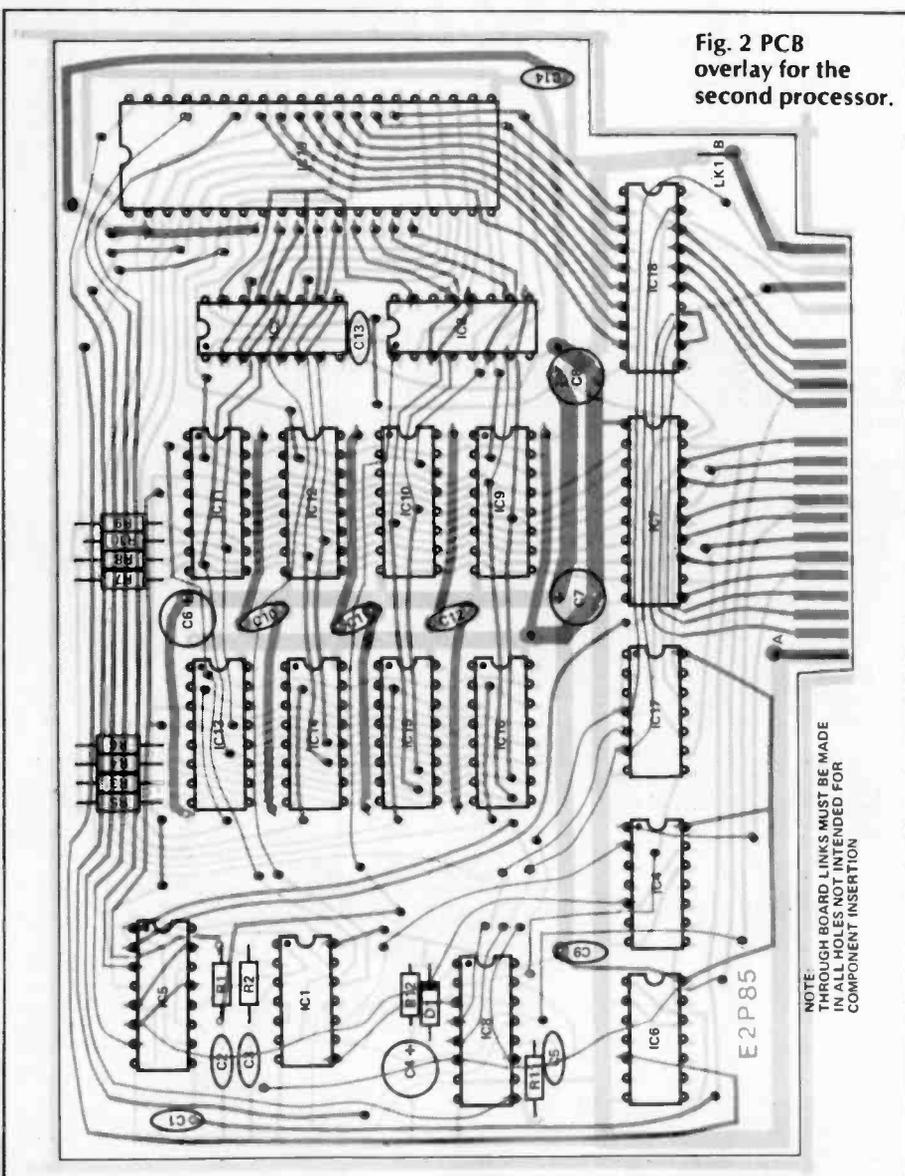
Fig. 2 PCB overlay for the second processor.
