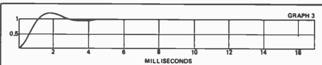
Graph 3 Print-out of active low pass filter simulation.
