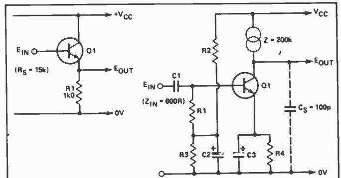
Fig. 3 A transistor arranged as an emitter follower.
