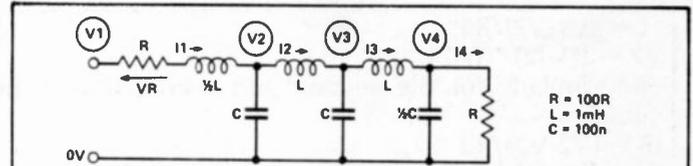
Fig.4 Lumped constant transmission line - equivalent circuit.
