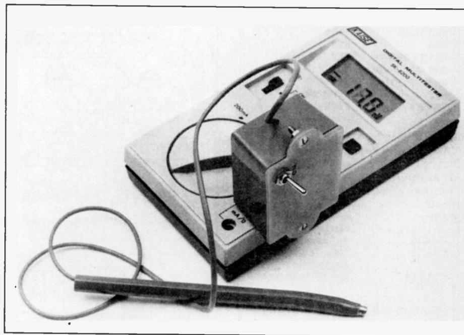
to 10mV per °C. Low power semiconductors are used making the quiescent current drain of the Heat Pen less than 1mA.
