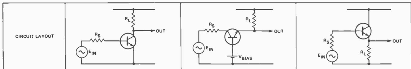
Table 1 Junction transistor performance calculations using h parameters.
