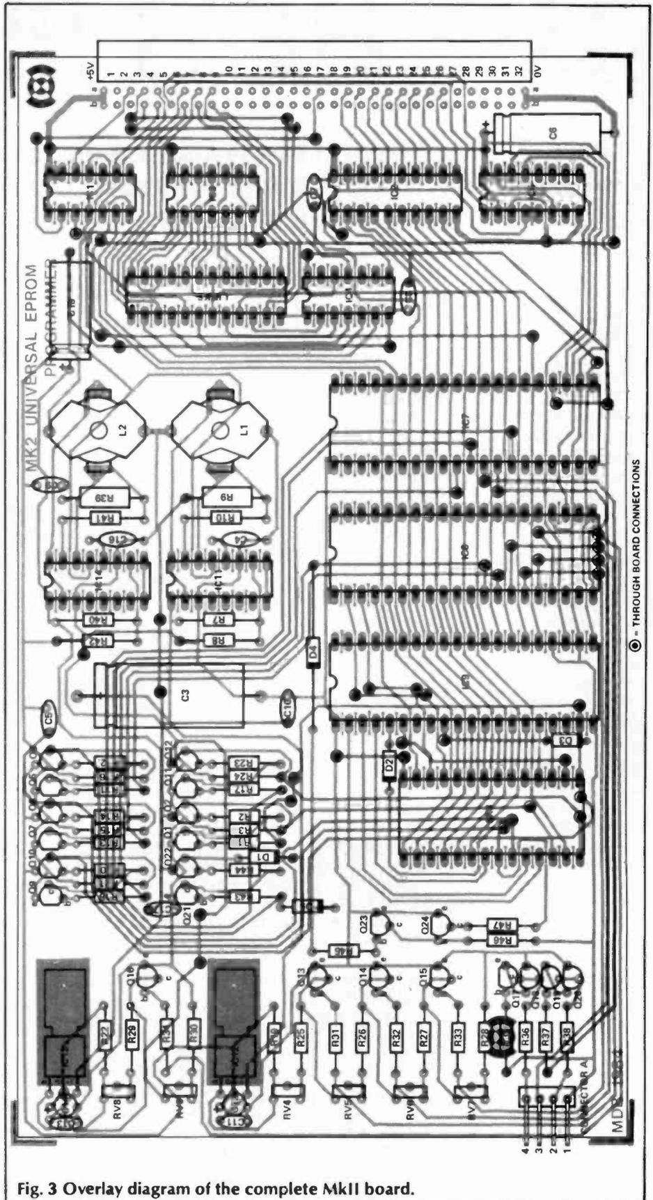
Fig. 3 Overlay diagram of the complete MkII board.
