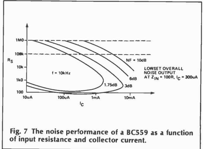
Fig. 7 The noise performance of a BC559 as a function of input resistance and collector current.
