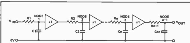
Fig.2 Cascaded time constant circuit.
