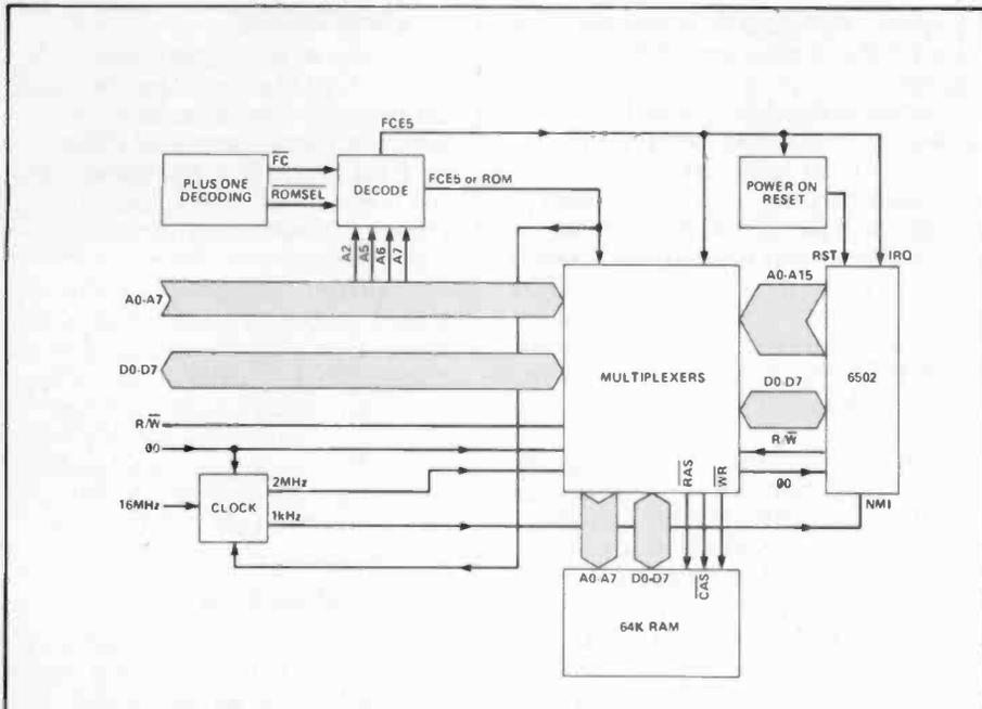
Fig. 1 Block diagram of the second processor board.
