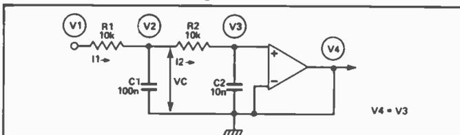
Fig.3 Active low pass filter circuit.
