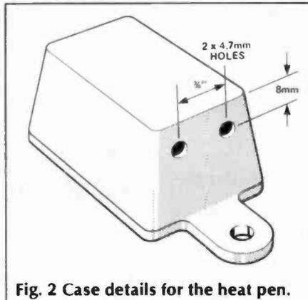
Fig. 2 Case details for the heat pen.
