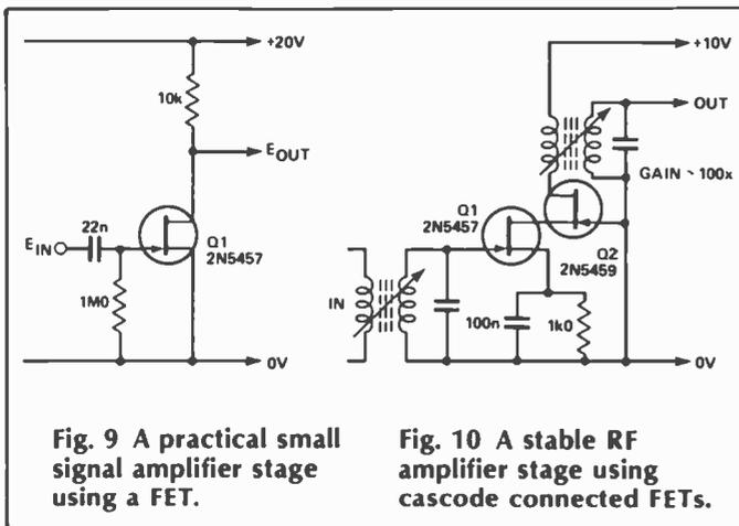
Fig. 9 A practical small signal amplifier stage using a FET.
