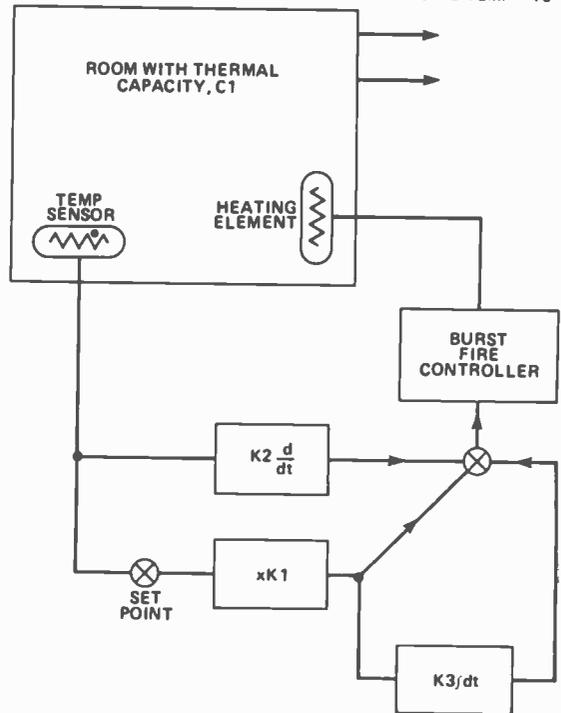
Fig. 6 Block diagram of heater control circuitry.
