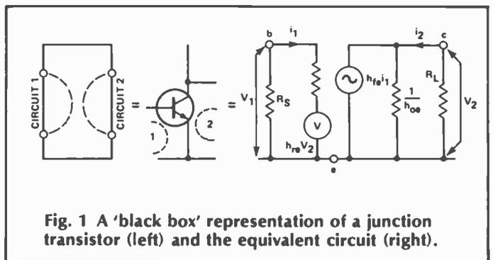
Fig. 1 A 'black box' representation of a junction transistor (left) and the equivalent circuit (right).
