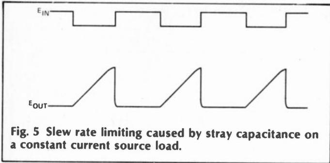
Fig. 5 Slew rate limiting caused by stray capacitance on a constant current source load.
