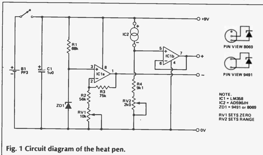
Fig. 1 Circuit diagram of the heat pen.
