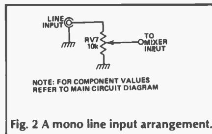
Fig. 2 A mono line input arrangement.
