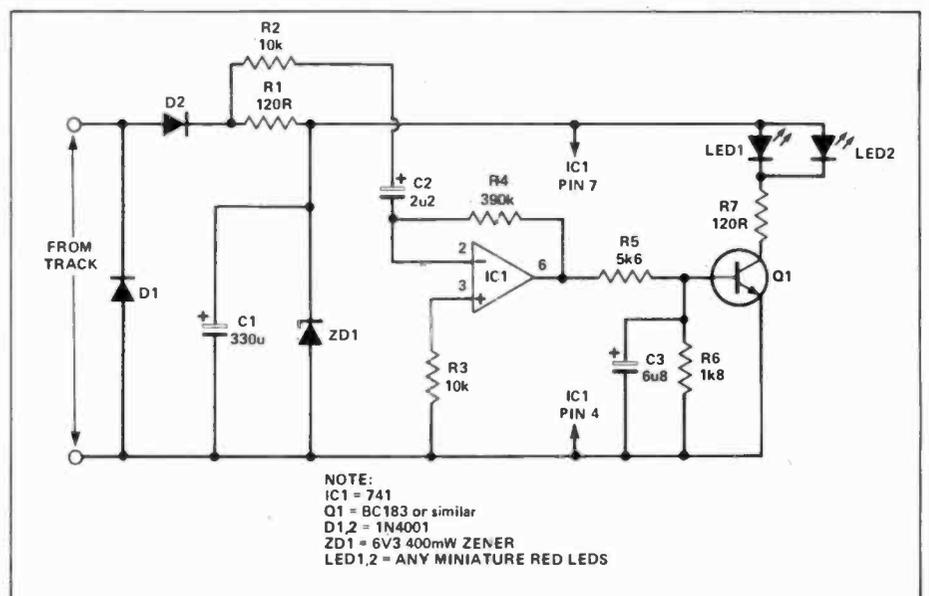
form a potential divider which holds Q1 just off under these conditions and C3 removes most of the AC. When the voltage across the track drops and the car slows down, the output of the IC rises to around 4V increase sound output. and Q1 switches on, lighting the LEDs.
