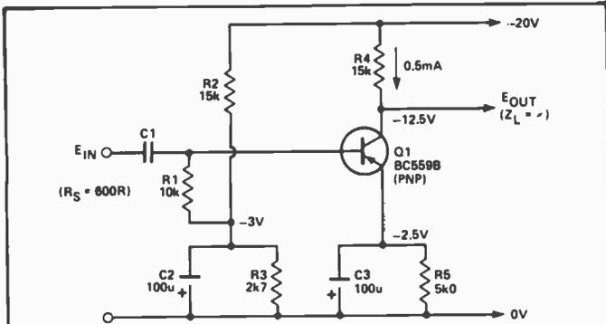
Fig. 2 A practical, common-emitter transistor gain stage which may be used for performance calculations.
