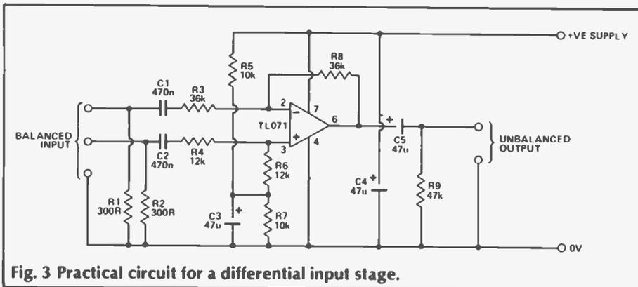
Fig. 3 Practical circuit for a differential input stage.
