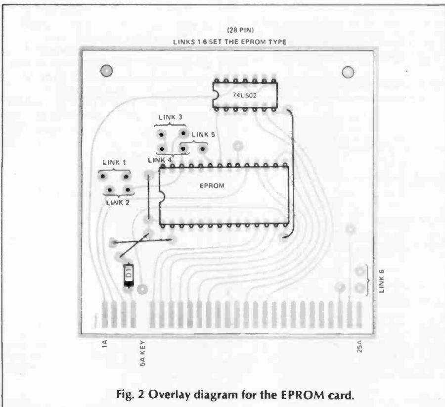
Fig. 2 Overlay diagram for the EPROM card.
