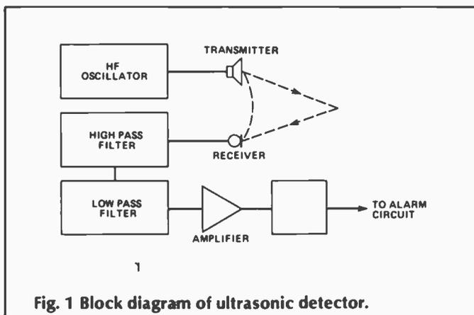
Fig. 1 Block diagram of ultrasonic detector.
