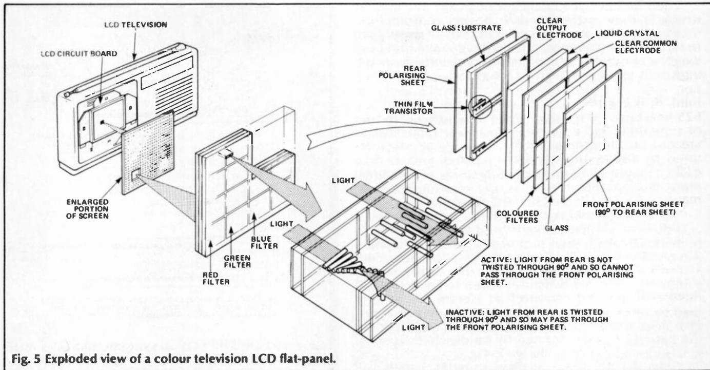
Fig. 5 Exploded view of a colour television LCD flat-panel.
