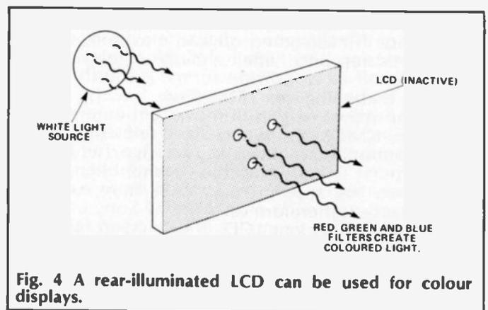
Fig. 4 A rear-illuminated LCD can be used for colour displays.
