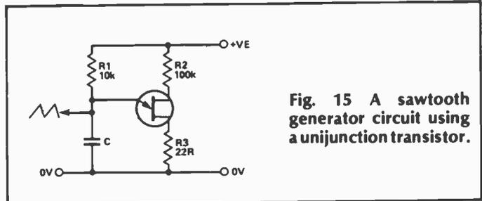
become even more strongly forward biased. The emitter current therefore increases regeneratively until it is limited by the external resistance. This allows the construction of a very simple 'sawtooth' generator, of the form shown in Fig. 15.
