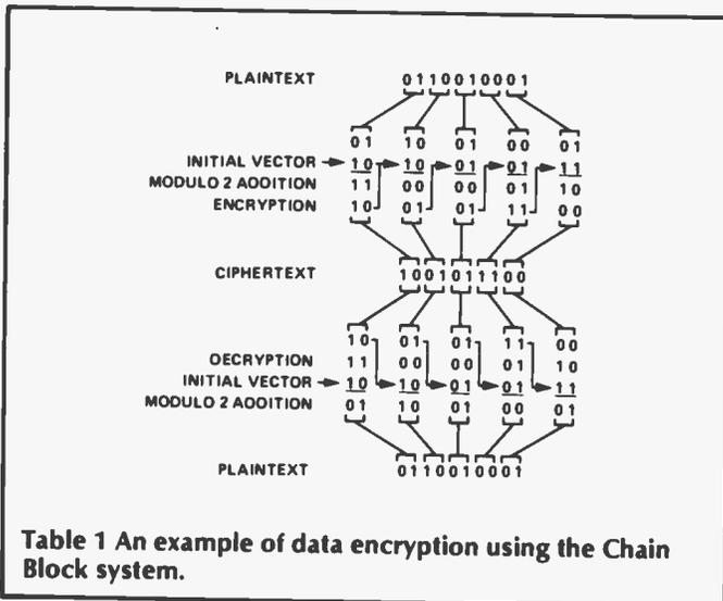
Table 1 An example of data encryption using the Chain Block system.
