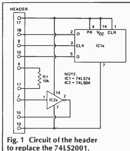
Fig. 1 Circuit of the header to replace the 74LS2001.
