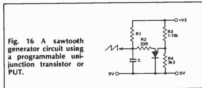
0.55V), when it will suddenly conduct and discharge the capacitor. When the current flow falls below the holding value, the device will turn off and the charge cycle will begin again, as in the normal unijunction transistor circuit shown in Fig. 14.
