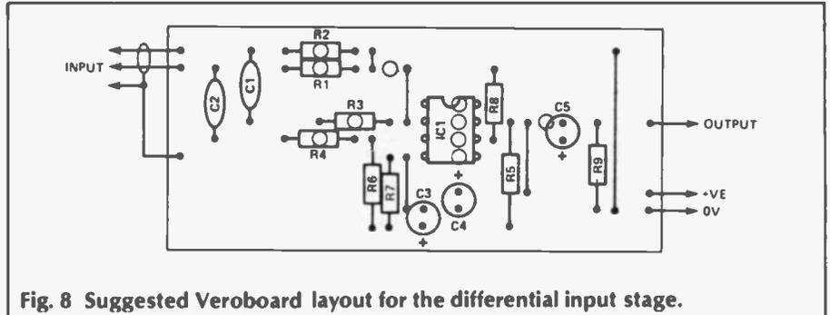
Fig. 8 Suggested Veroboard layout for the differential input stage.
