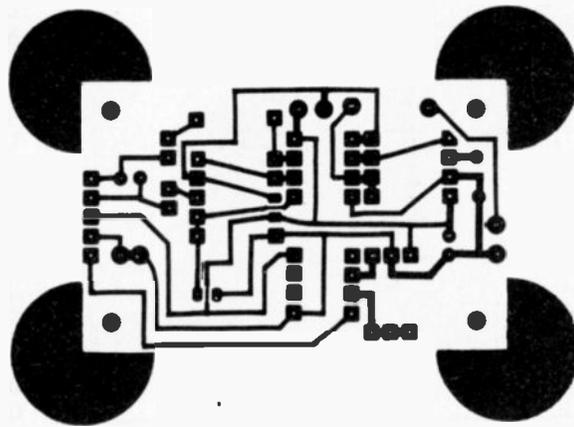
The foil pattern for the direct injection box board.
