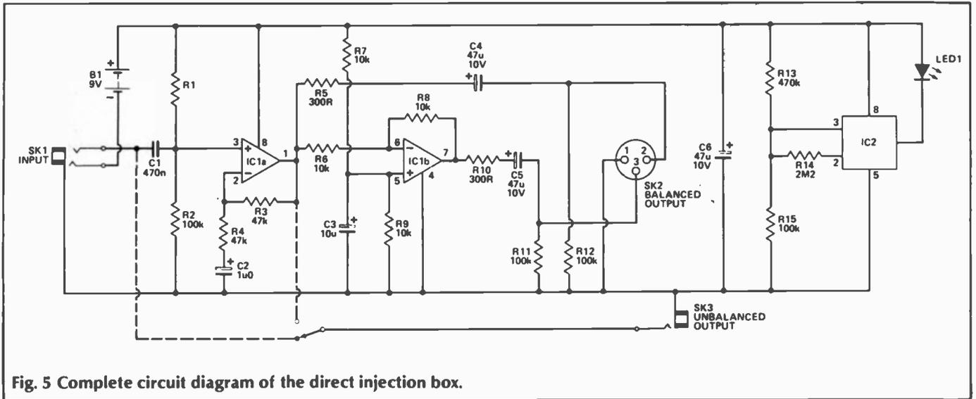
Fig. 5 Complete circuit diagram of the direct injection box.
