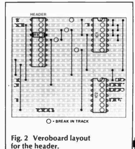
Fig. 2 Veroboard layout for the header.
