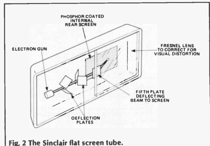
Fig. 2 The Sinclair flat screen tube.
