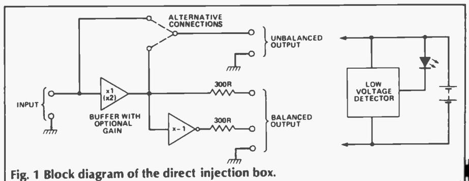
Fig. 1 Block diagram of the direct injection box.
