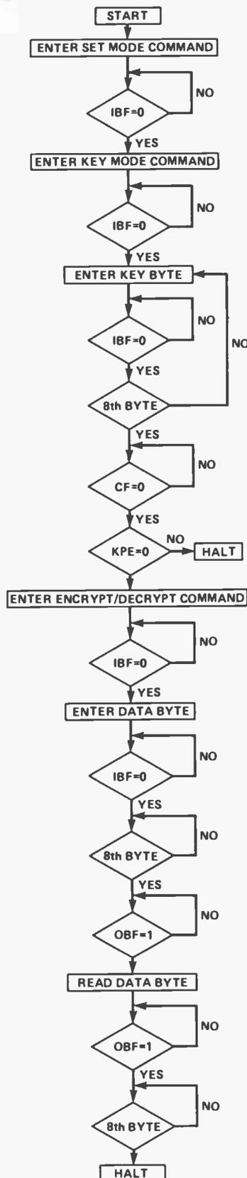
Fig. 2 A data conversion sequence for the circuit shown in Fig. 1.
