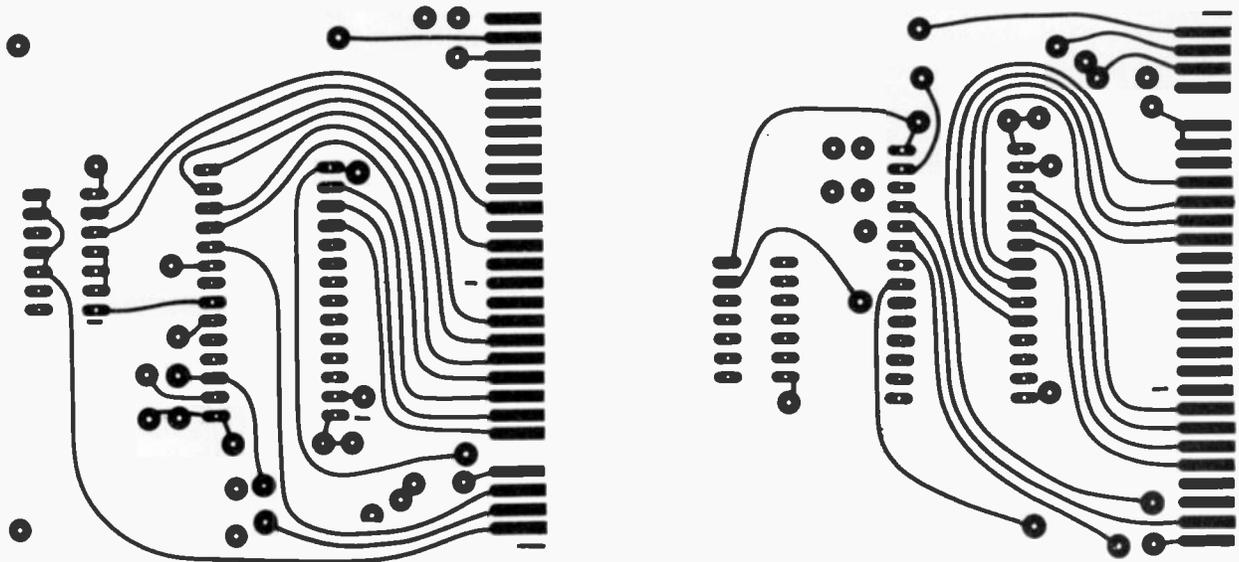
The top and bottom foils for the SpectROM board.
