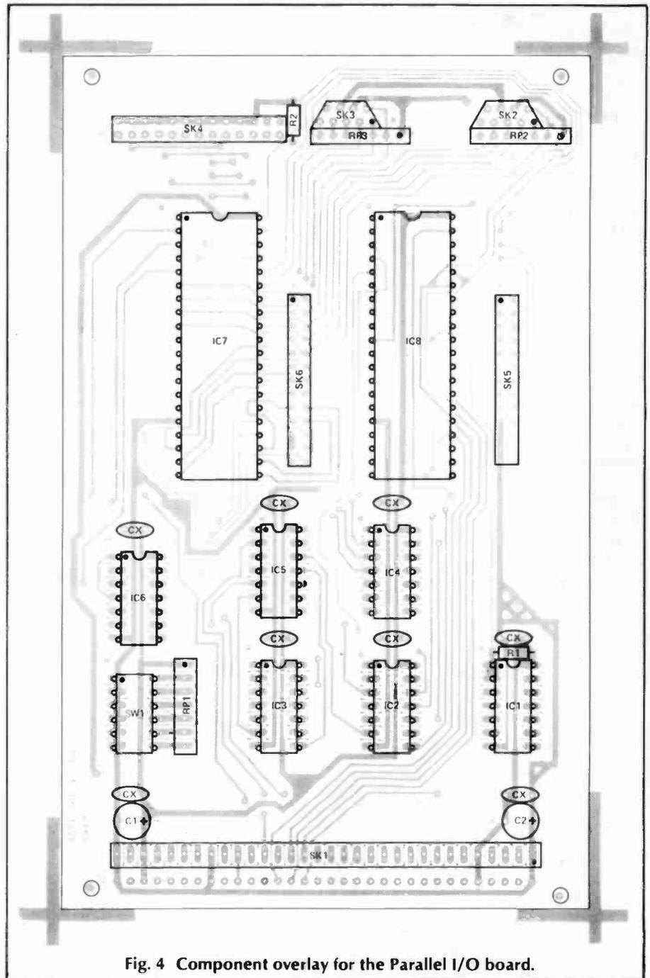
Fig. 4 Component overlay for the Parallel I/O board.
