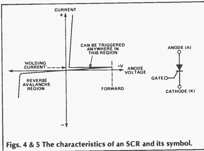
Figs. 4 & 5 The characteristics of an SCR and its symbol.
