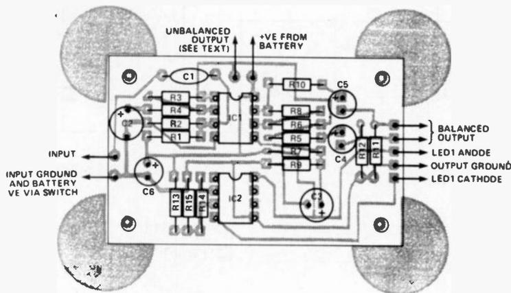
Fig. 6 Component overlay for the DI box PCB.
