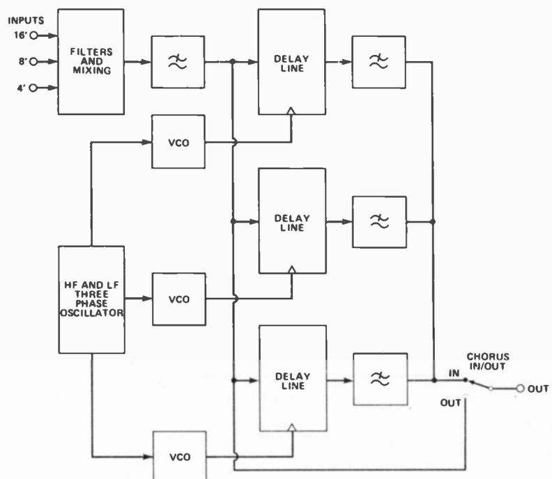
Fig. 6 Block diagram of the chorus section.
