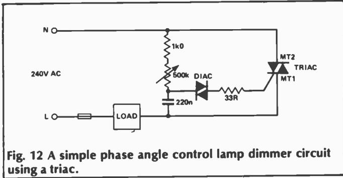
This is a most useful type of circuit, and is much used for living-room lamp dimming and similar applications. It is also used in fade-dissolve circuits in photographic slide projection, though in these applications it is usual to employ more exotic firing circuits to allow prearranged rates of fade or operation from pre-recorded input tone signals.
