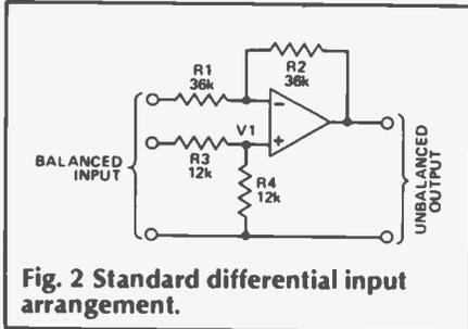
Fig. 2 Standard differential input arrangement.
