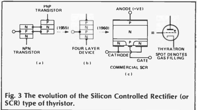
Fig. 3 The evolution of the Silicon Controlled Rectifier (or SCR) type of thyristor.
