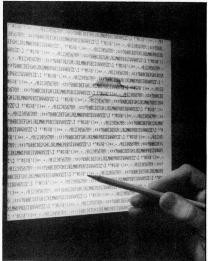
The latest LCD display from STC using smectic A liquid crystals which retain their opacity and therefore do not need thin film transistors.
