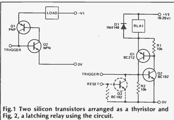
Fig.1 Two silicon transistors arranged as a thyristor and Fig. 2, a latching relay using the circuit.
