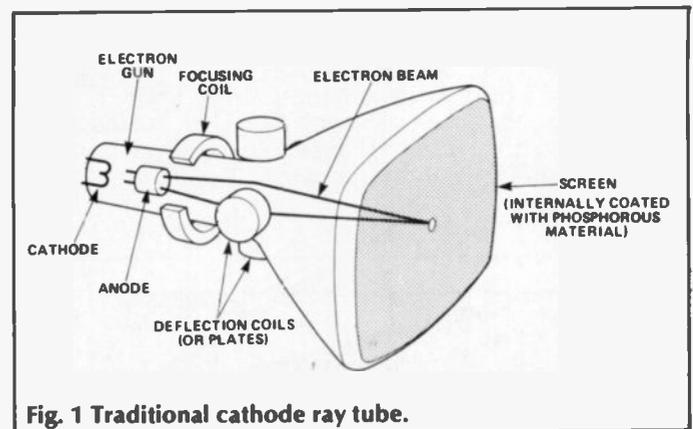
Fig. 1 Traditional cathode ray tube.
