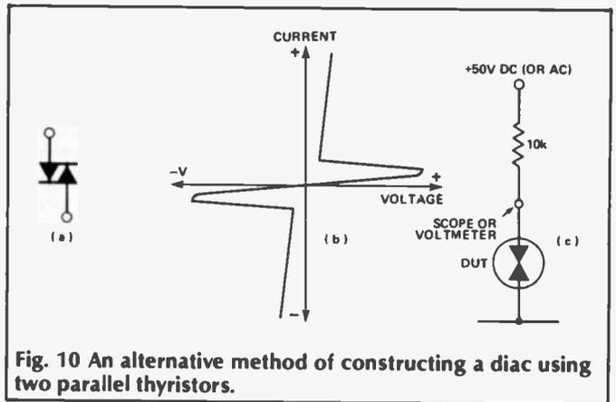
**Fig. 10** An alternative method of constructing a diac using two parallel thyristors.
