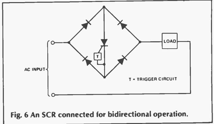
Fig. 6 An SCR connected for bidirectional operation.
