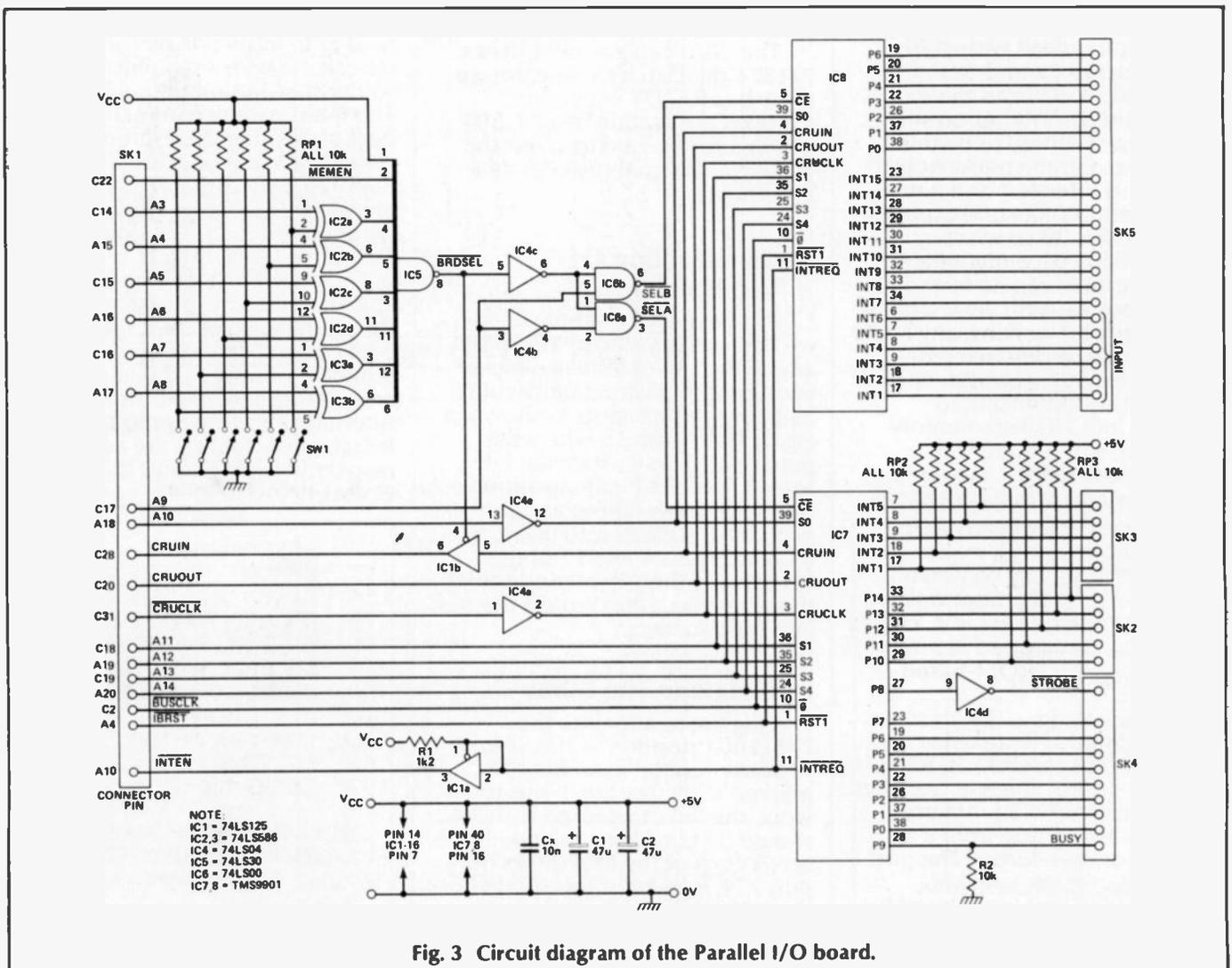
Fig. 3 Circuit diagram of the Parallel I/O board.
