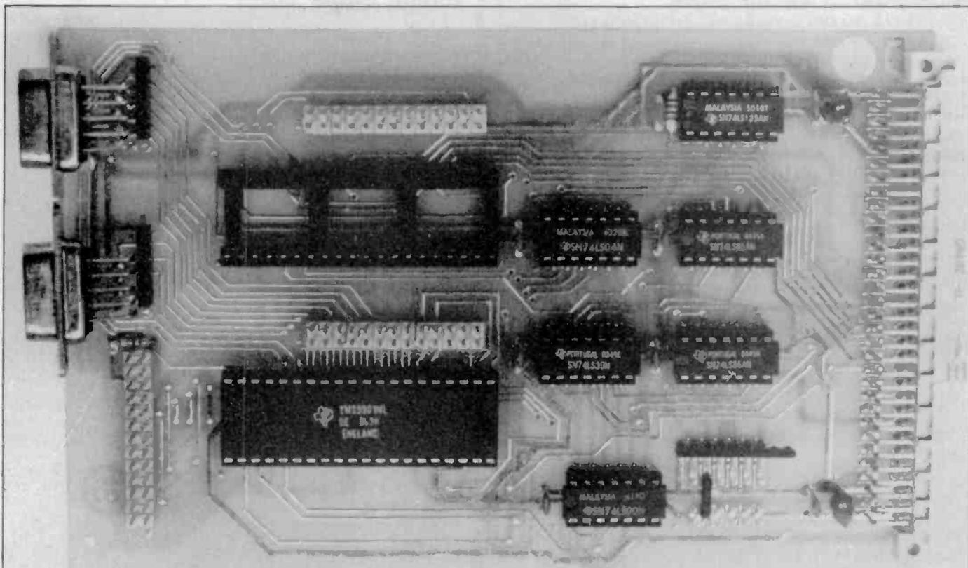
The cortex parallel I/O board configured for Centronics port and two joysticks only.
