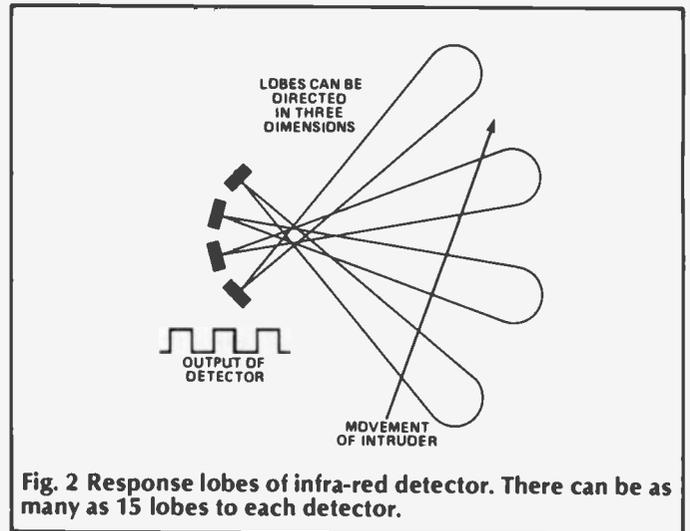
Fig. 2 Response lobes of infra-red detector. There can be as many as 15 lobes to each detector.
