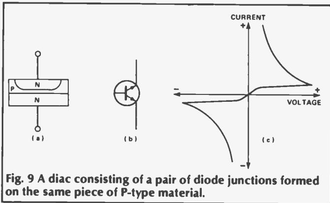
**Fig. 9** A diac consisting of a pair of diode junctions formed on the same piece of P-type material.
