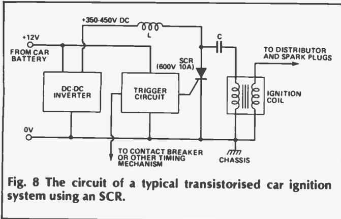
**Fig. 8** The circuit of a typical transistorised car ignition system using an SCR.
