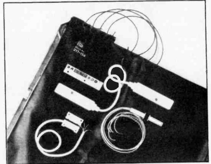
Alarm kit showing (clockwise from bottom right) surface mounting proximity switch (reed plus magnet), flexible tamper-proof jumper lead for bridging doors and windows (in two parts) and flush mounting proximity switch — all sitting on an undercarpet pressure mat.
