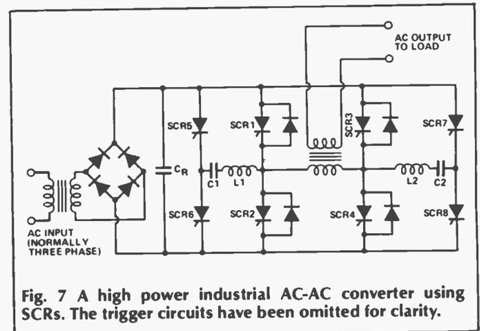
Fig. 7 A high power industrial AC-AC converter using SCRs. The trigger circuits have been omitted for clarity.
