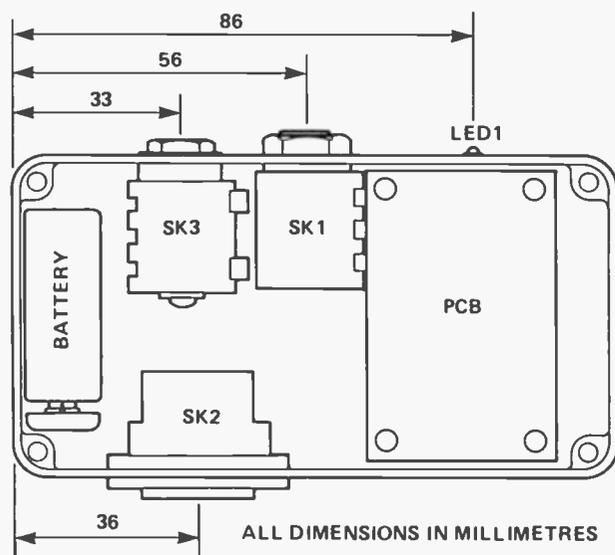
Fig. 7 Layout of the major components within the case.
