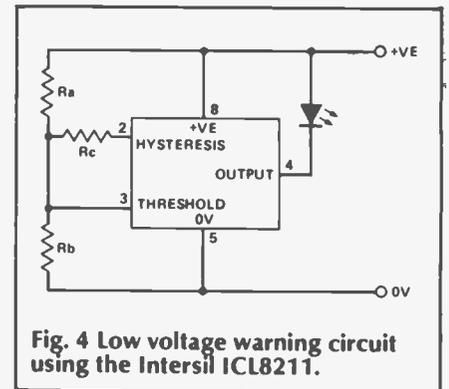
Fig. 4 Low voltage warning circuit using the Intersil ICL8211.
