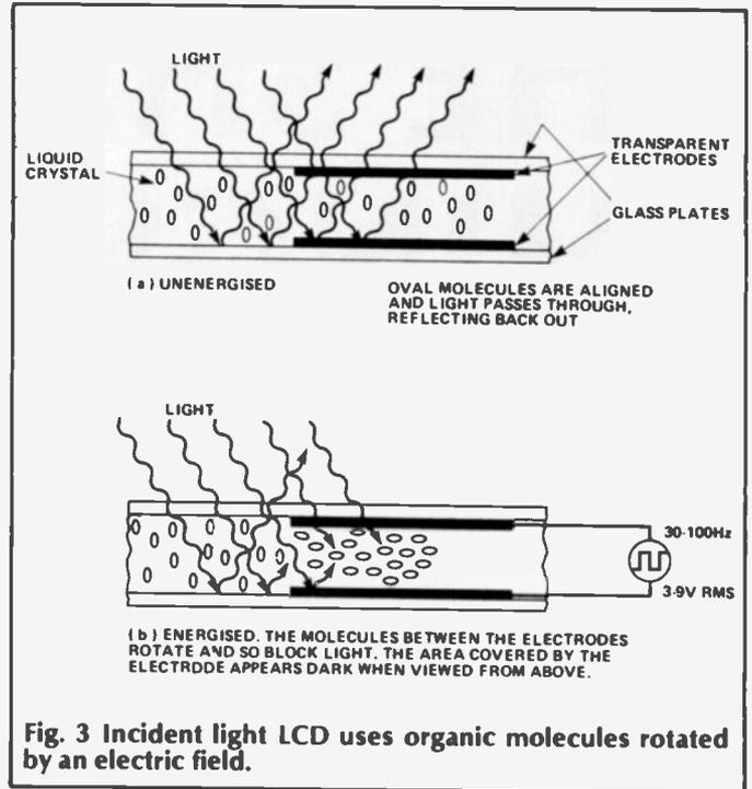
Fig. 3 Incident light LCD uses organic molecules rotated by an electric field.
