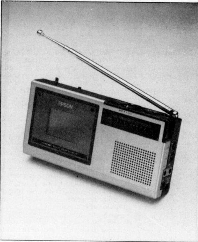
The Epson Elf, the first LCD colour television in the world. The Elf's two inch LCD flat-panel — a completely integrated display.
