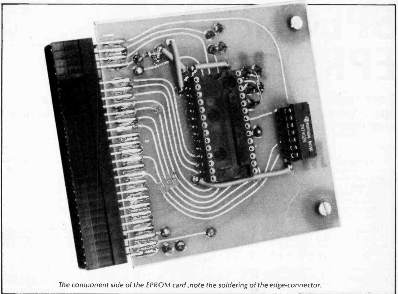
The component side of the EPROM card, note the soldering of the edge-connector.
