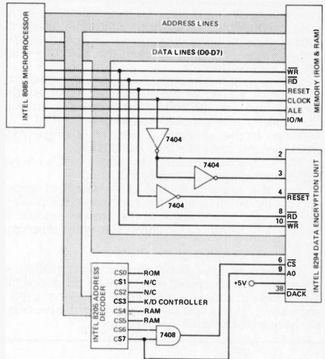
Fig. 1 The 8294 Data Encryption Unit connected to an 8085 microprocessor.
