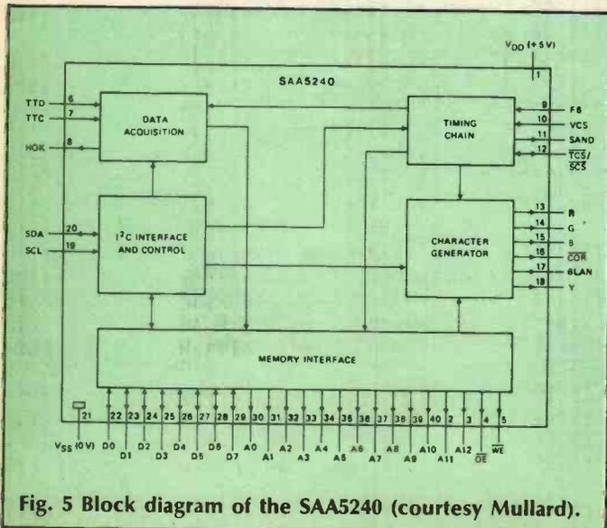
Fig. 5 Block diagram of the SAA5240 (courtesy Mullard).
