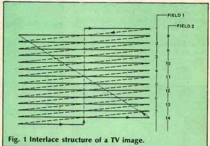
Fig. 1 Interlace structure of a TV image.
