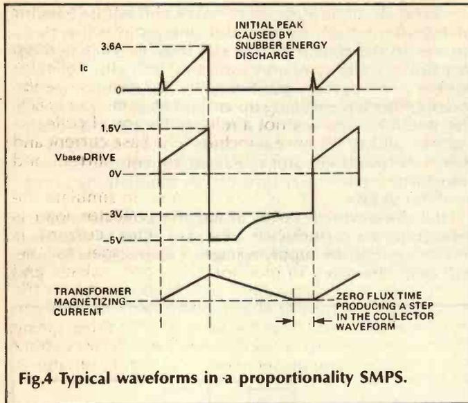
Fig.4 Typical waveforms in a proportionality SMPS.
