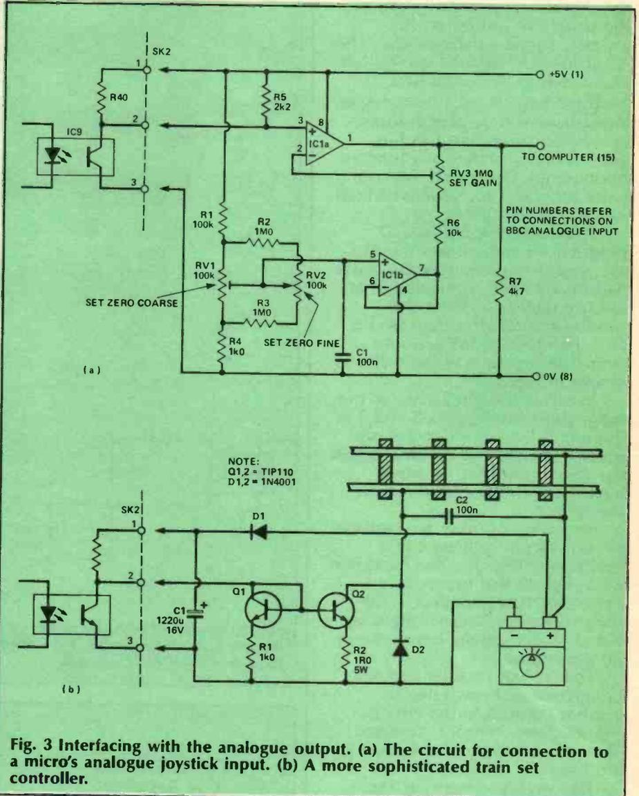
Fig. 3 Interfacing with the analogue output. (a) The circuit for connection to a micro's analogue joystick input. (b) A more sophisticated train set controller.
