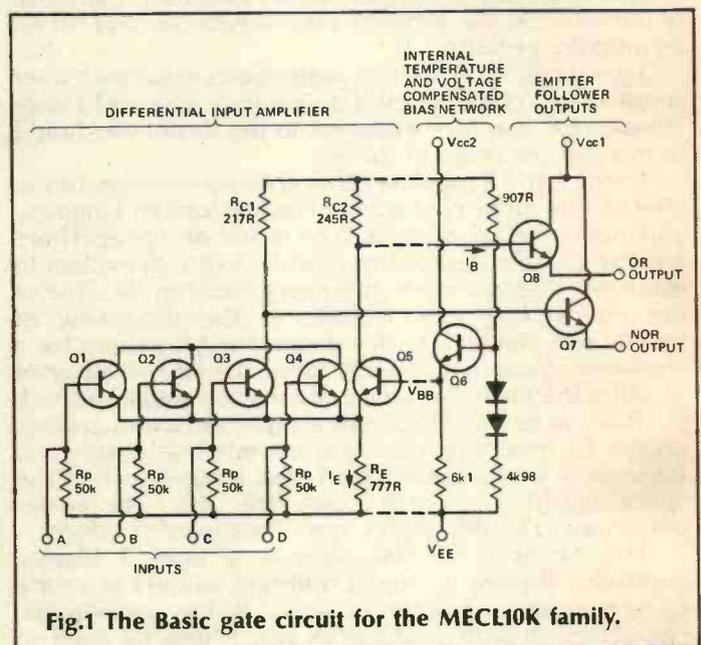
Fig.1 The Basic gate circuit for the MECL10K family.
