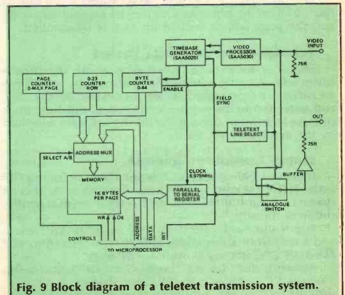
Fig. 9 Block diagram of a teletext transmission system.
