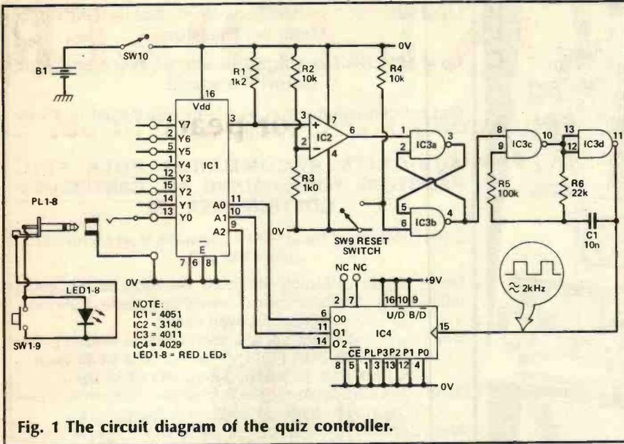
Fig. 1 The circuit diagram of the quiz controller.
