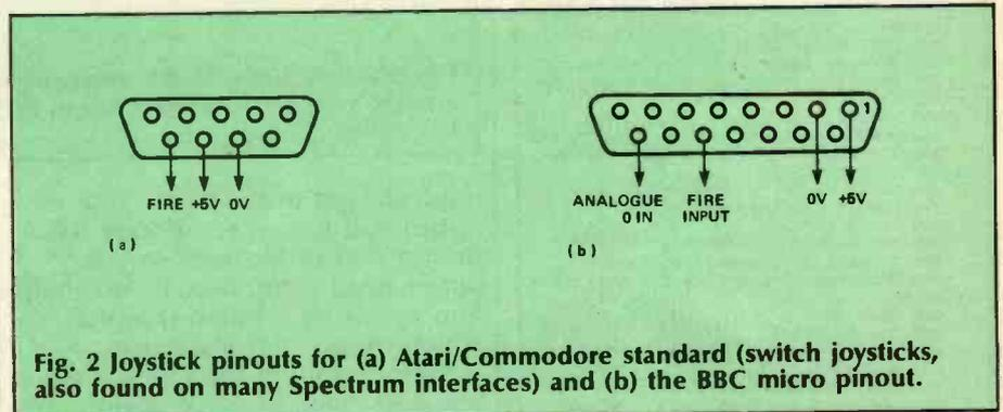
Fig. 2 Joystick pinouts for (a) Atari/Commodore standard (switch joysticks, also found on many Spectrum interfaces) and (b) the BBC micro pinout.
