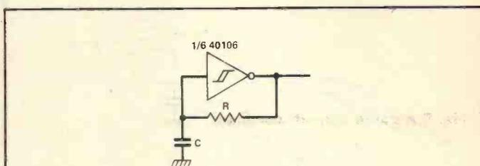
Fig. 1 The Basic Schmitt oscillator.
