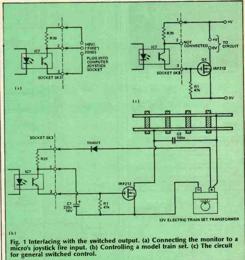
Fig. 1 Interfacing with the switched output. (a) Connecting the monitor to a micro's joystick fire input. (b) Controlling a model train set. (c) The circuit for general switched control.
