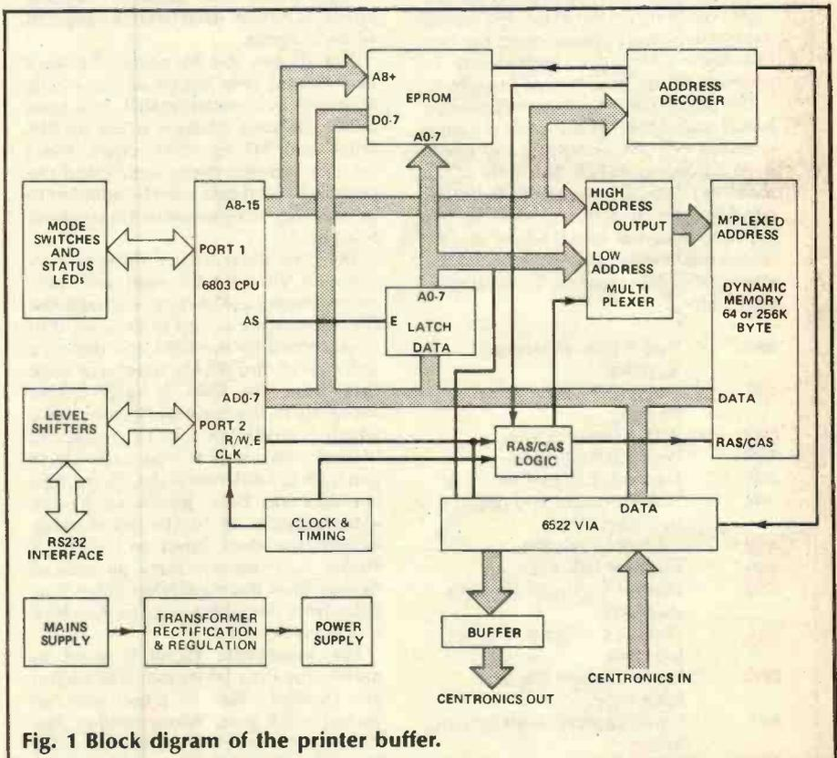
Fig. 1 Block diagram of the printer buffer.
