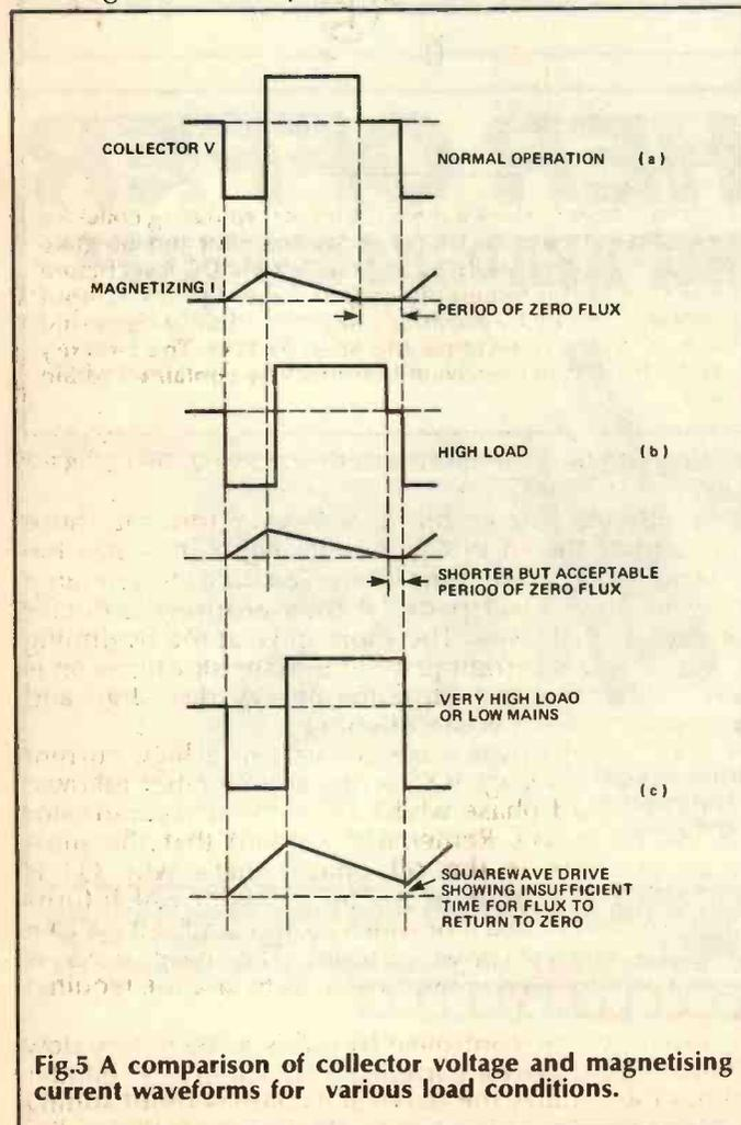
Fig.5 A comparison of collector voltage and magnetising current waveforms for various load conditions.
