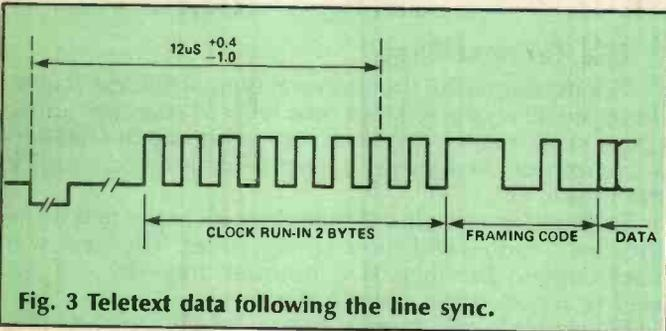
Fig. 3 Teletext data following the line sync.
