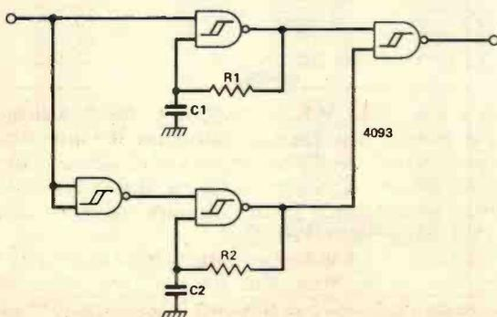
Fig. 8 A digitally selected two frequency oscillator.
