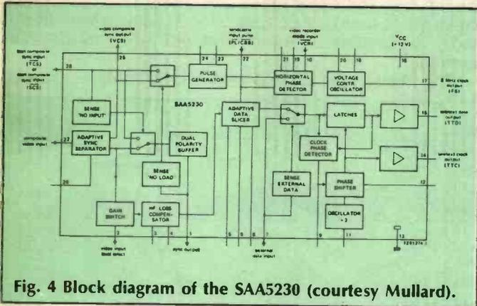
Fig. 4 Block diagram of the SAA5230 (courtesy Mullard).
