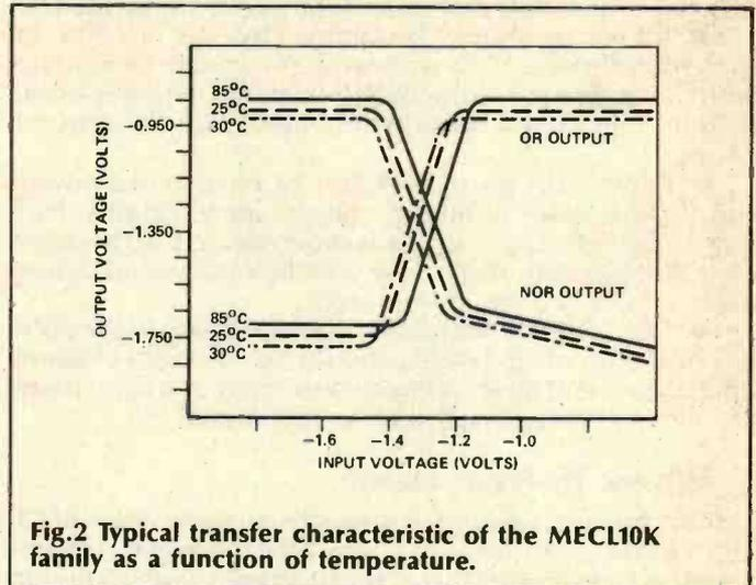
Fig.2 Typical transfer characteristic of the MECL10K family as a function of temperature.
