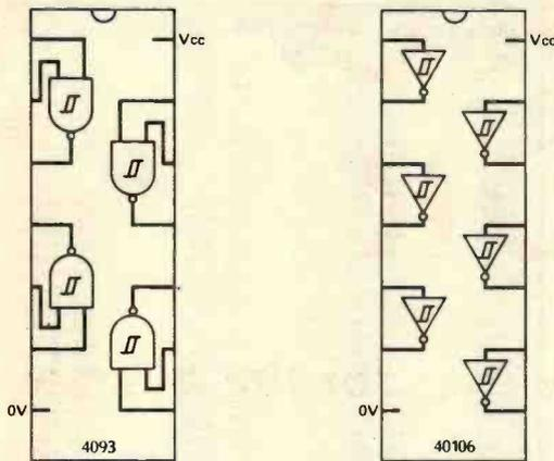
Fig. 4 Pinouts of the Schmitt trigger chips used.
