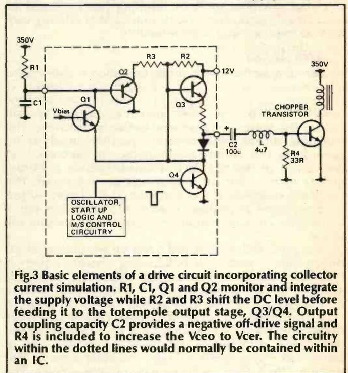
**Fig.3 Basic elements of a drive circuit incorporating collector current simulation. R1, C1, Q1 and Q2 monitor and integrate the supply voltage while R2 and R3 shift the DC level before feeding it to the totempole output stage, Q3/Q4. Output coupling capacity C2 provides a negative off-drive signal and R4 is included to increase the  $V_{ce0}$  to  $V_{ce}$ . The circuitry within the dotted lines would normally be contained within an IC.**
