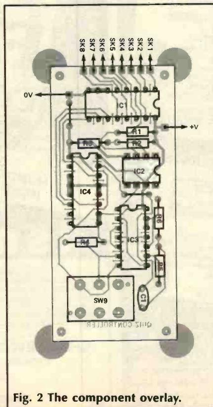
Fig. 2 The component overlay.
