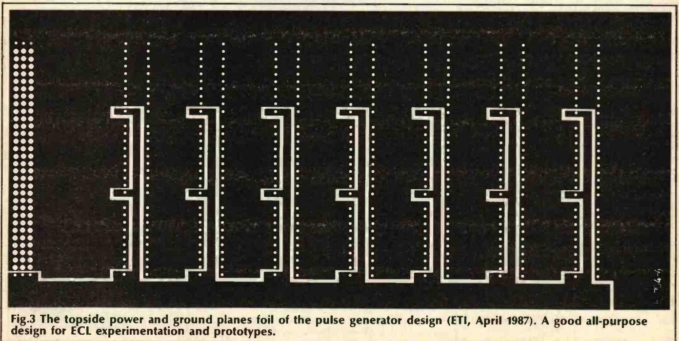
Fig.3 The topside power and ground planes foil of the pulse generator design (ETI, April 1987). A good all-purpose design for ECL experimentation and prototypes.
