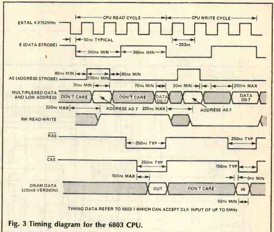
Fig. 3 Timing diagram for the 6803 CPU.
