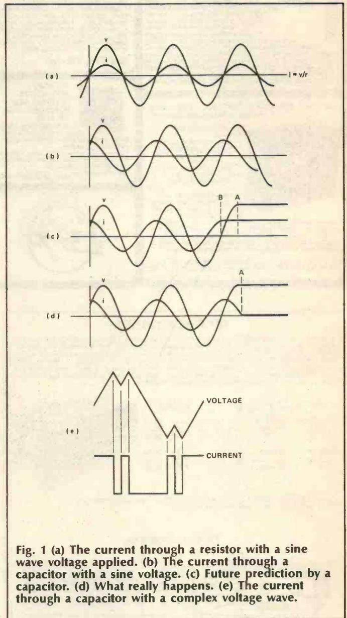
Fig. 1 (a) The current through a resistor with a sine wave voltage applied. (b) The current through a capacitor with a sine voltage. (c) Future prediction by a capacitor. (d) What really happens. (e) The current through a capacitor with a complex voltage wave.
