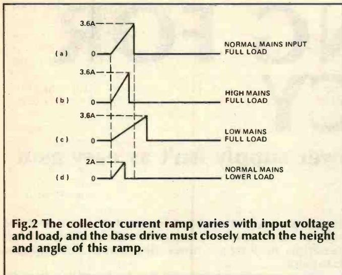
**Fig.2 The collector current ramp varies with input voltage and load, and the base drive must closely match the height and angle of this ramp.**
