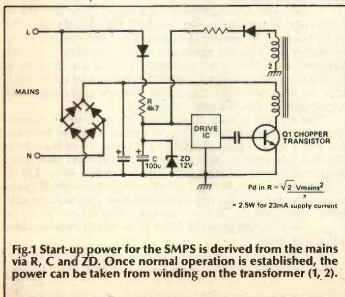
Fig.1 Start-up power for the SMPS is derived from the mains via R, C and ZD. Once normal operation is established, the power can be taken from winding on the transformer (1, 2).
