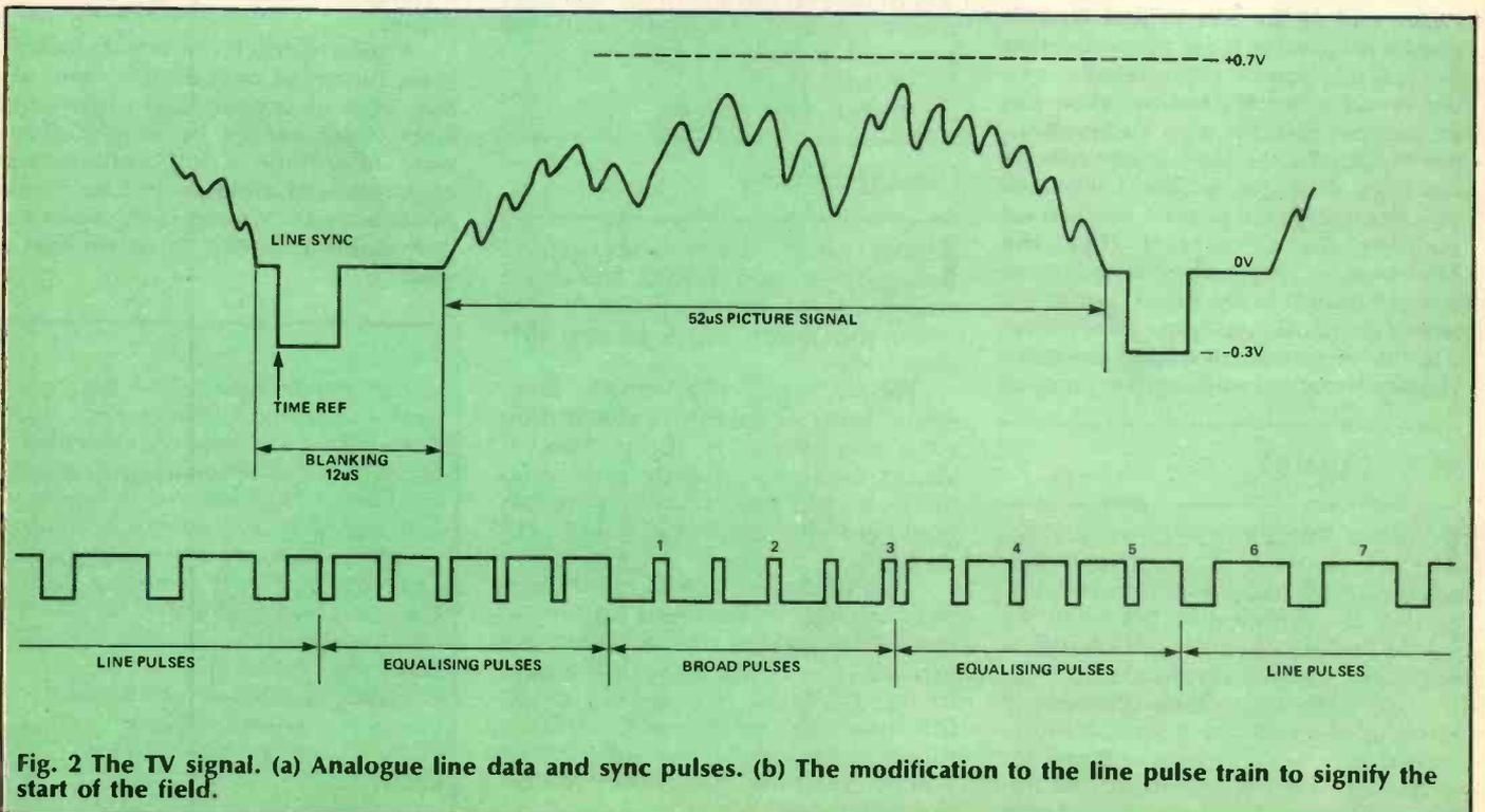
Fig. 2 The TV signal. (a) Analogue line data and sync pulses. (b) The modification to the line pulse train to signify the start of the field.
