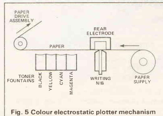
Fig. 5 Colour electrostatic plotter mechanism
