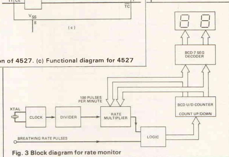
Fig. 3 Block diagram for rate monitor
