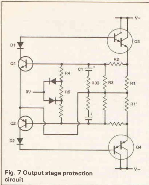
Fig. 7 Output stage protection circuit
