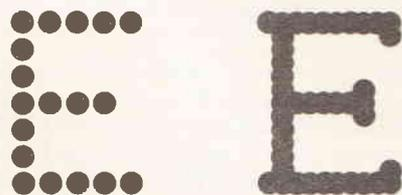
ON DOT MATRIX PRINTERS RECOGNISABLE CHARACTERS ARE BUILT UP IN DRAFT MODE WITH RELATIVELY FEW DOTS
