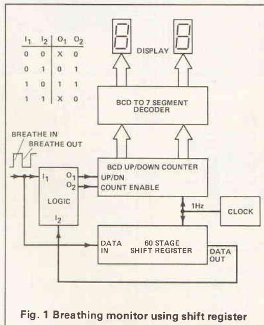
Fig. 1 Breathing monitor using shift register
