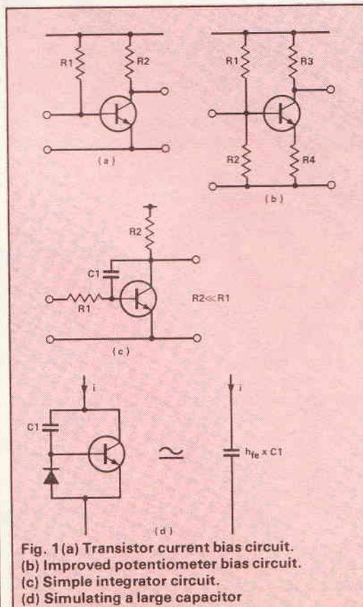
The drawback of transistors is that individually they don't have a lot of gain to give up. Useful circuit building blocks are made not from one but several devices. They also suffer from being direct embodiments of a basic physical process and make about as much concession to practicality as a piece of school laboratory equipment. The 0.7V base-emitter voltage exists not because designers want it that way but because that's how transistors are. It's how the physics works.
