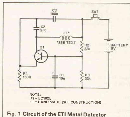
Fig. 1 Circuit of the ETI Metal Detector
