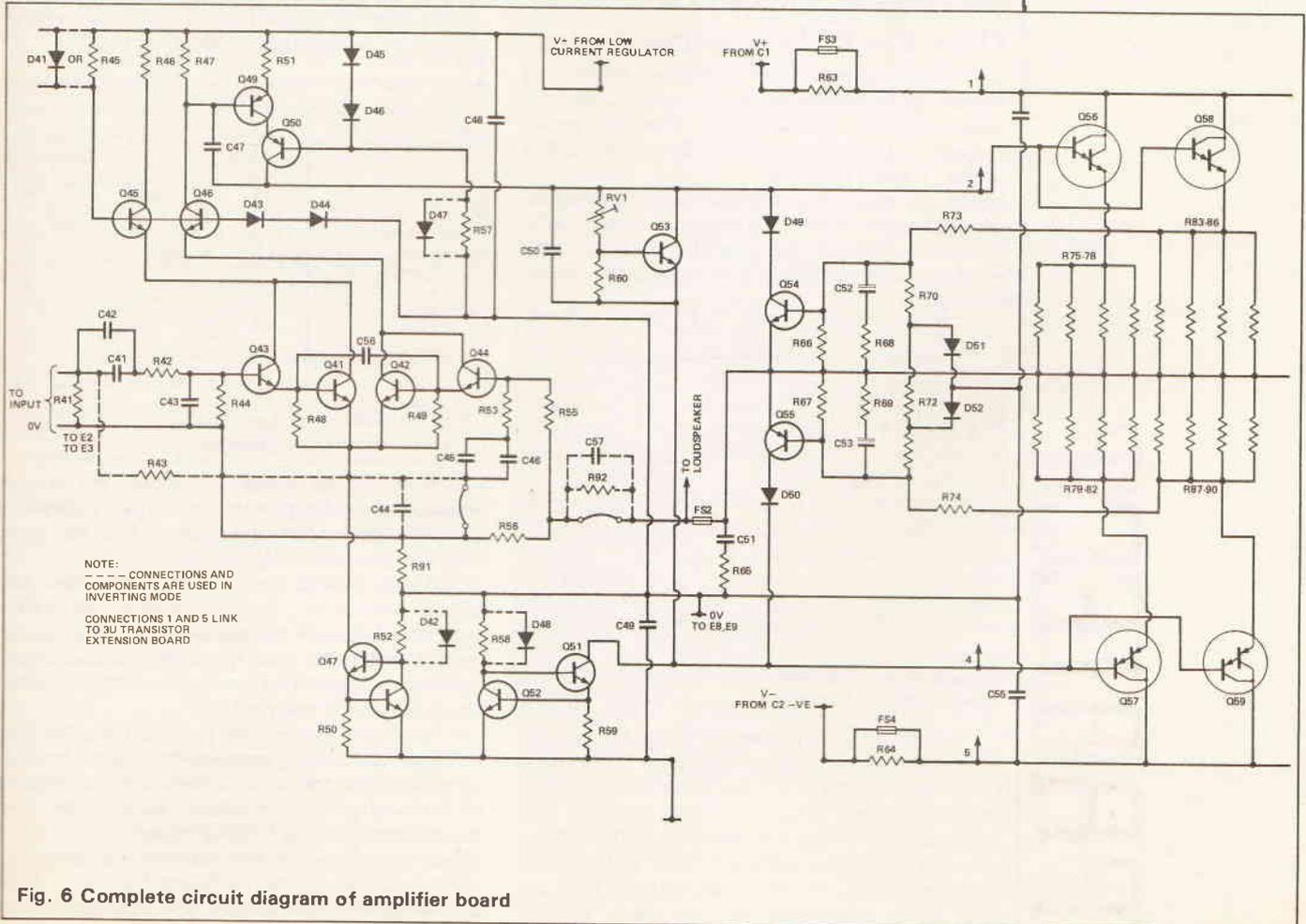
Fig. 6 Complete circuit diagram of amplifier board
