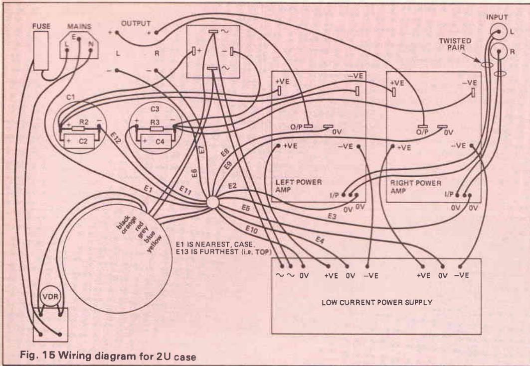
Fig. 15 Wiring diagram for 2U case
