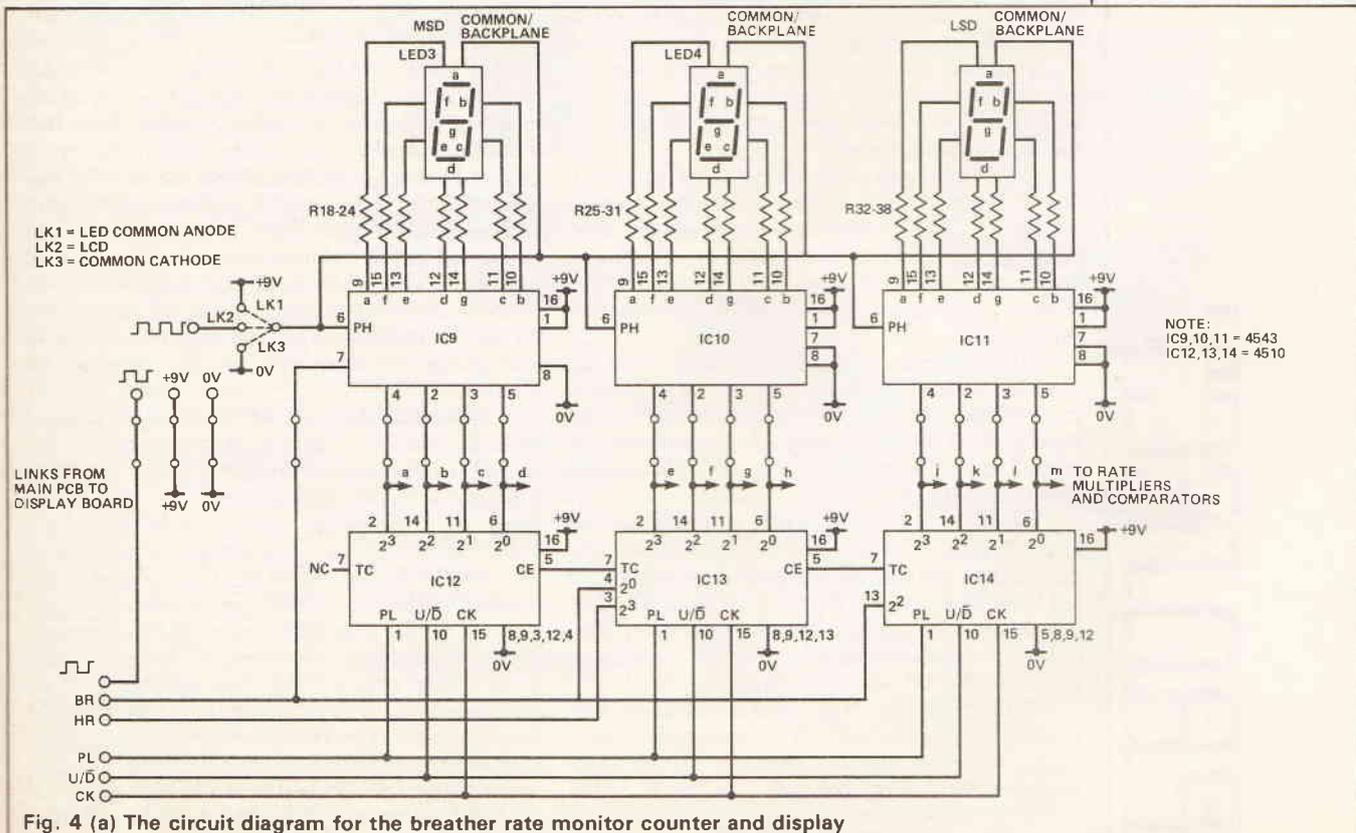
Fig. 4 (a) The circuit diagram for the breather rate monitor counter and display
