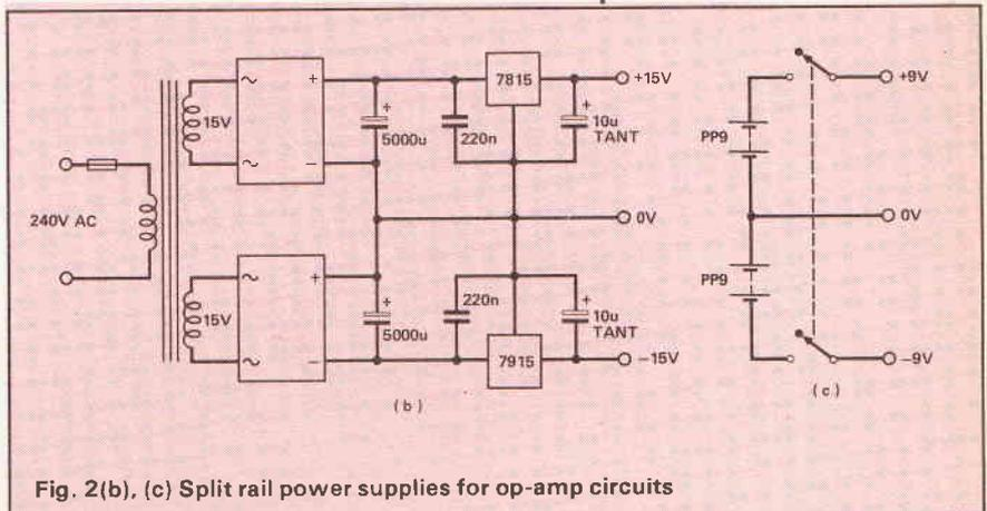
Fig. 2(b), (c) Split rail power supplies for op-amp circuits
