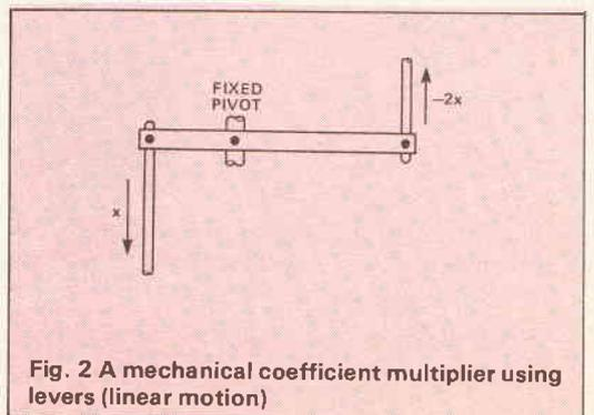
Fig. 2 A mechanical coefficient multiplier using levers (linear motion)
