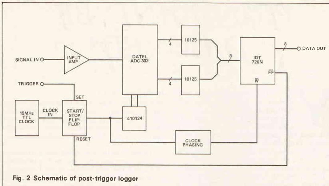
Fig. 2 Schematic of post-trigger logger
