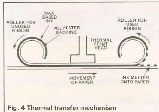
Fig. 4 Thermal transfer mechanism
