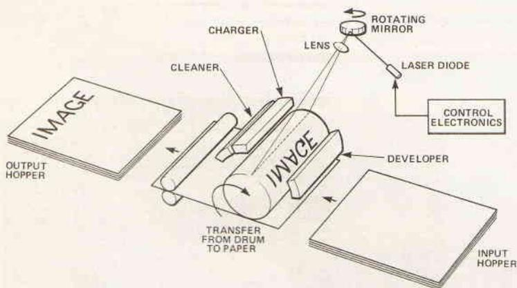
Fig. 6 Laser printer operation
