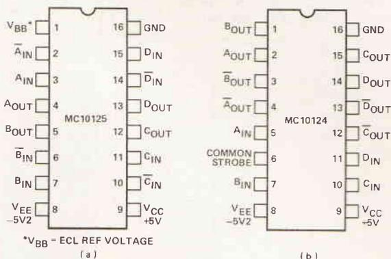
Fig. 1 (a) ECL to TTL translator. (b) TTL to ECL translator
