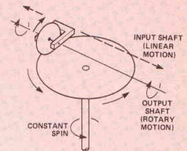
Fig. 4 The principal of the spinning disc integrator
