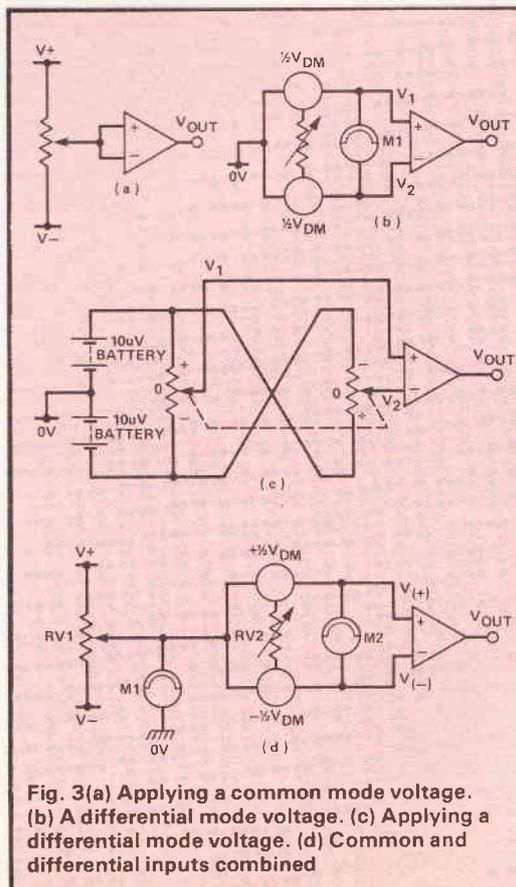
Fig. 3(a) Applying a common mode voltage. (b) A differential mode voltage. (c) Applying a differential mode voltage. (d) Common and differential inputs combined
