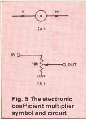
Fig. 5 The electronic coefficient multiplier symbol and circuit
