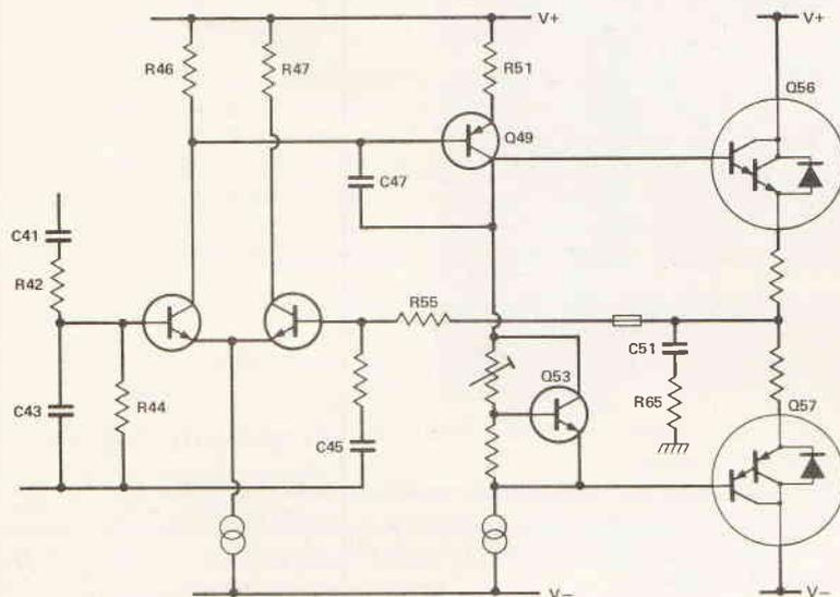
Fig. 5 Simplified circuit diagram of Virtuoso
