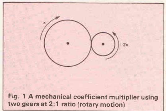
Fig. 1 A mechanical coefficient multiplier using two gears at 2:1 ratio (rotary motion)
