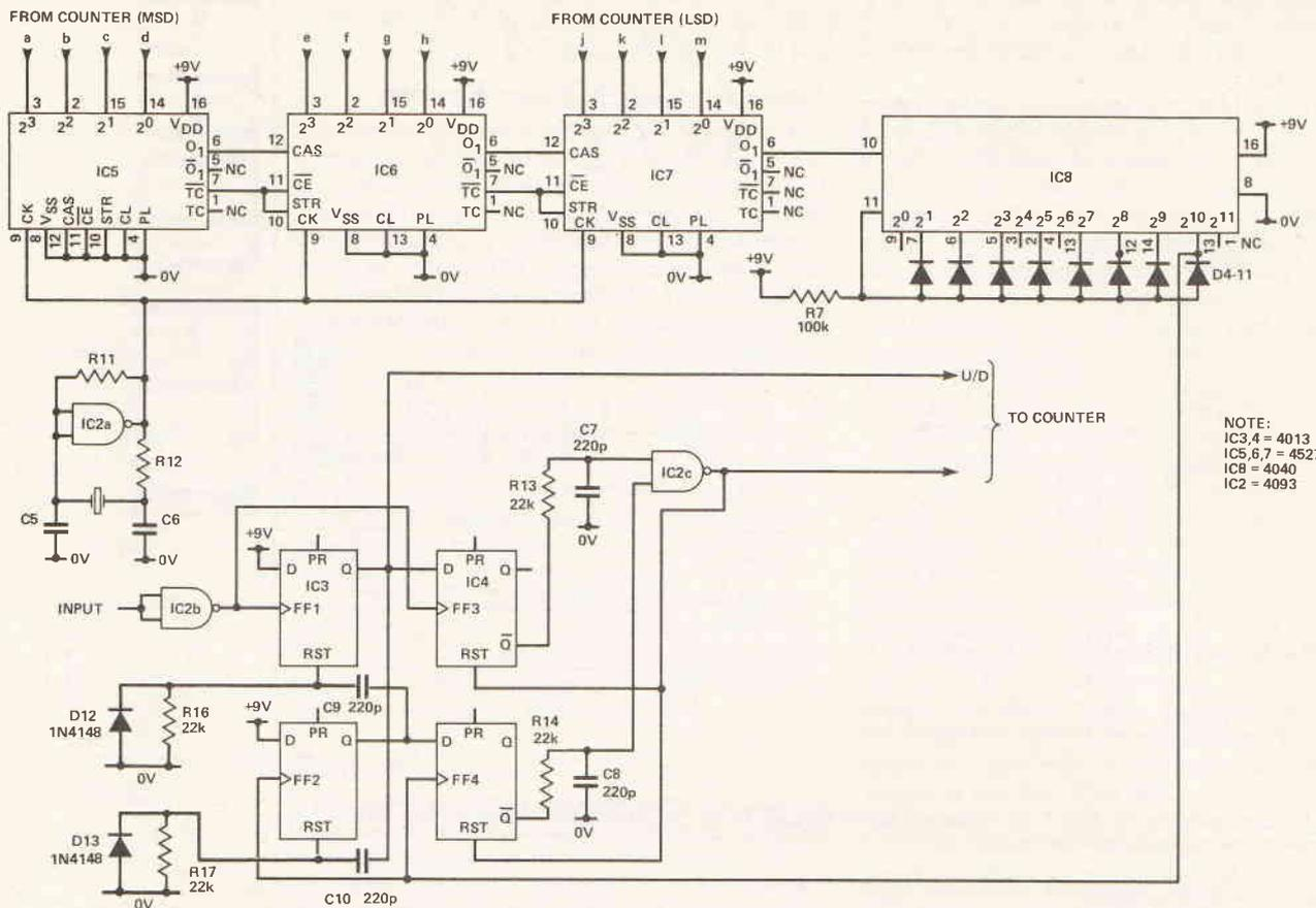
Fig. 4 (b) The rate multiplication circuit
