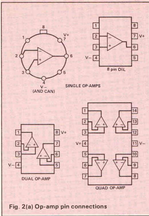
Fig. 2(a) Op-amp pin connections
