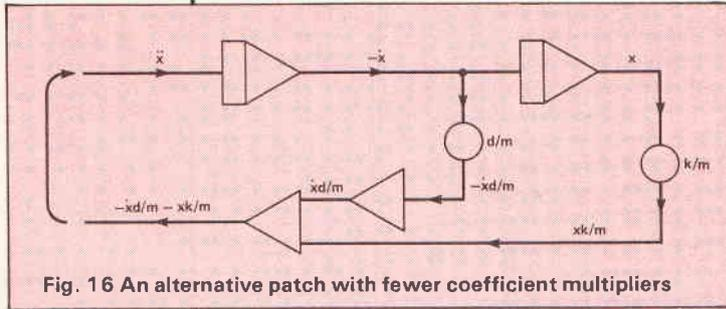
Fig. 16 An alternative patch with fewer coefficient multipliers
