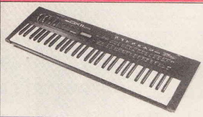
**T**he latest DX keyboard from Yamaha is the DX11, an eight note polyphonic instrument with a five octave velocity sensitive keyboard.
