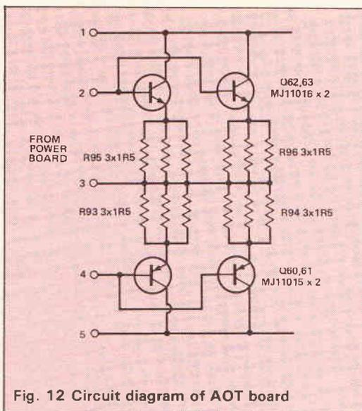
Fig. 12 Circuit diagram of AOT board
