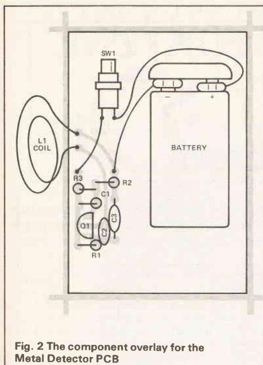
Fig. 2 The component overlay for the Metal Detector PCB
