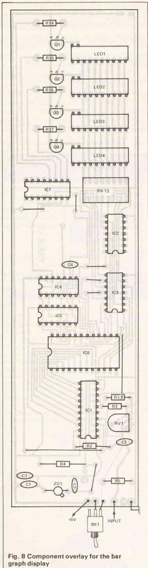
Fig. 8 Component overlay for the bar graph display
