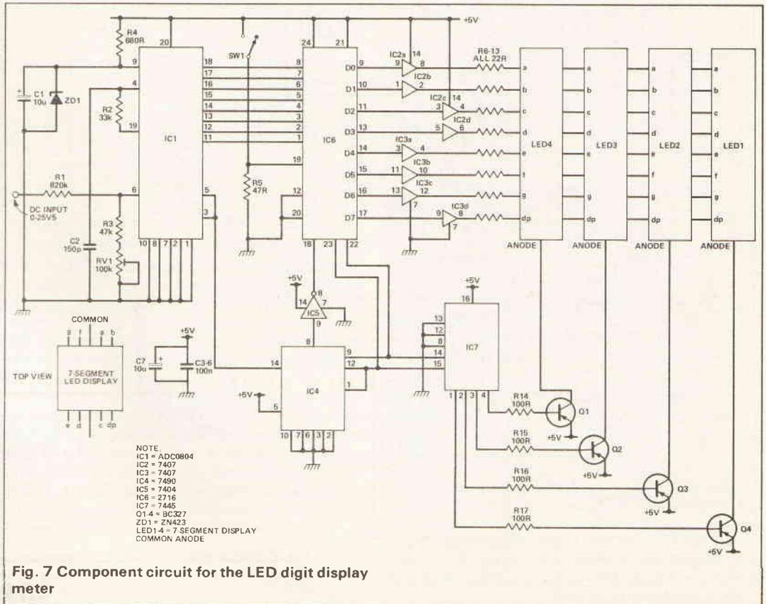
Fig. 7 Component circuit for the LED digit display meter
