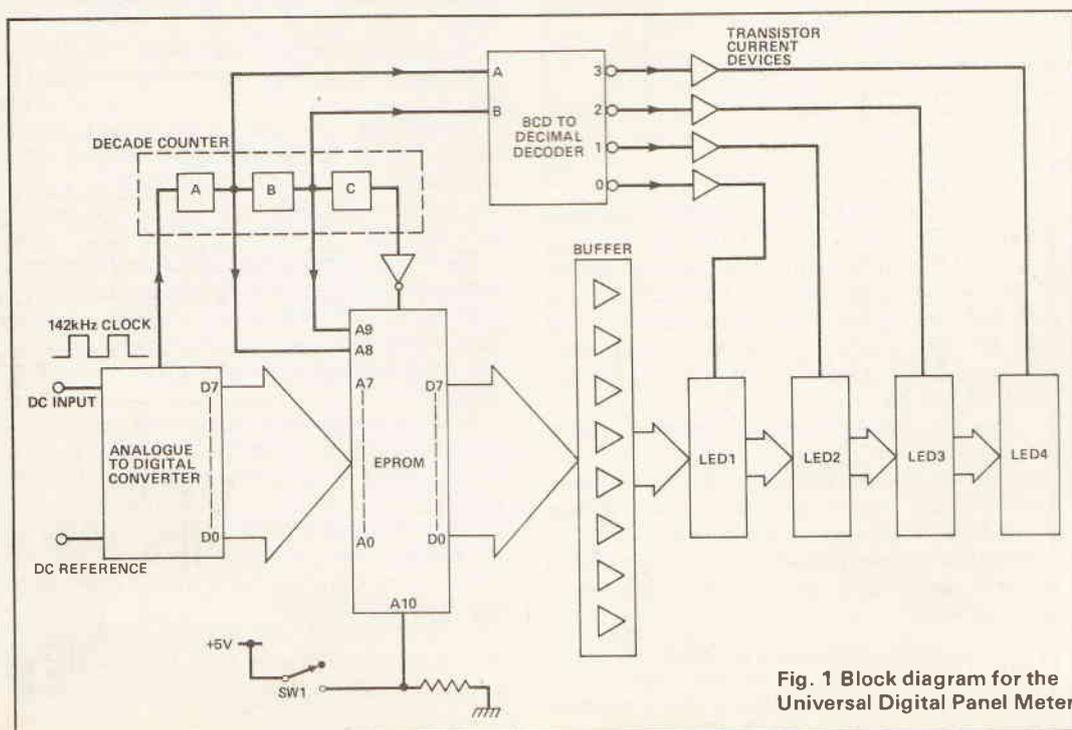
Fig. 1 Block diagram for the Universal Digital Panel Meter
