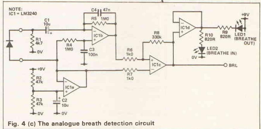
Fig. 4 (c) The analogue breath detection circuit
