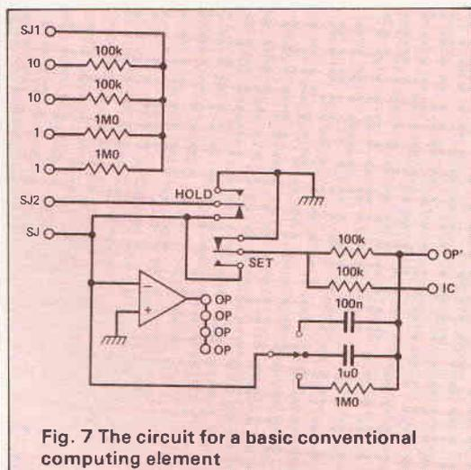
Fig. 7 The circuit for a basic conventional computing element
