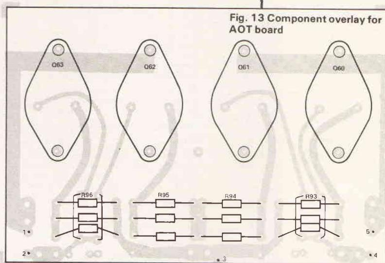
Fig. 13 Component overlay for AOT board
