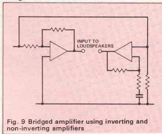
Fig. 9 Bridged amplifier using inverting and non-inverting amplifiers
