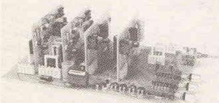
Complete record and replay circuits for very high quality low noise stereo cassette recorder. Circuits are optimised for our HS16 Super Quality Sendust Alloy Head. Switched bias and equalisation to cater for chrome and ferric tapes. Very easy to assemble on plug-in PCBs. Complete with full instructions.
