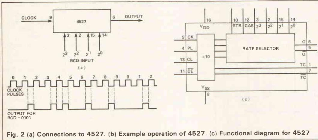
Fig. 2 (a) Connections to 4527. (b) Example operation of 4527. (c) Functional diagram for 4527
