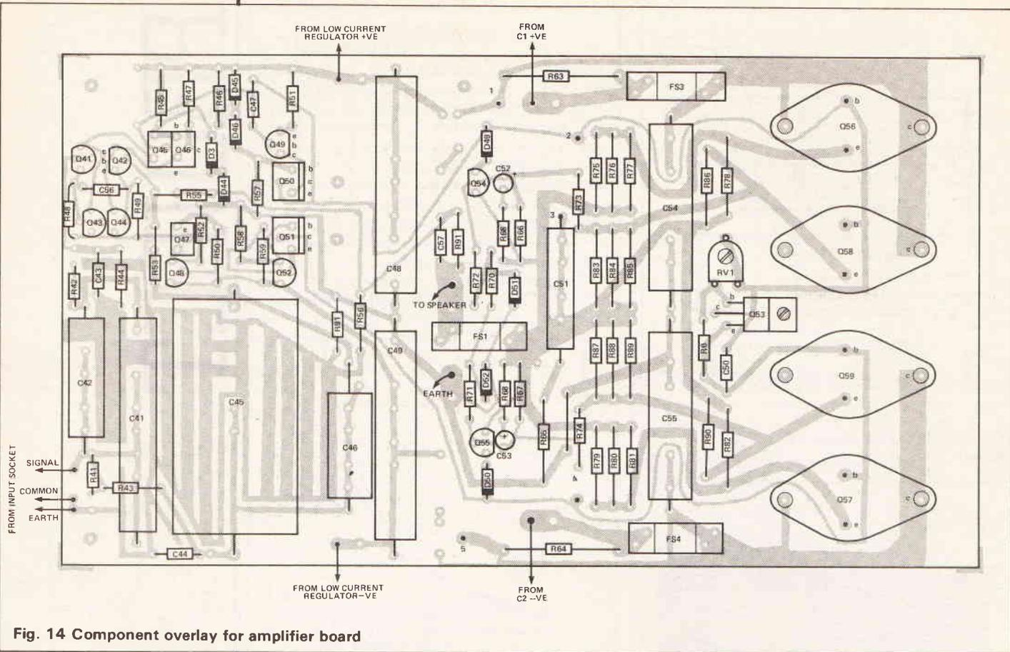
Fig. 14 Component overlay for amplifier board
