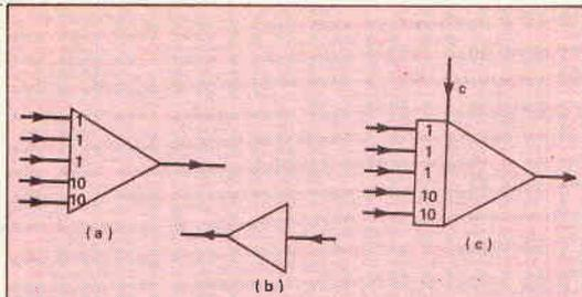
**Fig. 9 Symbols for the Aberdeen unit computing elements (a) Summer (b) Inverter (c) Integrator**
