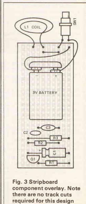
Fig. 3 Stripboard component overlay. Note there are no track cuts required for this design
