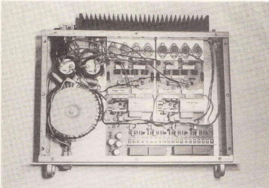
In the third and final article on the Virtuoso Power Amplifier I will look at the power amplifier board itself and at the decisions that were taken concerning its design. First comes the choice whether to operate in class A, sliding class A or class AB.
