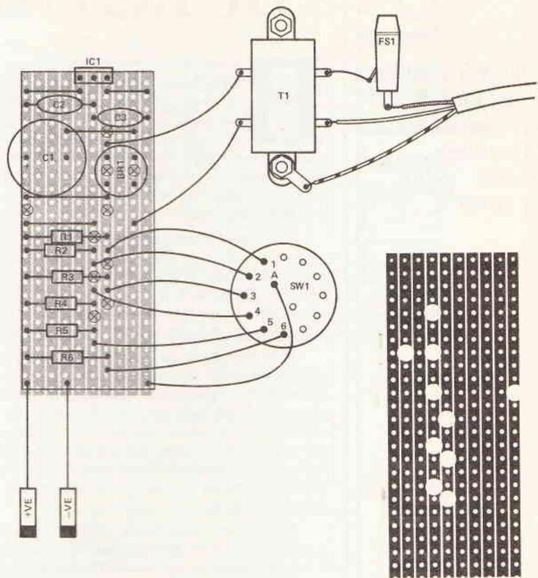
Fig.4 Stripboard layout wiring, and track cuts on reverse
