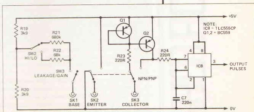
Fig. 4 The circuit diagram of the input section
