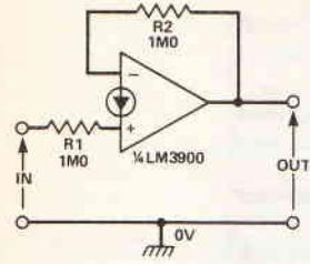
Fig. 11 DC voltage-following buffer
