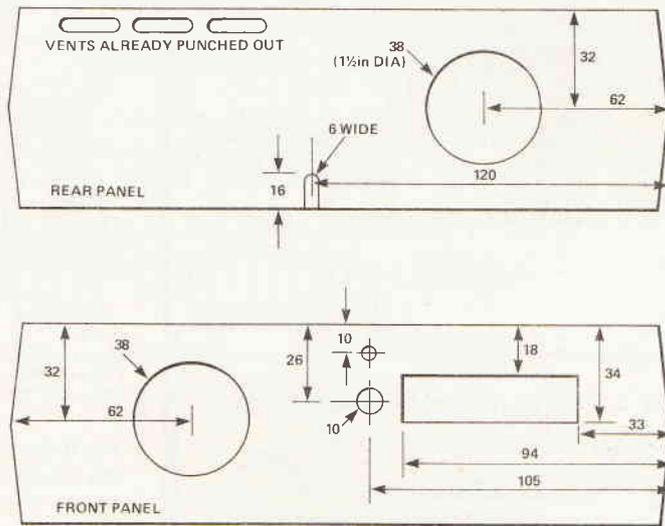
Fig. 10 Case cutouts for the recommended case
