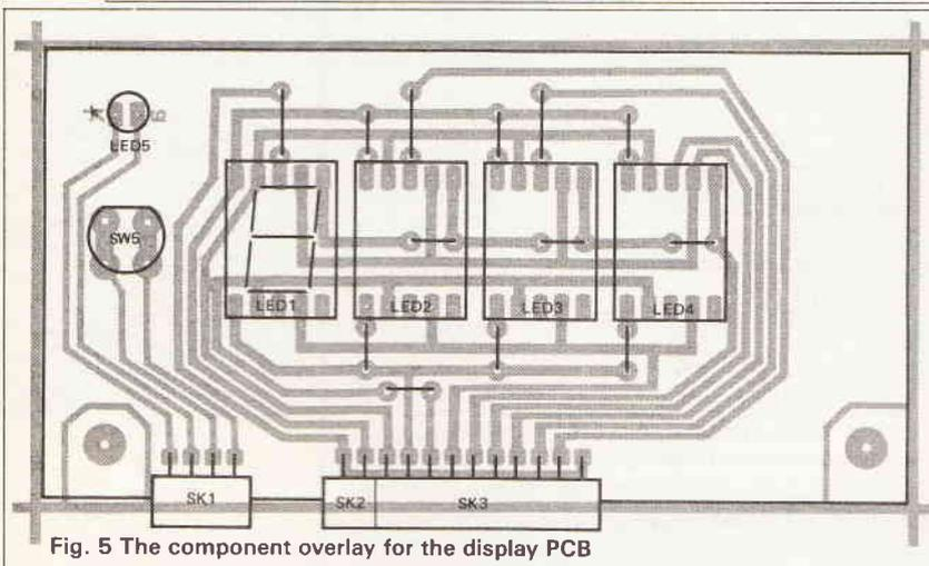
Fig. 5 The component overlay for the display PCB
