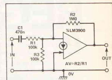
Fig. 7 Inverting AC amplifier with  $N \times V_{be}$  biassing
