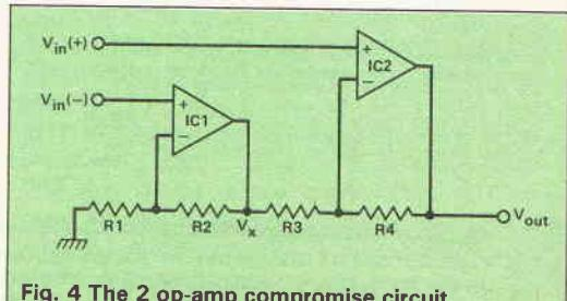
Fig. 4 The 2 op-amp compromise circuit
