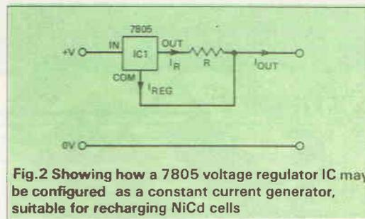
Fig.2 Showing how a 7805 voltage regulator IC may be configured as a constant current generator, suitable for recharging NiCd cells
