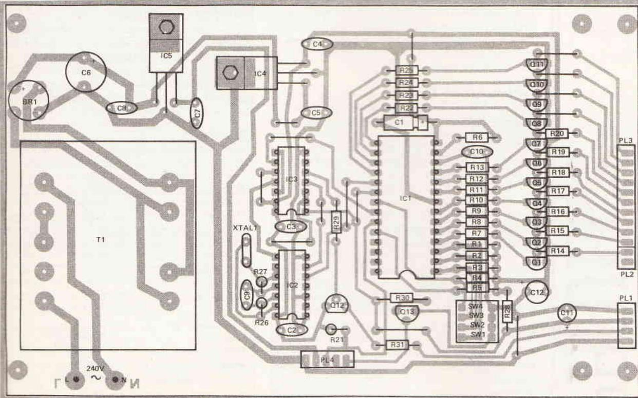
Fig. 3 The component overlay for the counter PCB
