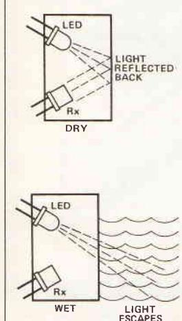
Fig. 3. A refractive fluid level sensor
