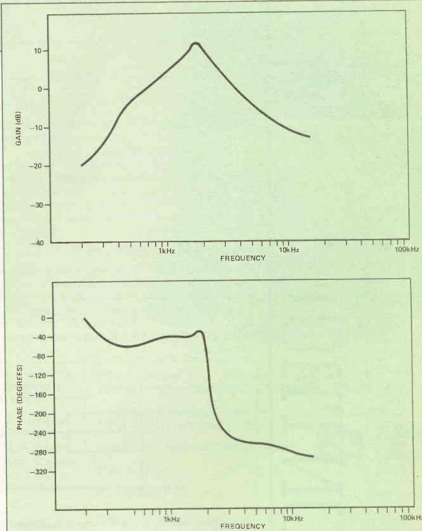
Fig. 9 Final Bode plot estimate of closed-loop frequency response of the system of Fig. 5 when its feedback loop has been closed. Taken from closed-loop response as shown on the Nichols chart of Fig. 8
