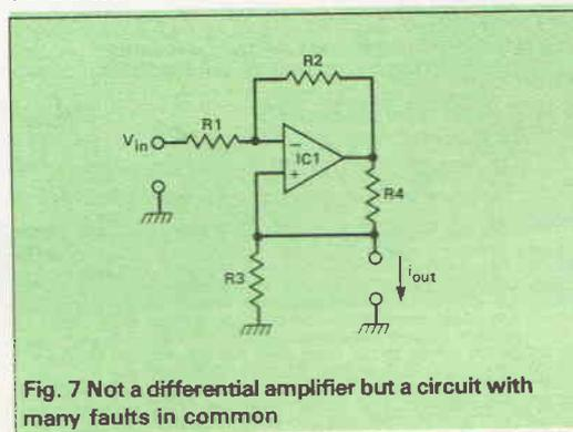
Fig. 7 Not a differential amplifier but a circuit with many faults in common
