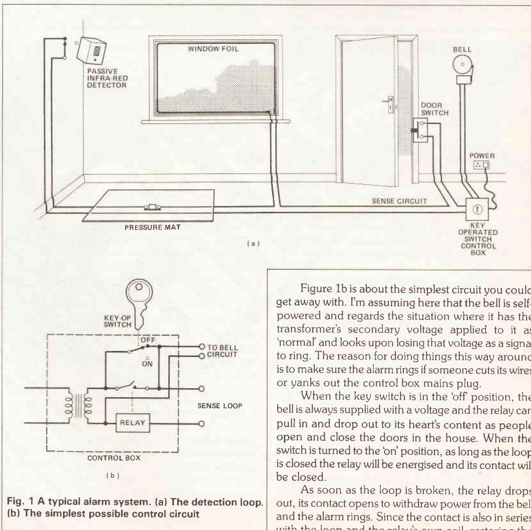
Fig. 1 A typical alarm system. (a) The detection loop. (b) The simplest possible control circuit
