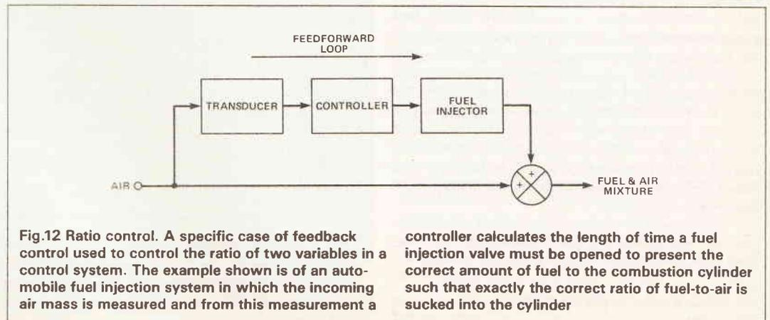
Fig. 12 Ratio control. A specific case of feedback control used to control the ratio of two variables in a control system. The example shown is of an automobile fuel injection system in which the incoming air mass is measured and from this measurement a
