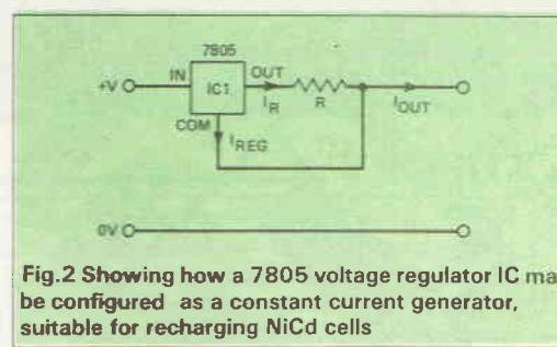
Fig.2 Showing how a 7805 voltage regulator IC may be configured as a constant current generator, suitable for recharging NiCd cells
