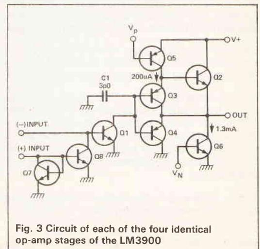
Fig. 3 Circuit of each of the four identical op-amp stages of the LM3900
