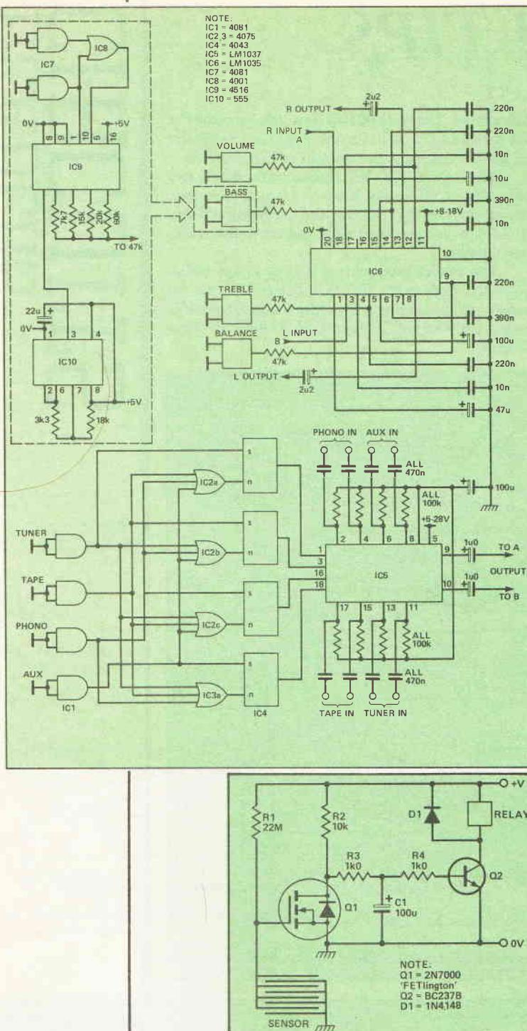
**A** touch controlled pre-amp with touch plate selection of inputs and volume, bass, treble and balance can be easily constructed with the help of the LM1037 and 1035 audio control ICs.
