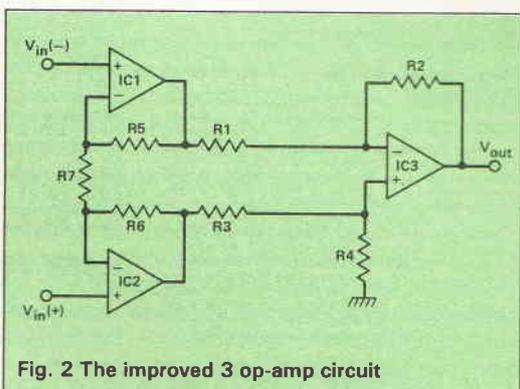
Fig. 2 The improved 3 op-amp circuit
