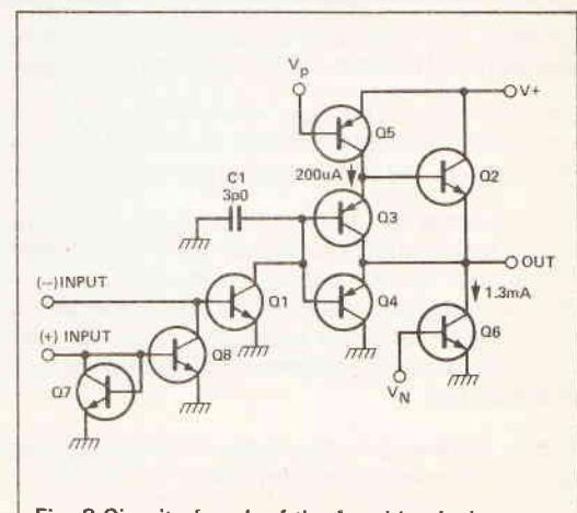
Fig. 3 Circuit of each of the four identical op-amp stages of the LM3900
