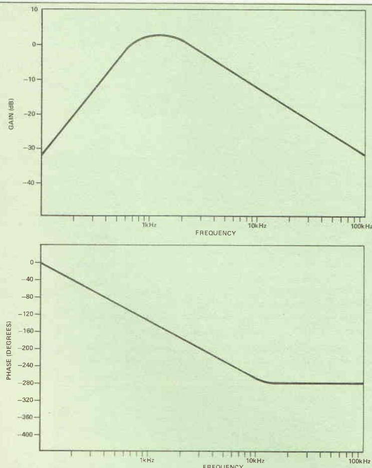
Fig. 7 Estimate of final pair of Bode plots of the system in Fig. 5, found by adding together gains and phase shifts of all three pairs of plots at each frequency
