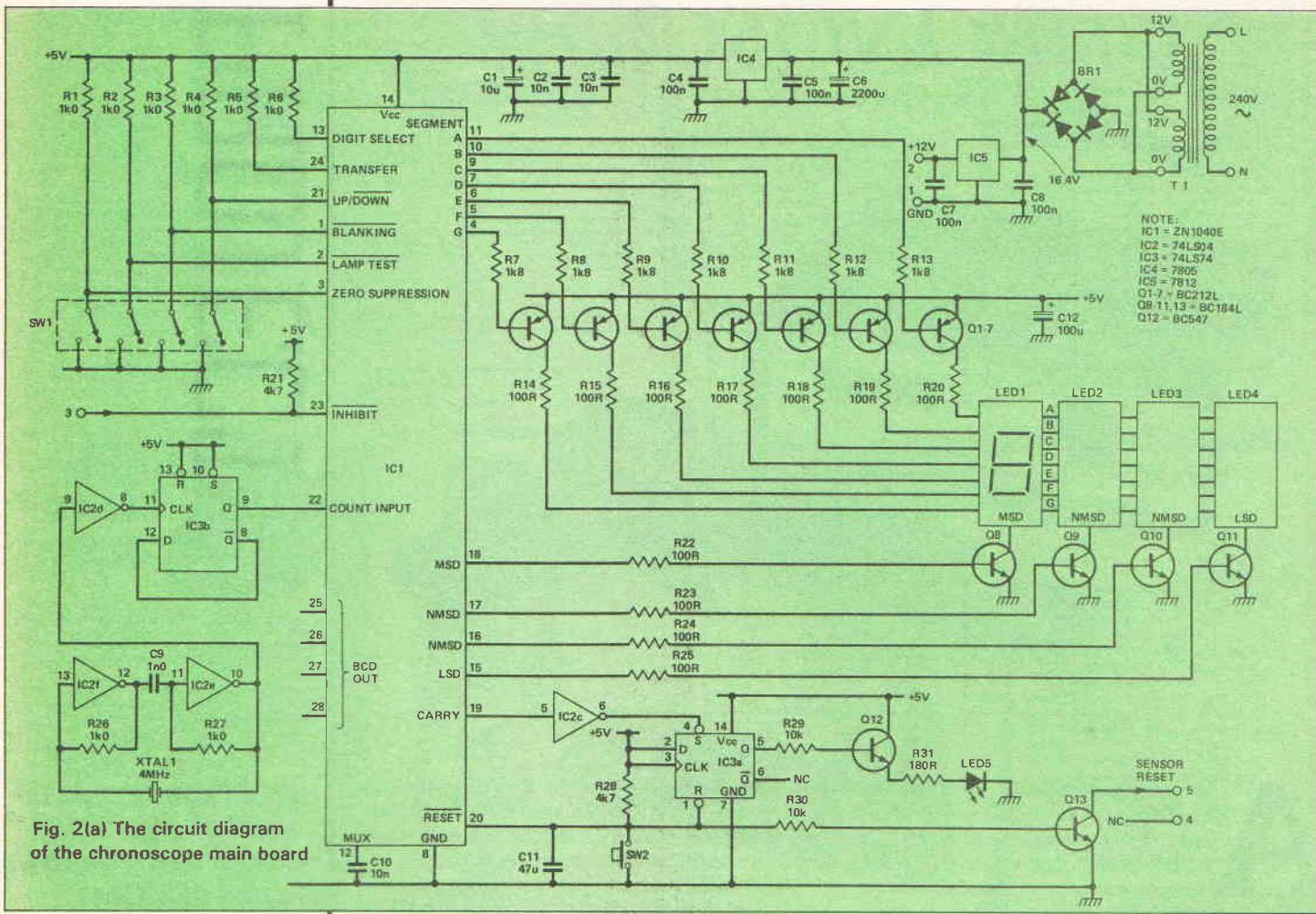
Fig. 2(a) The circuit diagram of the chronoscope main board
