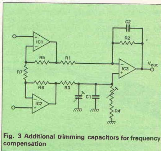
Fig. 3 Additional trimming capacitors for frequency compensation
