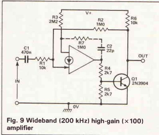
Fig. 9 Wideband (200 kHz) high-gain ( $\times 100$ ) amplifier
