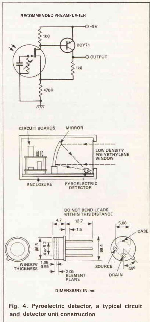
Fig. 4. Pyroelectric detector, a typical circuit and detector unit construction
