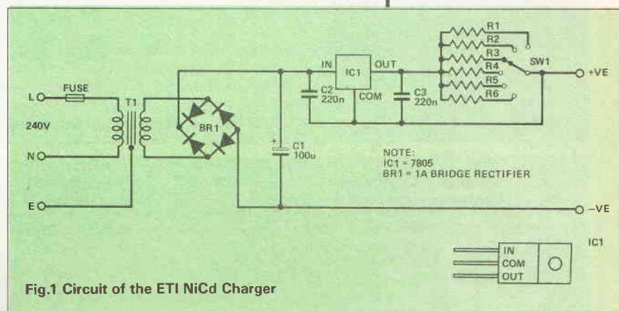
Fig.1 Circuit of the ETI NiCd Charger
