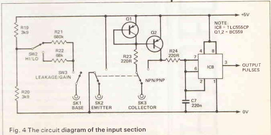
Fig. 4 The circuit diagram of the input section
