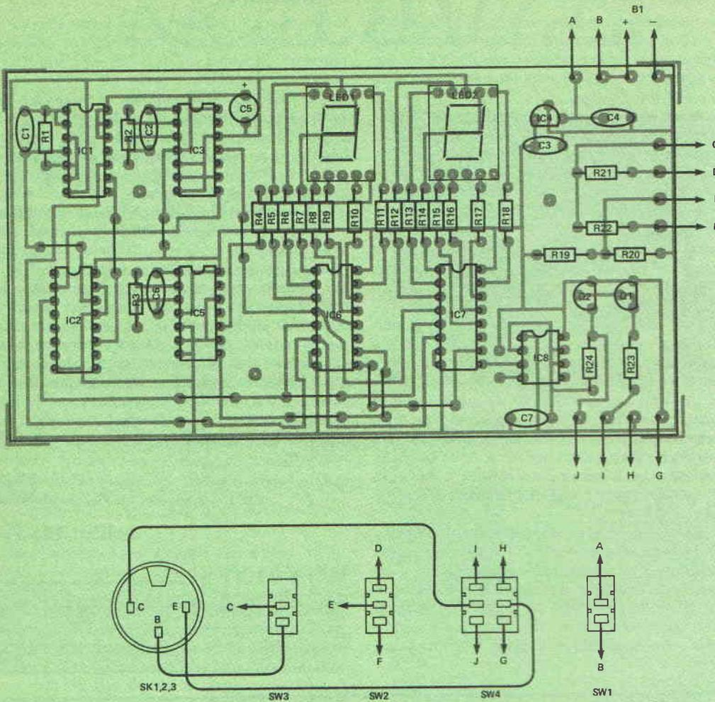
Fig. 5 Component overlay and inter-wiring diagrams for the digital transistor tester
