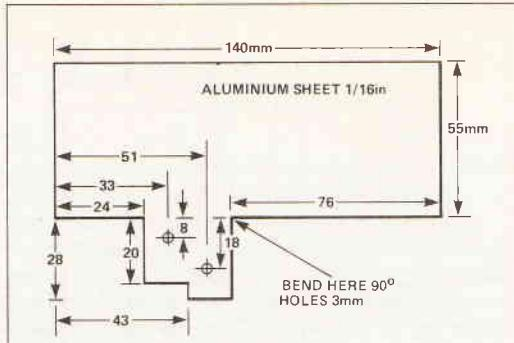
Fig. 6 The heatsink for IC4,5
