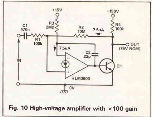
Fig. 10 High-voltage amplifier with  $\times 100$  gain
