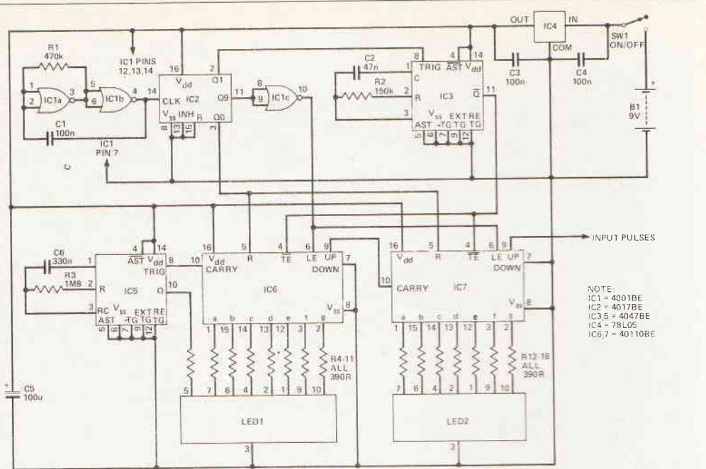
Fig. 3 The circuit diagram of the display section
