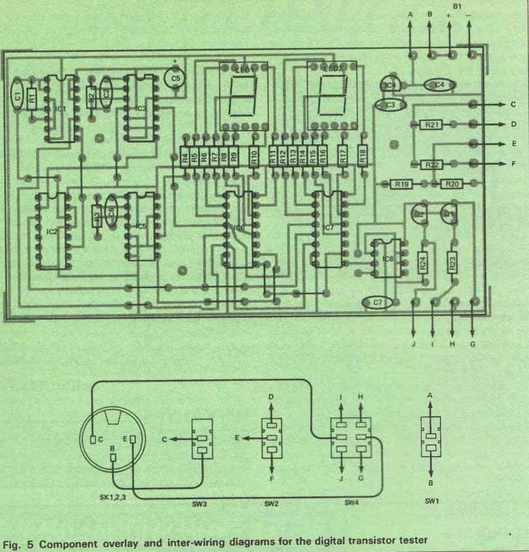
Fig. 5 Component overlay and inter-wiring diagrams for the digital transistor tester
