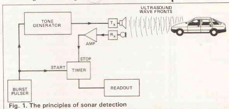
Fig. 1. The principles of sonar detection
