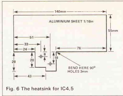
Fig. 6 The heatsink for IC4,5
