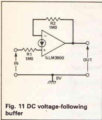
Fig. 11 DC voltage-following buffer
