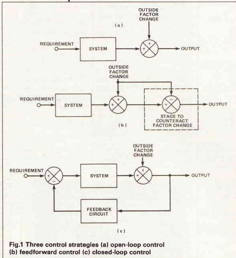
Fig.1 Three control strategies (a) open-loop control (b) feedforward control (c) closed-loop control
