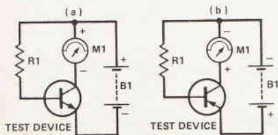
Fig. 1 Basic test circuits for NPN and PNP transistors
