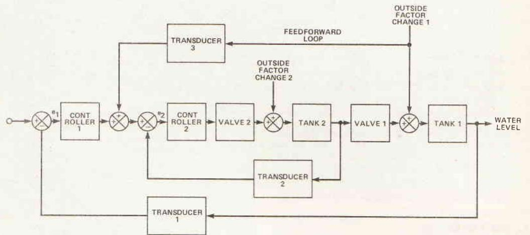
Fig. 11 Feedback control, used with the cascade control example of Fig. 11 to reduce the effects of disturbances which take place outside the inner cascade loop
