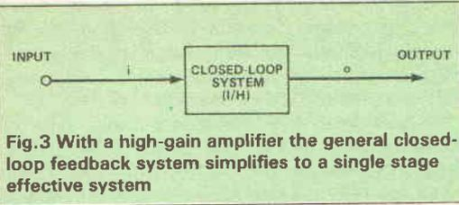
Fig. 3 With a high-gain amplifier the general closed-loop feedback system simplifies to a single stage effective system
