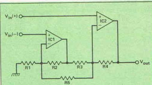
Fig. 6 The improved 2 op-amp circuit
