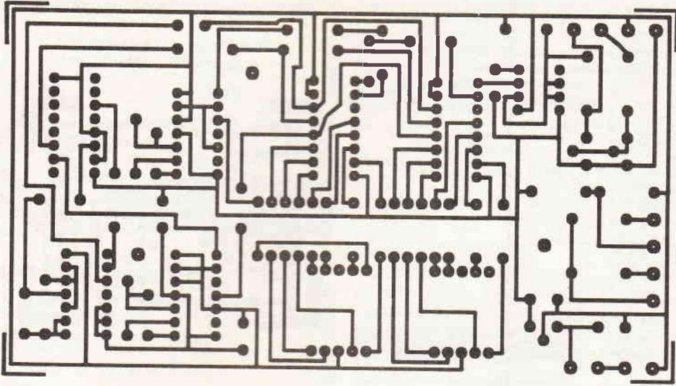
The Chronoscope display PCB
