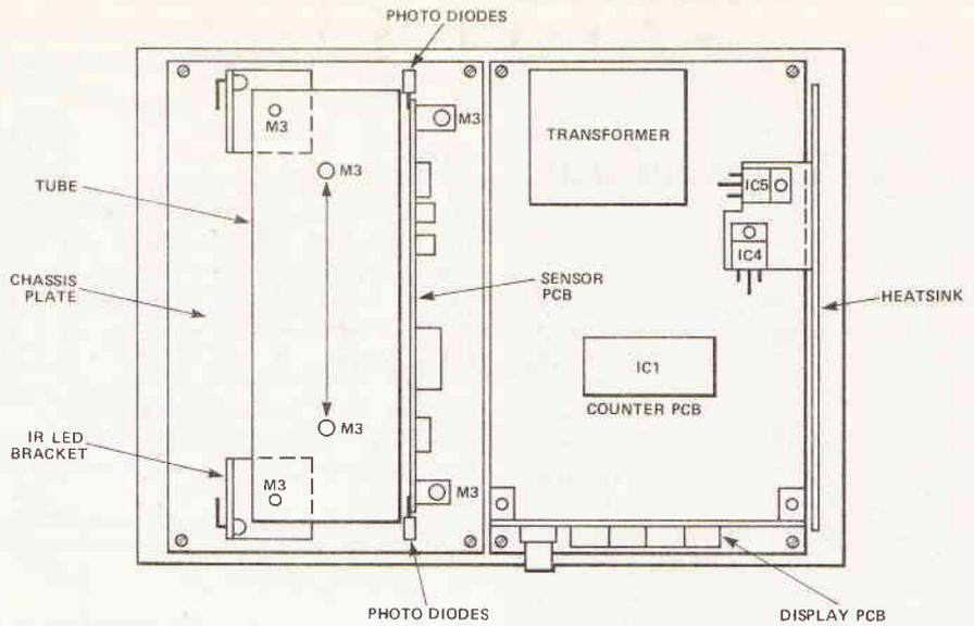
Fig. 9 The layout of the major parts of the prototype chronoscope
