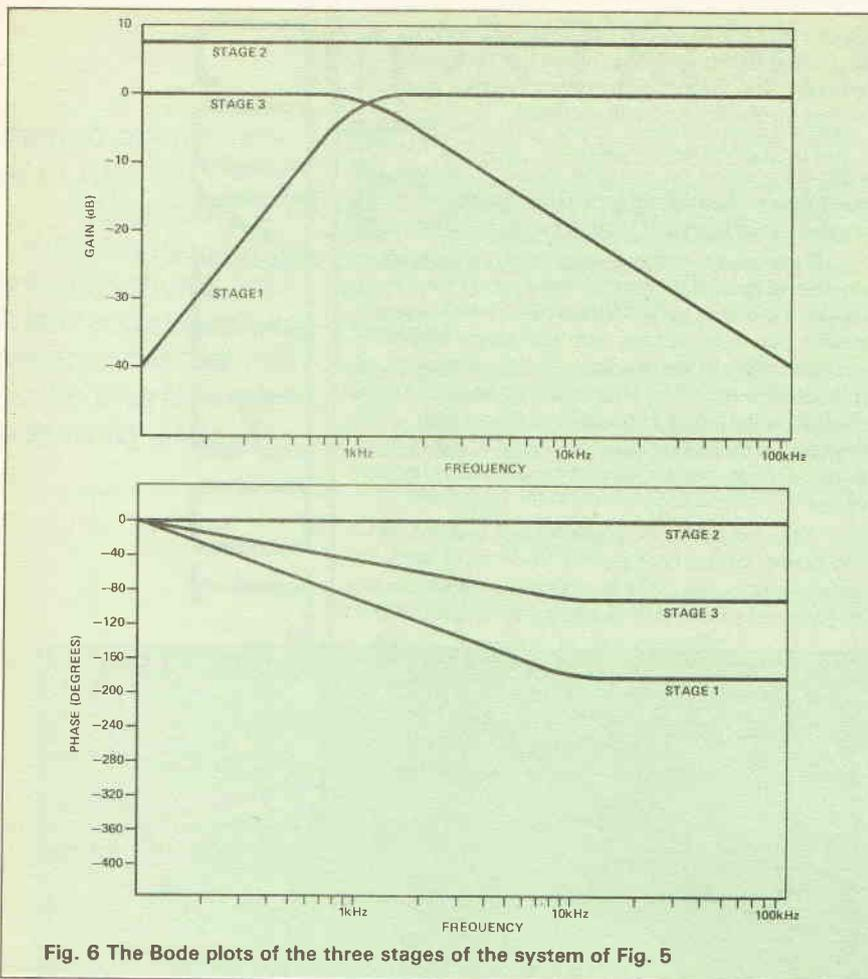
Fig. 6 The Bode plots of the three stages of the system of Fig. 5
