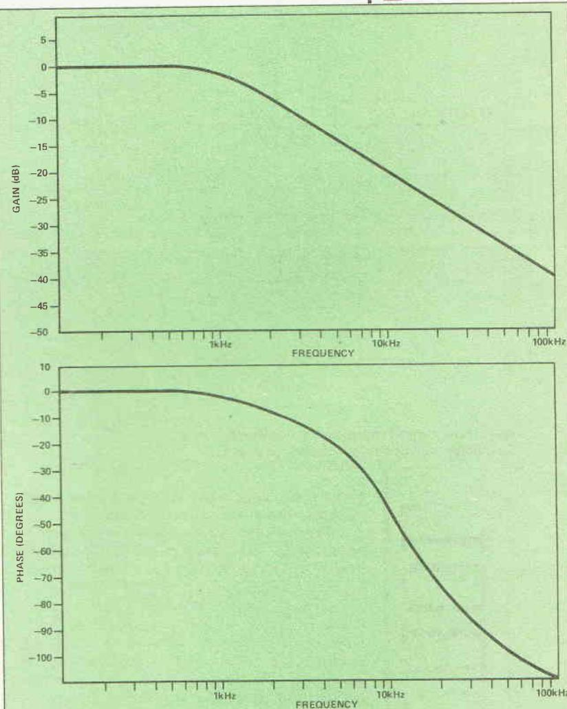
Fig. 4 A possible pair of Bode plots. The upper plot has gain (in dB) as the vertical axis with frequency as the horizontal axis. The lower plot has phase shift (in degrees) as its vertical axis
