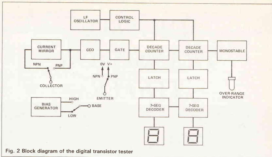
Fig. 2 Block diagram of the digital transistor tester
