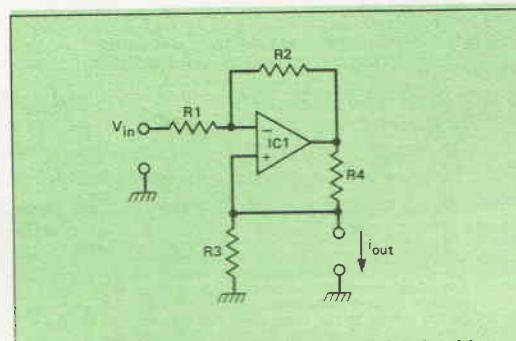
Fig. 7 Not a differential amplifier but a circuit with many faults in common
