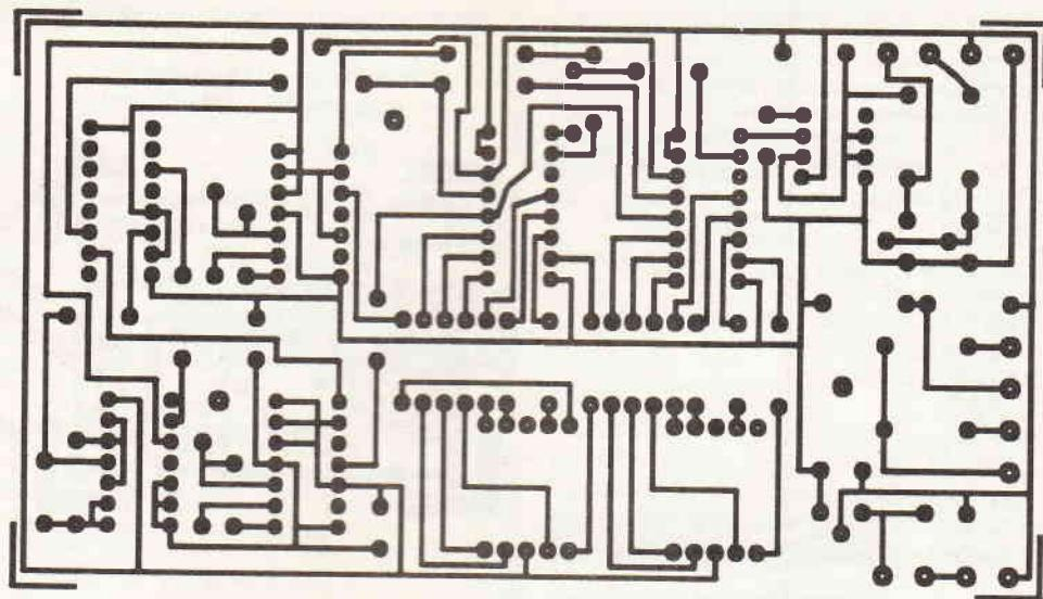
The Chronoscope display PCB
