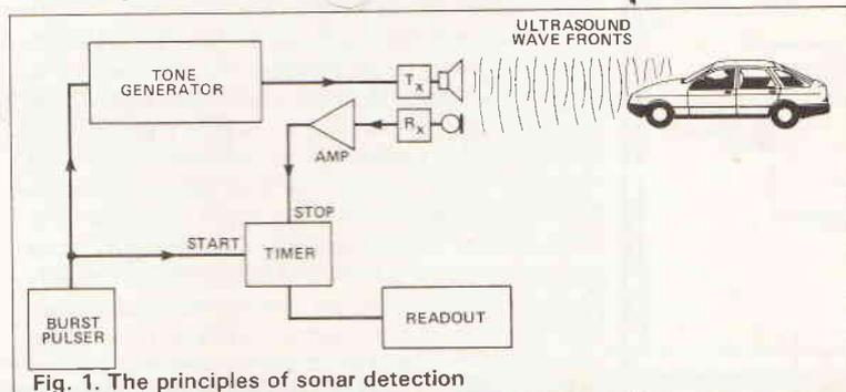
Fig. 1. The principles of sonar detection
