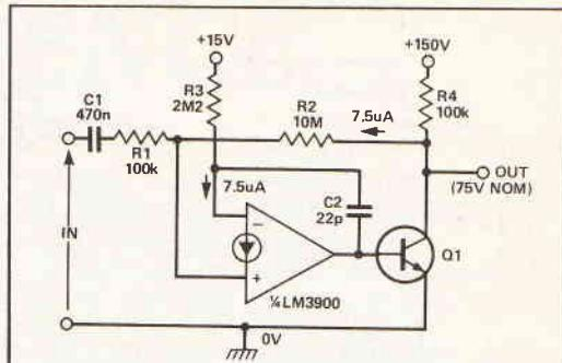
Fig. 10 High-voltage amplifier with  $\times 100$  gain
