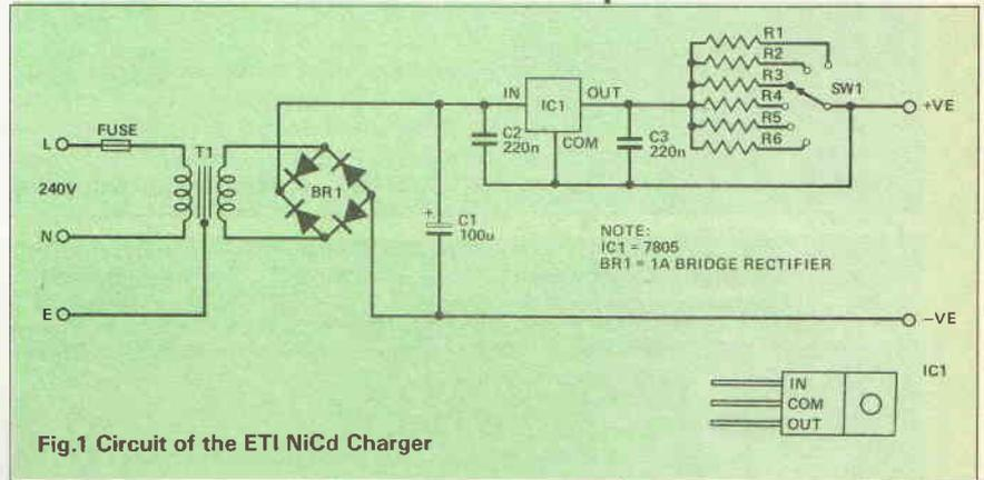
Fig.1 Circuit of the ETI NiCd Charger
