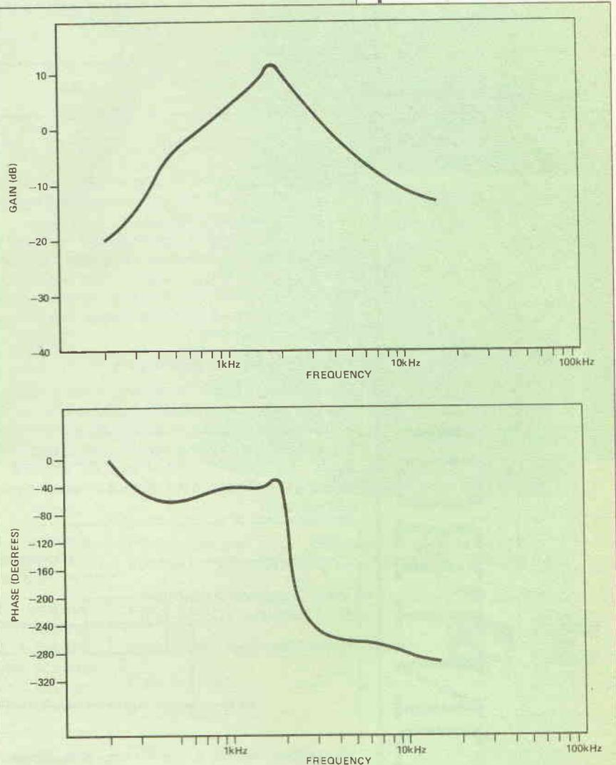
**Fig. 9** Final Bode plot estimate of closed-loop frequency response of the system of Fig. 5 when its feedback loop has been closed. Taken from closed-loop response as shown on the Nichols chart of Fig. 8
