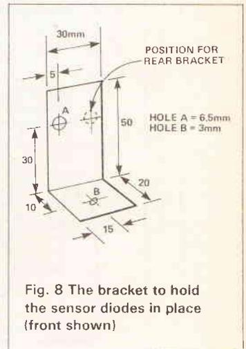
Fig. 8 The bracket to hold the sensor diodes in place (front shown)
