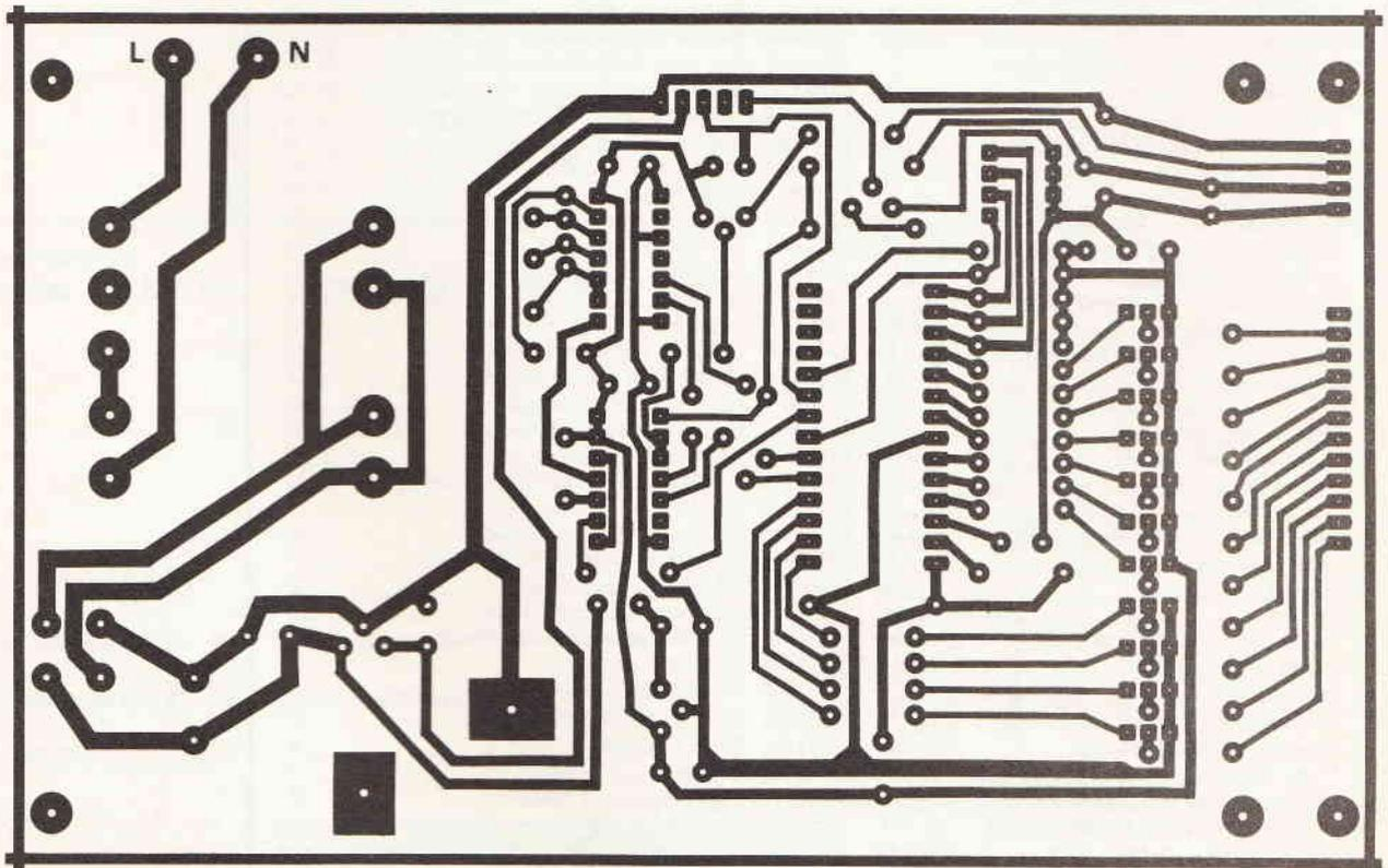
The Chronoscope counter PCB
