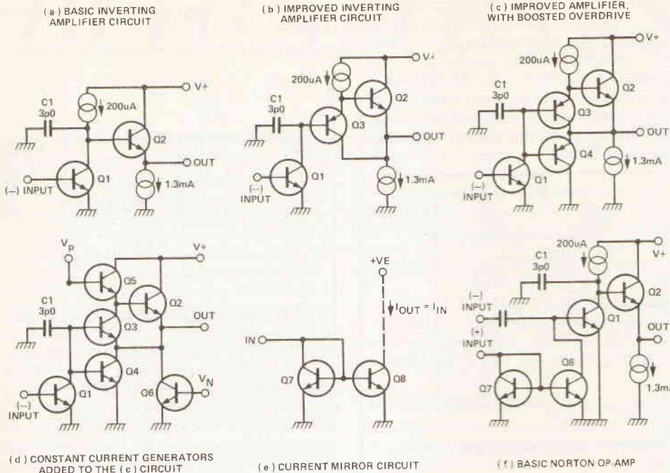
Fig. 4 Development of the LM3900 op-amp circuit
