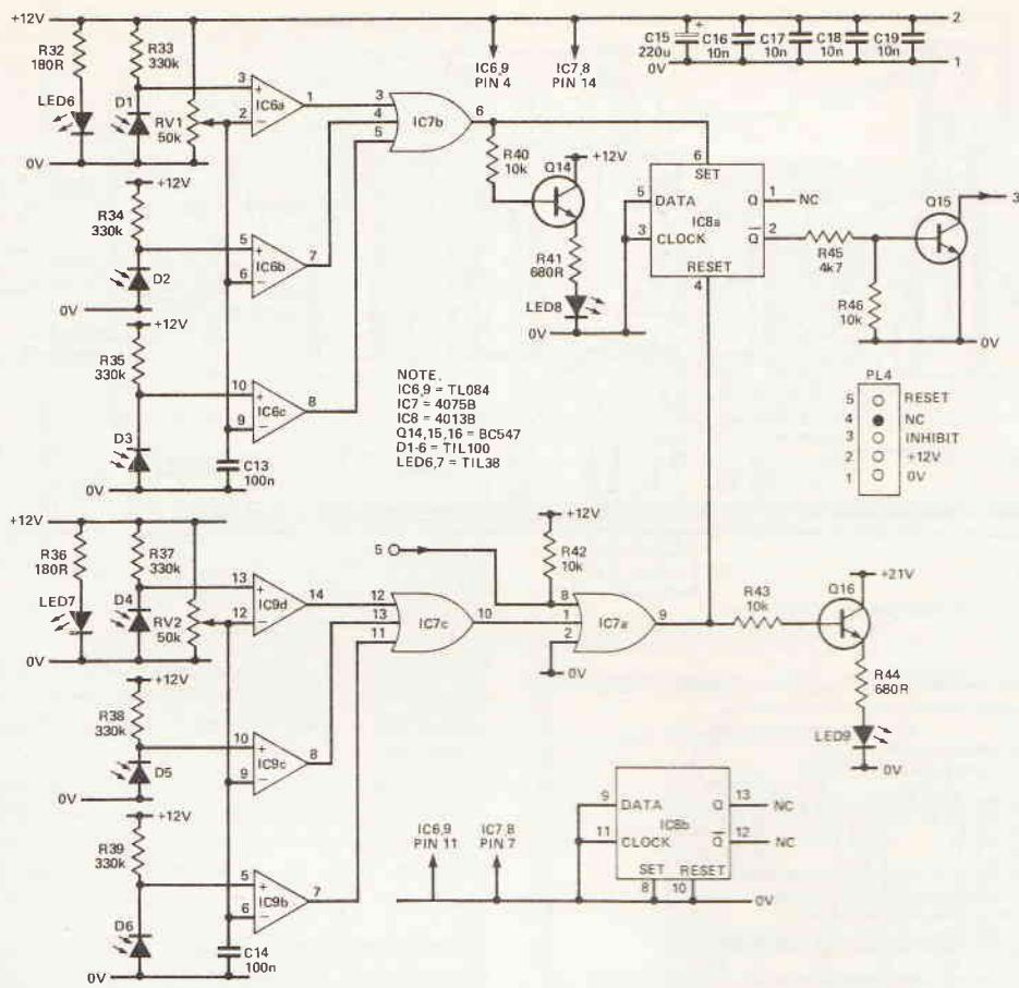
Fig. 2(b) Circuit diagram of the sensor board
