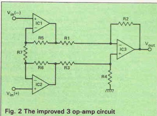
Fig. 2 The improved 3 op-amp circuit
