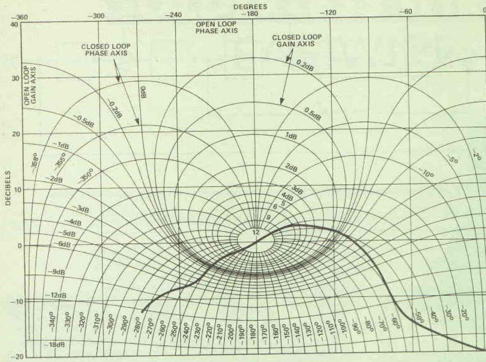
**Fig. 8** A Nichols chart showing open and closed-loop gain and phase shift axes with a frequency response curve, taken from the results of the Bode plots of Fig. 7, transferred onto a Nichols chart
