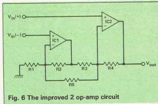
Fig. 6 The improved 2 op-amp circuit
