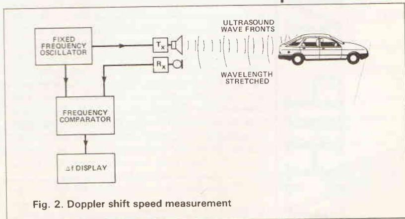
Fig. 2. Doppler shift speed measurement
