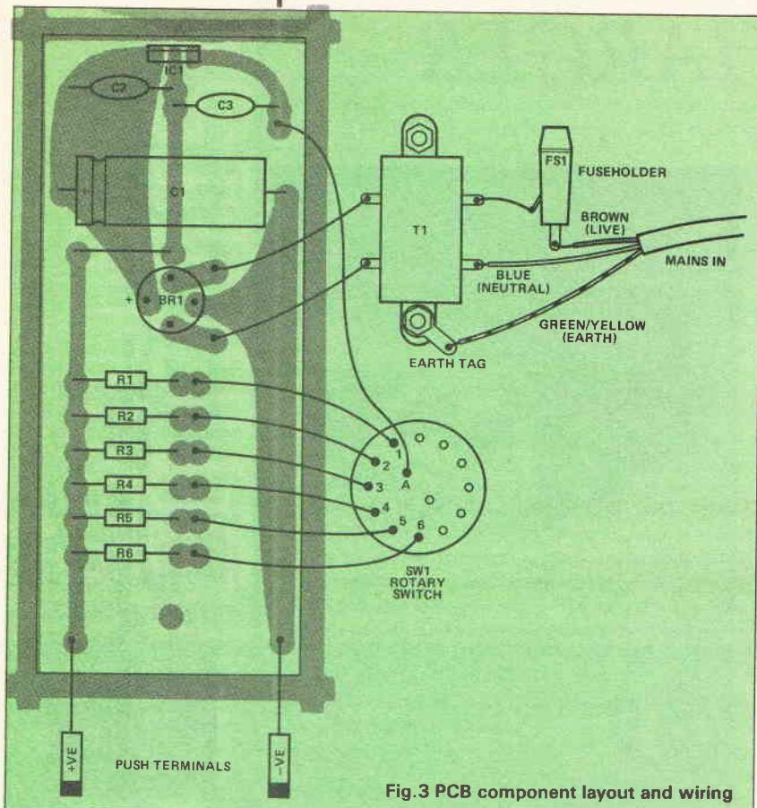
Fig.3 PCB component layout and wiring
