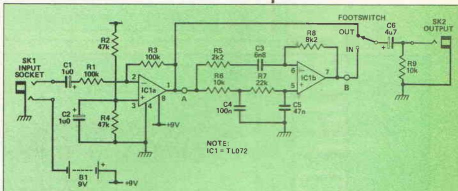
The circuit can be built as a footpedal powered from a PP3 (no power LED is included to extend battery life). If fitted in your amplifier between preamp and power amp then the buffering and level shifting circuitry can be omitted leaving just the components between A and B.
