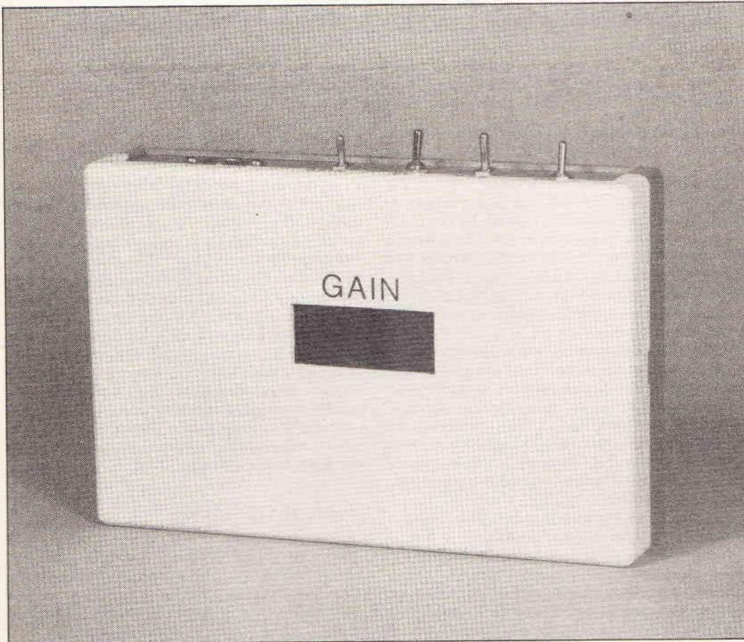
**T**his transistor tester was developed to fulfil the need for a unit that would provide a quick and convenient means of testing DC current gain ( $h_{fe}$ ) and leakage. Some other testers are inexpensive to build but provide only basic go/no-go checking or are relatively slow and difficult to use.
