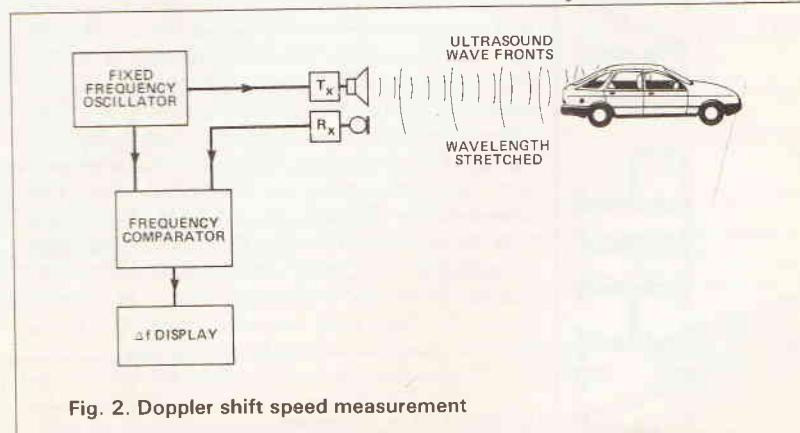
Fig. 2. Doppler shift speed measurement
