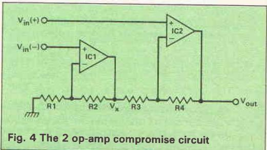
Fig. 4 The 2 op-amp compromise circuit
