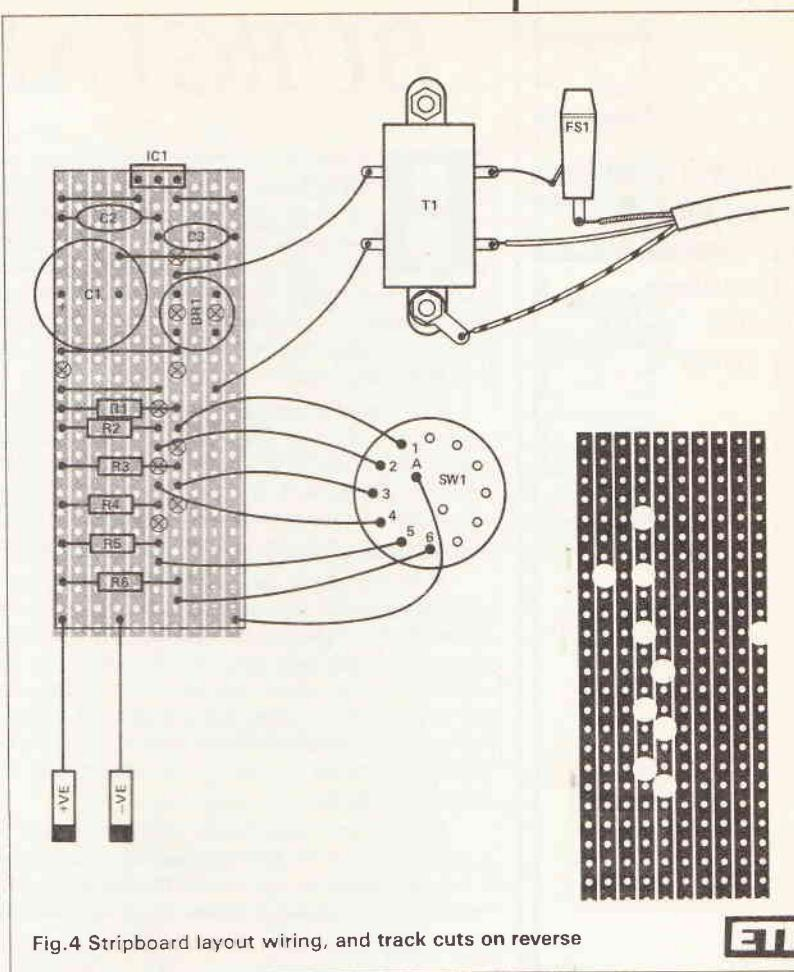
Fig.4 Stripboard layout wiring, and track cuts on reverse
