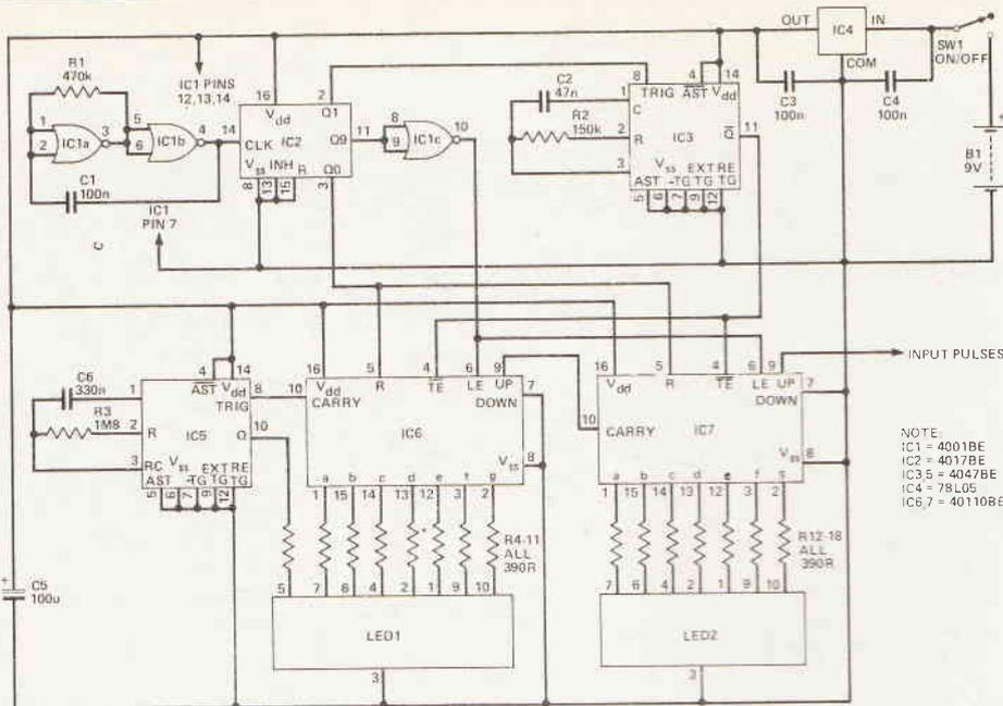
Fig. 3 The circuit diagram of the display section
