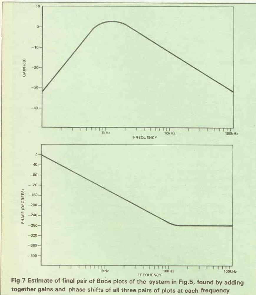
Fig. 7 Estimate of final pair of Bode plots of the system in Fig. 5, found by adding together gains and phase shifts of all three pairs of plots at each frequency
