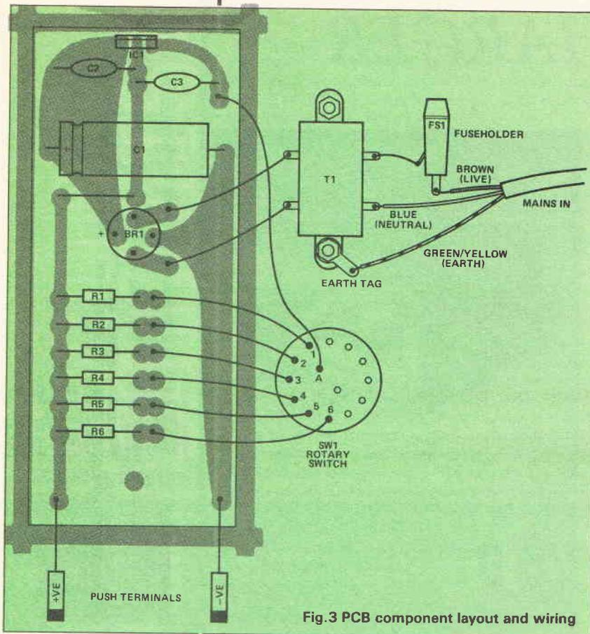
Fig. 3 PCB component layout and wiring
