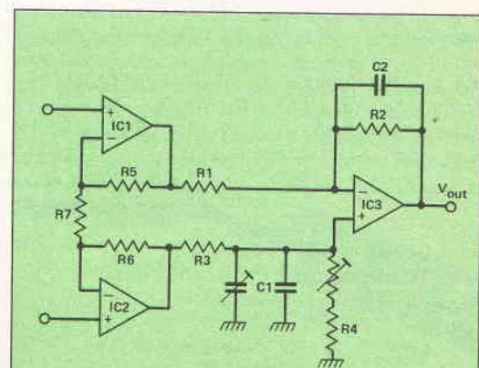
Fig. 3 Additional trimming capacitors for frequency compensation
