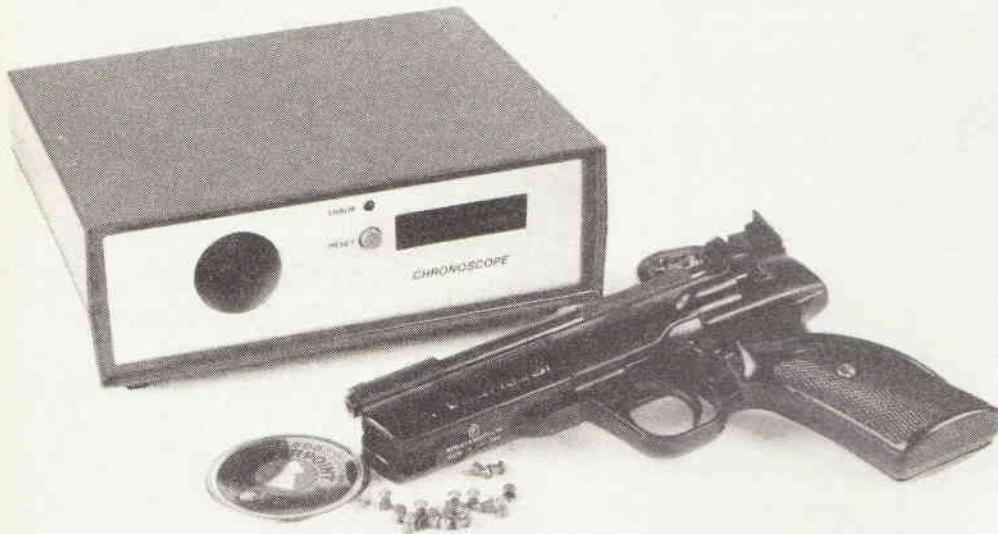
**A** chronoscope is a device for measuring the velocity of an air gun pellet. Those of the shooting fraternity will realise how useful a chronoscope can be, to check the consistency of the gun, monitor its power output and compare how different pellets perform.
