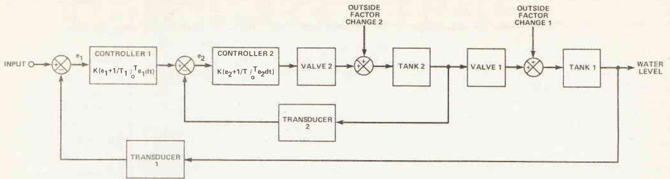
Fig. 10 An example of cascade control, a multi-loop closed-loop control strategy. Disturbances in the inner loop may be greatly reduced by cascade control
