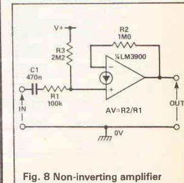
Fig. 8 Non-inverting amplifier
