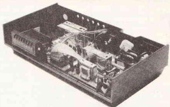
8-way "Preomat" T.V. Tuning of band 1-111 & UHF with AFC, Mains power supply 240V, in cabinet 14 x 7 1/2 x 3 1/2 inches.
