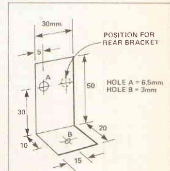
Fig. 8 The bracket to hold the sensor diodes in place (front shown)
