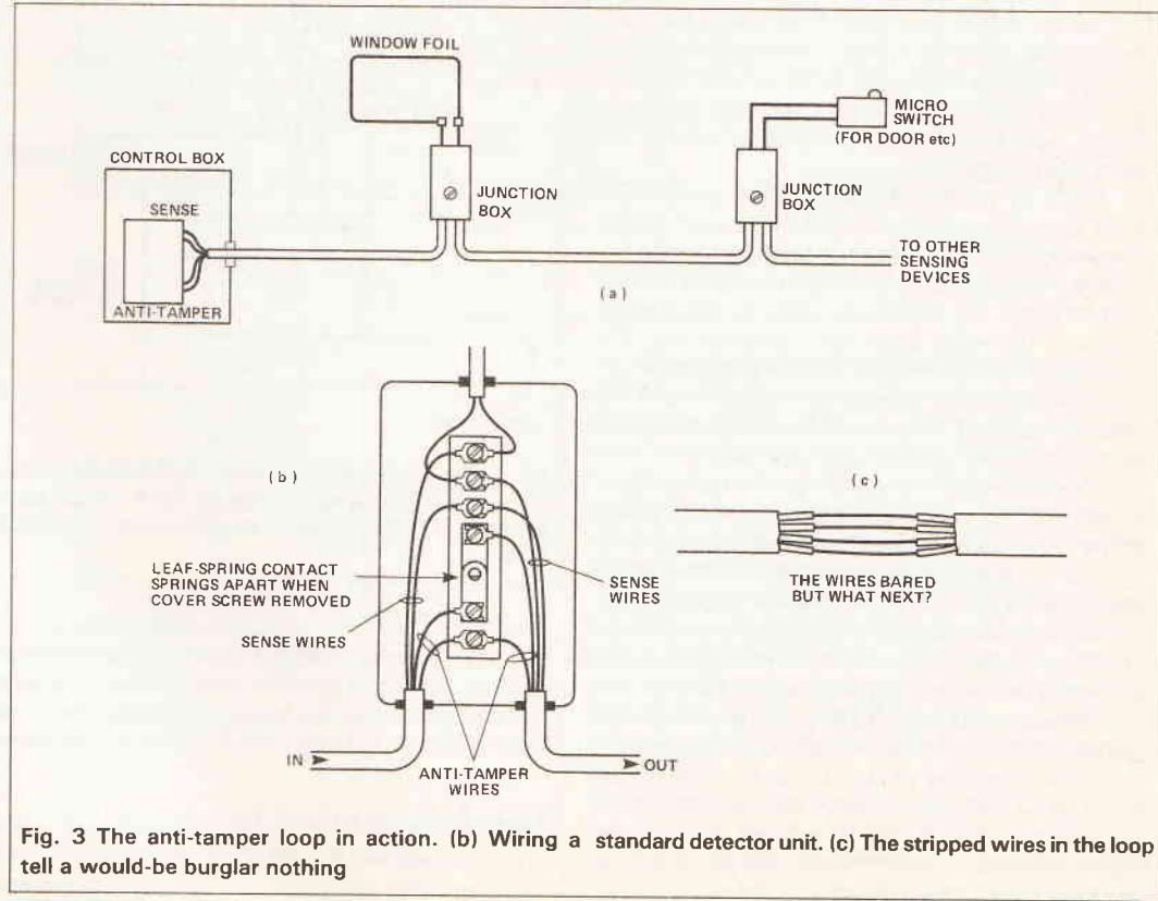
Fig. 3 The anti-tamper loop in action. (b) Wiring a standard detector unit. (c) The stripped wires in the loop tell a would-be burglar nothing
