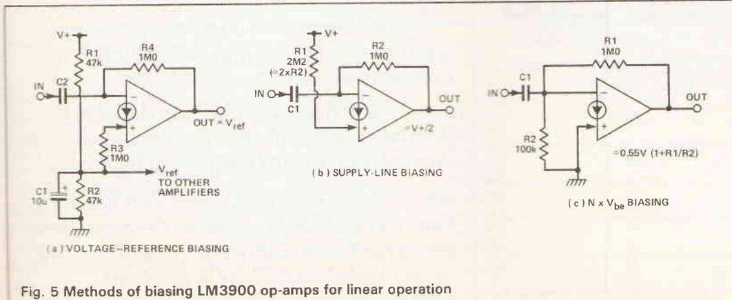
Fig. 5 Methods of biasing LM3900 op-amps for linear operation
