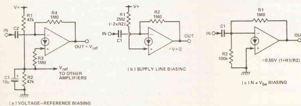
Fig. 5 Methods of biassing LM3900 op-amps for linear operation
