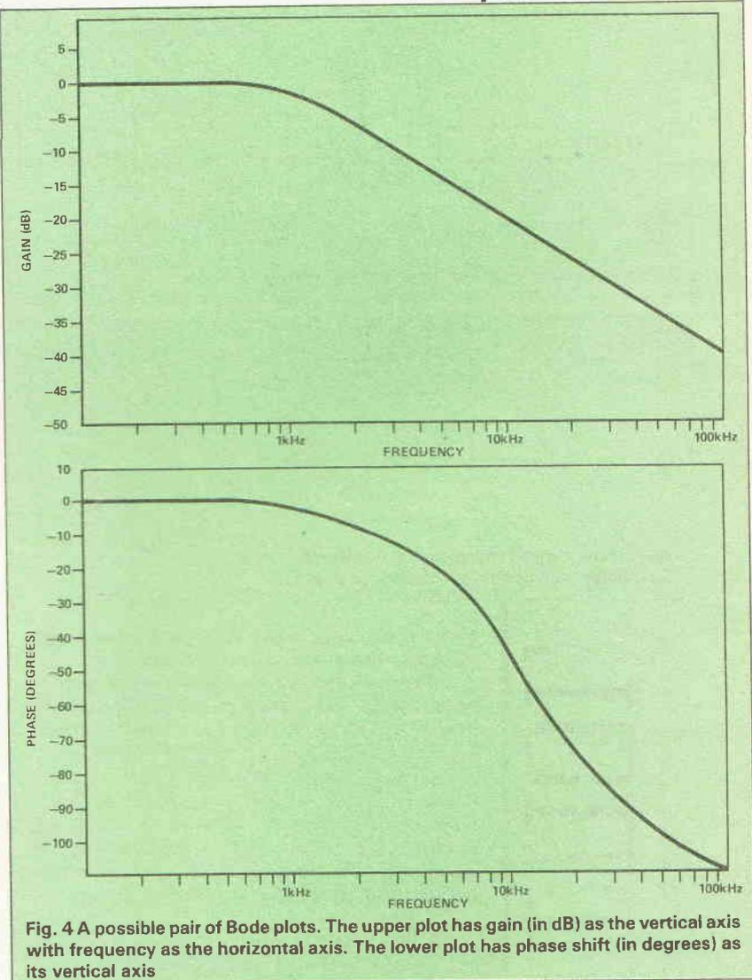
Fig. 4 A possible pair of Bode plots. The upper plot has gain (in dB) as the vertical axis with frequency as the horizontal axis. The lower plot has phase shift (in degrees) as its vertical axis
