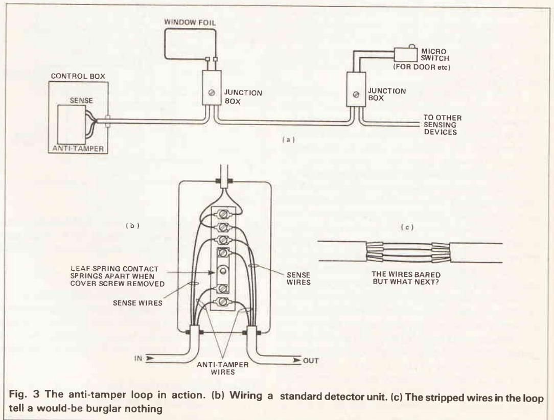
Fig. 3 The anti-tamper loop in action. (b) Wiring a standard detector unit. (c) The stripped wires in the loop tell a would-be burglar nothing
