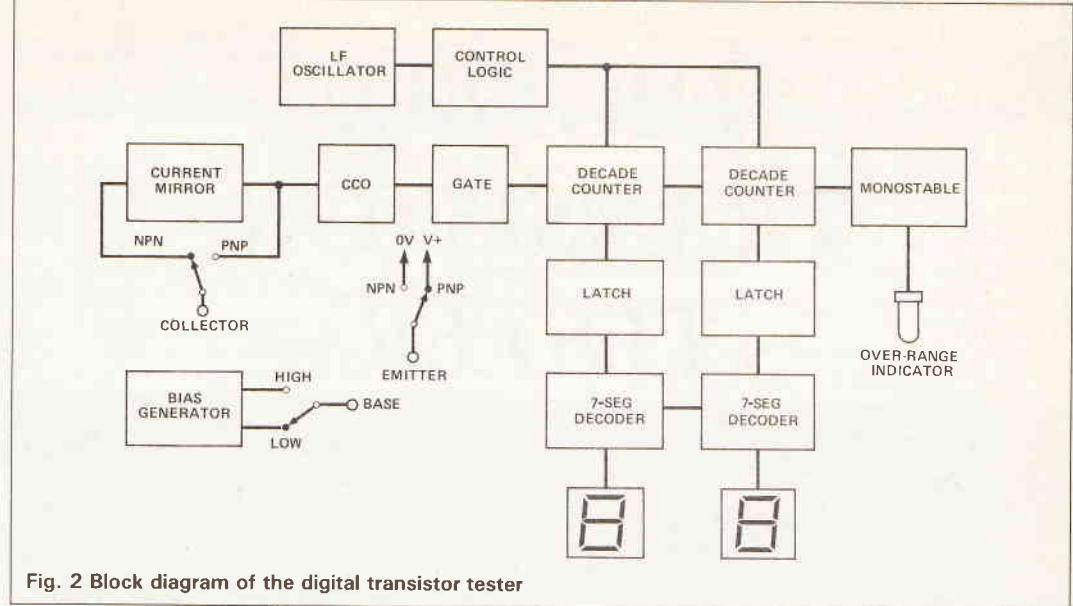
registers the flow of current in the collector circuit. The current flow from the collector to the emitter is normally very low and would typically be about one microamp or less for a silicon device. This is termed the 'leakage' current. Providing a small forward bias current to the base terminal results in a much larger flow of current in the collector circuit. The current gain of the transistor is equal to the collector current divided by the base current.
