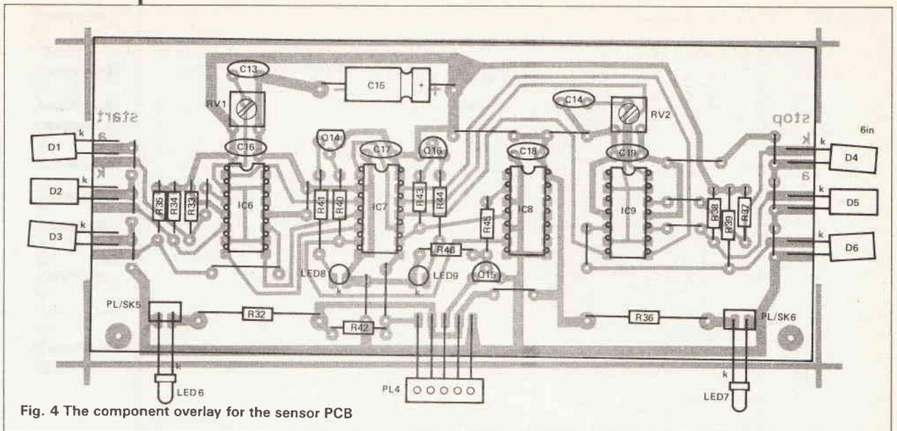
Fig. 4 The component overlay for the sensor PCB
