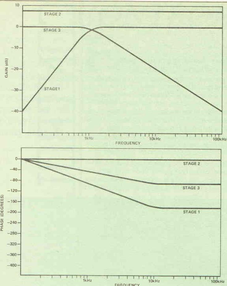
Fig. 6 The Bode plots of the three stages of the system of Fig. 5
