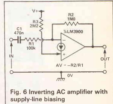
Fig. 6 Inverting AC amplifier with supply-line biassing
