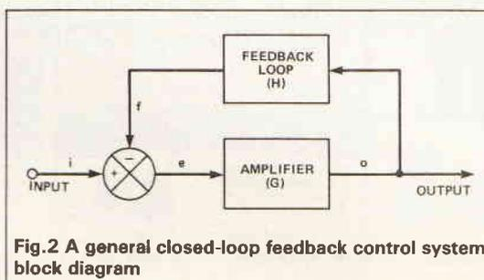
Fig.2 A general closed-loop feedback control system block diagram
