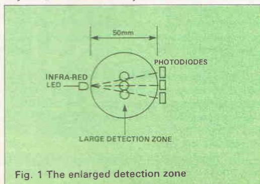
Fig. 1 The enlarged detection zone
