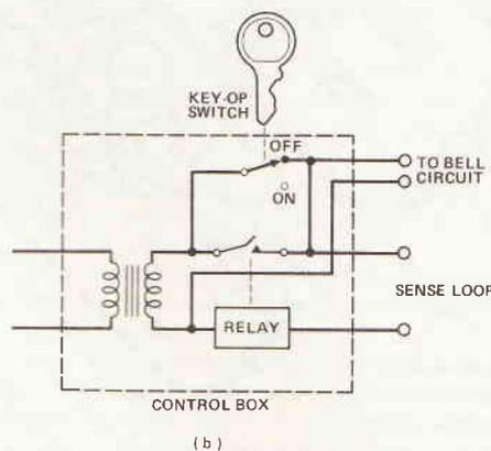
Fig. 1 A typical alarm system. (a) The detection loop. (b) The simplest possible control circuit
