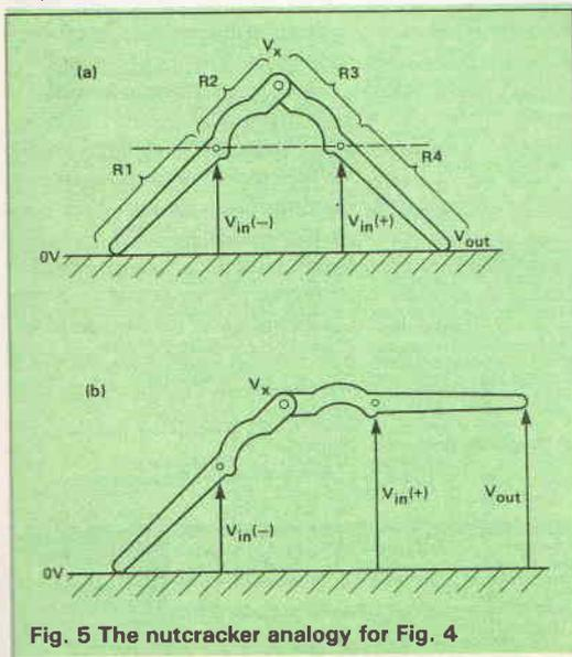
Fig. 5 The nutcracker analogy for Fig. 4
