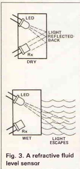
Fig. 3. A refractive fluid level sensor
