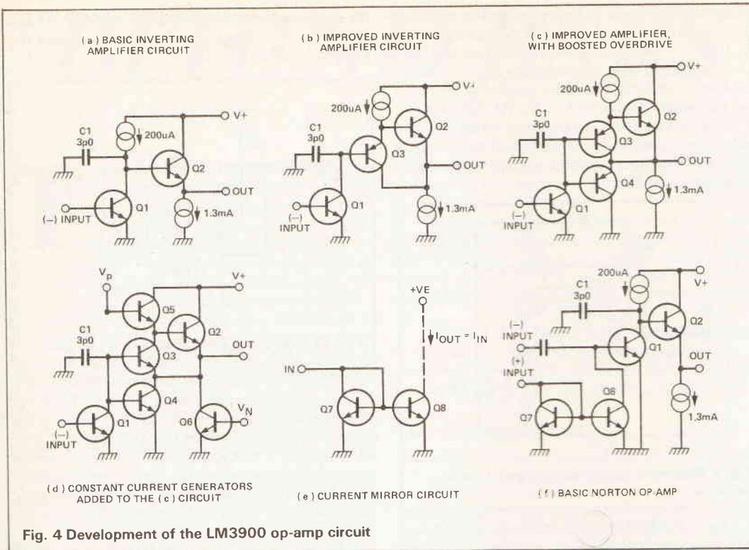
Fig. 4 Development of the LM3900 op-amp circuit
