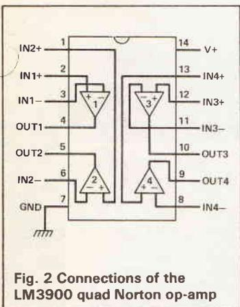
Fig. 2 Connections of the LM3900 quad Norton op-amp
