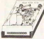
The massive filter section contains thirteen capacitors and two current balanced inductors, together with a bank of six VDRs to remove every last trace of impulsive and RF interference. A ten LED logarithmic display gives a second by second indication of the amount of interference removed. Our approved parts set consists of case, PCB, all components (including high permeability toroidal cores, ICS transformers, class X and Y suppression capacitors, VDRs, etc.) and full instructions.
