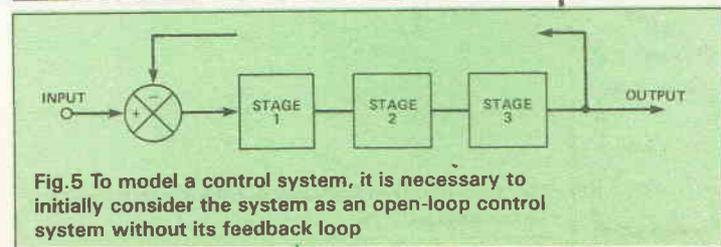
Fig. 5 To model a control system, it is necessary to initially consider the system as an open-loop control system without its feedback loop
