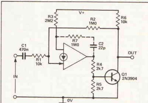
Fig. 9 Wideband (200 kHz) high-gain ( $\times 100$ ) amplifier
