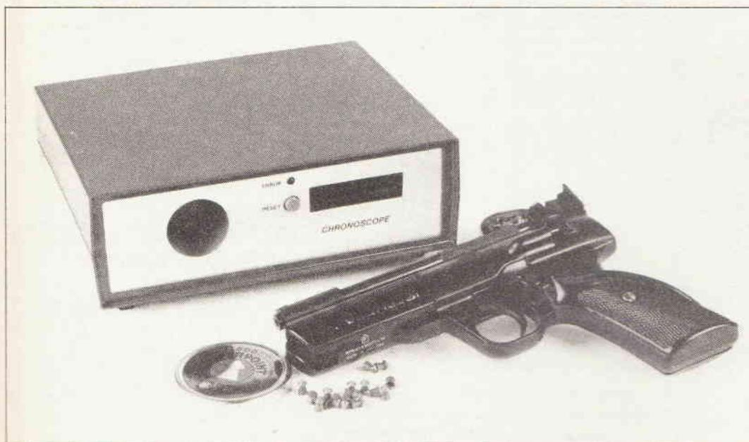
**A** chronoscope is a device for measuring the velocity of an air gun pellet. Those of the shooting fraternity will realise how useful a chronoscope can be, to check the consistency of the gun, monitor its power output and compare how different pellets perform.
