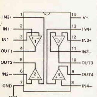
Fig. 2 Connections of the LM3900 quad Norton op-amp
