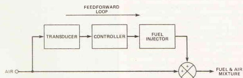
Fig. 12 Ratio control. A specific case of feedback control used to control the ratio of two variables in a control system. The example shown is of an automobile fuel injection system in which the incoming air mass is measured and from this measurement a controller calculates the length of time a fuel injection valve must be opened to present the correct amount of fuel to the combustion cylinder such that exactly the correct ratio of fuel-to-air is sucked into the cylinder
