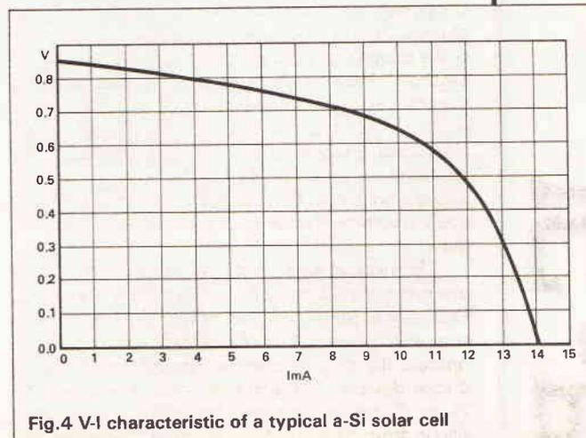
Fig.4 V-I characteristic of a typical a-Si solar cell
