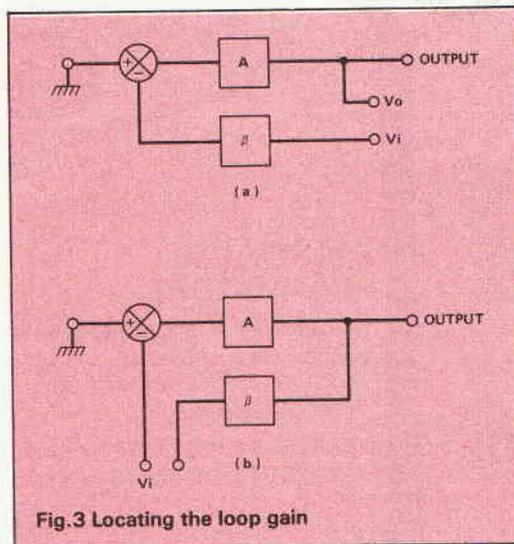
Fig.3 Locating the loop gain
