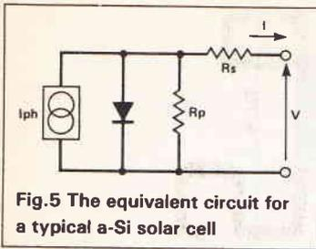
Fig. 5 The equivalent circuit for a typical a-Si solar cell
