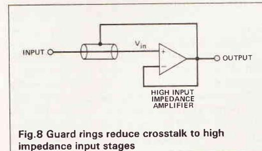
Fig.8 Guard rings reduce crosstalk to high impedance input stages
