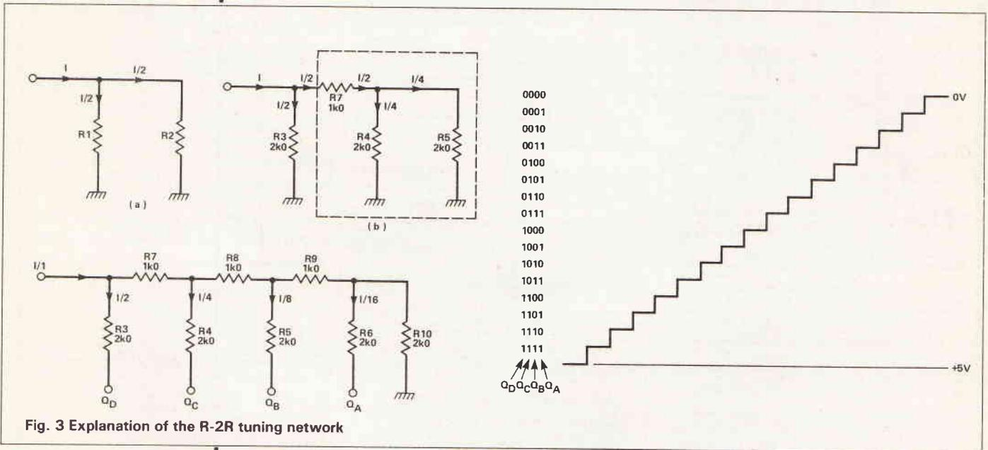
Fig. 3 Explanation of the R-2R tuning network
