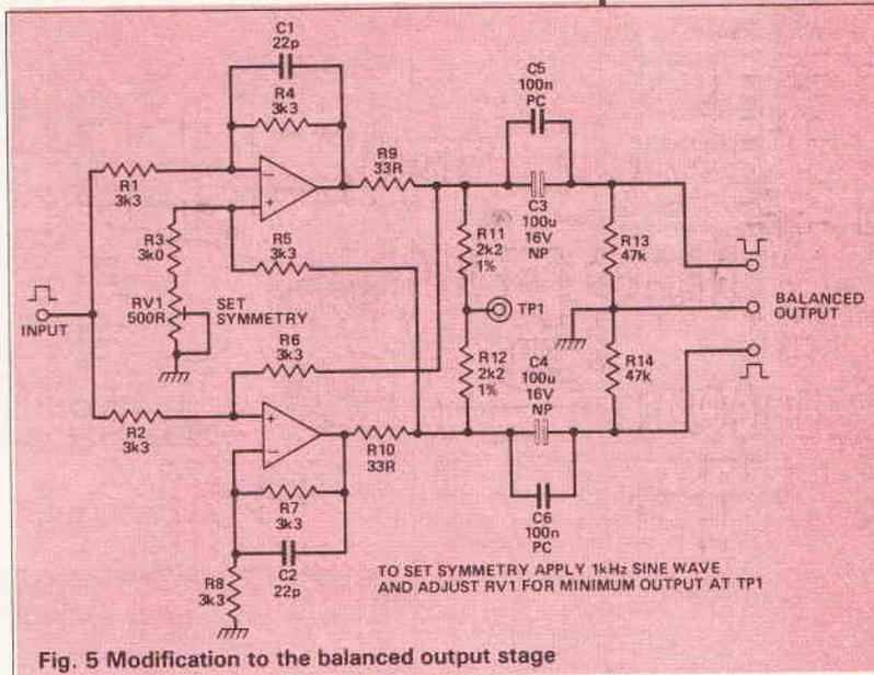
Fig. 5 Modification to the balanced output stage
