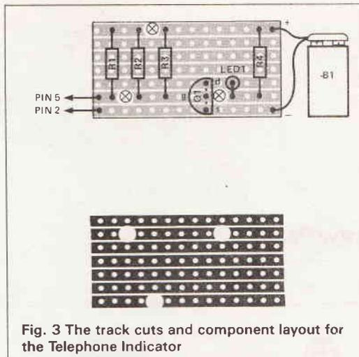
Fig. 3 The track cuts and component layout for the Telephone Indicator
