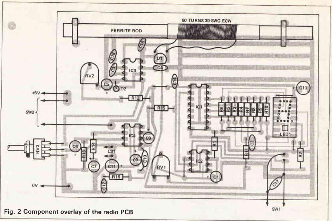
Fig. 2 Component overlay of the radio PCB
