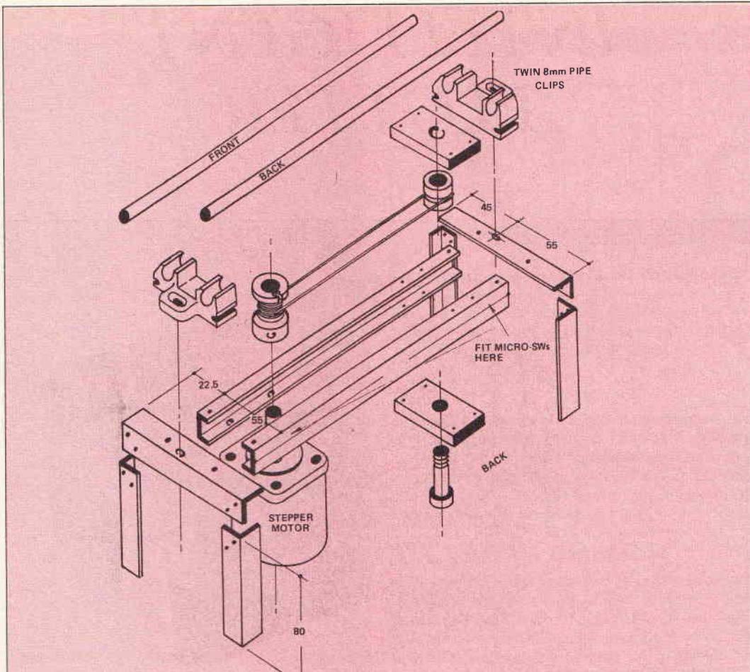
Fig. 1 Details of the x-axis mechanics
