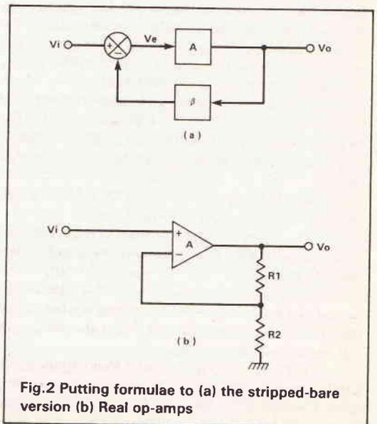
Fig.2 Putting formulae to (a) the stripped-bare version (b) Real op-amps
