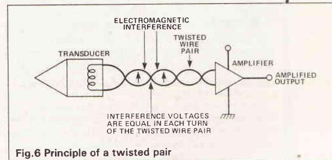
Fig.6 Principle of a twisted pair
