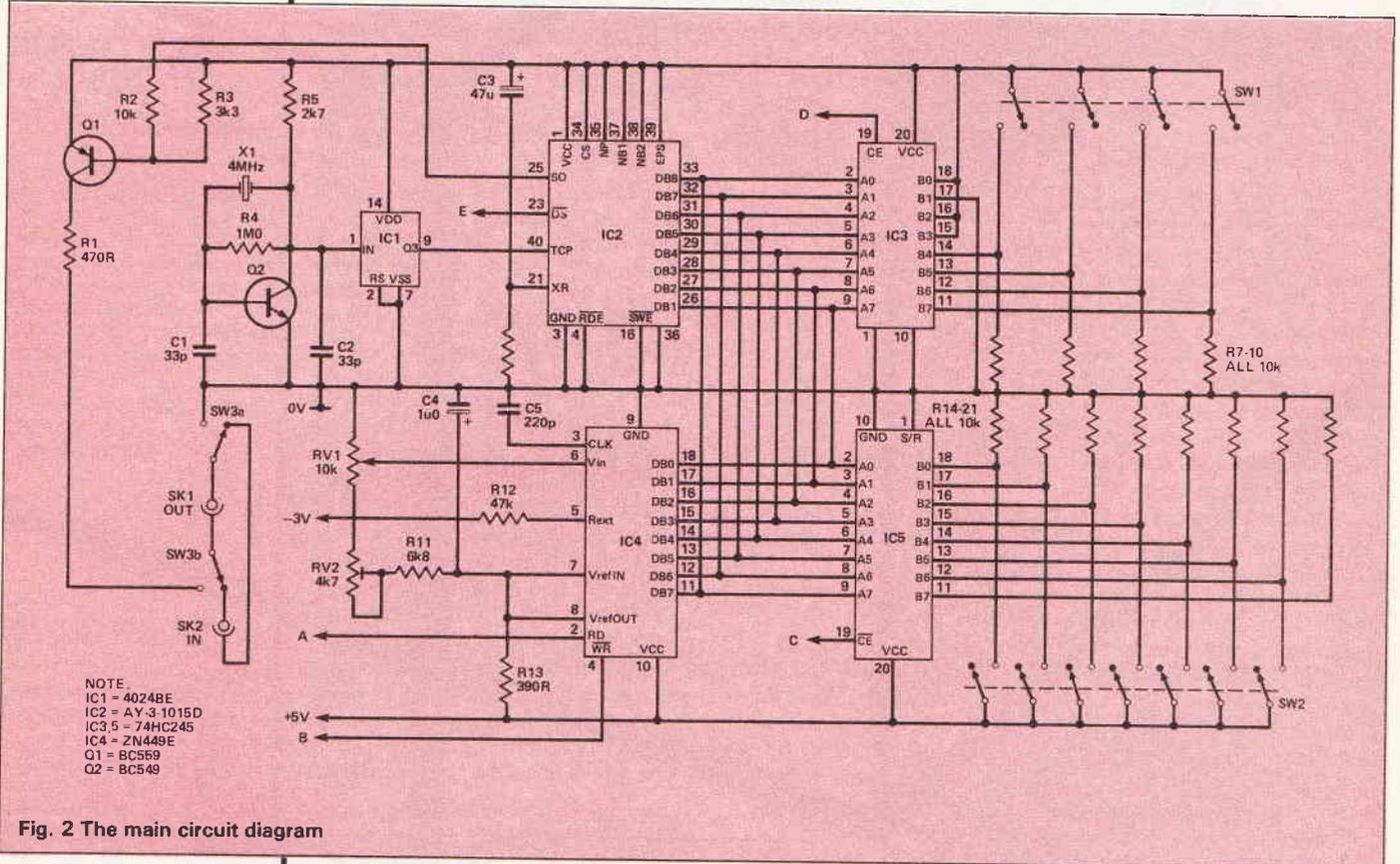
Fig. 2 The main circuit diagram
