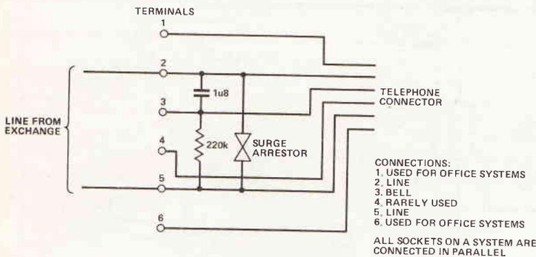
Fig. 1 The connections to a BT master socket
