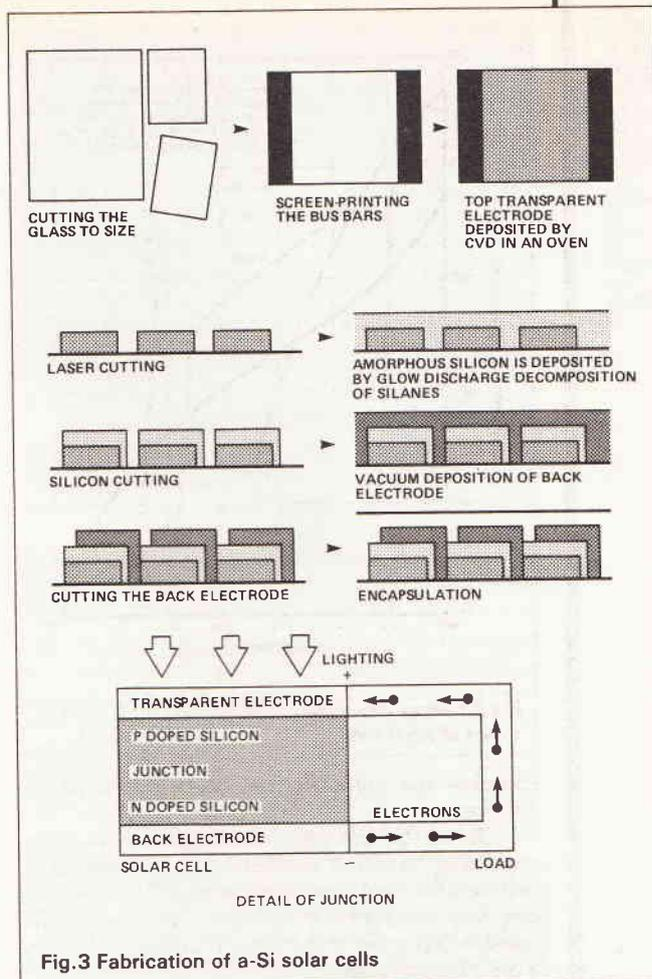
Fig.3 Fabrication of a-Si solar cells
