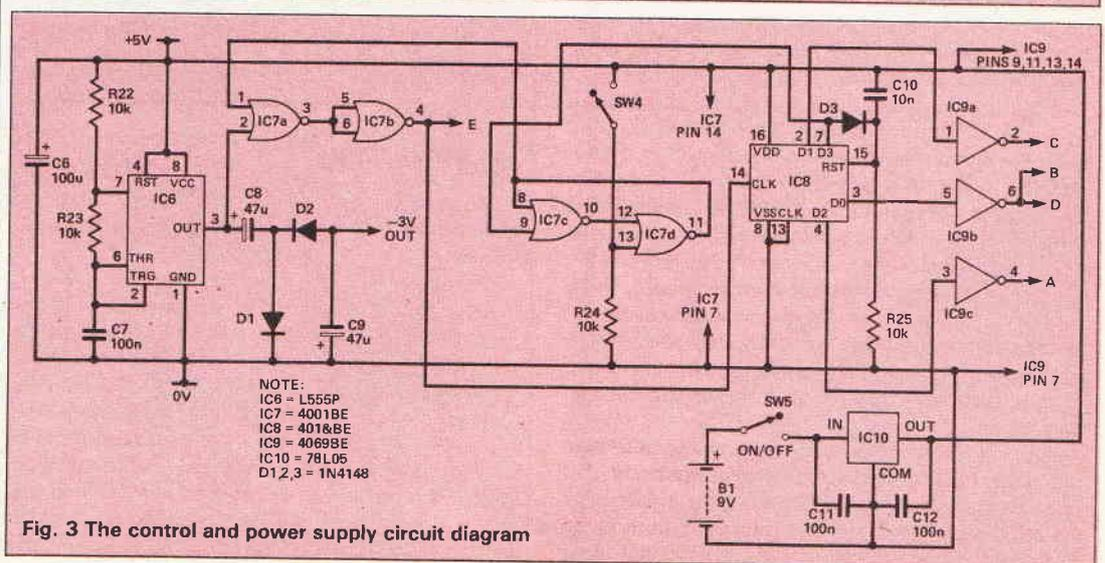
Fig. 3 The control and power supply circuit diagram
