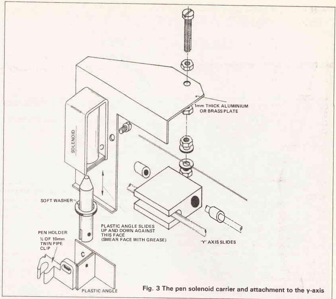
Fig. 3 The pen solenoid carrier and attachment to the y-axis
