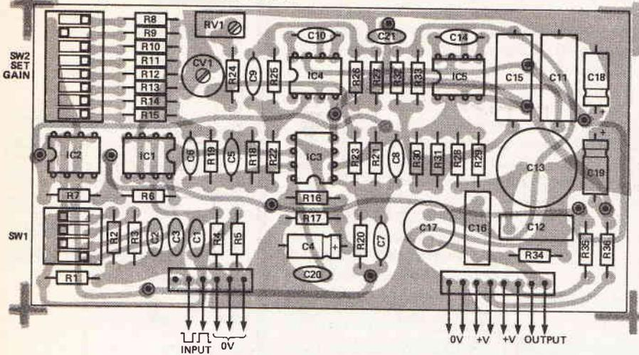
Fig. 3 The component overlay for the updated PCB
