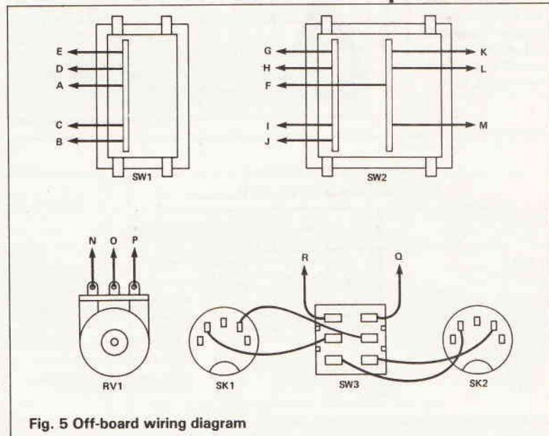
Fig. 5 Off-board wiring diagram
