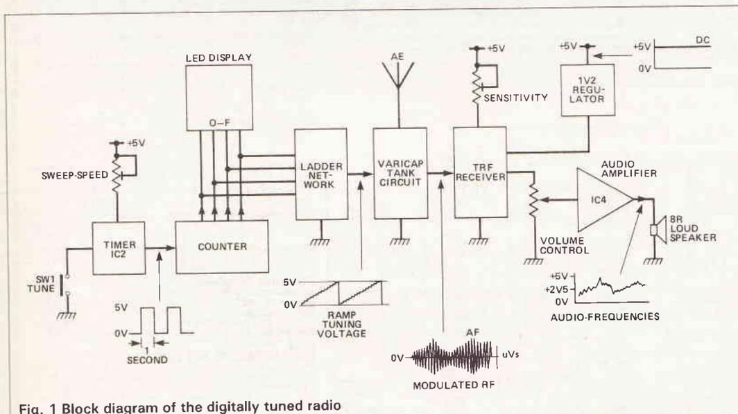
Fig. 1 Block diagram of the digitally tuned radio
