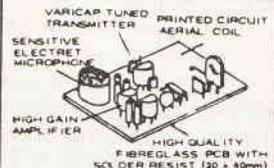
Only 45x25x15mm, including built-in mic. 88-100MHz (standard FM radio). Range approx. 300m depending on terrain. Powered by 9V PP3 (7mA). Ideal for surveillance, baby alarm etc. .... £5.50
