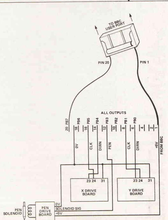
Fig. 7 Connections to a BBC computer
