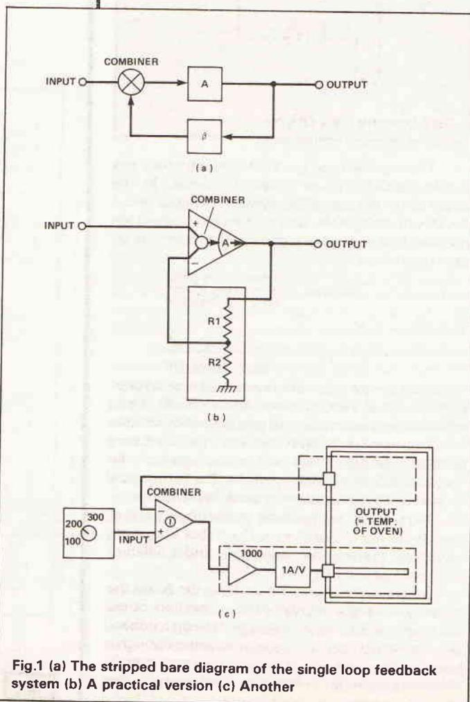
Fig.1 (a) The stripped bare diagram of the single loop feedback system (b) A practical version (c) Another
