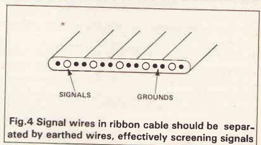
**Fig. 4 Signal wires in ribbon cable should be separated by earthed wires, effectively screening signals**
