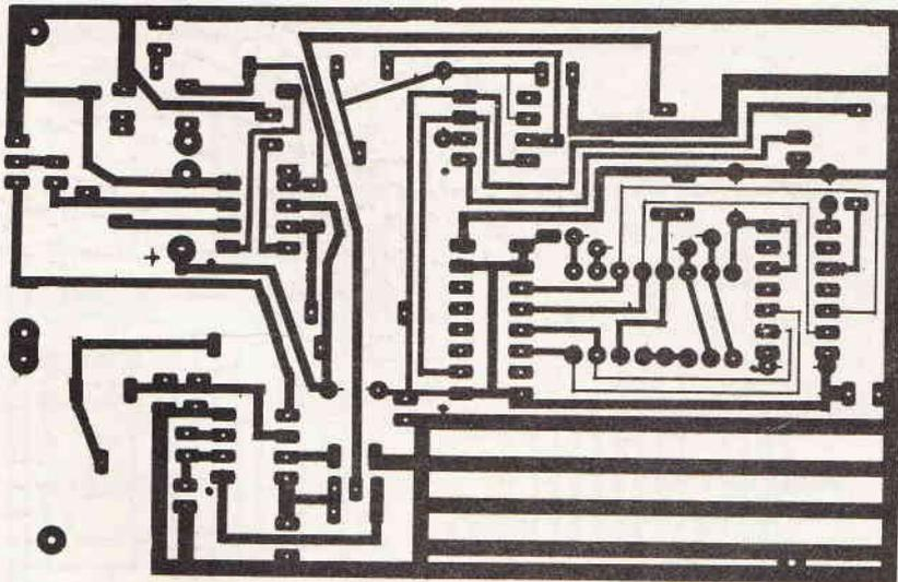
The digitally tuned radio PCB foil
