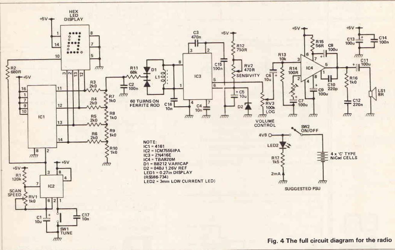
Fig. 4 The full circuit diagram for the radio
