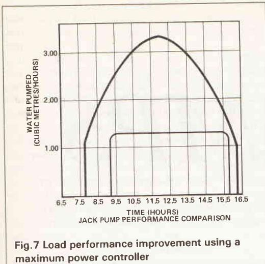
Fig. 7 Load performance improvement using a maximum power controller
