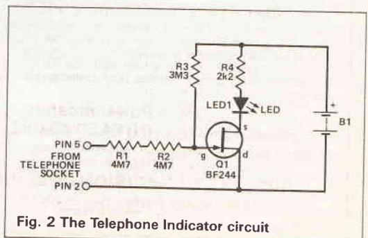
Fig. 2 The Telephone Indicator circuit
