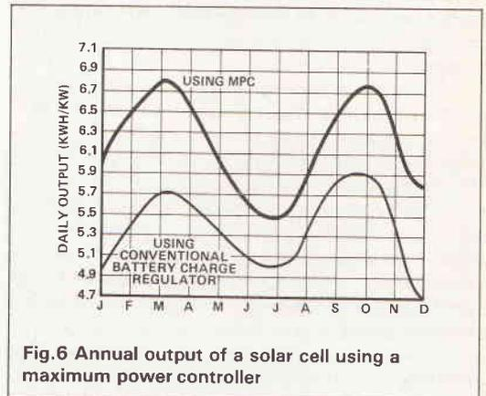
Fig. 6 Annual output of a solar cell using a maximum power controller
