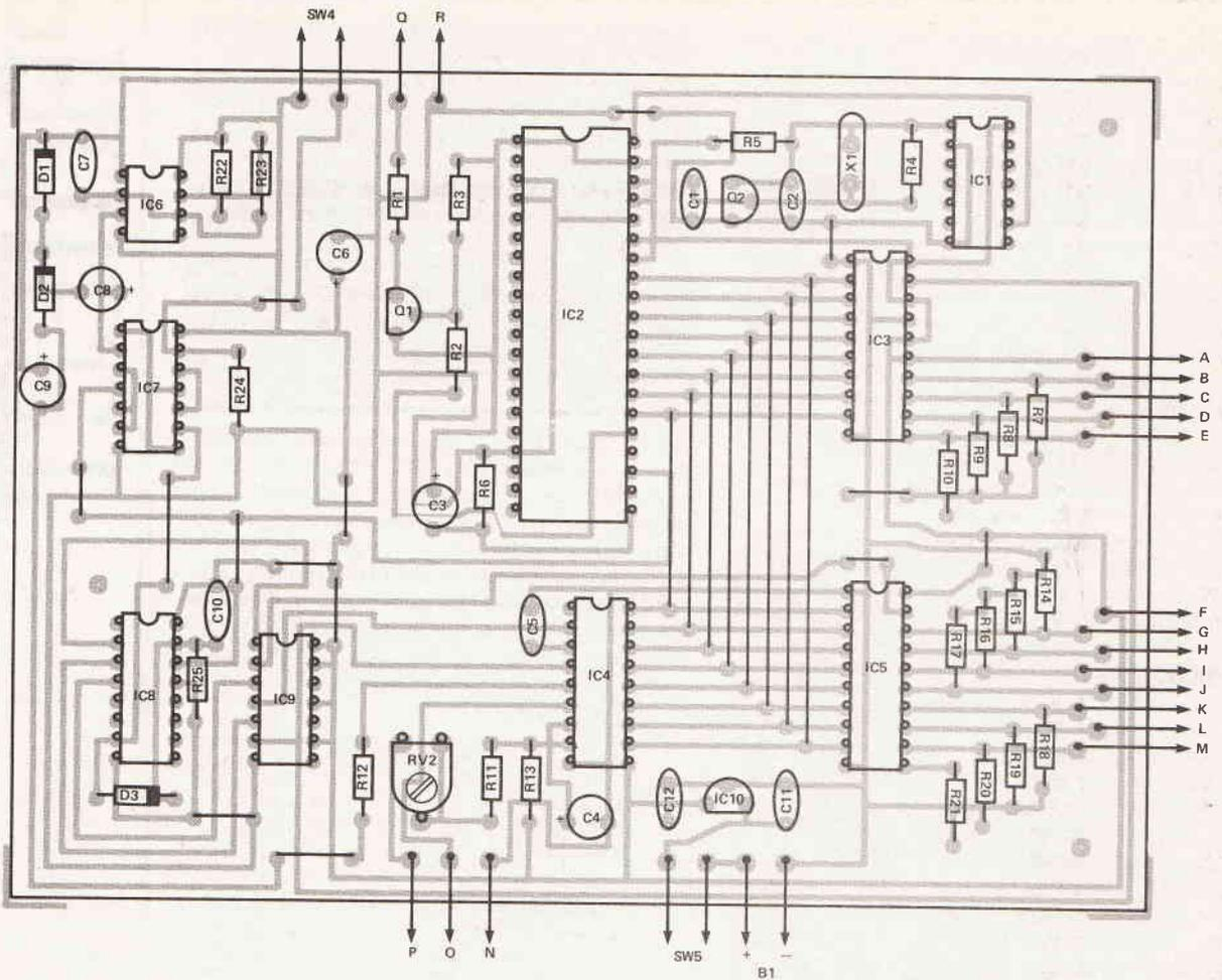
Fig. 4 Component overlay for the MIDI programmer
