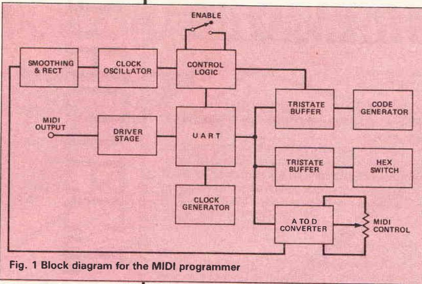
Fig. 1 Block diagram for the MIDI programmer
