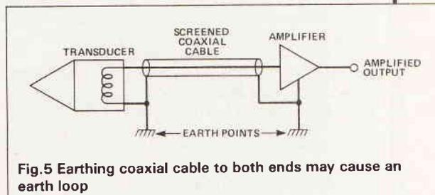
Fig.5 Earthing coaxial cable to both ends may cause an earth loop
