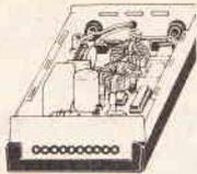
The massive filter section contains thirteen capacitors and two current balanced inductors. Together with a bank of six VDRs, to remove every last trace of impulsive and HF interference. A ten LED logarithmic display gives a second by second indication of the amount of interference removed. Our approved parts set consists of case, PCB, all components (including high permeability ferritic cores, ICs, transistors, class K and Y suppression capacitors, VDRs, etc.) and full instructions.
