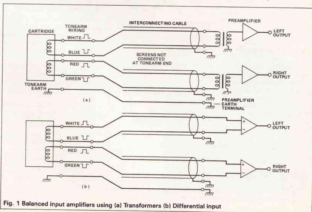
Fig. 1 Balanced input amplifiers using (a) Transformers (b) Differential input
