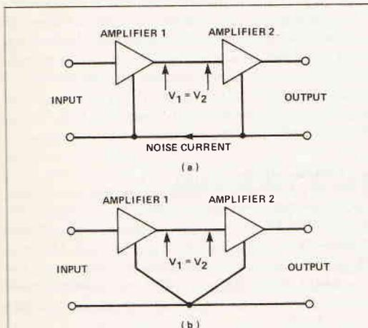
Fig.7 Earth loops can occur at PCB level (a) if separate earth points are used but (b) can be eliminated with a common earth
