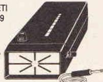
The Q-ion is a hand-held meter which sniffs out ions in the air. It can tell the good ones from the dusts if you're thinking of buying a commercial ioniser, check the efficiency and output of one you've made yourself.
