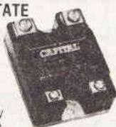
Zero voltage switching - no radio interference. 2.5KV input to output isolation. 4 KV terminals to heatsink. 3V to 32V input voltage easily interfaced to TTL or CMOS logic. 24V to 240V rms load voltage. Inductive load switching. Built-in snubber network. 10A max. 4A with no heatsink at 40°C.
