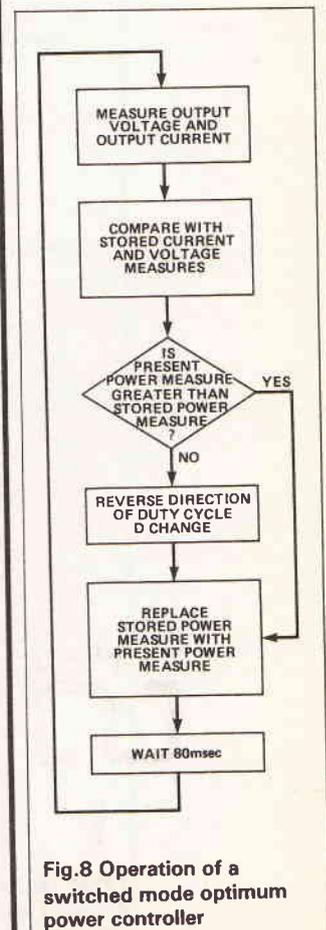
Fig. 8 Operation of a switched mode optimum power controller
