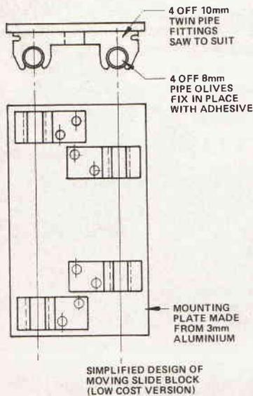
Fig. 5 Simplified low-cost moving slide block design
