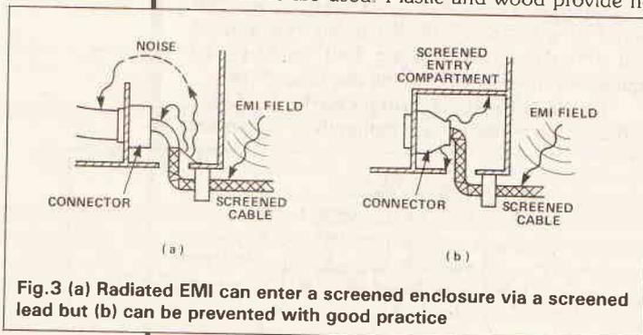
**Fig. 3 (a) Radiated EMI can enter a screened enclosure via a screened lead but (b) can be prevented with good practice**
