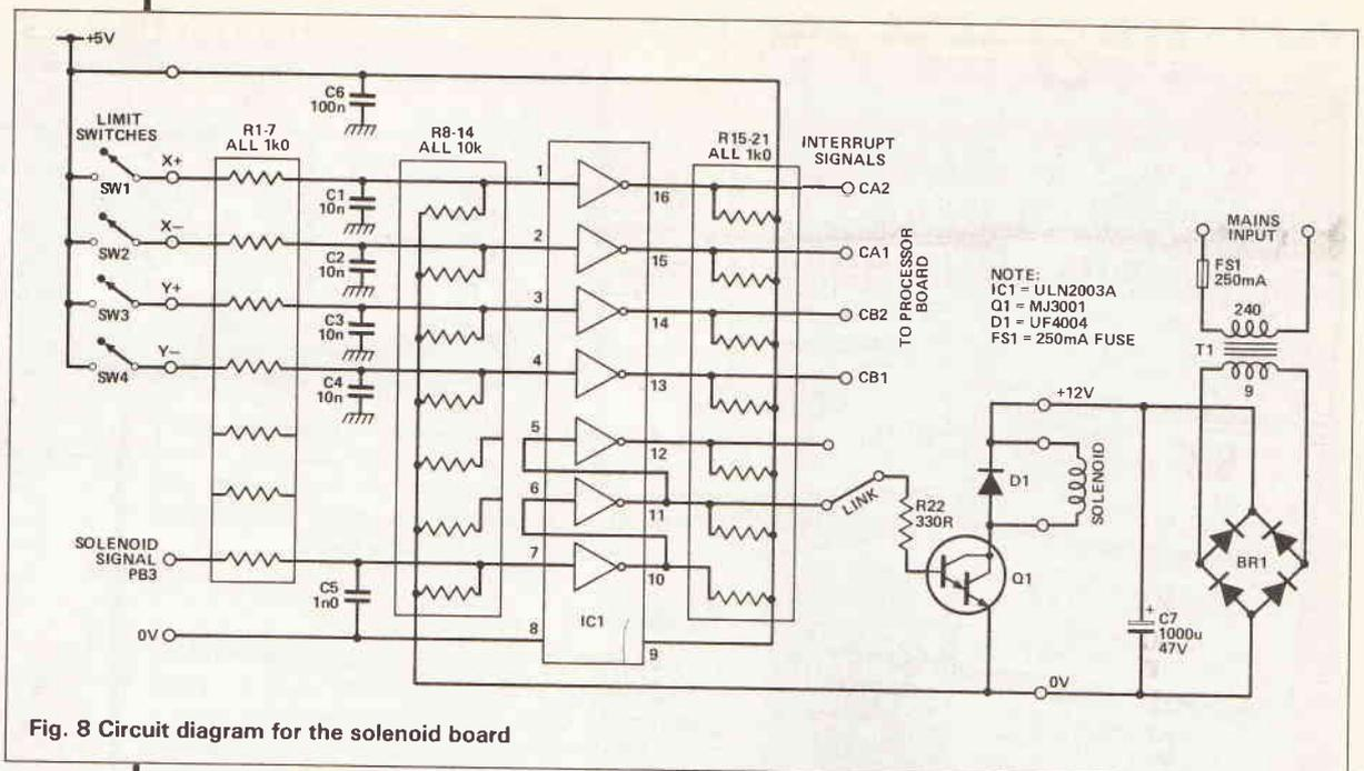
Fig. 8 Circuit diagram for the solenoid board
