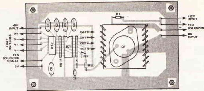
Fig. 6 Component overlay for the solenoid board
