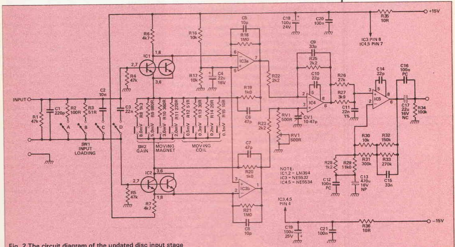
Fig. 2 The circuit diagram of the updated disc input stage
