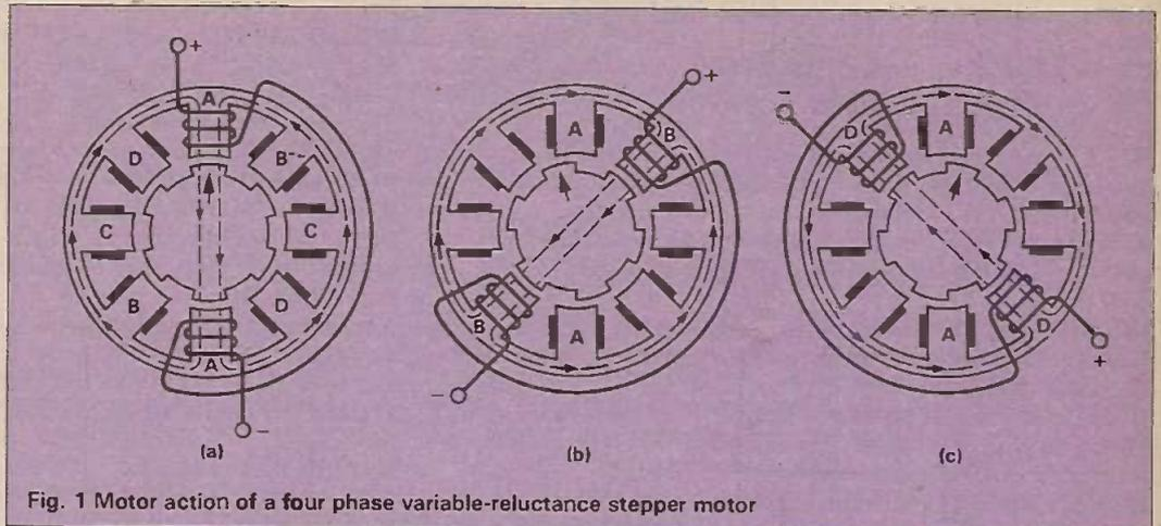
Fig. 1 Motor action of a four phase variable-reluctance stepper motor
