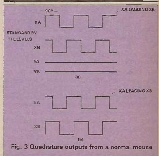
Fig. 3 Quadrature outputs from a normal mouse
