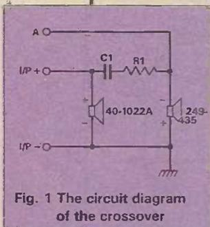
Fig. 1 The circuit diagram of the crossover
