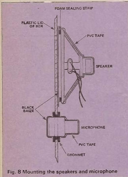
Fig. 8 Mounting the speakers and microphone
