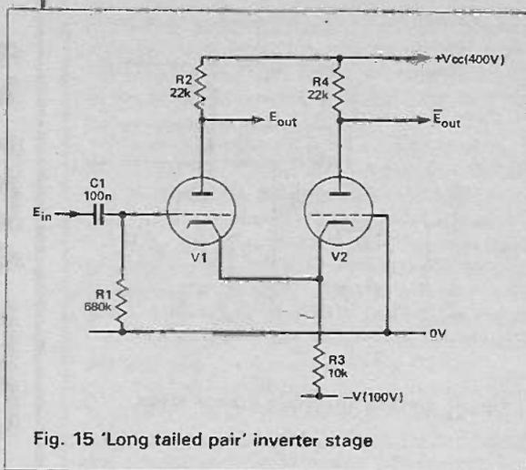
Fig. 15 'Long tailed pair' inverter stage
