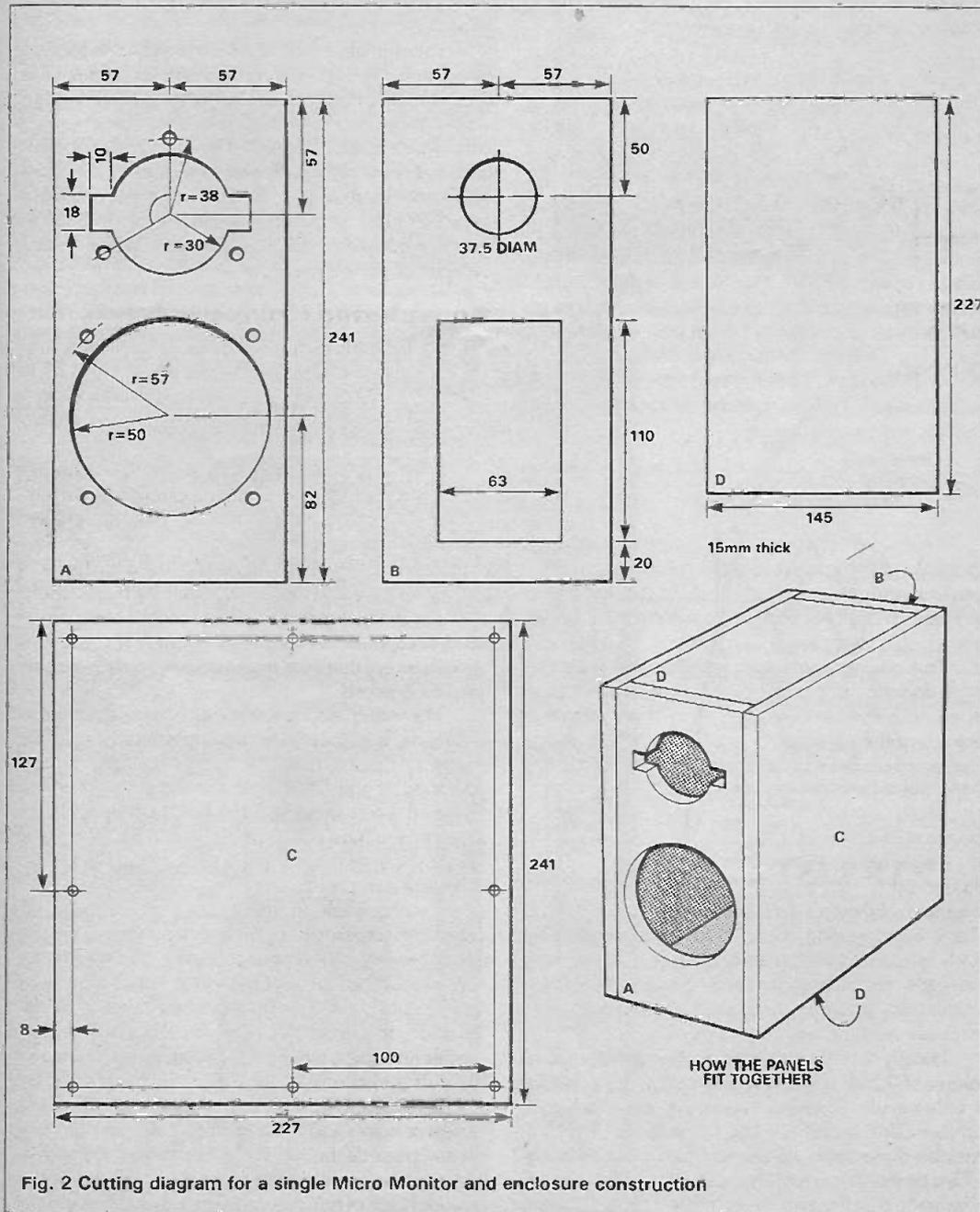
Fig. 2 Cutting diagram for a single Micro Monitor and enclosure construction
