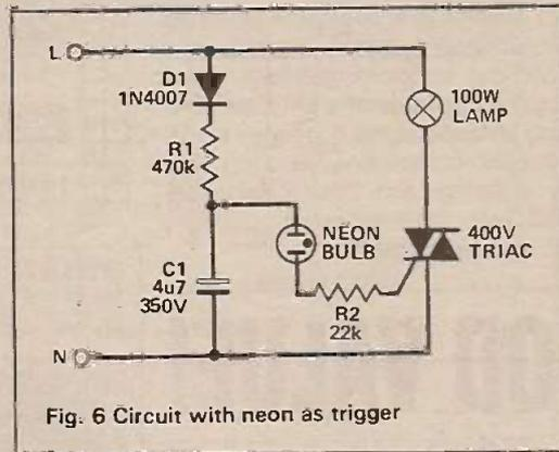
Fig. 6 Circuit with neon as trigger
