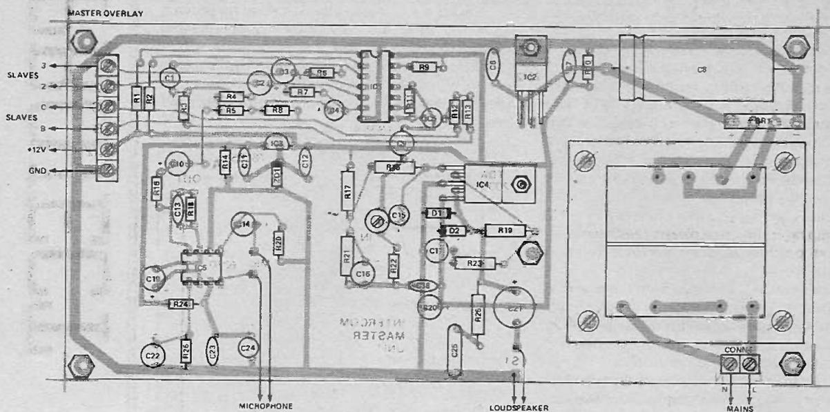
Fig. 6 Component overlay for the master station
