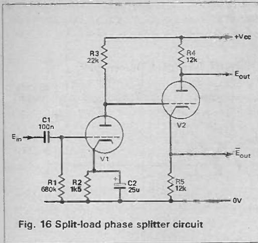
Fig. 16 Split-load phase splitter circuit
