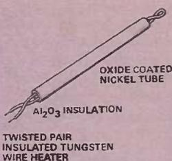
Fig. 1-Cathode structure of an indirectly heated valve
