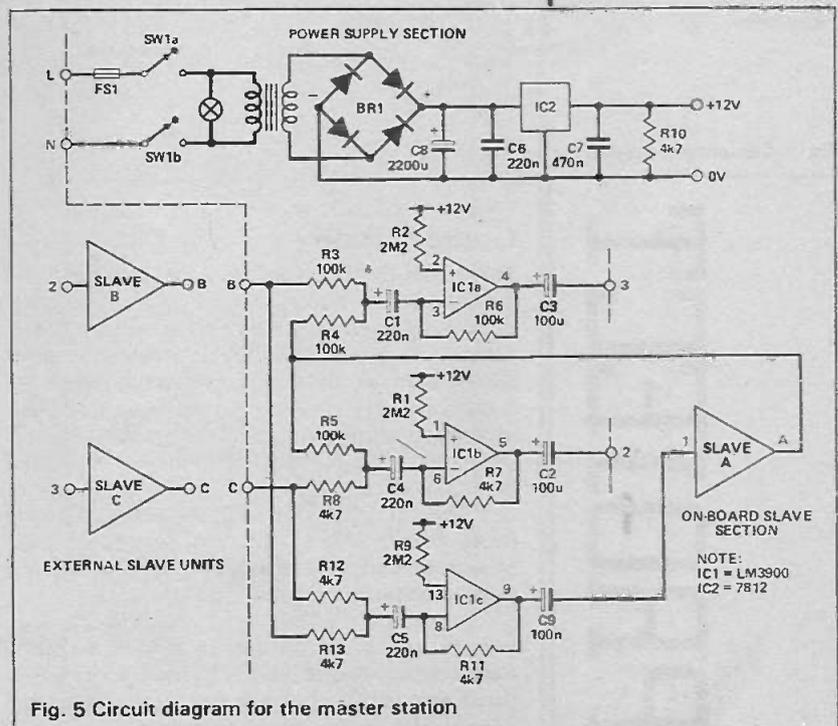
Fig. 5 Circuit diagram for the master station
