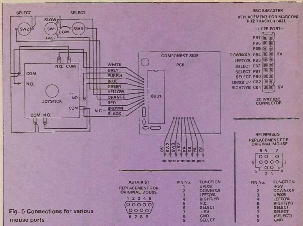
Fig. 5 Connections for various mouse ports
