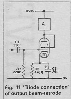
Fig. 11 'Triode connection' of output beam-tetrode
