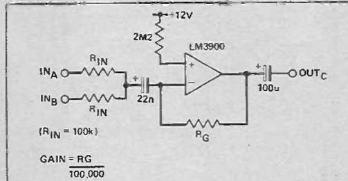
Fig. 4 Signal mixer using LM3900 Norton op-amp
