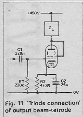
Fig. 11 'Triode connection' of output beam-tetrode
