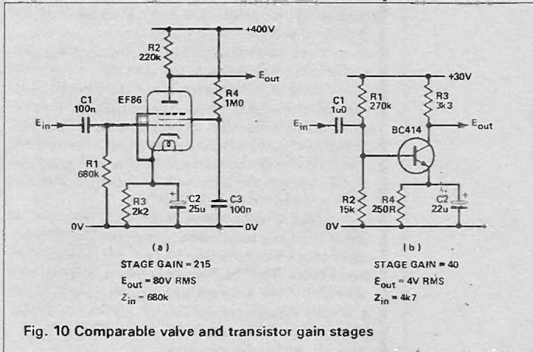
Fig. 10 Comparable valve and transistor gain stages
