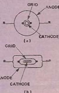
Fig. 3 Comparative structures of triode valves (a) high gain (b) low gain
