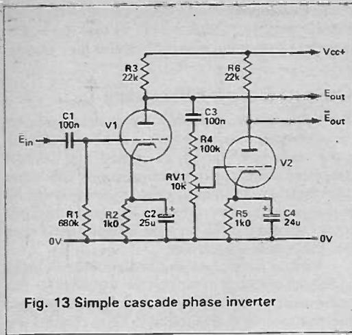
Fig. 13 Simple cascade phase inverter
