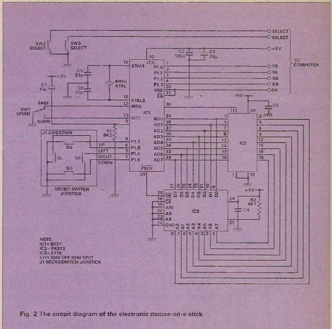
Fig. 2 The circuit diagram of the electronic mouse-on-a-stick
