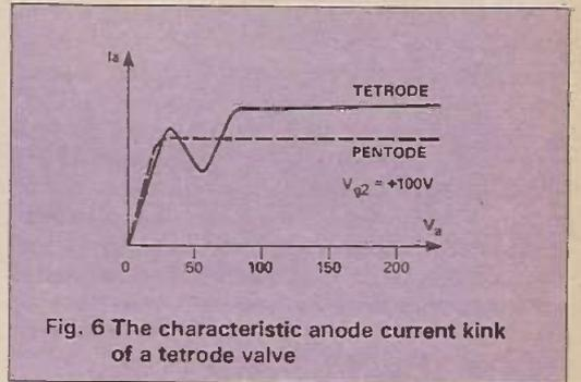
Fig. 6 The characteristic anode current kink of a tetrode valve
