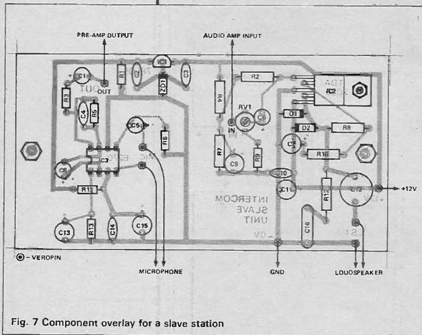
Fig. 7 Component overlay for a slave station
