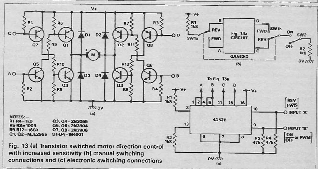
Fig. 13 (a) Transistor switched motor direction control with increased sensitivity (b) manual switching connections and (c) electronic switching connections
