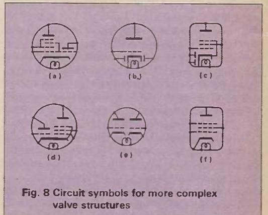
Fig. 8 Circuit symbols for more complex valve structures
