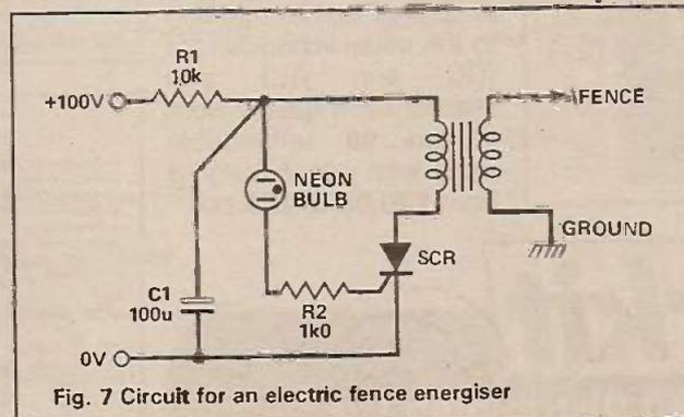
Fig. 7 Circuit for an electric fence energiser
