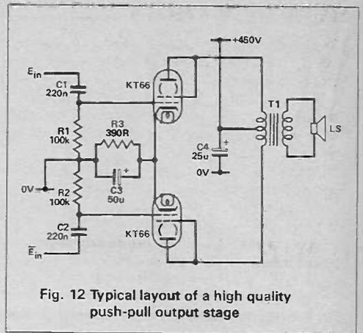
Fig. 12 Typical layout of a high quality push-pull output stage
