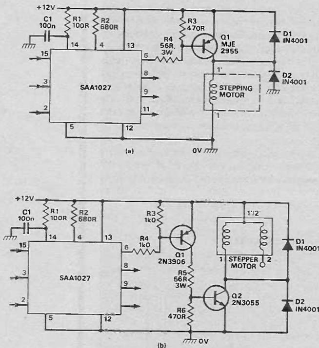
Fig. 8 Two circuits to boost the drive current (a) using independent phase windings and (b) coupled phase windings
