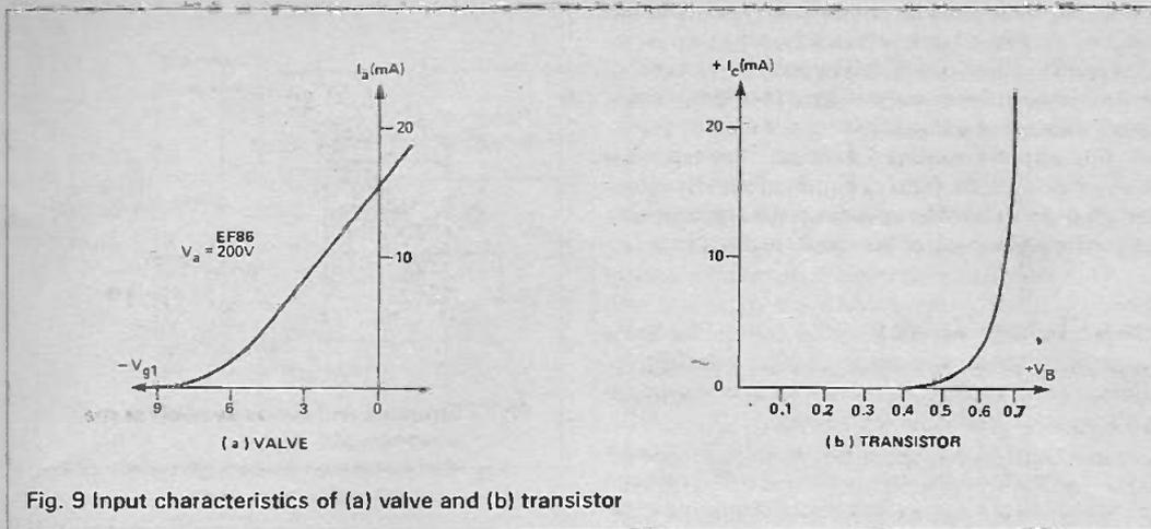
Fig. 9 Input characteristics of (a) valve and (b) transistor
