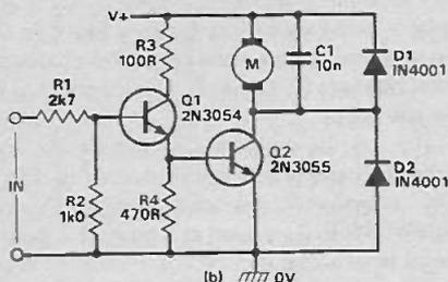
Fig. 10 On/off motor control using transistor switching and (b) increased sensitivity
