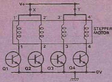
Fig. 3 Basic transistor driven stepper motor circuit
