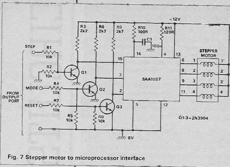
Fig. 7 Stepper motor to microprocessor interface
