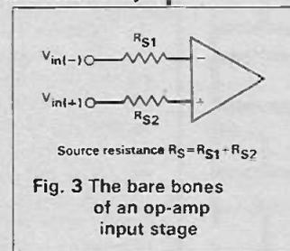
Fig. 3 The bare bones of an op-amp input stage
