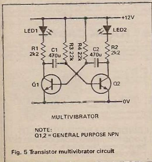
Fig. 5 Transistor multivibrator circuit
