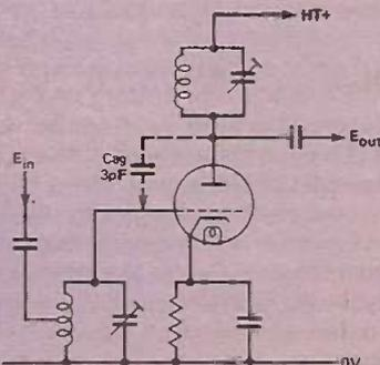
Fig. 4 HF amplifying stage
