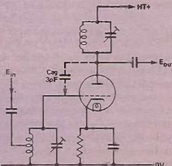
Fig. 4 HF amplifying stage
