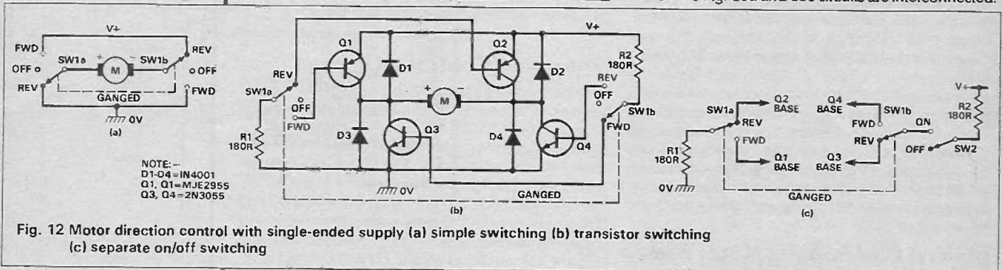
Fig. 12 Motor direction control with single-ended supply (a) simple switching (b) transistor switching (c) separate on/off switching
