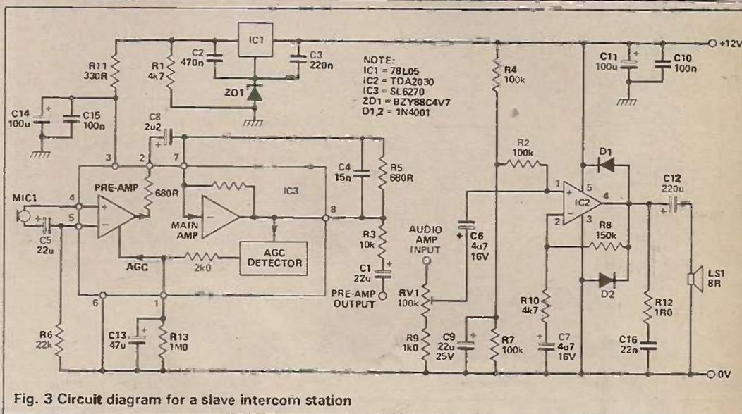
Fig. 3 Circuit diagram for a slave intercom station
