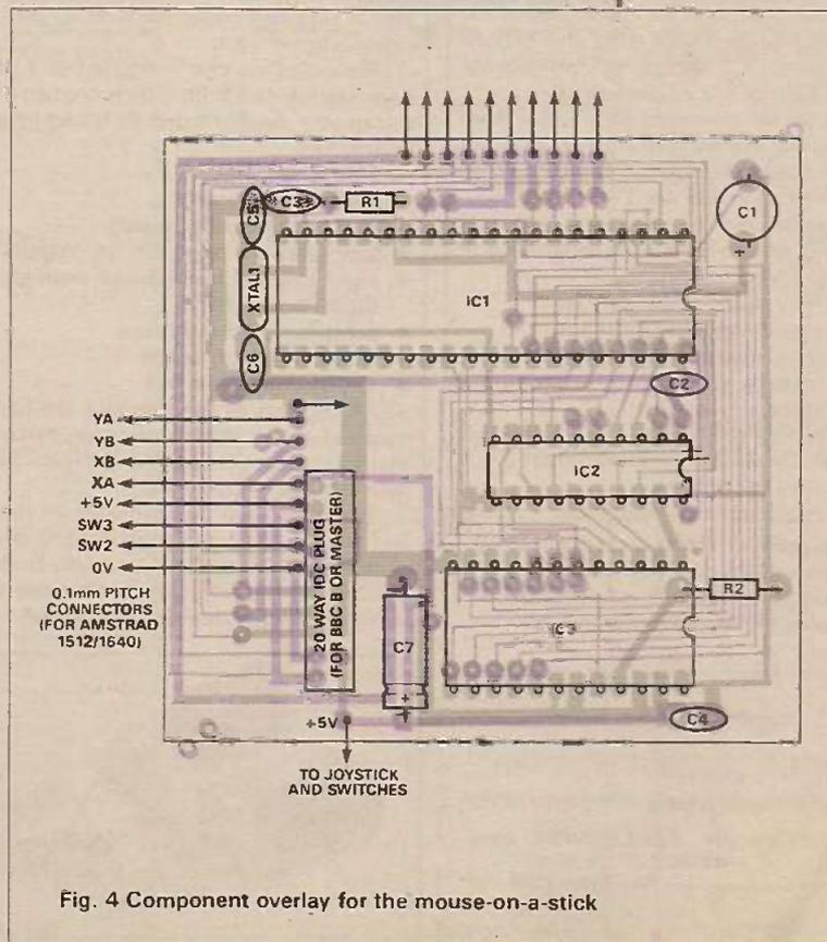
Fig. 4 Component overlay for the mouse-on-a-stick
