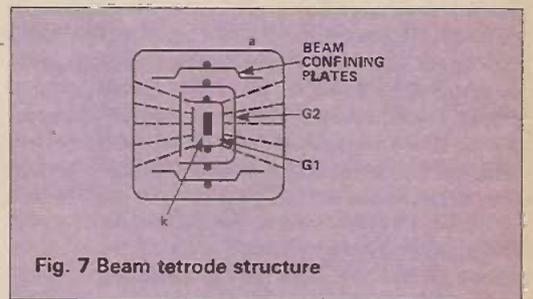
Fig. 7 Beam tetrode structure
