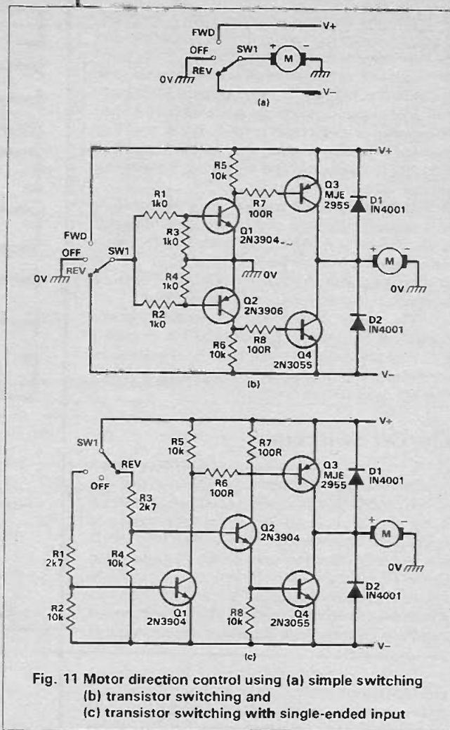
Fig. 11 Motor direction control using (a) simple switching (b) transistor switching and (c) transistor switching with single-ended input
