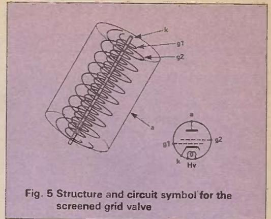
Fig. 5 Structure and circuit symbol for the screened grid valve
