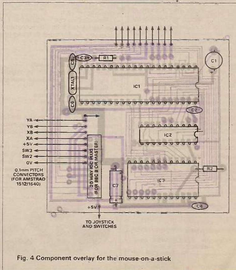
Fig. 4 Component overlay for the mouse-on-a-stick
