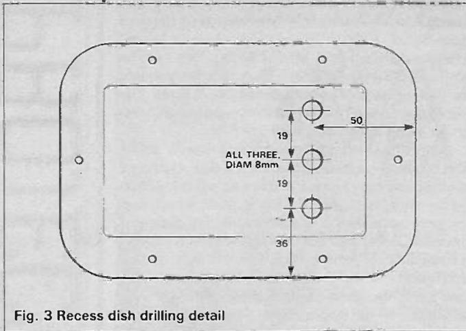
Fig. 3 Recess dish drilling detail
