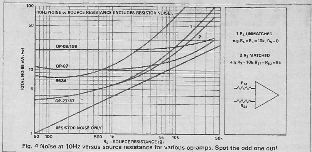
Fig. 4 Noise at 10Hz versus source resistance for various op-amps. Spot the odd one out!
