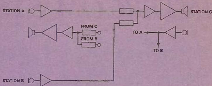
Fig. 2 Block system for three or more stations
