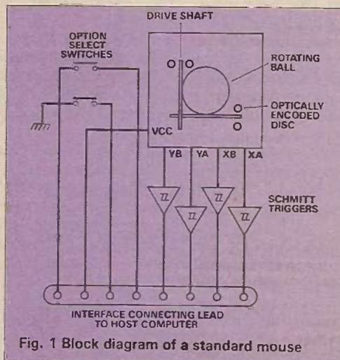
Fig. 1 Block diagram of a standard mouse
