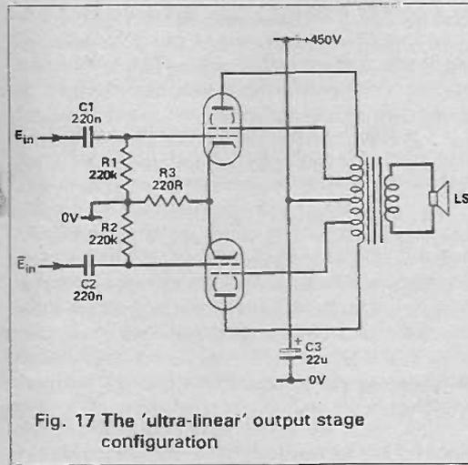
Fig. 17 The 'ultra-linear' output stage configuration
