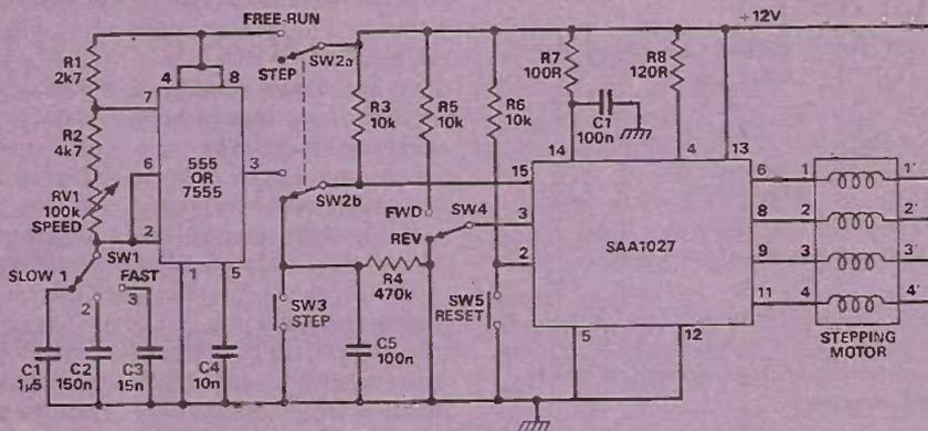
Fig. 6 Complete stepper motor drive and test circuit
