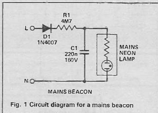
The circuit is shown in Fig. 1. On positive half-cycles of the mains, C1 charges up via D1 and R1. Eventually the voltage across C1 will be high enough for the neon to strike and glow. The current taken by the neon discharges C1 until the voltage is too low for the neon to continue glowing. It turns off, C1 begins to charge and the cycle repeats for ever more.
