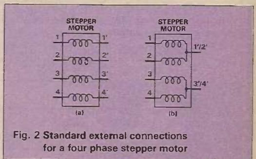
Fig. 2 Standard external connections for a four phase stepper motor
