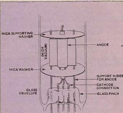
Fig. 2 Mechanical construction of a rectifier diode
