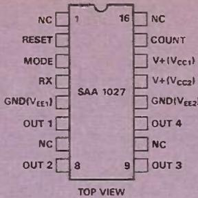
Fig. 4 Outline and pin designations of the SAA1027 stepper driver IC
