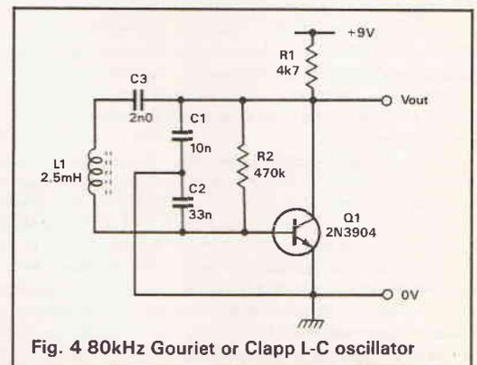
Fig. 4 80kHz Gouriet or Clapp L-C oscillator
