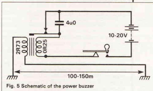
were instructed to periodically reverse the battery connections to ensure uniform wear of the make and break contacts.
