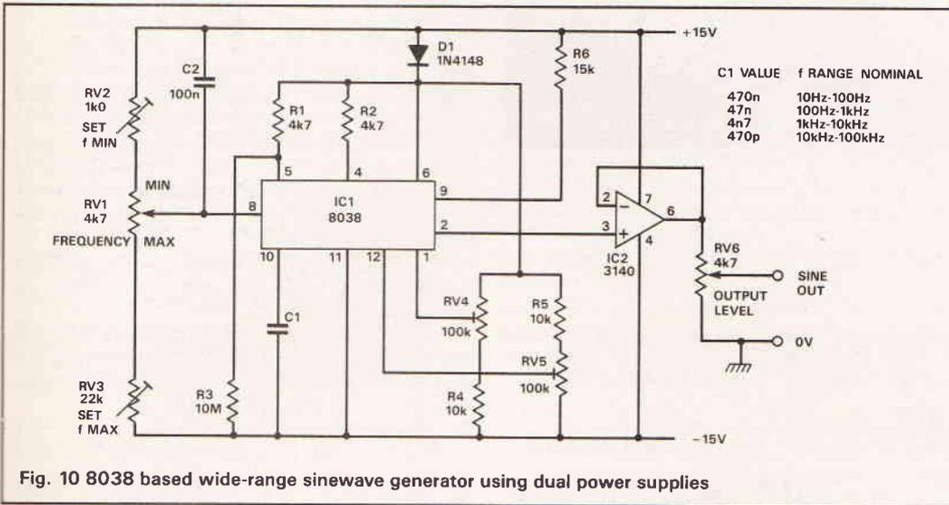
Fig. 10 8038 based wide-range sinewave generator using dual power supplies
