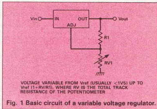
Fig. 1 Basic circuit of a variable voltage regulator.
