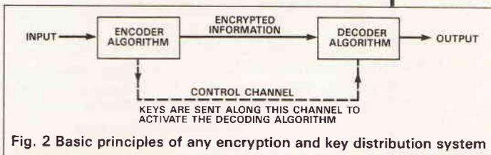
Fig. 2 Basic principles of any encryption and key distribution system
