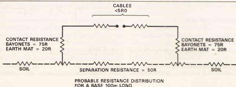
Fig. 2 Probable resistance distribution in a typical base
