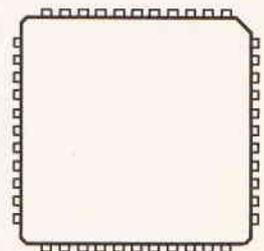
**Fig. 6 Plastic leaded chip carriers (PLCCs) house chip integrated circuits, and have J-shaped terminations**
