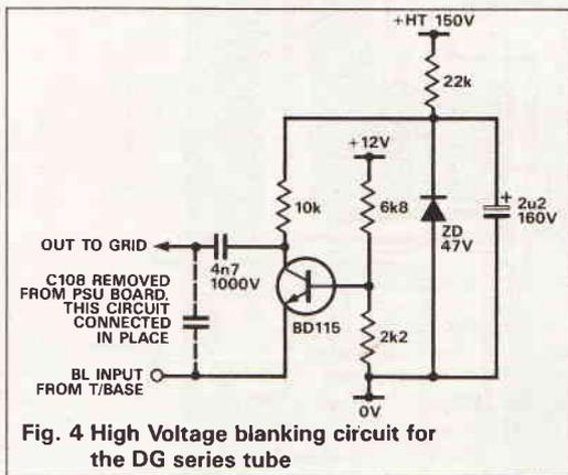
Fig. 4 High Voltage blanking circuit for the DG series tube
