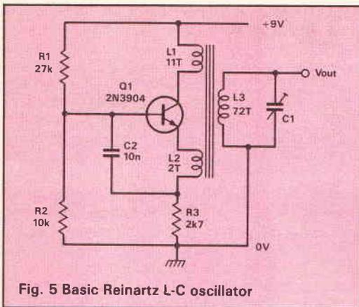
Fig. 5 Basic Reinartz L-C oscillator
