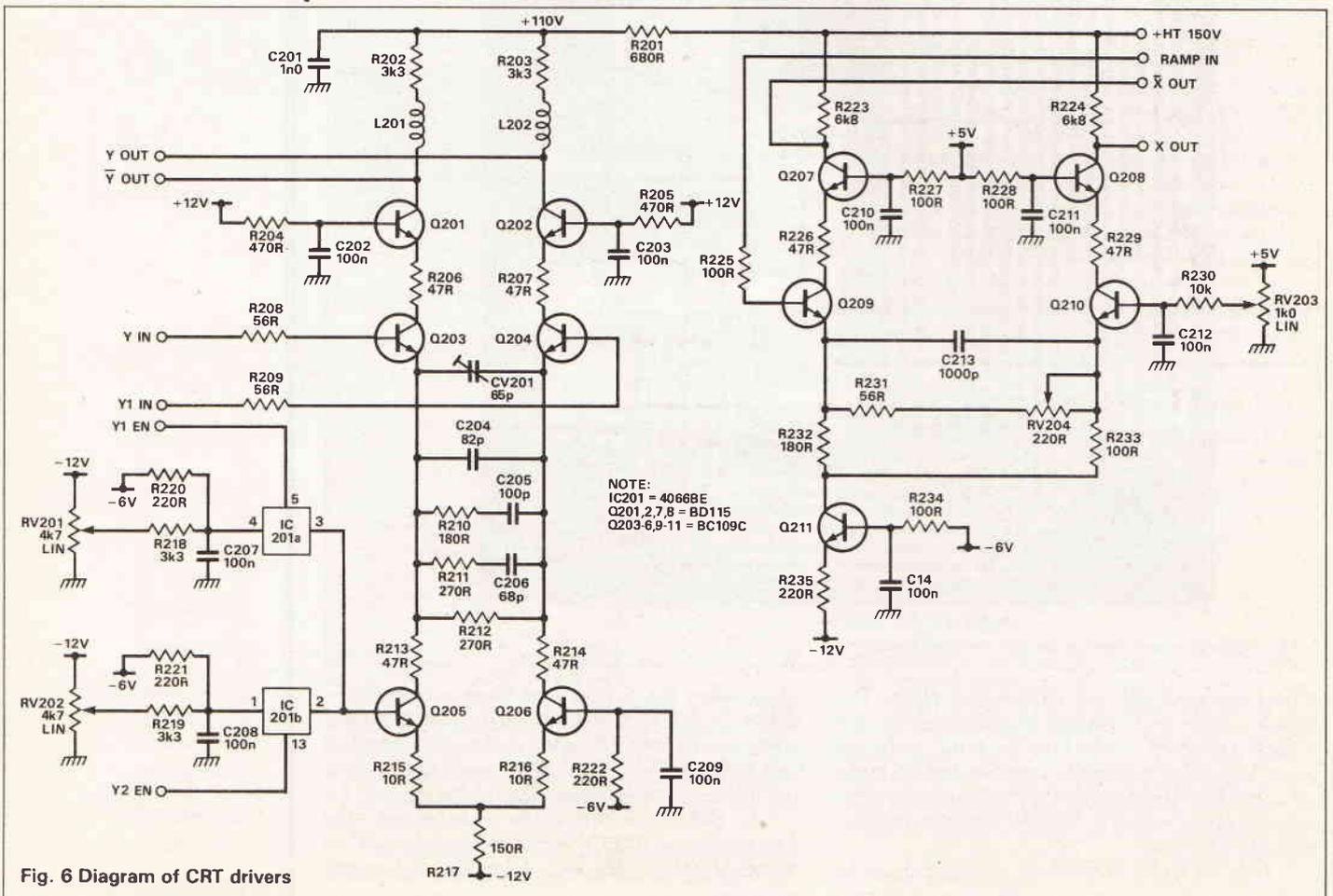
Fig. 6 Diagram of CRT drivers
