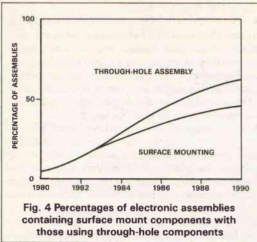
**Fig. 4 Percentages of electronic assemblies containing surface mount components with those using through-hole components**
