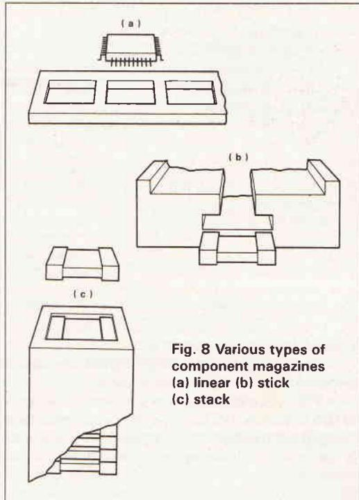
Fig. 8 Various types of component magazines (a) linear (b) stick (c) stack
