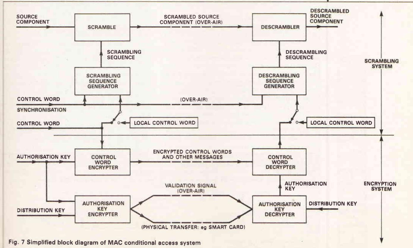
Fig. 7 Simplified block diagram of MAC conditional access system
