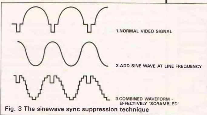
Fig. 3 The sinewave sync suppression technique
