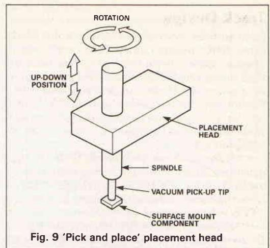
Fig. 9 'Pick and place' placement head
