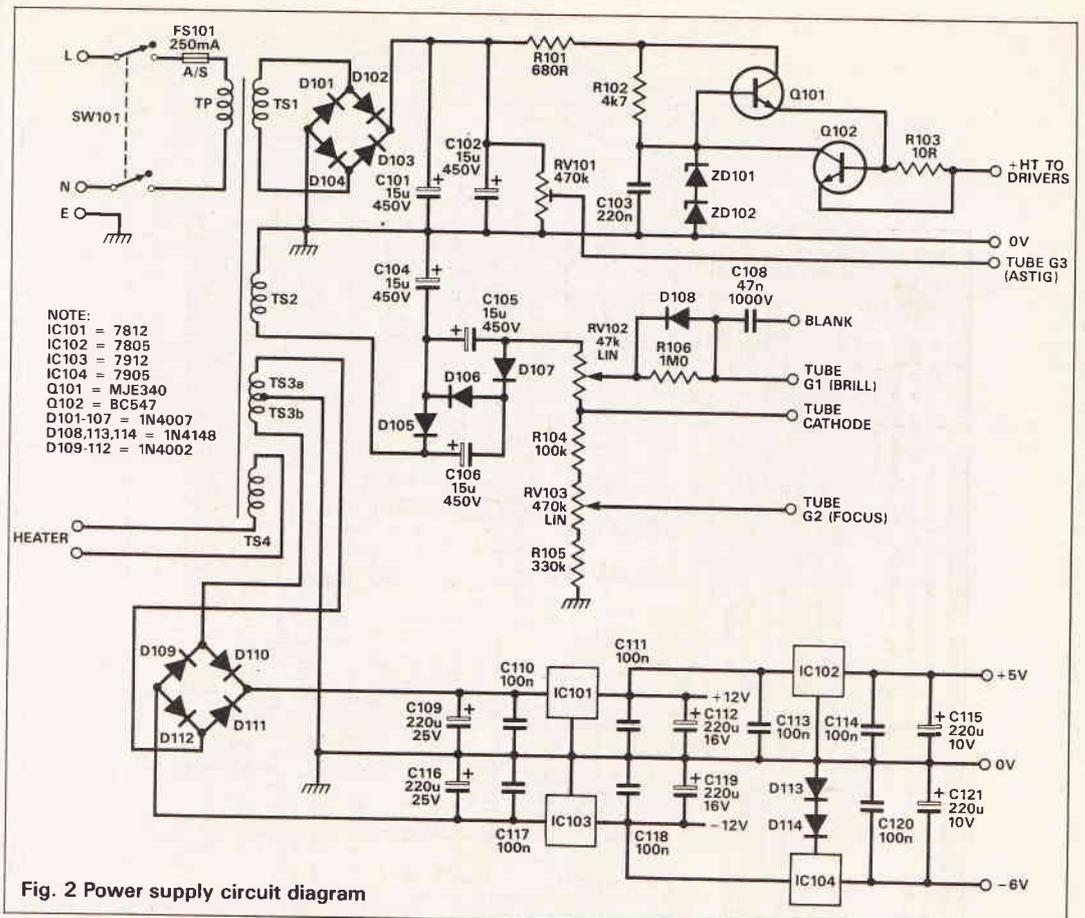
Fig. 2 Power supply circuit diagram
