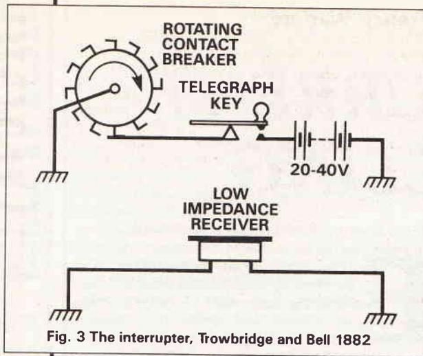
Fig. 3 The interrupter, Trowbridge and Bell 1882
