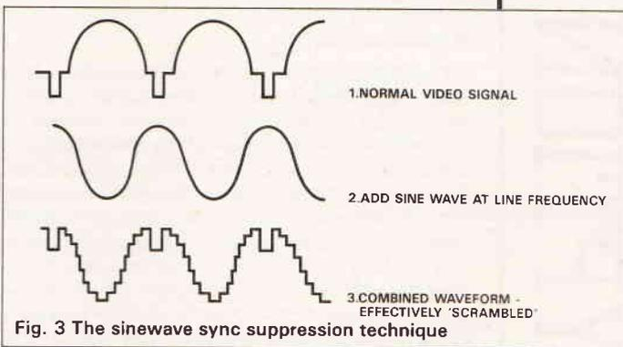
Fig. 3 The sinewave sync suppression technique
