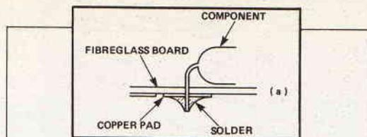
Fig. 1 A conventional through-hole PCB. A leaded component is inserted through holes in the board and soldered to the copper track on the other side
