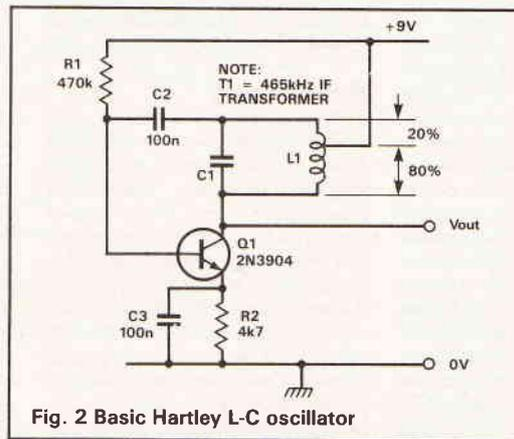
Fig. 2 Basic Hartley L-C oscillator
