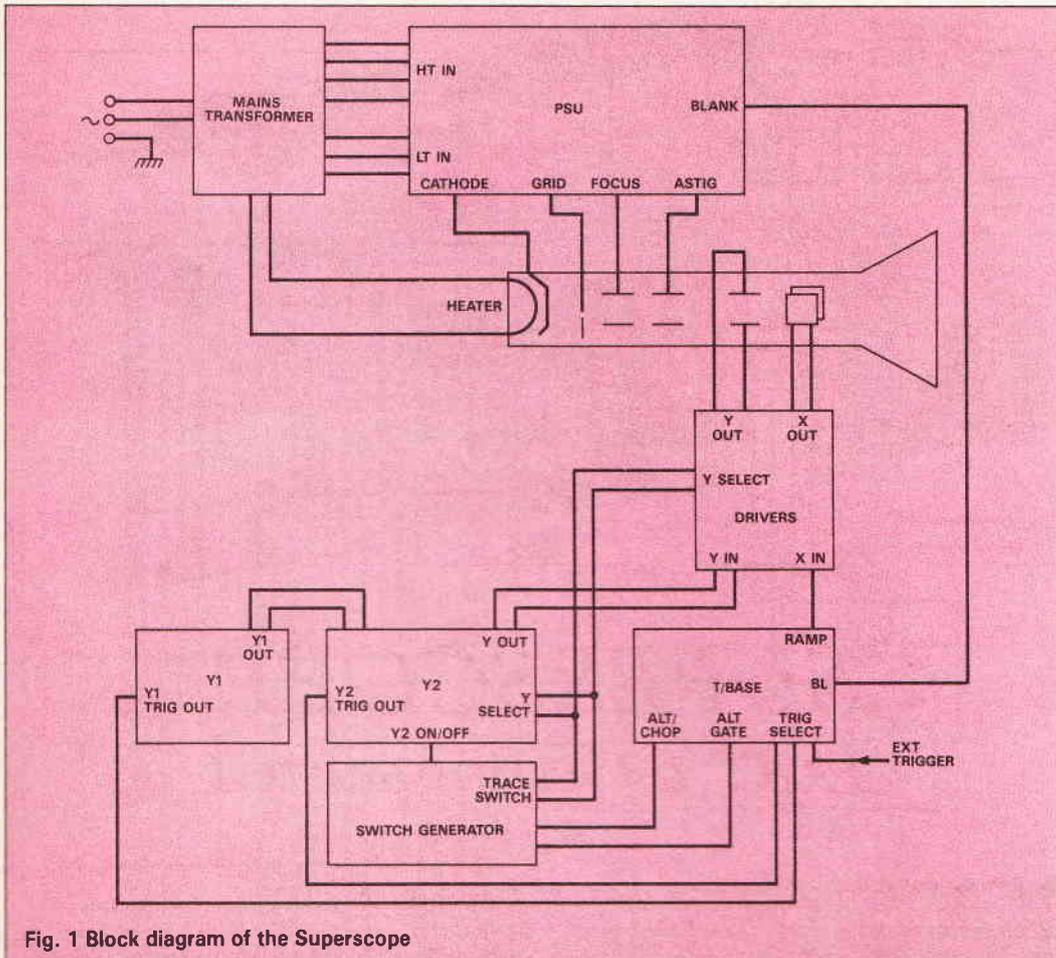
Fig. 1 Block diagram of the Superscope
