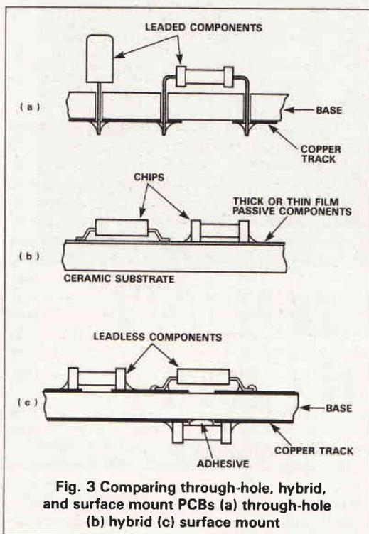
Fig. 3 Comparing through-hole, hybrid, and surface mount PCBs (a) through-hole (b) hybrid (c) surface mount
