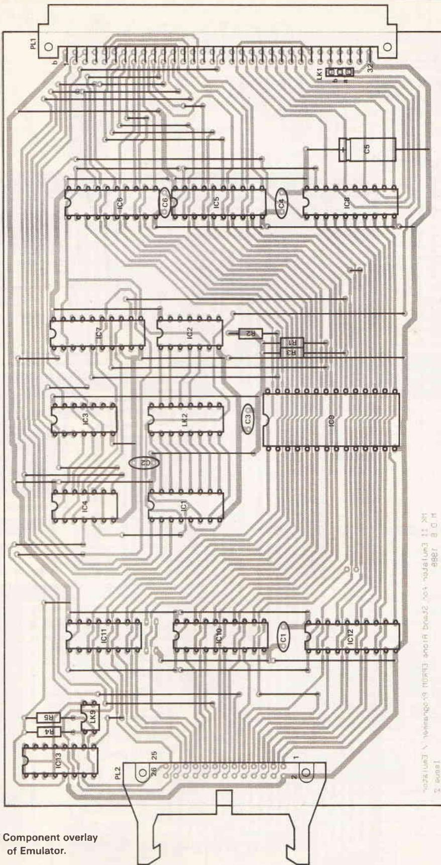
Fig.5 Component overlay of Emulator.
