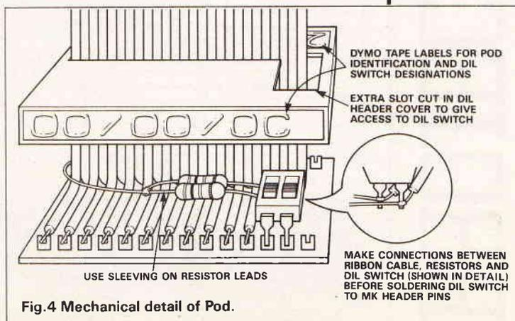
Fig.4 Mechanical detail of Pod.
