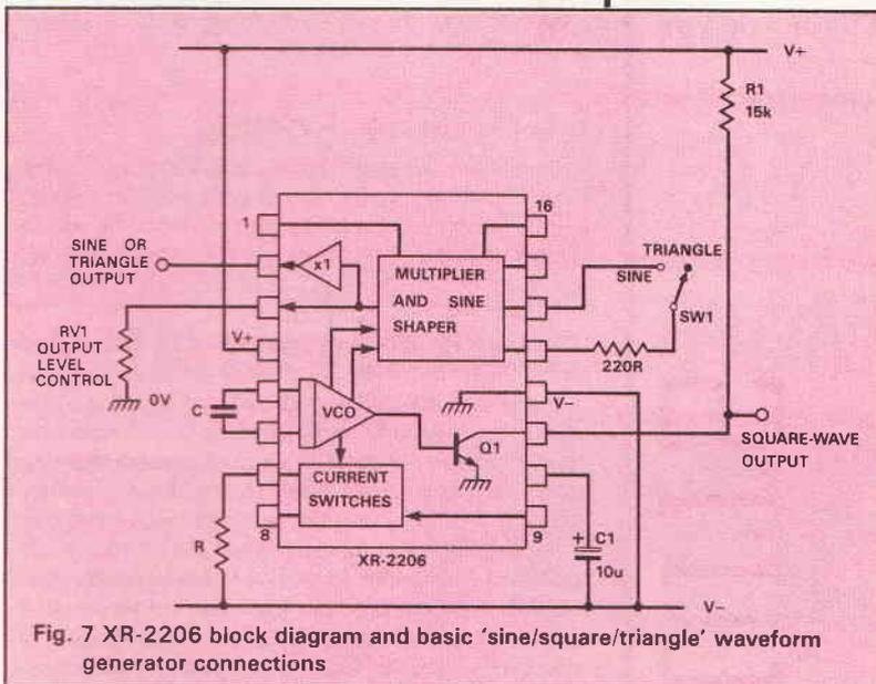
Fig. 7 XR-2206 block diagram and basic 'sine/square/triangle' waveform generator connections
