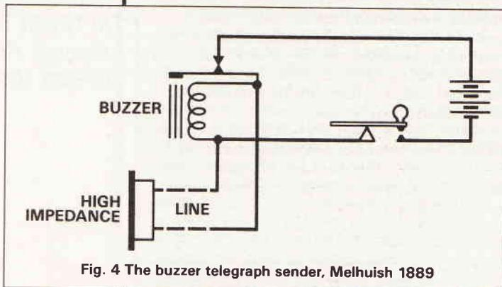
Fig. 4 The buzzer telegraph sender, Melhuish 1889
