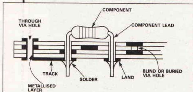
Fig. 2 Principle of a multi-layer PCB, where many layers of copper track are laminated together with insulating layers to form a single board. Holes can either go right through the board, or merely between two or more of the layers
