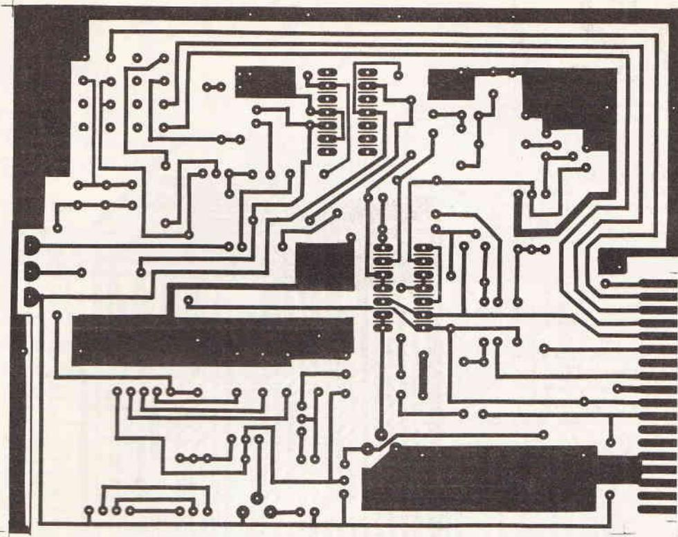
The Superscope timebase foil
