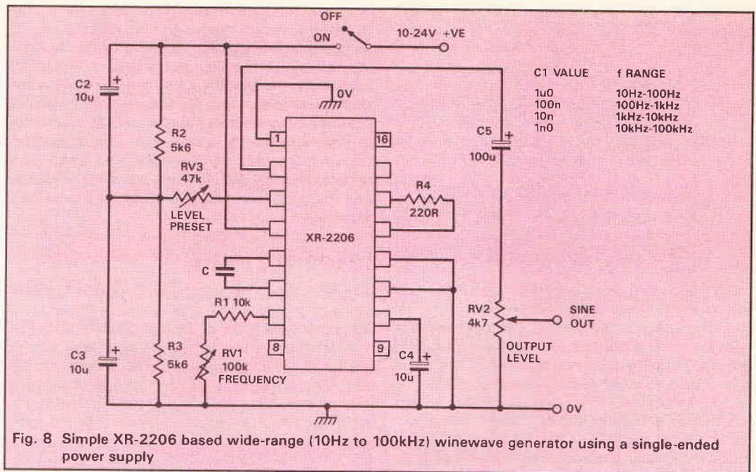
Fig. 8 Simple XR-2206 based wide-range (10Hz to 100kHz) winewave generator using a single-ended power supply
