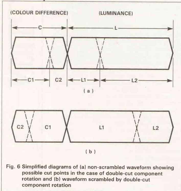
Fig. 6 Simplified diagrams of (a) non-scrambled waveform showing possible cut points in the case of double-cut component rotation and (b) waveform scrambled by double-cut component rotation
