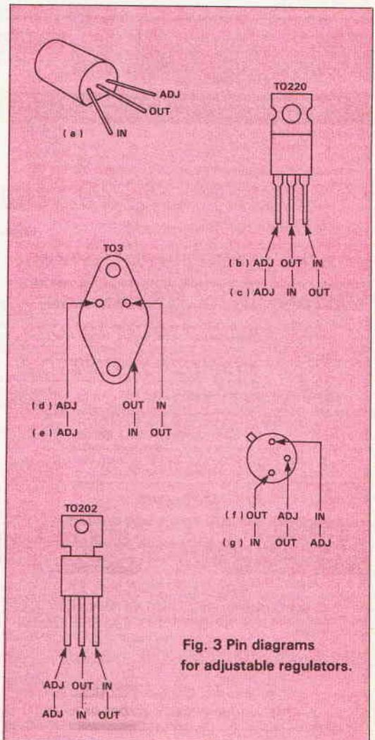
Fig. 3 Pin diagrams for adjustable regulators.
