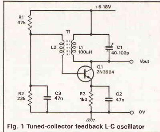
Fig. 1 Tuned-collector feedback L-C oscillator
