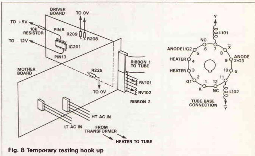
Fig. 8 Temporary testing hook up
