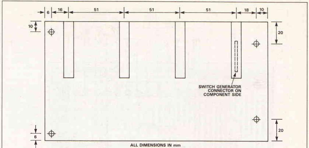
Fig. 5 Motherboard edge-connector mounting details
