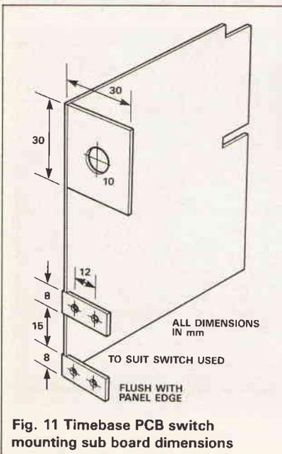
Fig. 11 Timebase PCB switch mounting sub board dimensions
