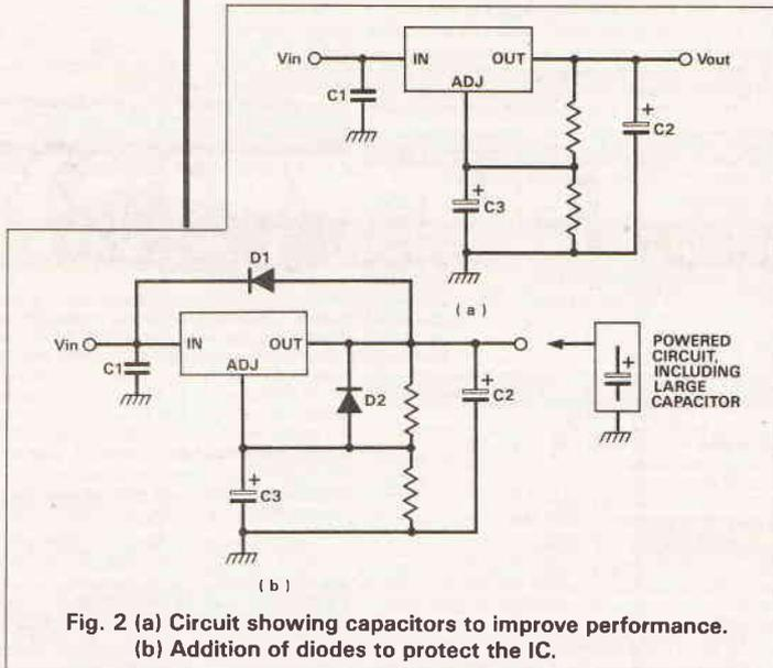
Fig. 2 (a) Circuit showing capacitors to improve performance. (b) Addition of diodes to protect the IC.
