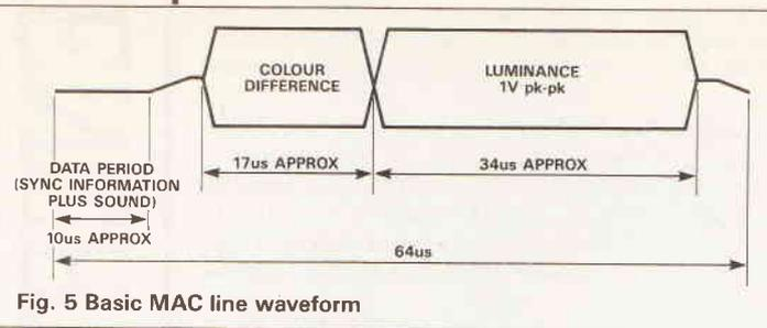
Fig. 5 Basic MAC line waveform
