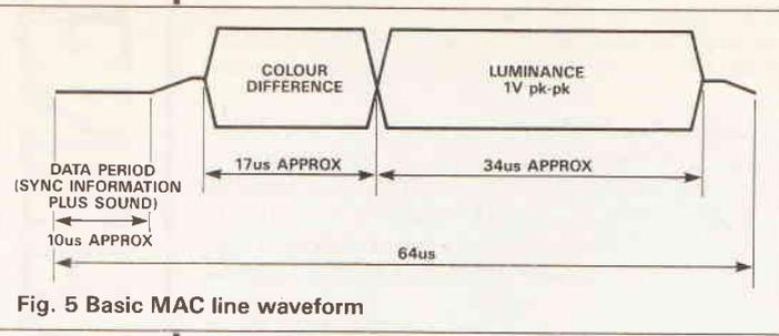
Fig. 5 Basic MAC line waveform
