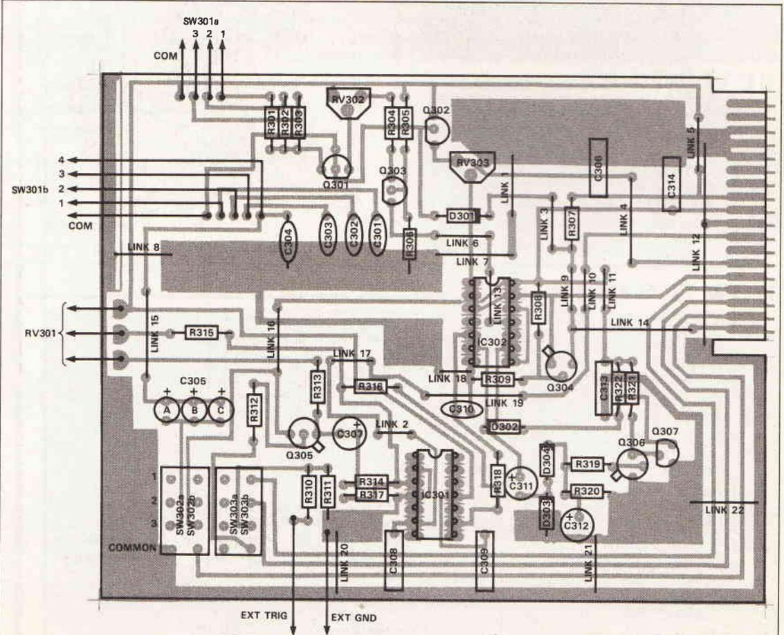
Fig. 10 Component overlay for timebase
