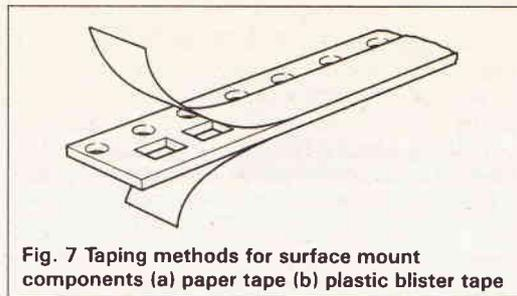
Fig. 7 Taping methods for surface mount components (a) paper tape (b) plastic blister tape
