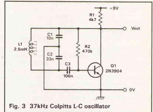
Fig. 3 37kHz Colpitts L-C oscillator
