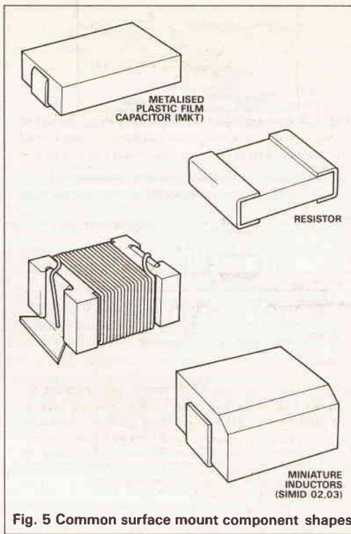
**Fig. 5 Common surface mount component shapes**
