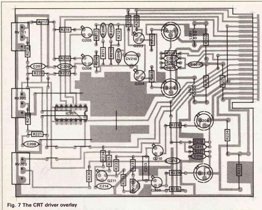
Fig. 7 The CRT driver overlay
