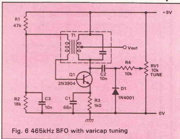
Fig. 6 465kHz BFO with varicap tuning
