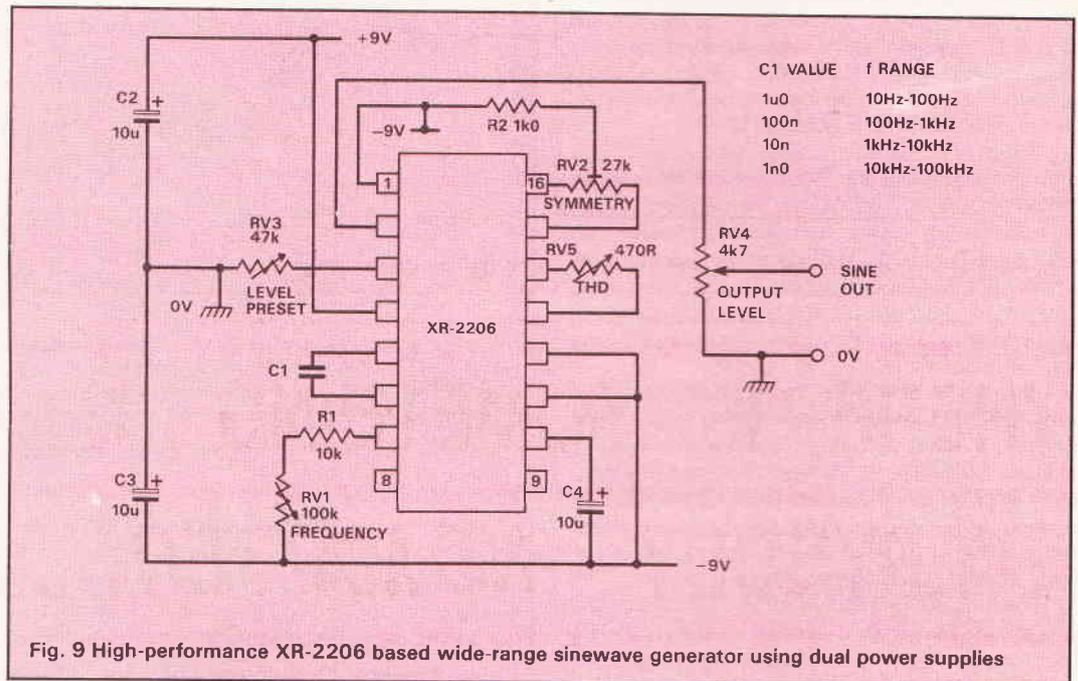
Fig. 9 High-performance XR-2206 based wide-range sinewave generator using dual power supplies
