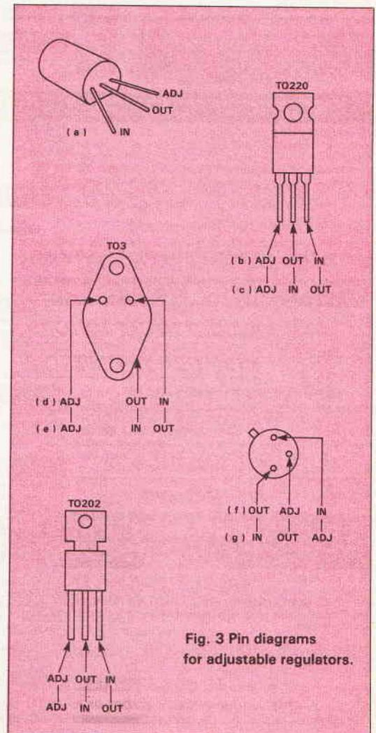
Fig. 3 Pin diagrams for adjustable regulators.
