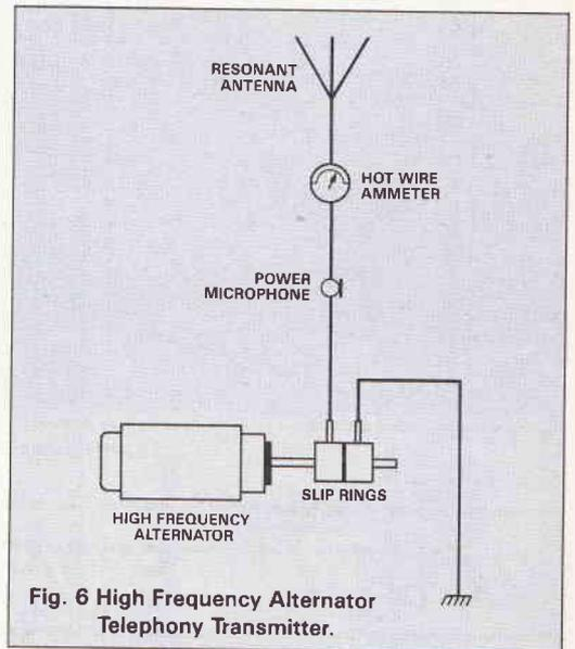
Fig. 6 High Frequency Alternator Telephony Transmitter.
