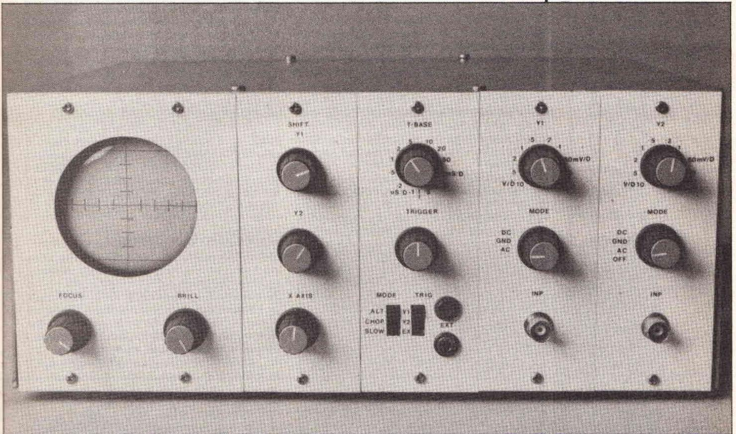
**T**his follow-up to the Superscope project published in ETI this February and March should give beginners an insight into how an oscilloscope works in general and how to get the best out of the Superscope in particular.
