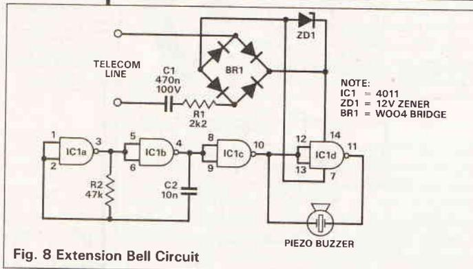
Fig. 8 Extension Bell Circuit
