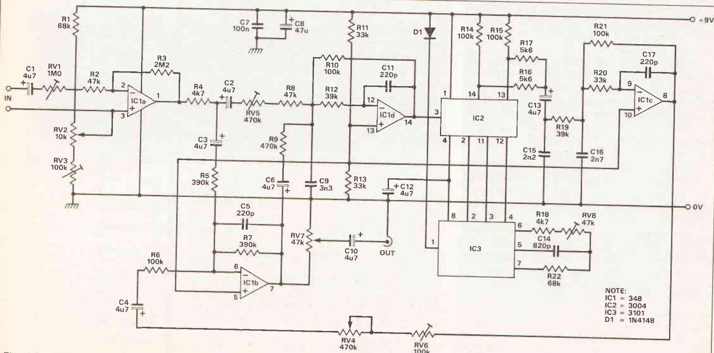
Fig. 1 ETI Fecko Box circuit
