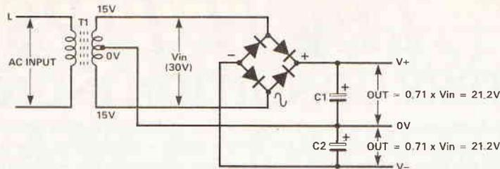
Fig 15. Dual (split) PSU using centre-tapped transformer and bridge rectifiers.
