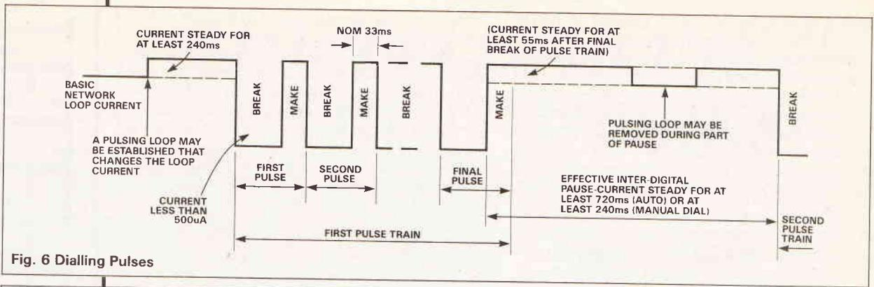
Fig. 6 Dialling Pulses
