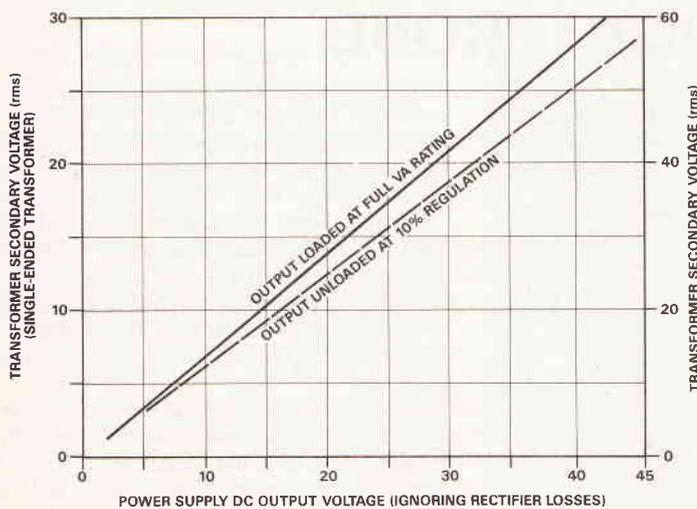
Fig 17. Transformer selection chart. Decide on the required loaded DC output voltage (say 21 volts), then read across to find the corresponding secondary voltage (15V single-ended or 30V centre-tapped).
