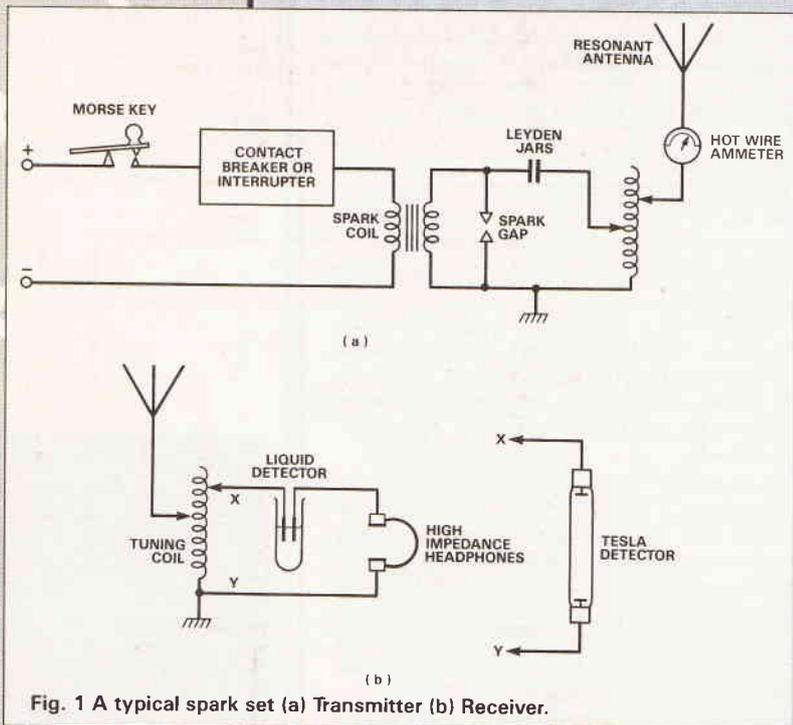
Fig. 1 A typical spark set (a) Transmitter (b) Receiver.
