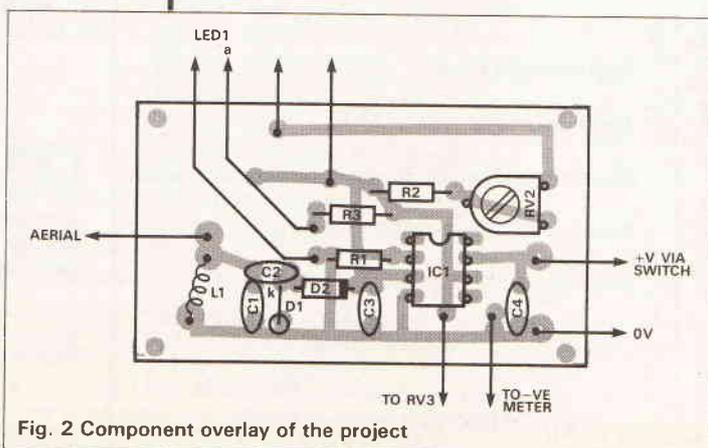
Fig. 2 Component overlay of the project
