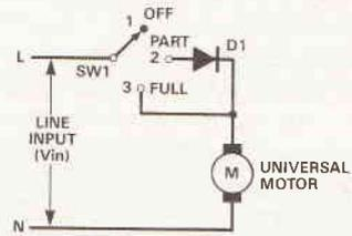
Fig 10. Drill motor runs at 70% of maximum speed in PART position.
