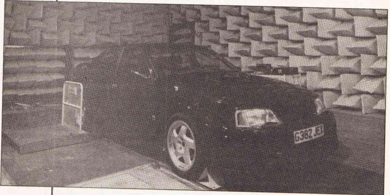
Noise measurements made in rooms with hard walls will include the sound reflected from the walls, as well as that radiated directly from the source. In a real situation, noise from a vehicle will be reflected only from the hard road surface. Noise radiated in other directions will be dissipated without reflection.
