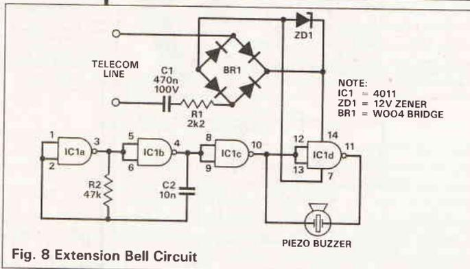
Fig. 8 Extension Bell Circuit
