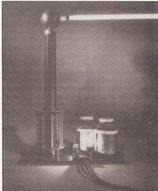
Replica of original Tesla coil, lighting fluorescent tube.
