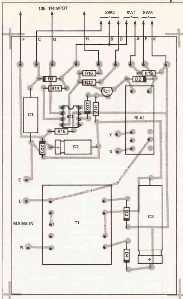
Fig.2 Component overlay of timer showing off-board connections
