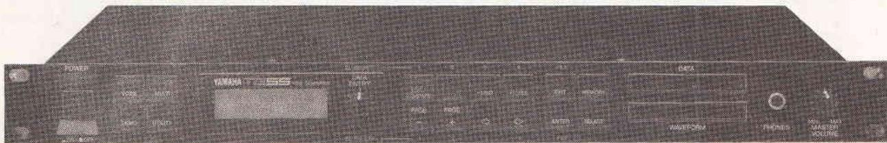
**F**ollowing closely behind the launch of the SY77 synthesiser workstation comes the TG55 from Yamaha, a rack mounted MIDI controlled tone generator that contains many of the features to be had in the SY77 featured in the audio news section last month.
