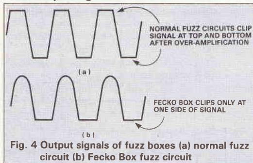
Fig. 4 Output signals of fuzz boxes (a) normal fuzz circuit (b) Fecko Box fuzz circuit
