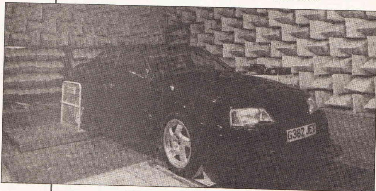
Noise measurements made in rooms with hard walls will include the sound reflected from the walls, as well as that radiated directly from the source. In a real situation, noise from a vehicle will be reflected only from the hard road surface. Noise radiated in other directions will be dissipated without reflection.
