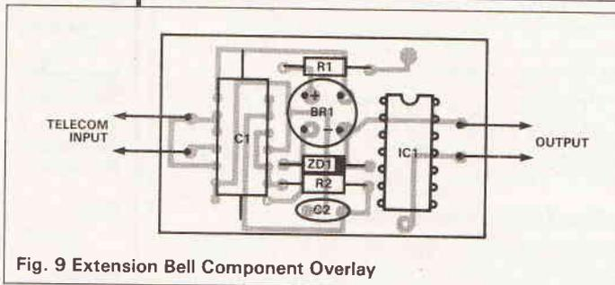
Fig. 9 Extension Bell Component Overlay
