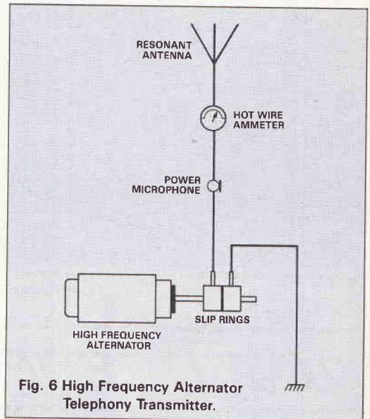
Fig. 6 High Frequency Alternator Telephony Transmitter.
