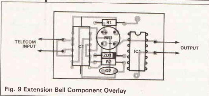
Fig. 9 Extension Bell Component Overlay
