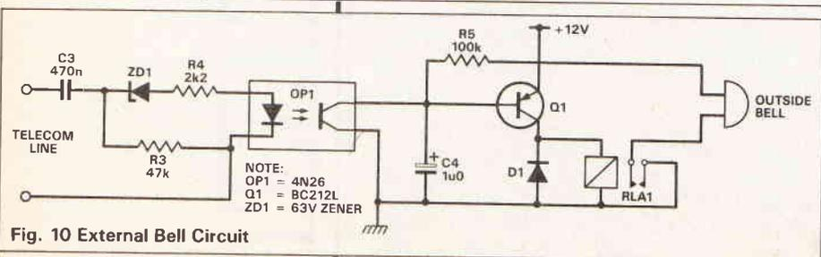
Fig. 10 External Bell Circuit
