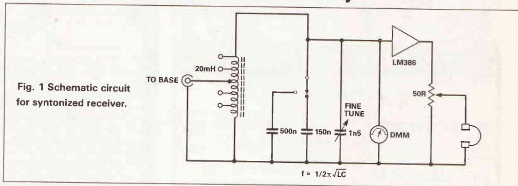
Fig. 1 Schematic circuit for syntonized receiver.
