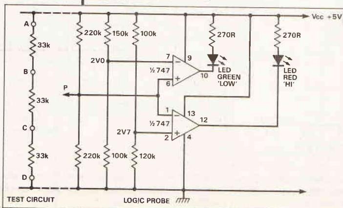
The reference levels are adjusted such that there is no output between 2V and 2.7V, and both LEDs are off. If the input to the probe at point P is below 2V the green LED comes on indicating a logic low state. If the input is above 2.7V the red LED is on indicating a logic high state. The inoperative window voltage levels can be adjusted, if required, by altering the reference levels at the inputs to the inverting and noninverting amplifiers, pins 7 and 2 respectively.
