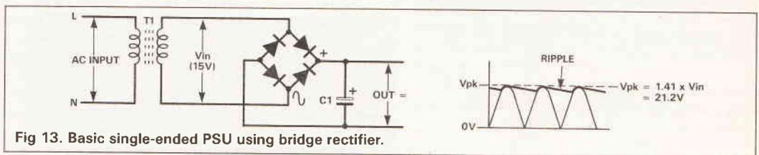
Fig 13. Basic single-ended PSU using bridge rectifier.
