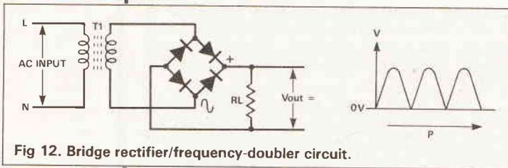
Fig 12. Bridge rectifier/frequency-doubler circuit.
