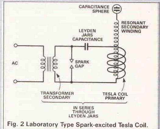
Fig. 2 Laboratory Type Spark-excited Tesla Coil.
