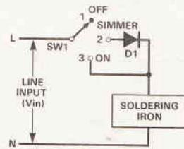
Fig 11. Soldering iron operates at 1/3 power in SIMMER position.
