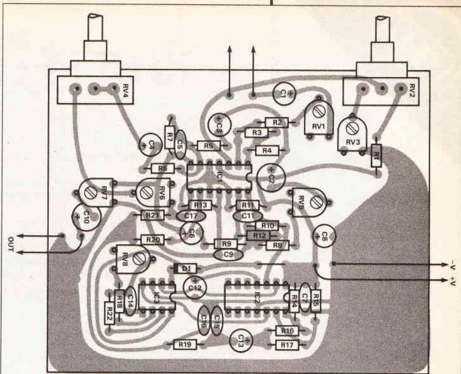
Fig. 2 Component overlay for the Fecko Box
