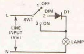
Fig 9. Lamp burns at half brightness in DIM position.
