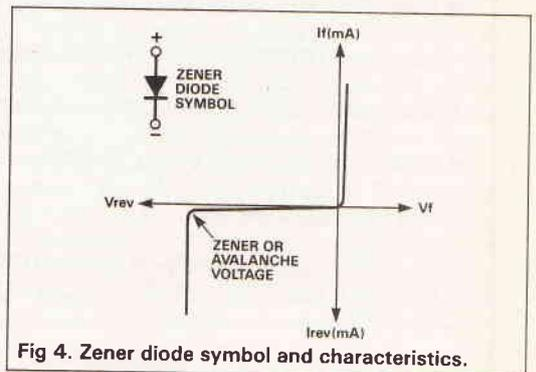
Fig 4. Zener diode symbol and characteristics.
