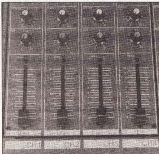
inputs is about right compared to the measured value but better figures could be achieved with careful design and choice of components. One also has to be careful of how many 'live' inputs there are feeding into the output bus high fader levels otherwise the noise may become unacceptable. I've always had reservations about introducing graphic equalisers into the signal path, but I was pleased to hear that the noise contribution made by the graphic was at an acceptably
