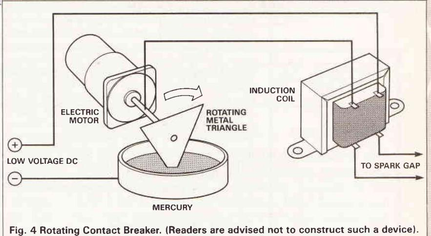
Fig. 4 Rotating Contact Breaker. (Readers are advised not to construct such a device).
