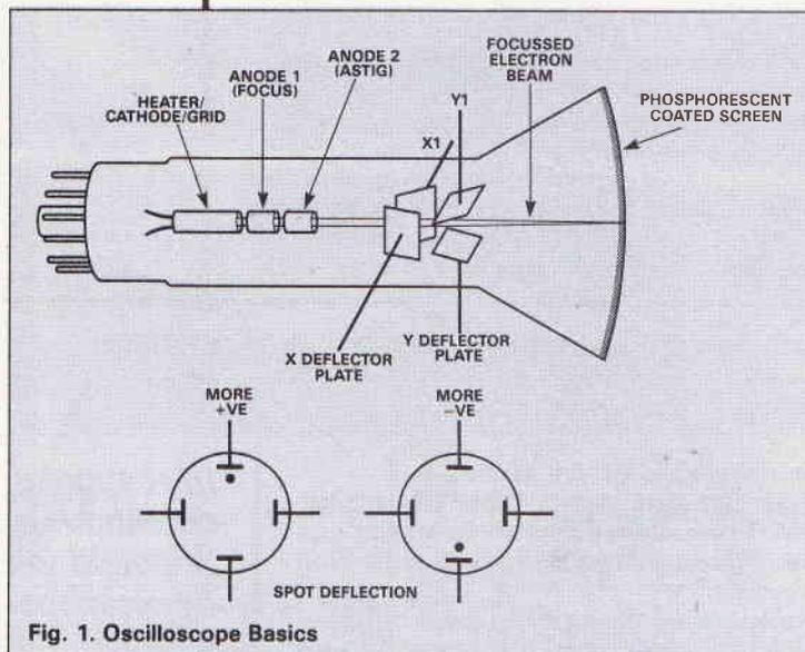
Fig. 1. Oscilloscope Basics
