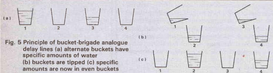
Fig. 5 Principle of bucket-brigade analogue delay lines (a) alternate buckets have specific amounts of water (b) buckets are tipped (c) specific amounts are now in even buckets
