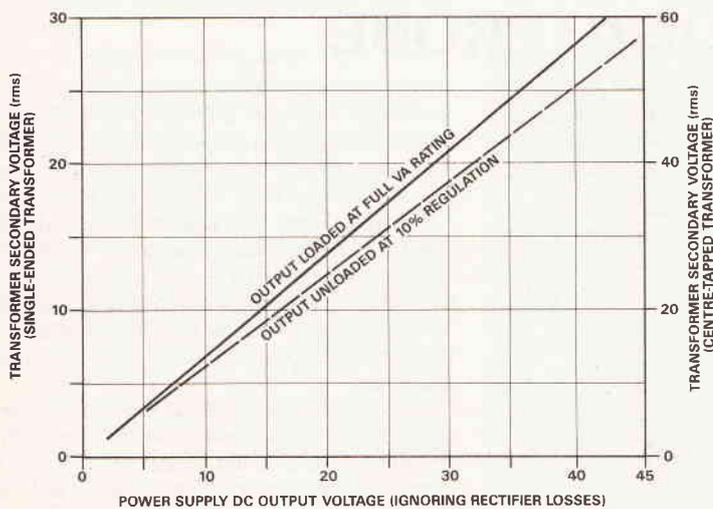
Fig 17. Transformer selection chart. Decide on the required loaded DC output voltage (say 21 volts), then read across to find the corresponding secondary voltage (15V single-ended or 30V centre-tapped).
