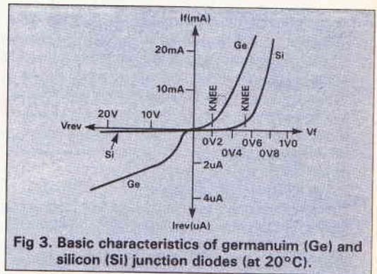
Fig 3. Basic characteristics of germanium (Ge) and silicon (Si) junction diodes (at 20°C).
