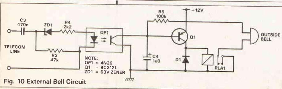
Fig. 10 External Bell Circuit
