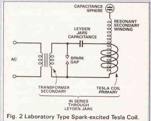
Fig. 2 Laboratory Type Spark-excited Tesla Coil.
