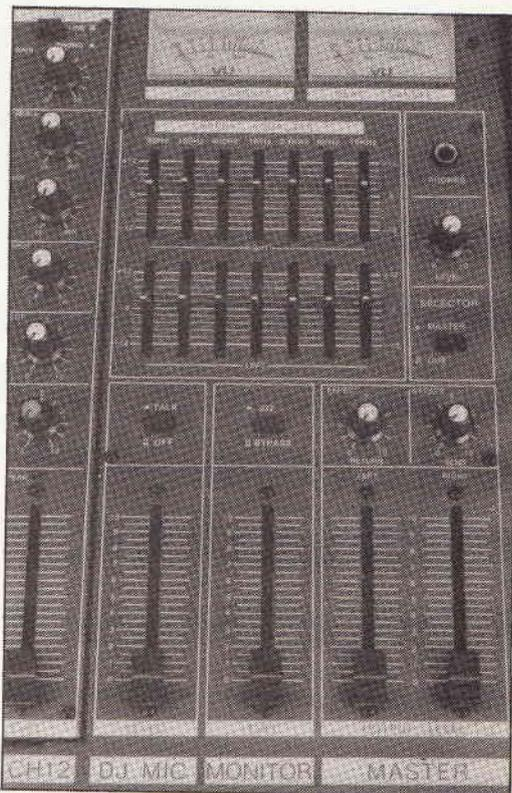
Just above the principal channel fader, an overload LED gives a handy and quick indication of overdrive to the input amplifier. The LED cuts in at around +4dB.
