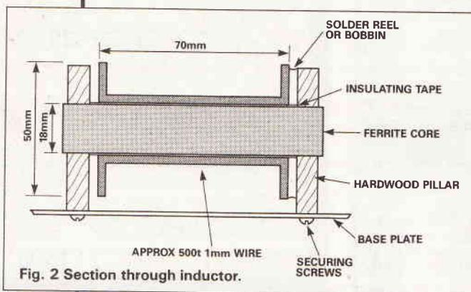
Fig. 2 Section through inductor.
