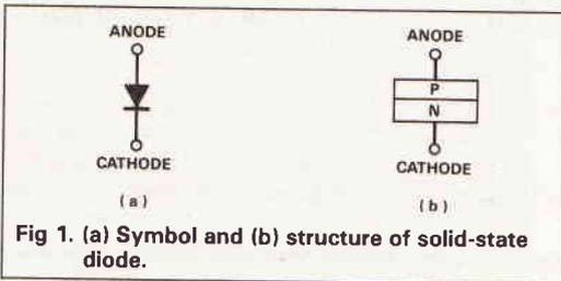
n junction. The p terminal is known as the *anode* and the n terminal as the *cathode*.
