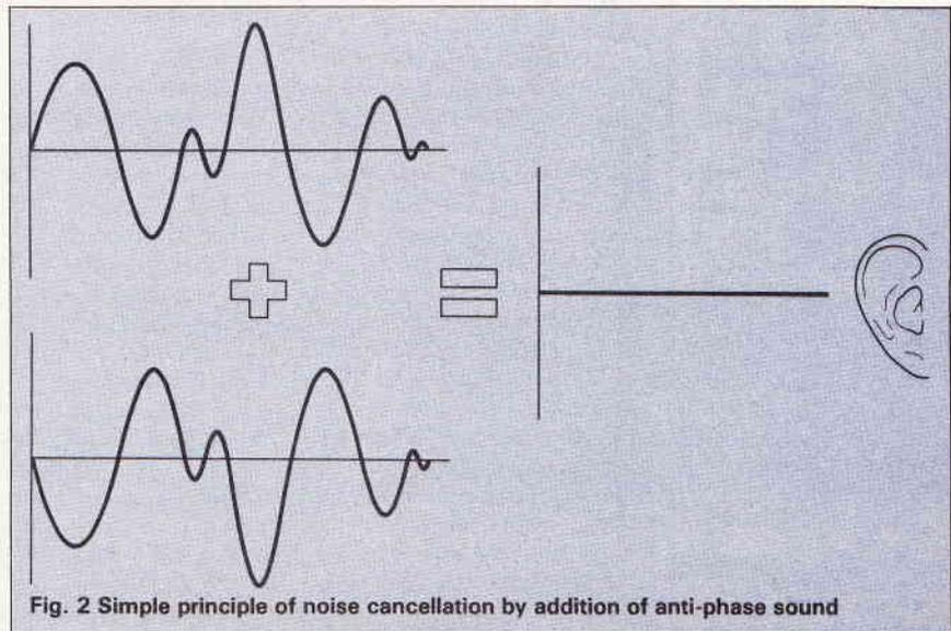
Fig. 2 Simple principle of noise cancellation by addition of anti-phase sound
