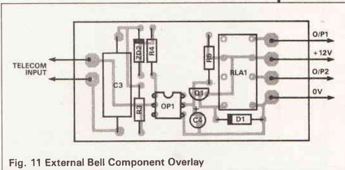
Fig. 11 External Bell Component Overlay
