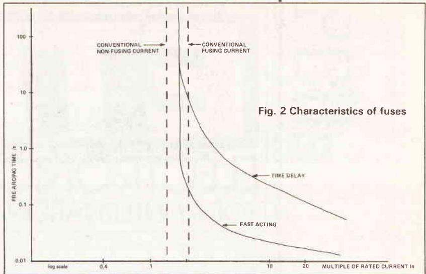
Fig. 2 Characteristics of fuses
