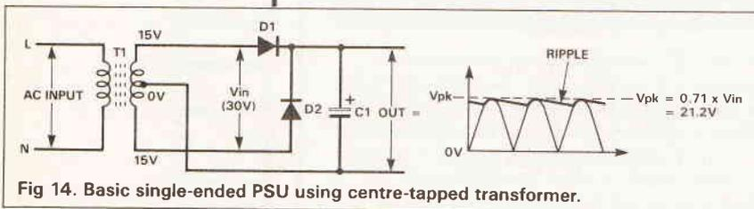
Fig 14. Basic single-ended PSU using centre-tapped transformer.
