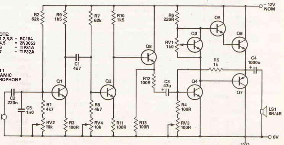
Fig. 3 Megaphone Amplifier Circuit
