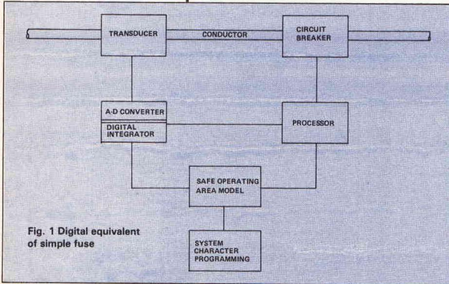
Fig. 1 Digital equivalent of simple fuse
