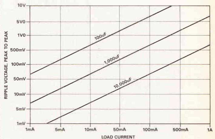
Fig 18. Filter capacitor selection chart, relating capacitor size to ripple voltage and load current in a full-wave rectified 50-60Hz powered circuit.
