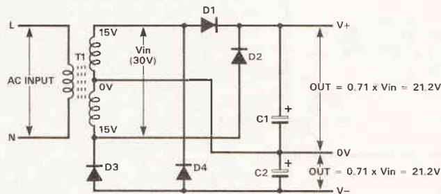
Fig 16. Dual (split) PSU using centre-tapped transformer and four rectifiers.
