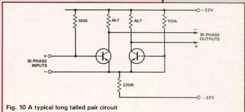
Fig. 10 A typical long tailed pair circuit
