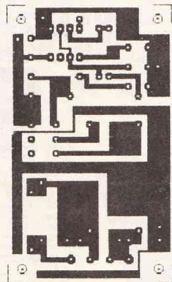
Remote Control Timeswitch Transmitter Board
