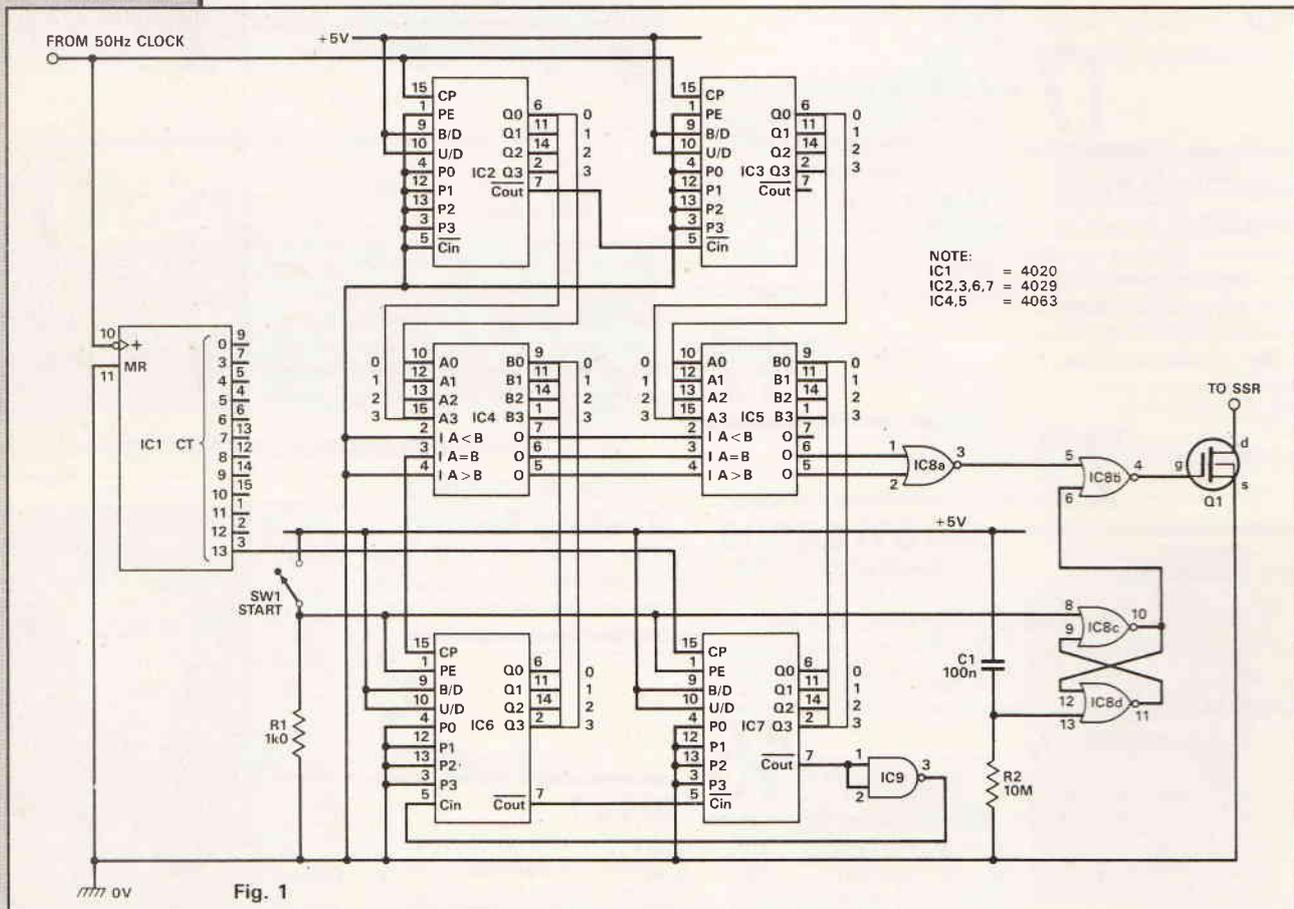
as 5V, although I showed a 12V supply in the previous issue. When I actually came to work out the details, there was nothing which could not run efficiently on 5V, and why use a higher voltage when a lower one will do the job? It turns out that 5V is convenient for the next phase of the design as well.
