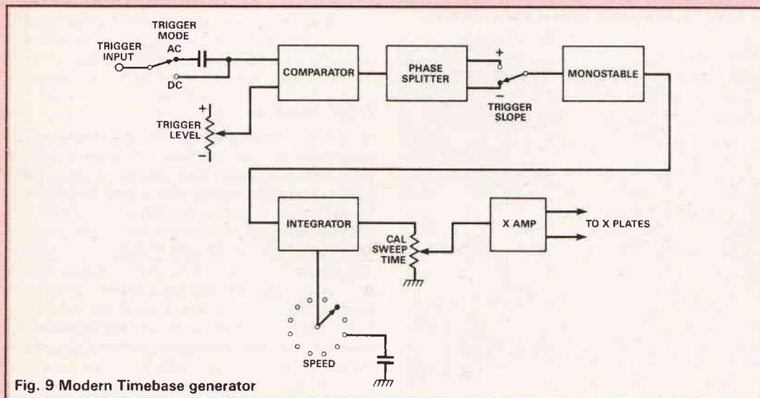
Fig. 9 Modern Timebase generator
