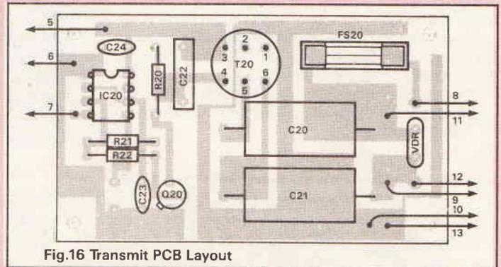
Fig.16 Transmit PCB Layout
