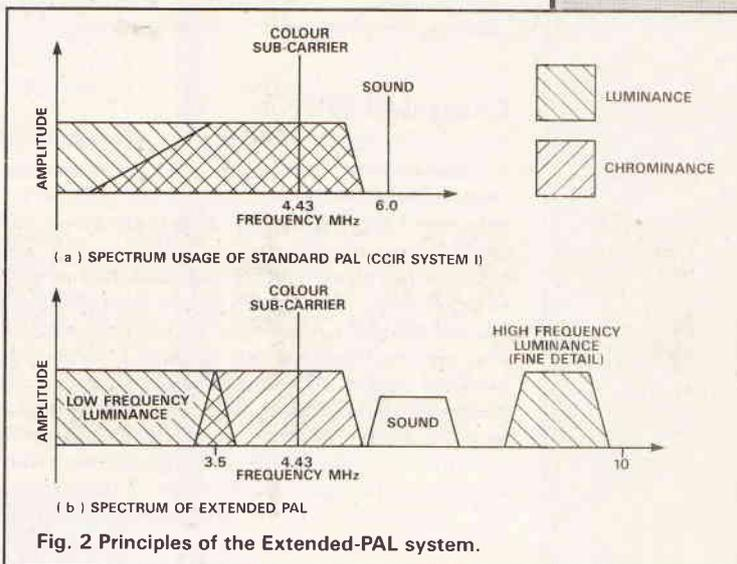
Fig. 2 Principles of the Extended-PAL system.
