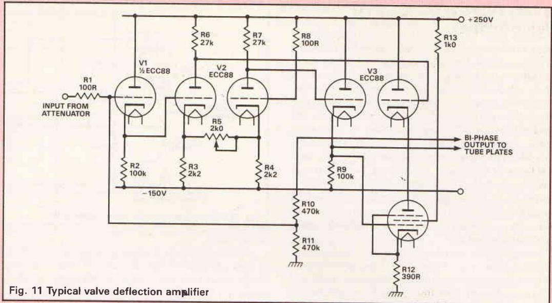
Fig. 11 Typical valve deflection amplifier
