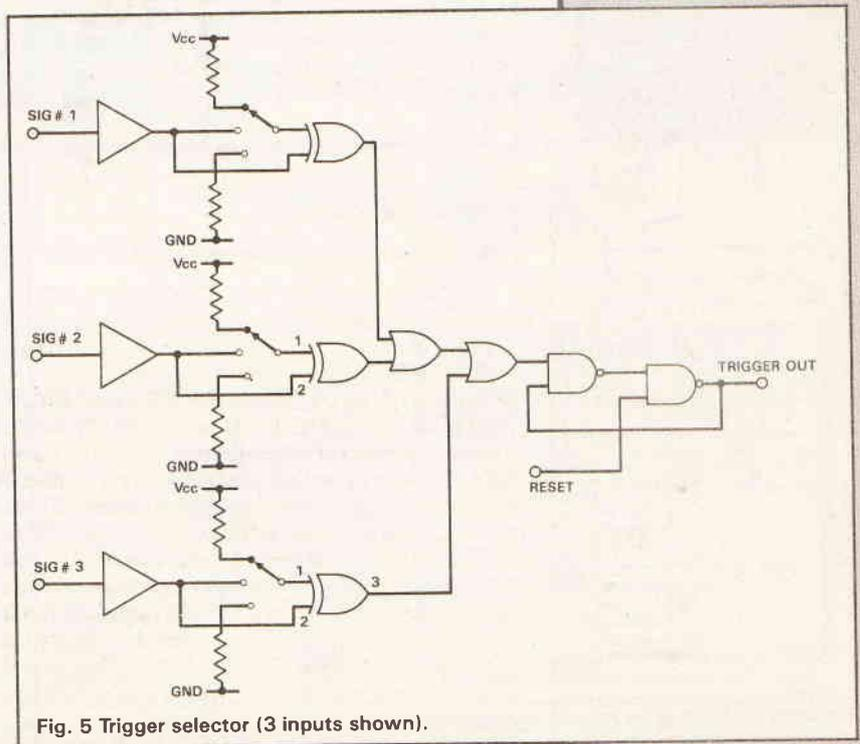
Fig. 5 Trigger selector (3 inputs shown).
