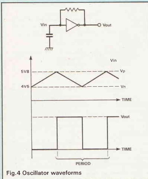
Fig.4 Oscillator waveforms
