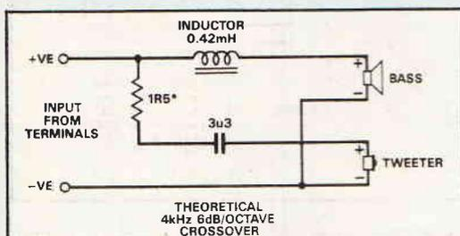
AS YOU CAN SEE IN THE DIAGRAM THE POSITIVE CONNECTION FROM THE INPUT IS CONNECTED TO THE INDUCTOR COIL AND THE 3u3 CAPACITOR. THE INDUCTOR GOES TO THE +VE ON THE BASS/MID UNIT AND THE CAPACITOR TO THE -VE ON THE TWEETER. THE NEGATIVE CONNECTIONS OF BOTH DRIVE UNITS GO DIRECTLY TO THE NEGATIVE INPUT.
