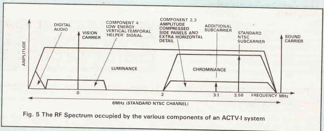
Fig. 5 The RF Spectrum occupied by the various components of an ACTV-I system
