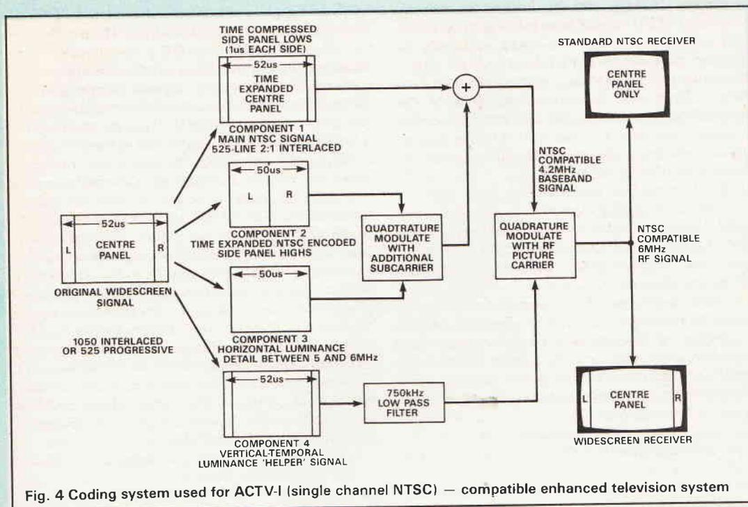
Fig. 4 Coding system used for ACTV-I (single channel NTSC) — compatible enhanced television system
