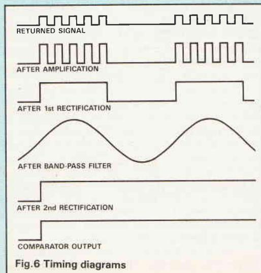
Fig.6 Timing diagrams
