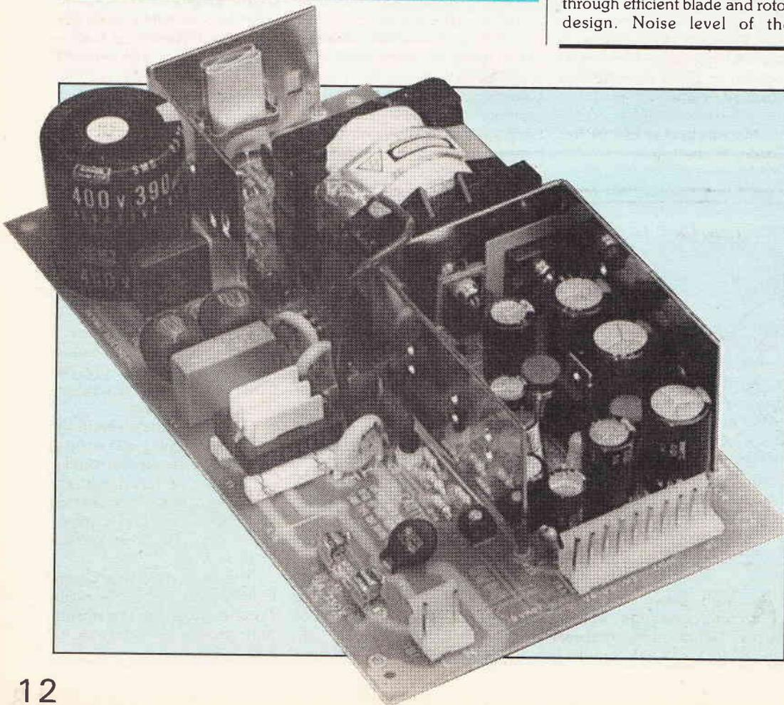
Skynet Electronic has launched a new range of 85W open frame, switched mode power supplies for portable computer systems, peripherals, robotics and instrumentation. With a wide universal input of 96 to 260V AC, over a frequency range of 47 to 440Hz, the SNP-318 series provides up to four outputs with a maximum of 85W continuous power over a 2.7kHz bandwidth.
