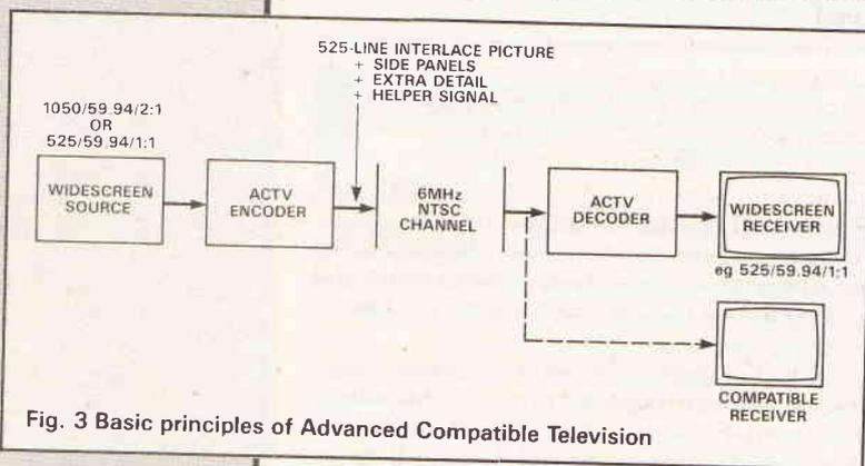
Fig. 3 Basic principles of Advanced Compatible Television
