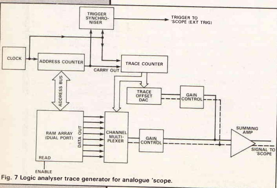
Fig. 7 Logic analyser trace generator for analogue 'scope.
