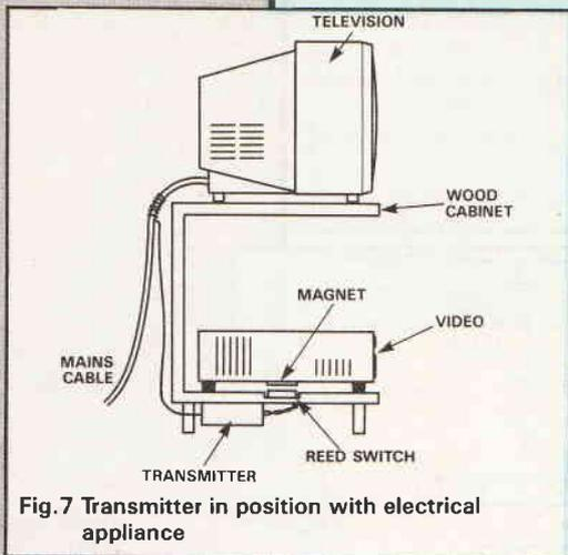
Fig. 7 Transmitter in position with electrical appliance
