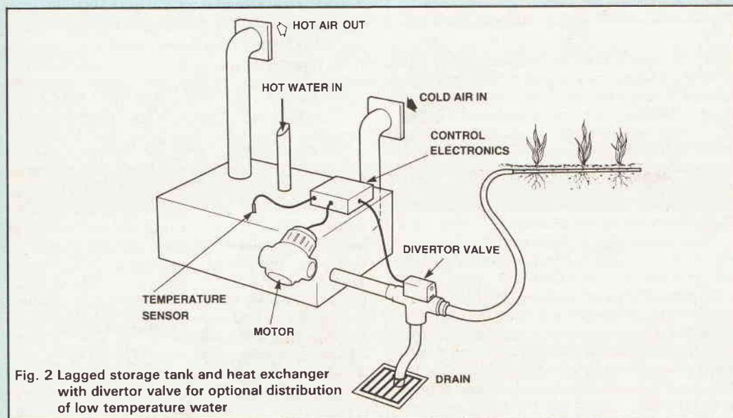
Fig. 2 Lagged storage tank and heat exchanger with divertor valve for optional distribution of low temperature water
