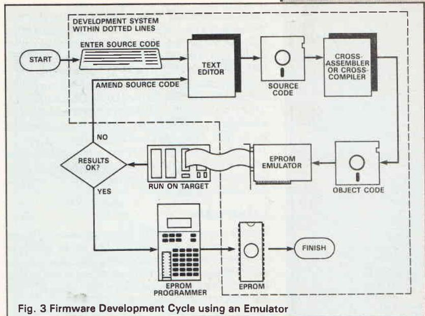
**Fig. 3 Firmware Development Cycle using an Emulator**
