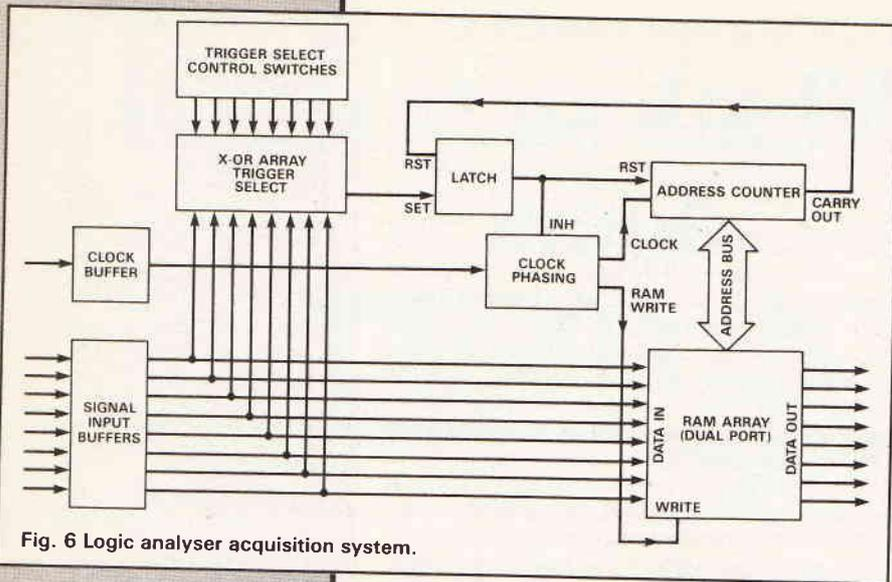
Fig. 6 Logic analyser acquisition system.
