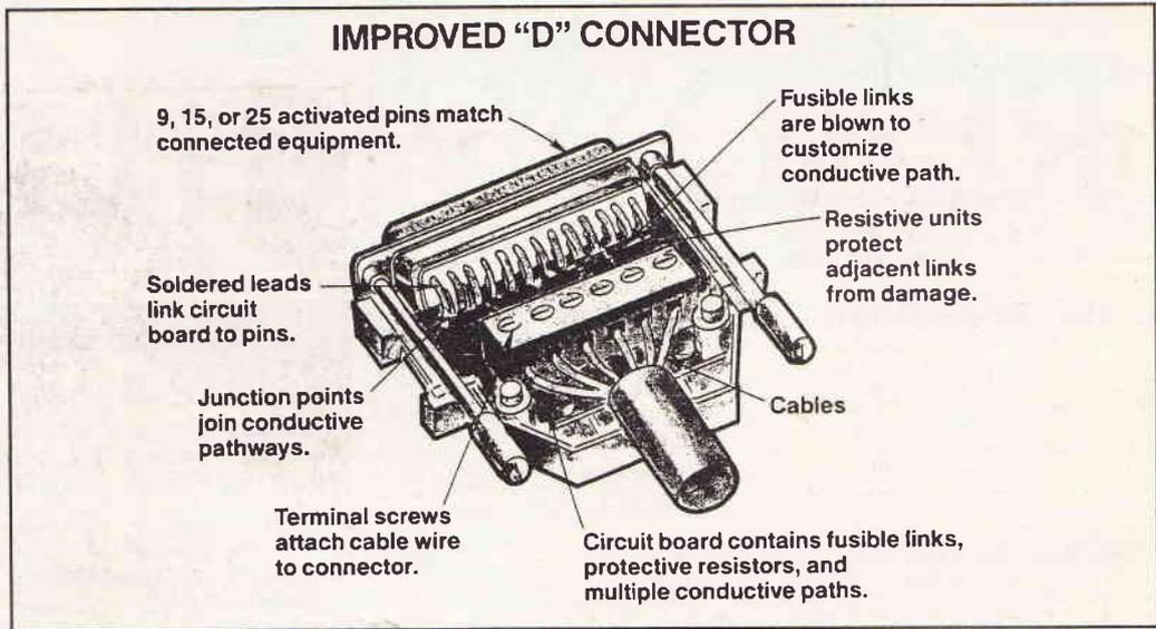
resistors and fuses, which permits multiple current paths. Shorting out the appropriate fuses provides a path matching the pin count of the manufacturer's device.
