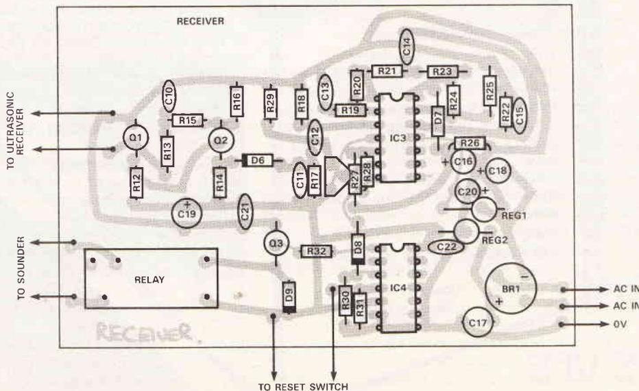
Fig.10 Component Overlay of Receiver
