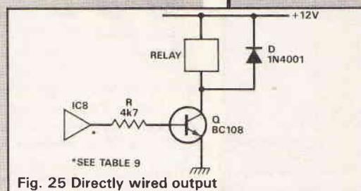
Fig. 25 Directly wired output
