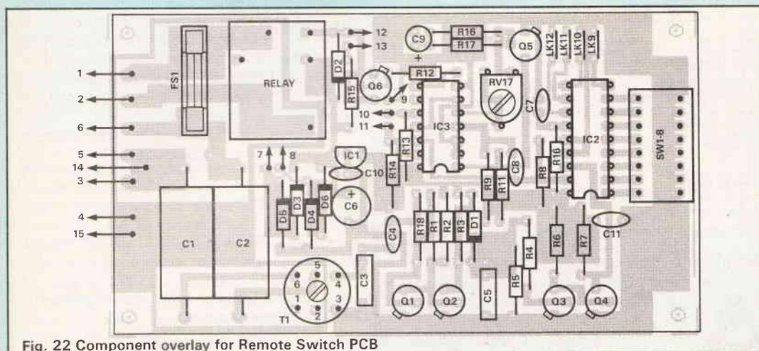
Fig. 22 Component overlay for Remote Switch PCB
