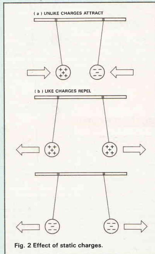
Fig. 2 Effect of static charges.
