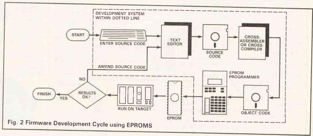
Fig. 2 Firmware Development Cycle using EPROMs
