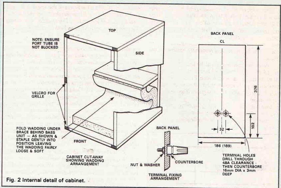
Fig. 2 Internal detail of cabinet.
