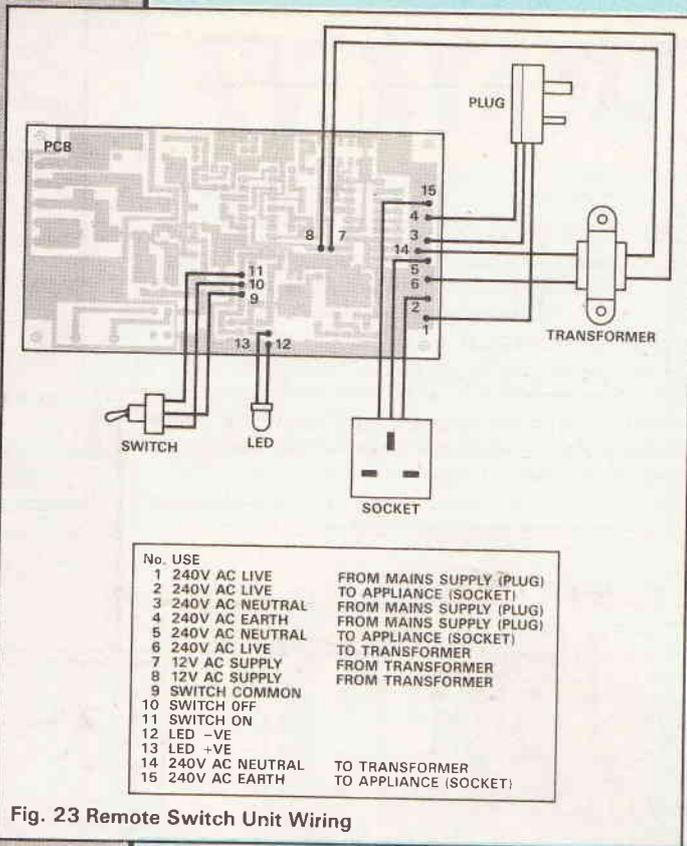
Fig. 23 Remote Switch Unit Wiring
