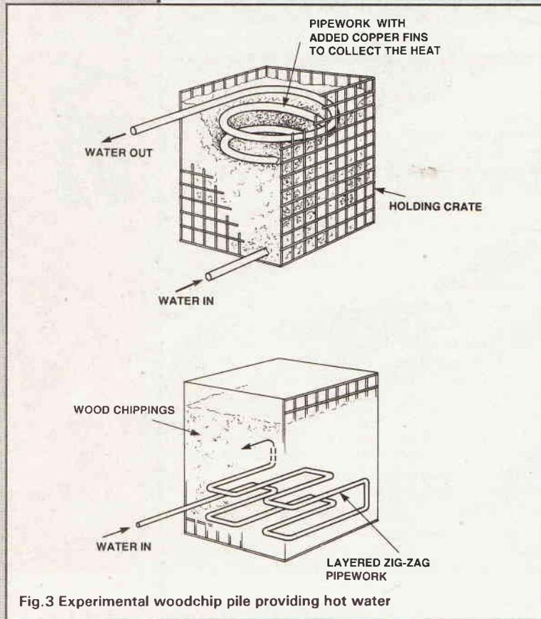
Fig.3 Experimental woodchip pile providing hot water
