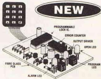
Keys could be a thing of the past with this new high security lock. Secure doors to sheds, garages, even your home or prevent the unauthorised use of computers, burglar alarms or cars. One 4-digit sequence will operate the lock while incorrect entries will sound an alarm. The number of incorrect entries allowed
