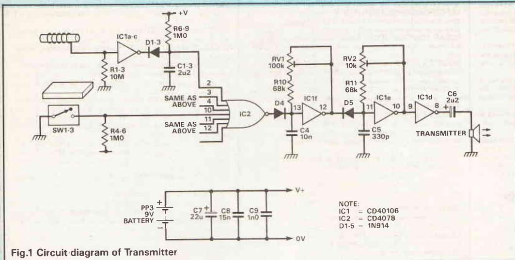
Fig.1 Circuit diagram of Transmitter
