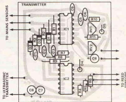
Fig.9 Component overlay of transmitter
