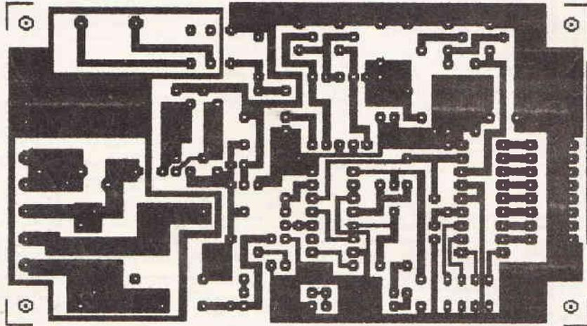
Remote Control Time switch — Receiver board
