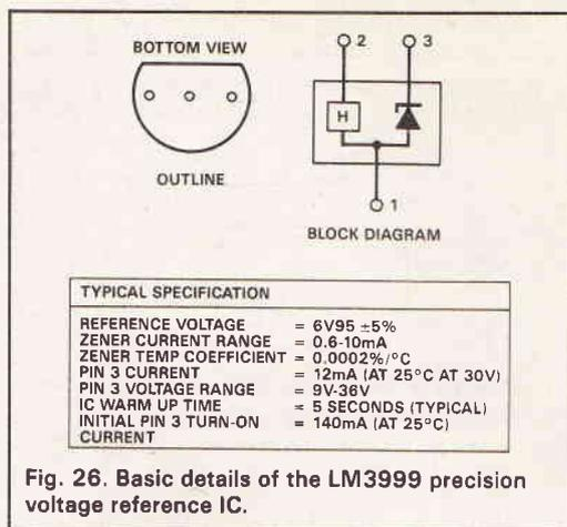
Fig. 26. Basic details of the LM3999 precision voltage reference IC.
