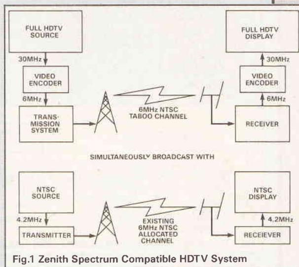
Fig.1 Zenith Spectrum Compatible HDTV System
