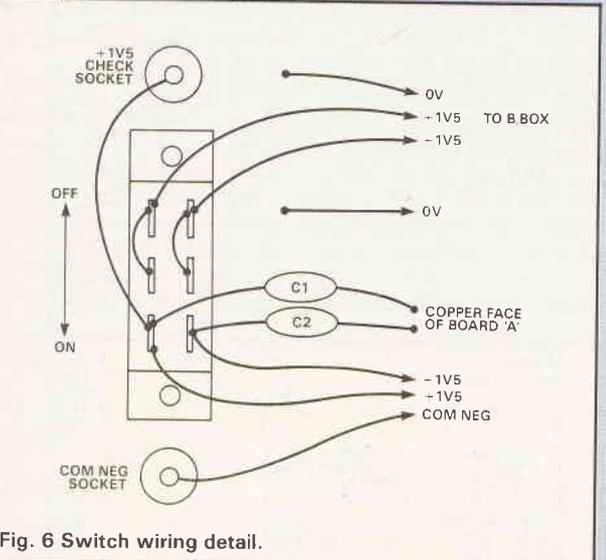
Fig. 6 Switch wiring detail.
