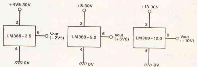
Fig. 17. Basic LM368 voltage-reference application circuits.
