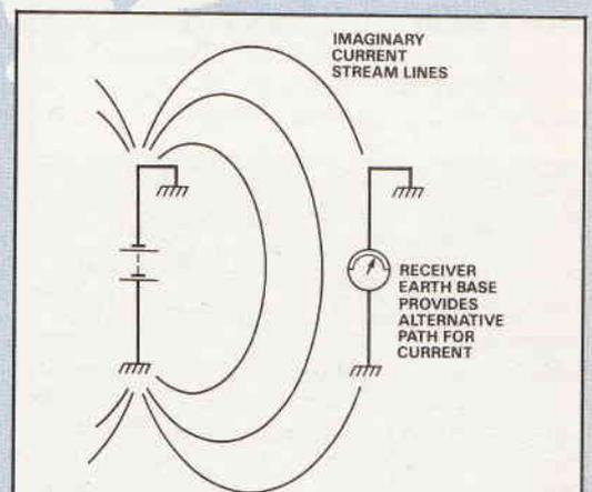
Fig. 2 DC Earth Current Signalling (After Steinheil).
