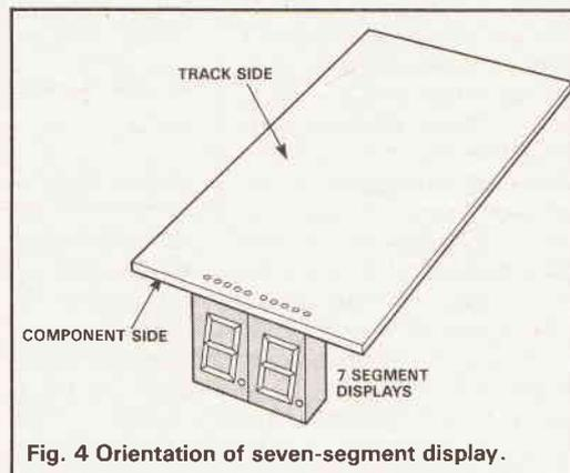
Fig. 4 Orientation of seven-segment display.
