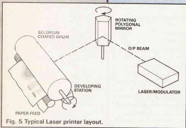
Fig. 5 Typical Laser printer layout.
