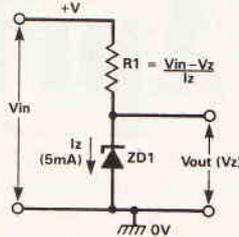
Fig. 1. Basic zener voltage reference circuit.
