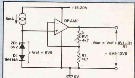
Fig. 4. Precision variable-value voltage-reference generator.
