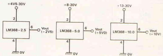
Fig. 17. Basic LM368 voltage-reference application circuits.
