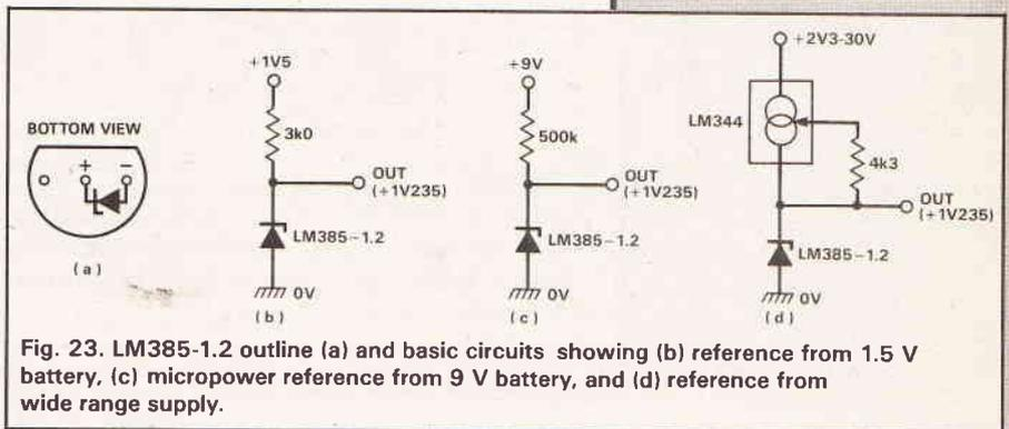
Fig. 23. LM385-1.2 outline (a) and basic circuits showing (b) reference from 1.5 V battery, (c) micropower reference from 9 V battery, and (d) reference from wide range supply.
