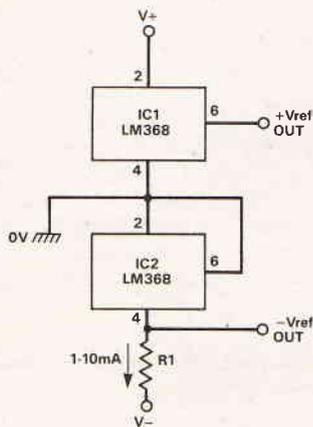
Fig. 21. LM368 dual-polarity voltage reference.
