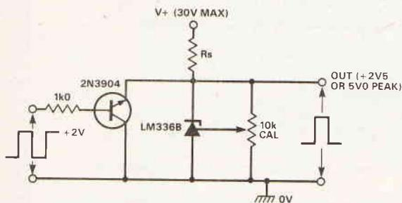
Fig. 16. LM336B-2.5 or -5.0 square wave calibrator circuit.
