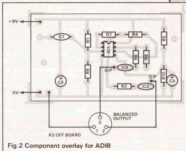
Fig.2 Component overlay for ADIB
