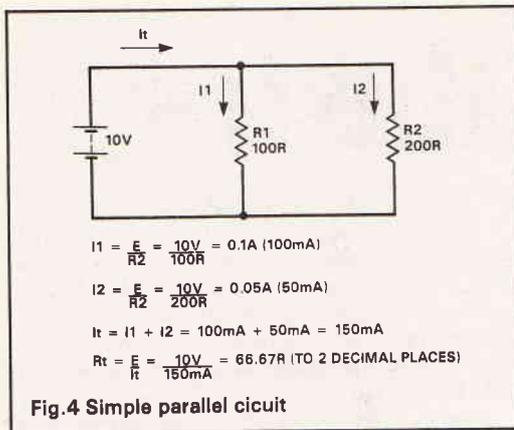
to calculate the total resistance, however. Figure 6 shows how Ohm's Law and Kirchoff's First Law can be used to develop a formula for calculating parallel resistance. This formula can be employed to calculate the total resistance of any number of parallel resistors. A useful point to remember is that if several resistors of the same value are connected in parallel, the total resistance is equal to the value of one resistor divided
