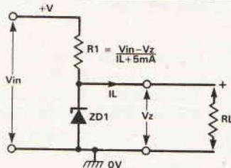
Fig. 2. Basic zener voltage regulator circuit.
