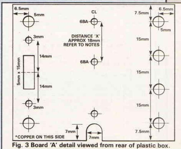
Fig. 3 Board 'A' detail viewed from rear of plastic box.
