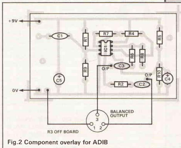
Fig.2 Component overlay for ADIB
