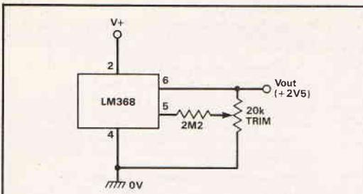
Fig. 19. Narrow-range trimmable ( $\pm 1\%$ ) version of the voltage reference circuit.
