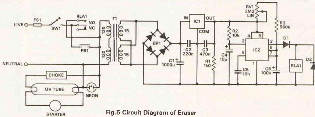
Fig.5 Circuit Diagram of Eraser
