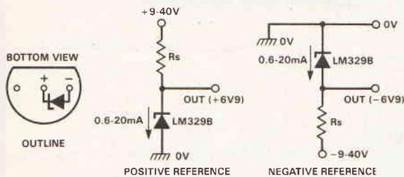
Fig. 10. LM329B outline and basic reference circuits.
