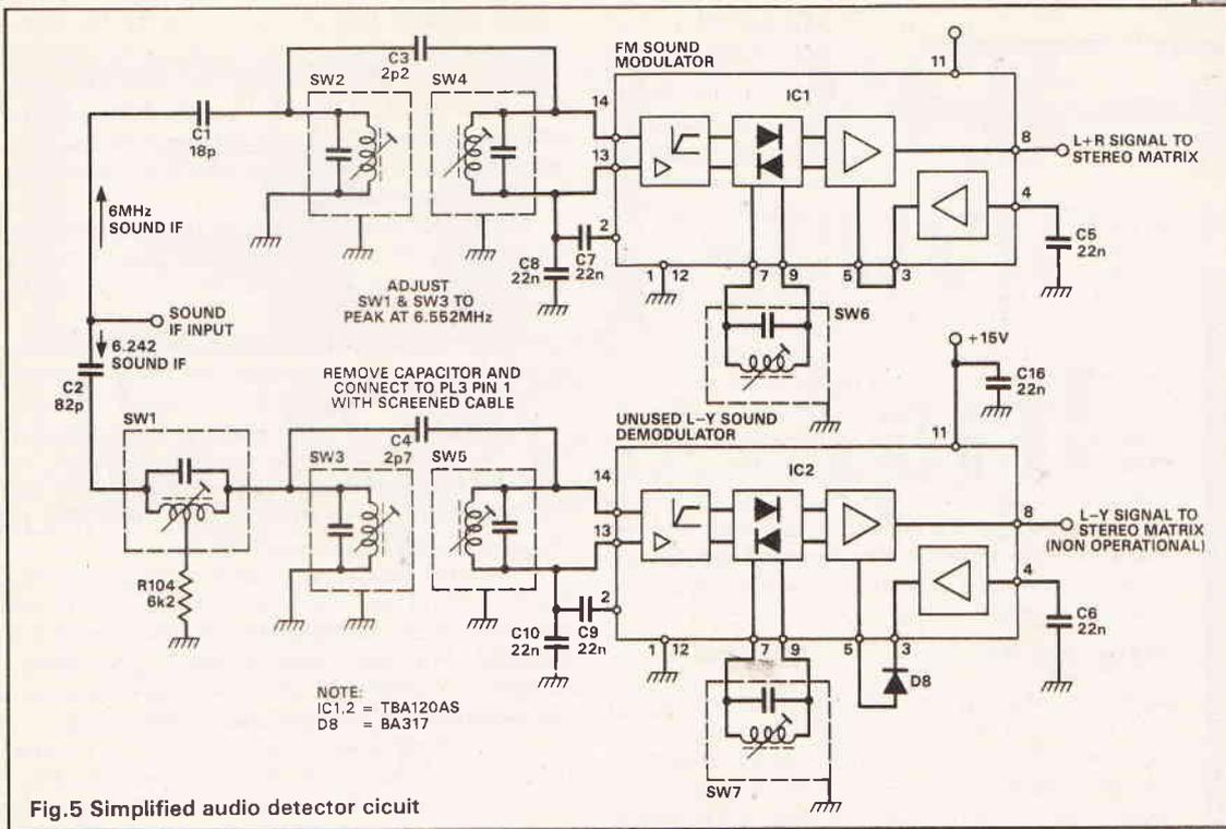
Fig.5 Simplified audio detector circuit
