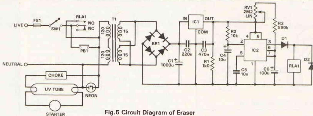
Fig.5 Circuit Diagram of Eraser
