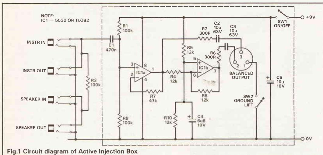
Fig.1 Circuit diagram of Active Injection Box
