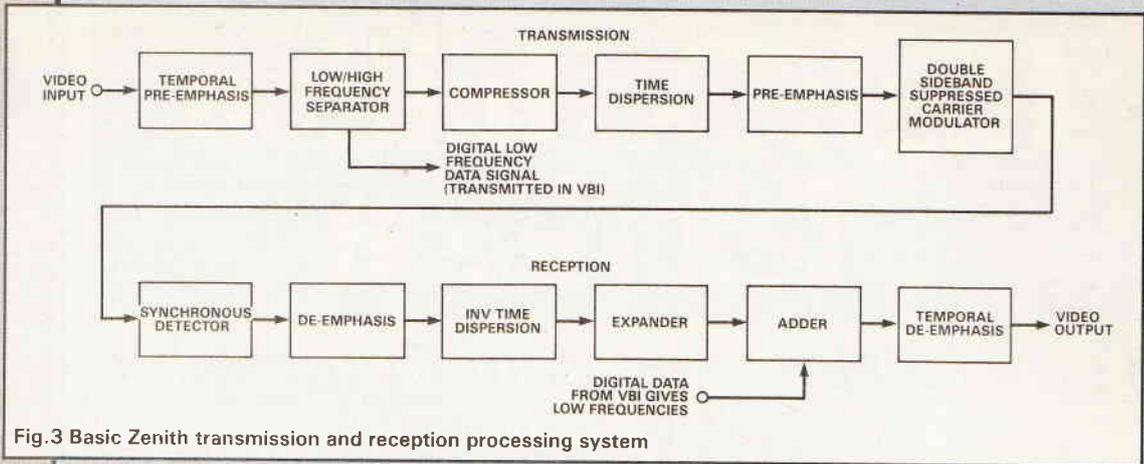
Fig.3 Basic Zenith transmission and reception processing system
