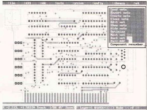
Full analogue, digital and SM support - ground and power planes - 45 degree, arced and any angle tracks with full net-based Design Rule
