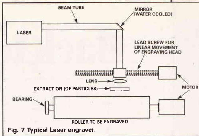
Fig. 7 Typical Laser engraver.
