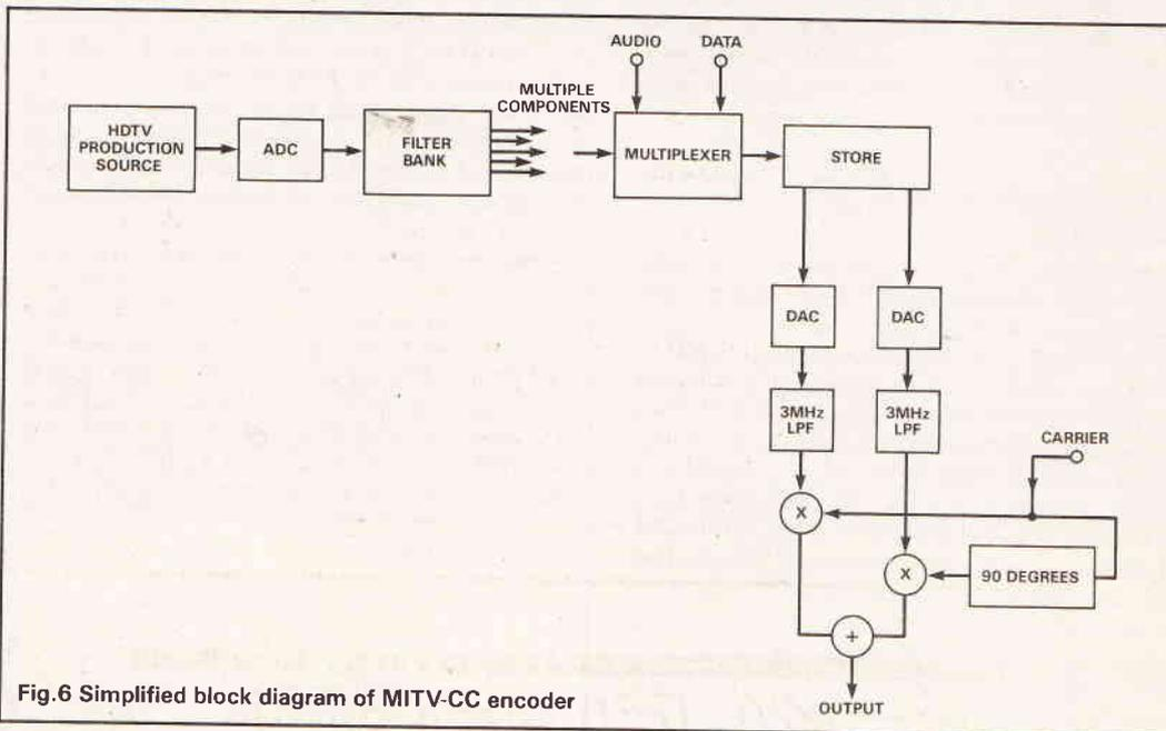
Fig.6 Simplified block diagram of MITV-CC encoder
