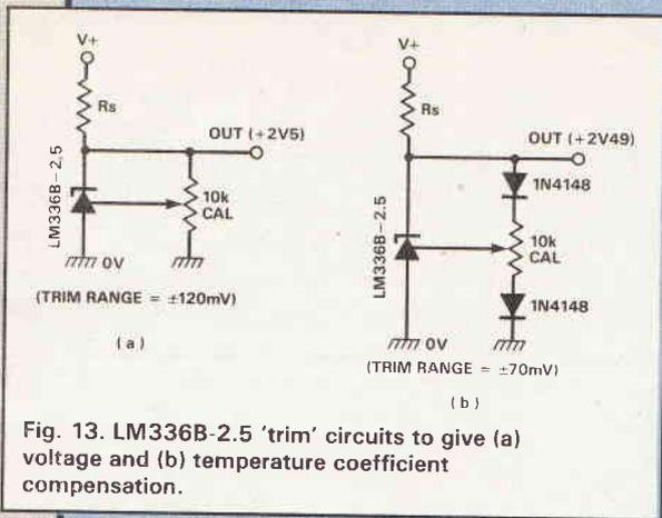
Fig. 13. LM336B-2.5 'trim' circuits to give (a) voltage and (b) temperature coefficient compensation.
