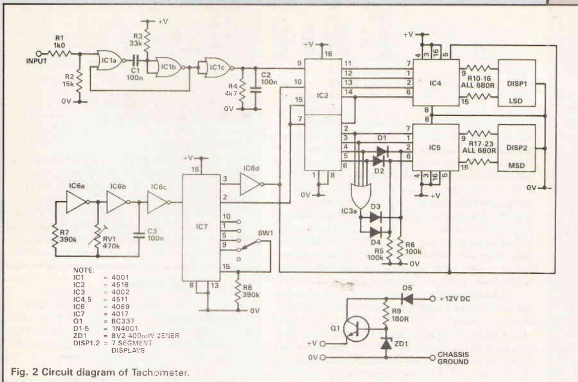
Fig. 2 Circuit diagram of Tachometer.
