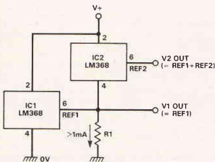
Fig. 22. LM368 multiple voltage reference.
