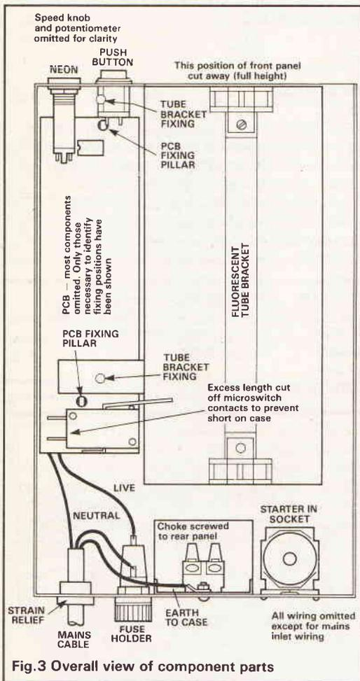
Fig. 3 Overall view of component parts
