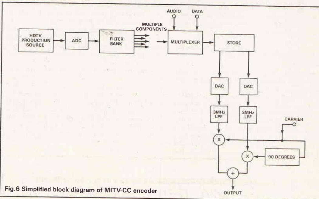
Fig.6 Simplified block diagram of MITV-CC encoder
