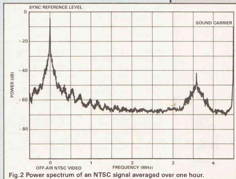
Fig.2 Power spectrum of an NTSC signal averaged over one hour.
