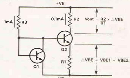
Fig. 5. Basic  $\Delta V_{BE}$  voltage-reference generator.
