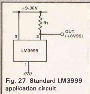
Fig. 27. Standard LM3999 application circuit.
