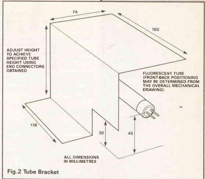
Fig. 2 Tube Bracket
