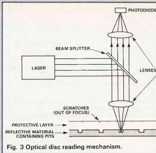
Fig. 3 Optical disc reading mechanism.
