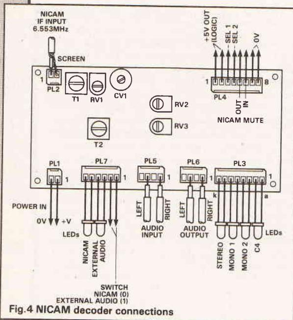
Fig.4 NICAM decoder connections
