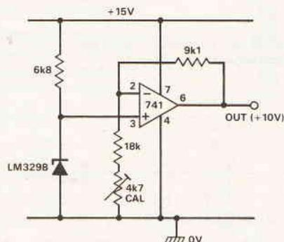
Fig. 11. Buffered 10.0V reference with single-ended supply.
