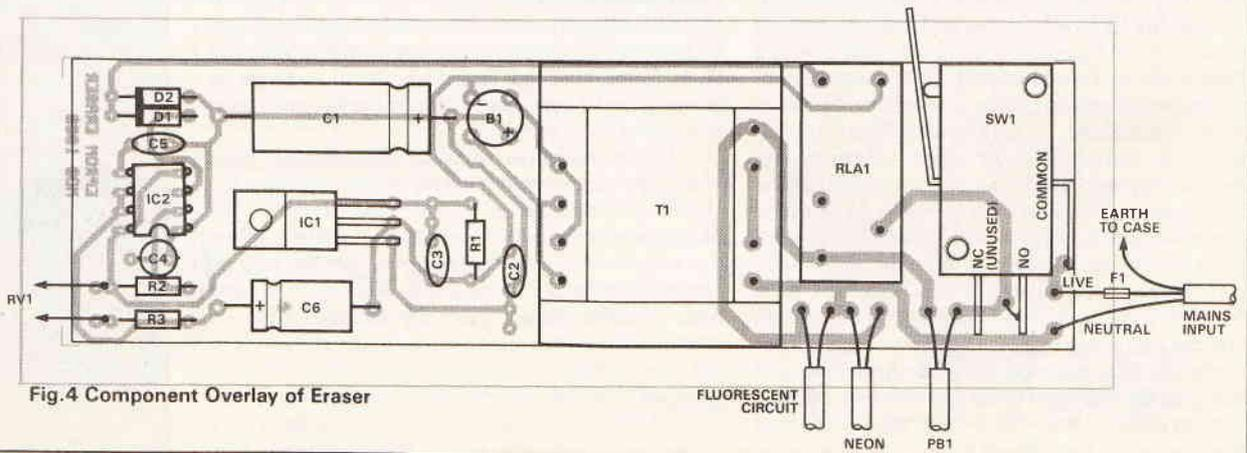
Fig.4 Component Overlay of Eraser
