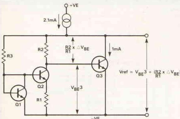
Fig. 8. Simple band-gap voltage-reference circuit.
