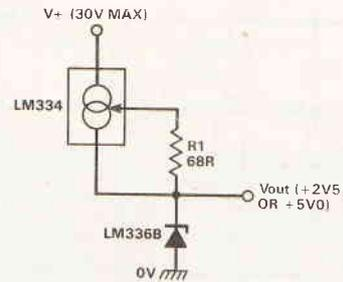
Fig. 15. LM336B-2.5 or -5.0 voltage reference, using wide supply voltage range.
