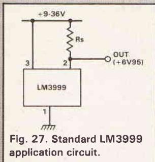
Fig. 27. Standard LM3999 application circuit.
