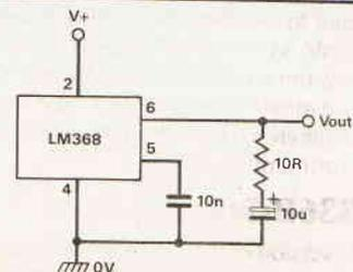
Fig. 18. Low-noise version of the voltage reference circuits.
