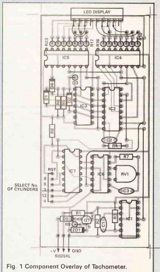
Fig. 1 Component Overlay of Tachometer.
