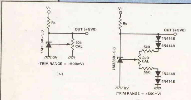
Fig. 14. LM336B-5.0 'trim' circuits to give (a) voltage and (b) temperature coefficient compensation.
