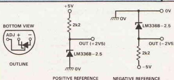
Fig. 12. LM336B-2.5 outline and basic reference circuits.
