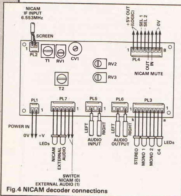
Fig.4 NICAM decoder connections
