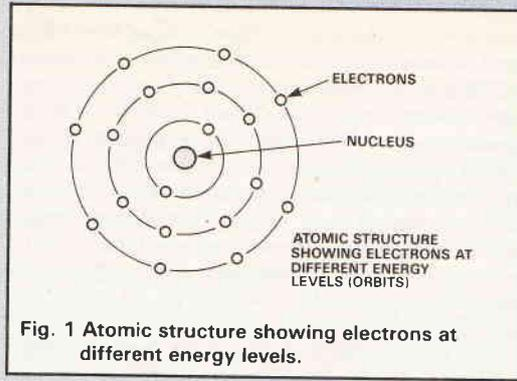
**Fig. 1 Atomic structure showing electrons at different energy levels.**
