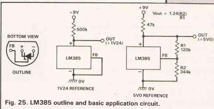
Fig. 25. LM385 outline and basic application circuit.
