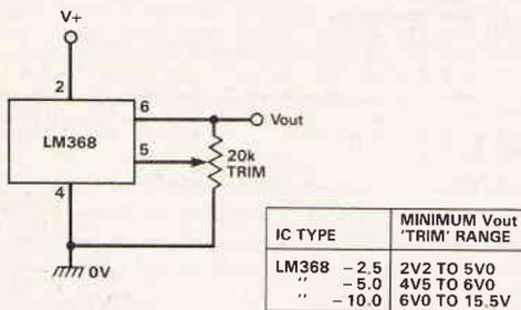
Fig. 20. Wide-range trimmable version of the LM368 voltage reference circuit.
