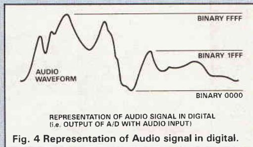
Fig. 4 Representation of Audio signal in digital.
