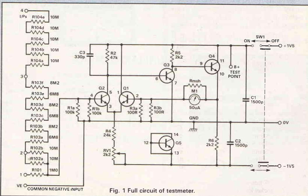
Fig. 1 Full circuit of testmeter.
