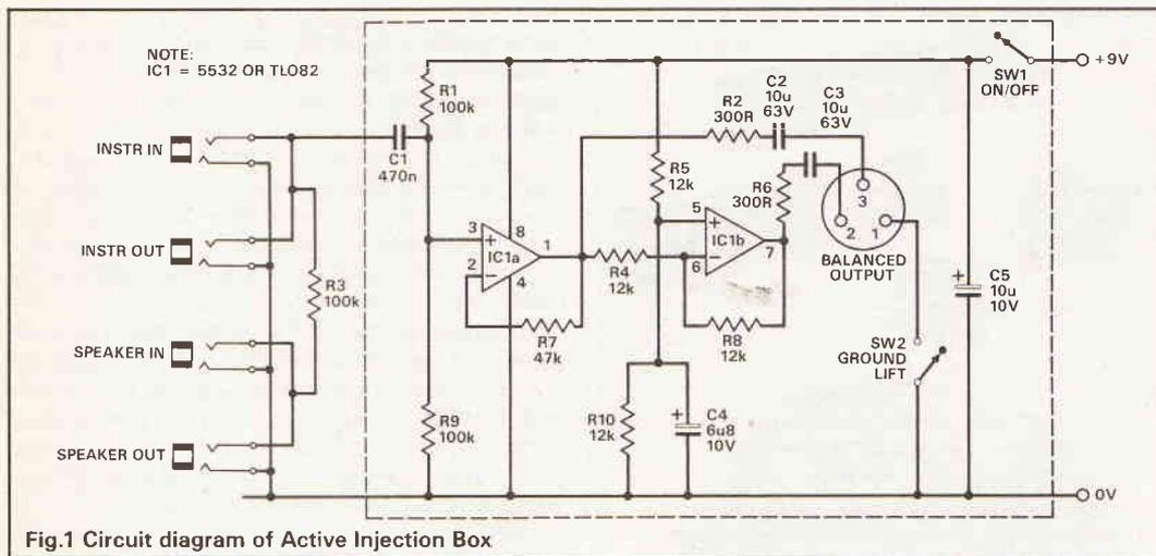
Fig.1 Circuit diagram of Active Injection Box
