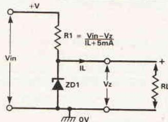
Fig. 2. Basic zener voltage regulator circuit.
