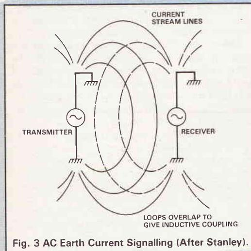
Fig. 3 AC Earth Current Signalling (After Stanley).
