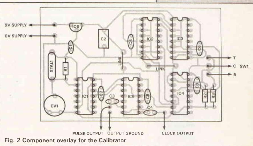
Fig. 2 Component overlay for the Calibrator
