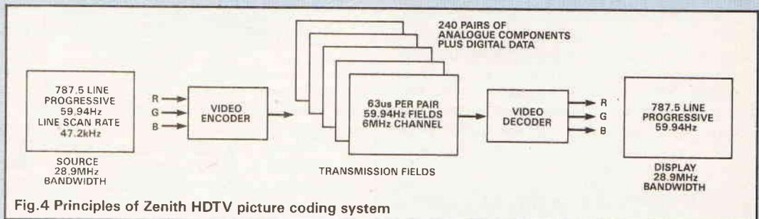
Fig.4 Principles of Zenith HDTV picture coding system
