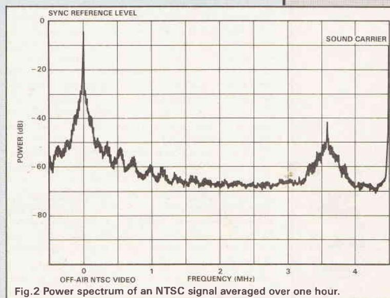
Fig.2 Power spectrum of an NTSC signal averaged over one hour.
