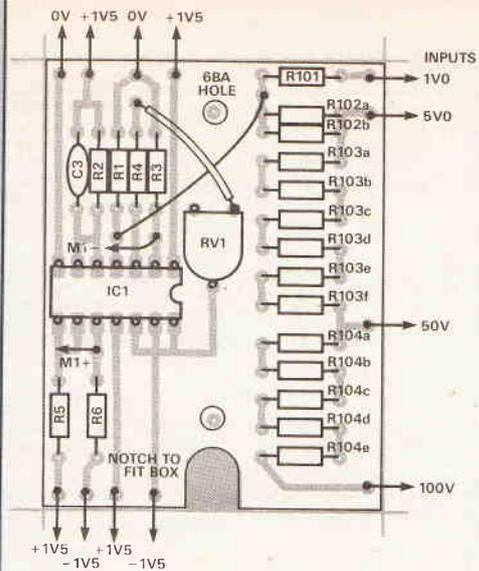
Fig. 4 Component Overlay for Testmeter.
