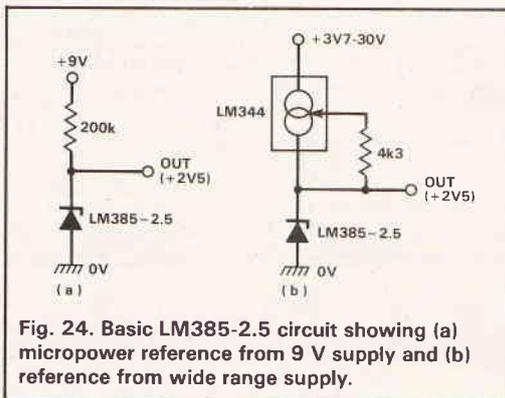
Fig. 24. Basic LM385-2.5 circuit showing (a) micropower reference from 9 V supply and (b) reference from wide range supply.
