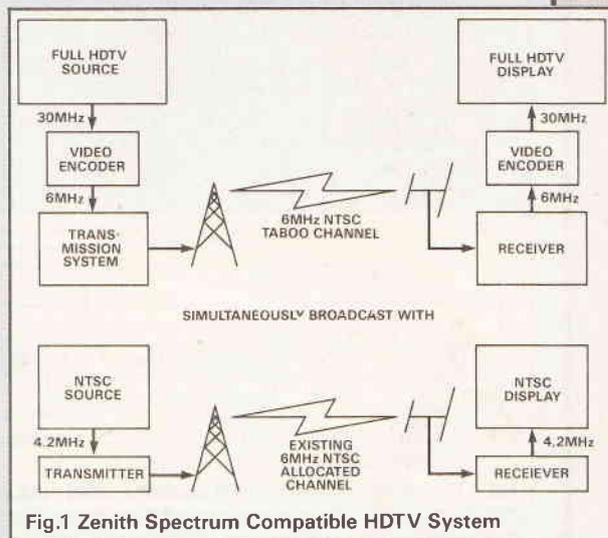
Fig.1 Zenith Spectrum Compatible HDTV System
