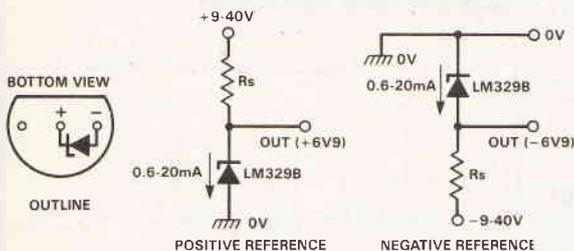
Fig. 10. LM329B outline and basic reference circuits.
