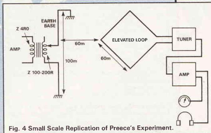
Fig. 4 Small Scale Replication of Preece's Experiment.
