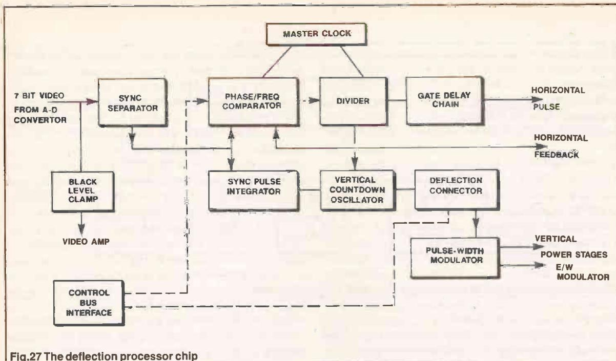
Fig.27 The deflection processor chip
