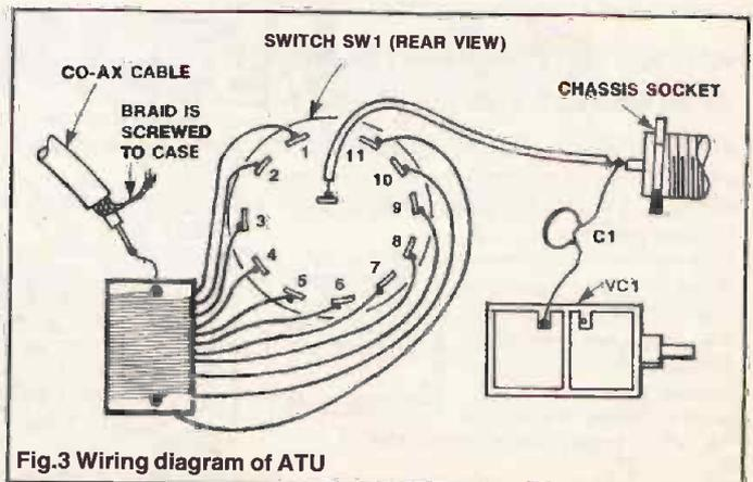
Fig.3 Wiring diagram of ATU
