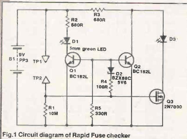
Fig.1 Circuit diagram of Rapid Fuse checker
