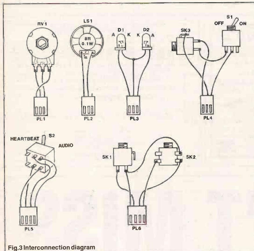
Fig.3 Interconnection diagram
