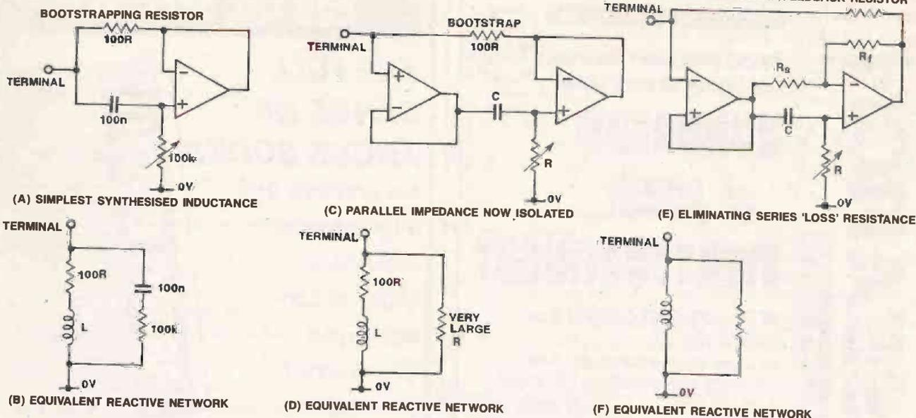
Fig.1 Synthesising the reactive properties of an inductor using 'bootstrapping techniques'
