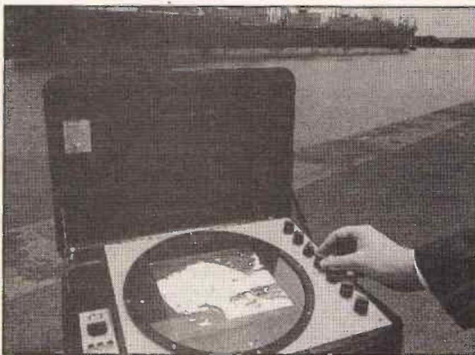
Using conventional telephone lines, a new portable navigation system will provide harbours with the facilities of conventional radar systems at a fraction of the usual cost. Marine pilots will now be able to view raw images transmitted from shore based radar stations independent of the ships own systems.
