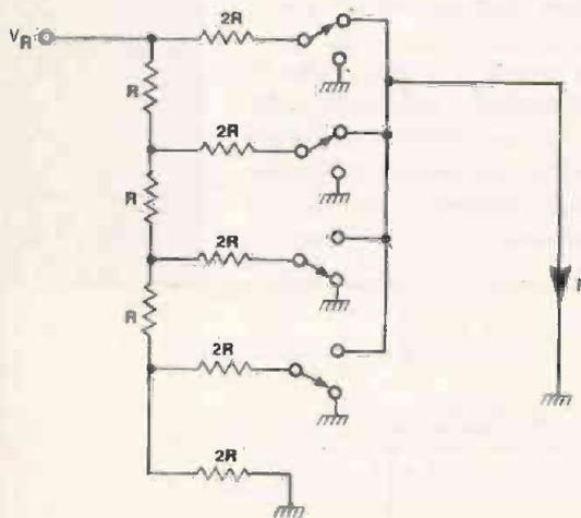
Fig.26 Principles of a digital to analogue convertor
