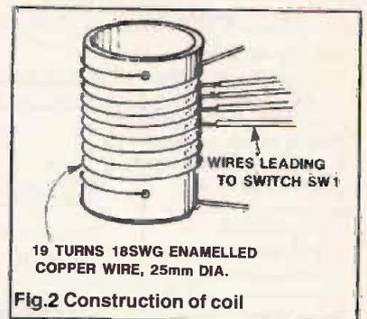
Fig.2 Construction of coil
