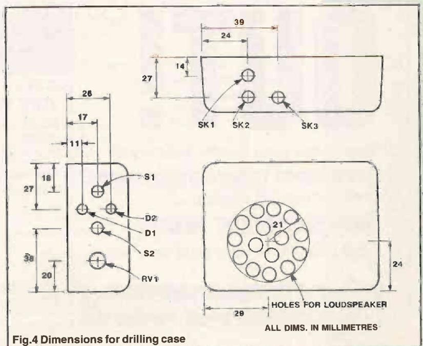
Fig.4 Dimensions for drilling case
