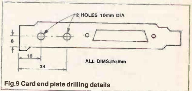
Fig.9 Card end plate drilling details
