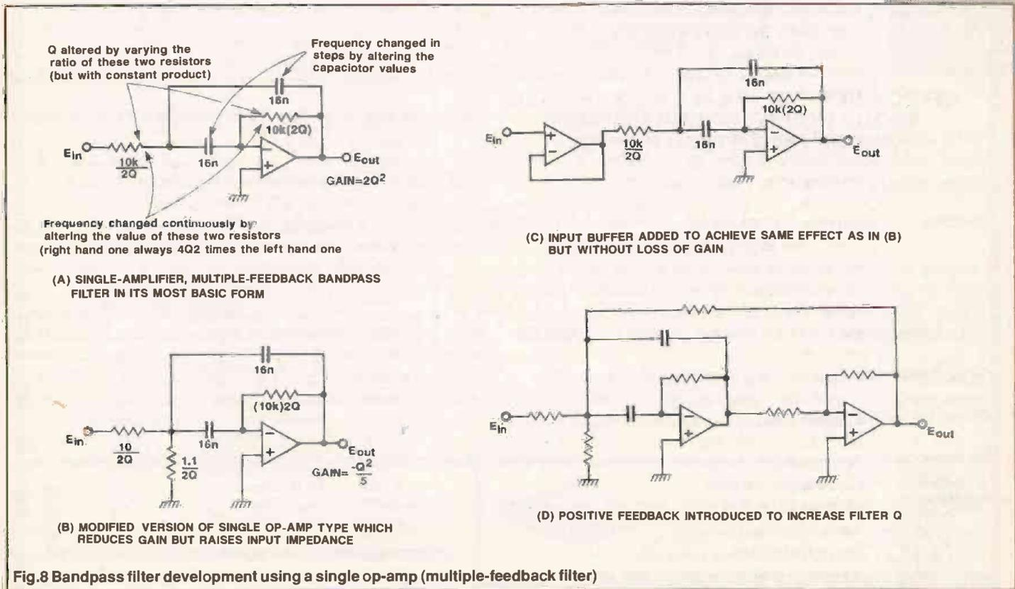
Fig.8 Bandpass filter development using a single op-amp (multiple-feedback filter)
