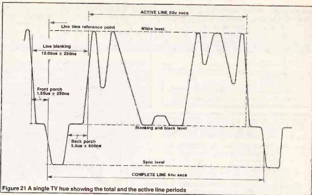
Figure 21 A single TV line showing the total and the active line periods
