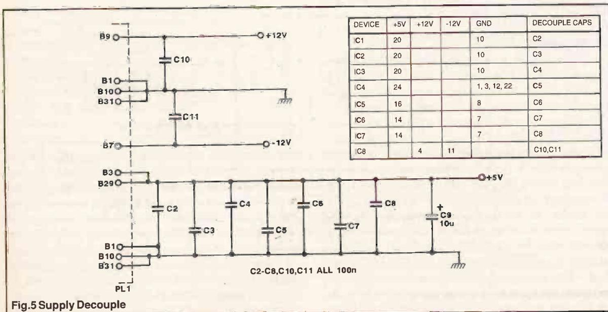
Fig.5 Supply Decouple
