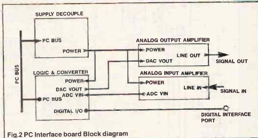
Fig.2 PC Interface board Block diagram
