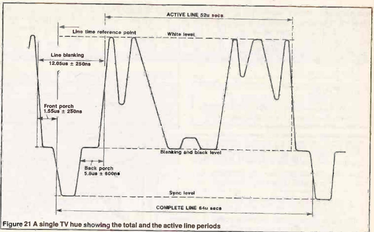
Figure 21 A single TV line showing the total and the active line periods
