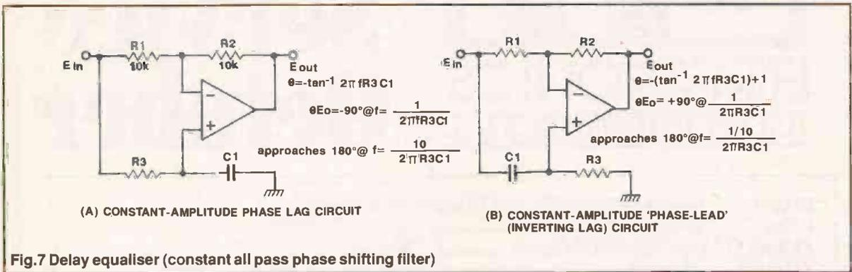
Fig.7 Delay equaliser (constant all pass phase shifting filter)
