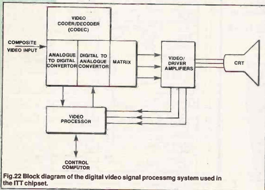
Fig.22 Block diagram of the digital video signal processing system used in the ITT chipset.
