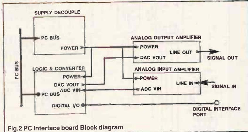
Fig.2 PC Interface board Block diagram
