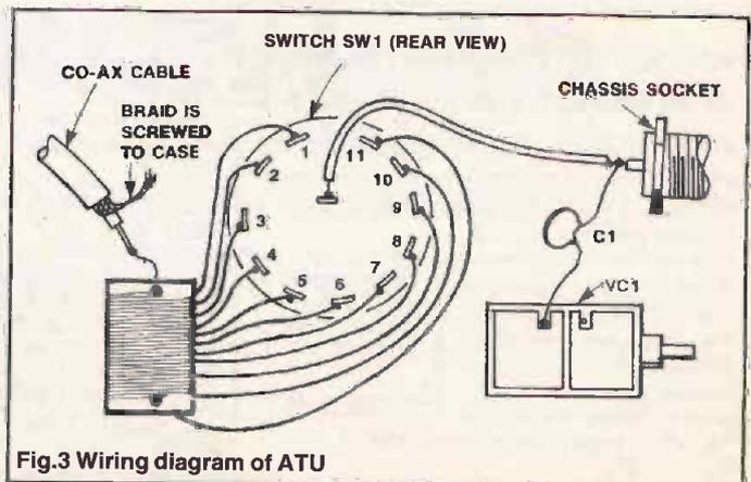
Fig. 3 Wiring diagram of ATU
