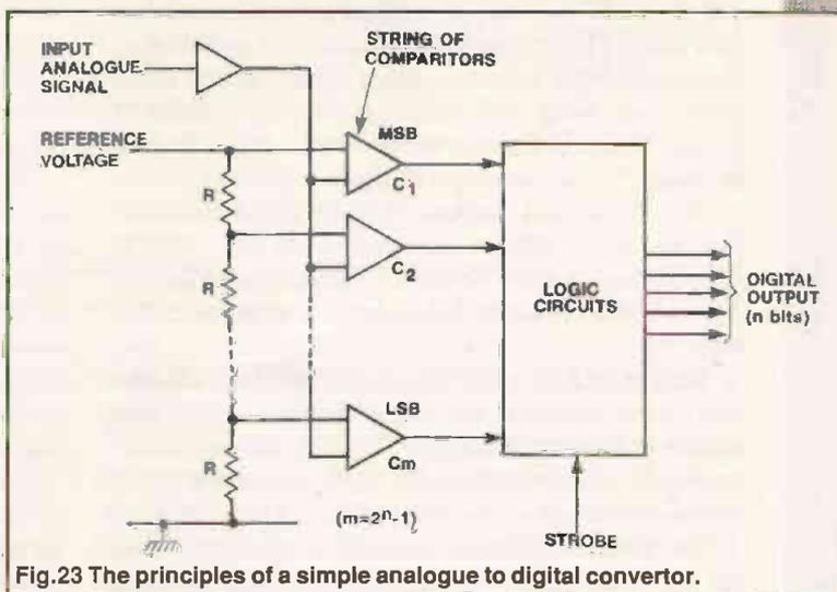
Fig.23 The principles of a simple analogue to digital convertor.
