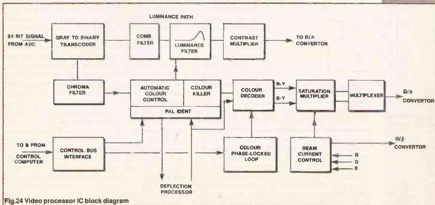
Fig.24 Video processor IC block diagram
