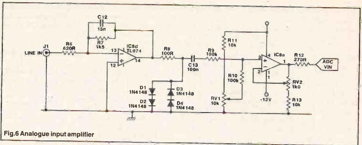
Fig.6 Analogue input amplifier
