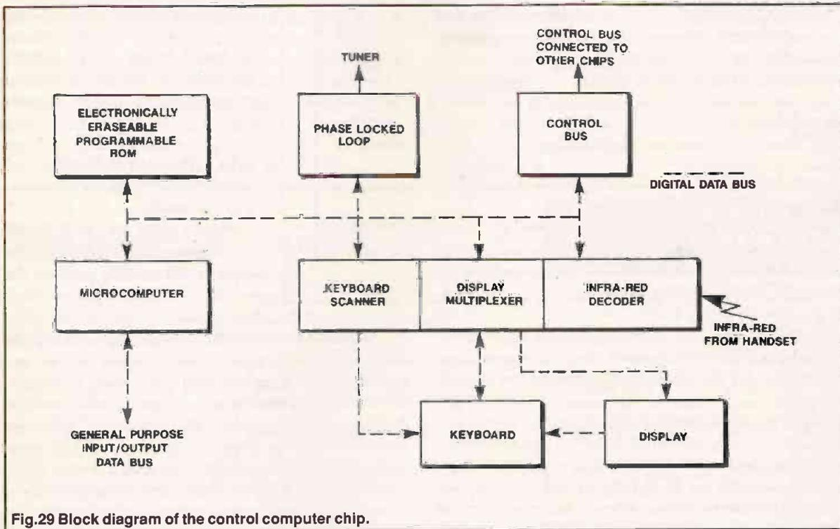
Fig.29 Block diagram of the control computer chip.
