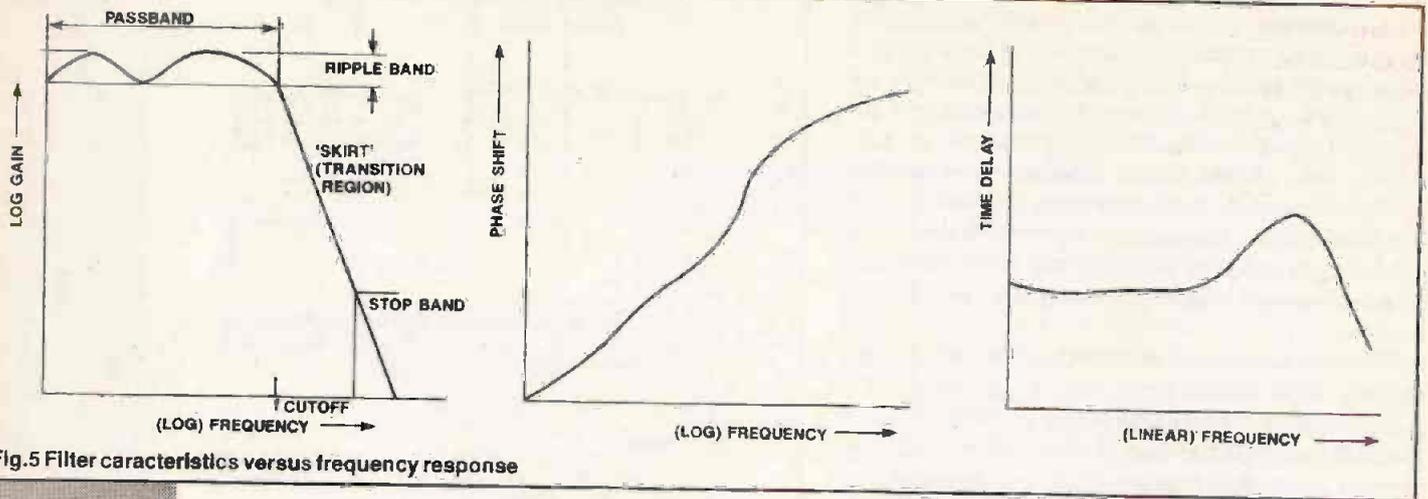
Fig.5 Filter characteristics versus frequency response
