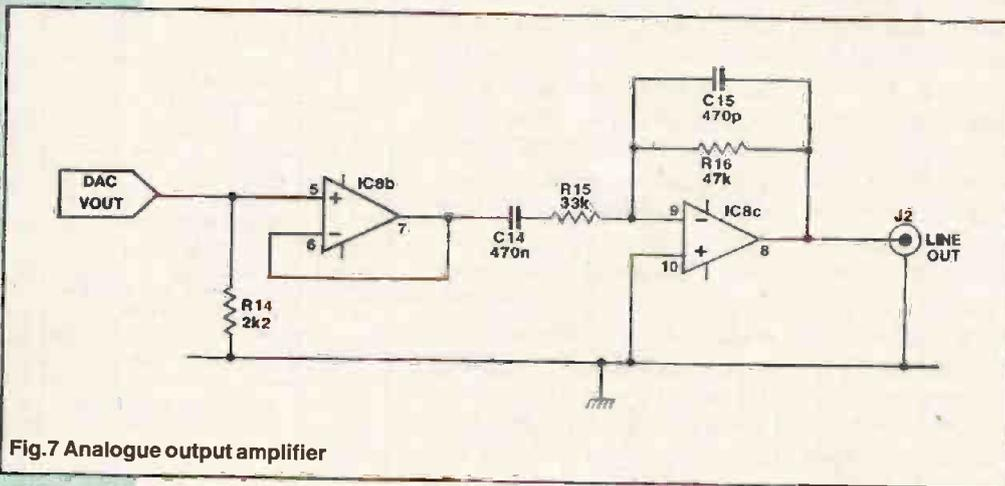
Fig.7 Analogue output amplifier
