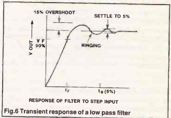
Fig.6 Transient response of a low pass filter
