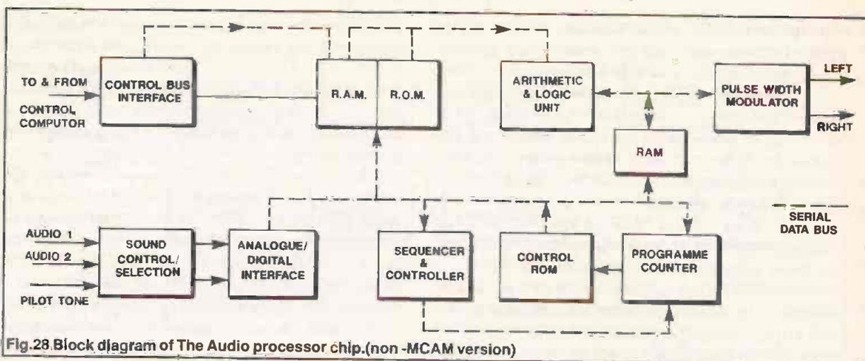
Fig.28 Block diagram of The Audio processor chip.(non -MCAM version)
