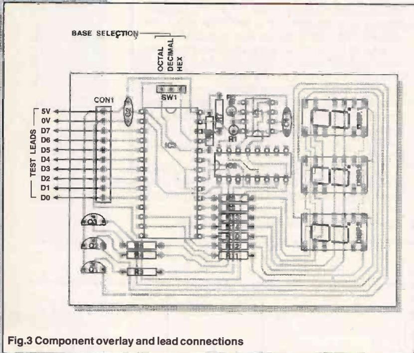
Fig. 3 Component overlay and lead connections
