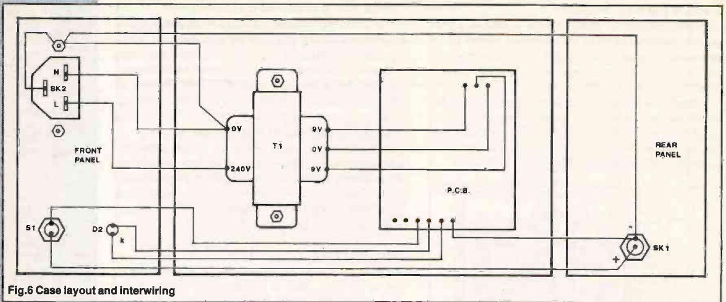
Fig. 6 Case layout and interwiring
