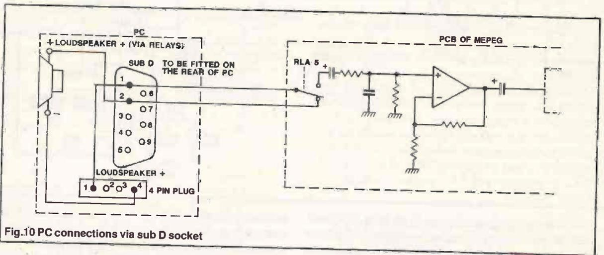
Fig.10 PC connections via sub D socket
