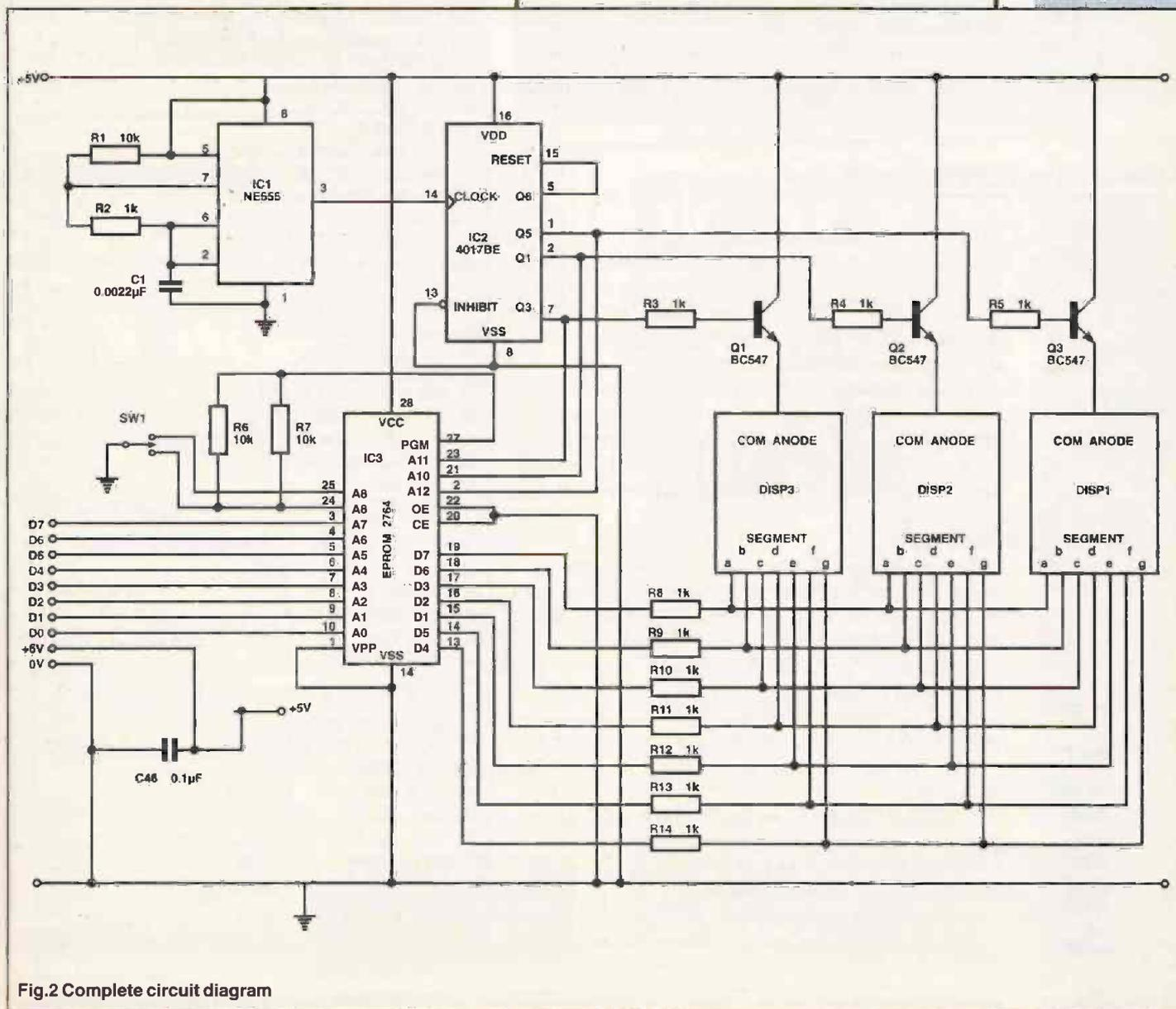
Fig.2 Complete circuit diagram
