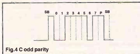
Fig.4 C odd parity
