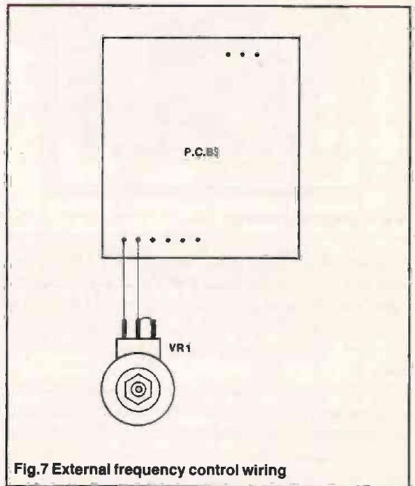
Fig. 7 External frequency control wiring
