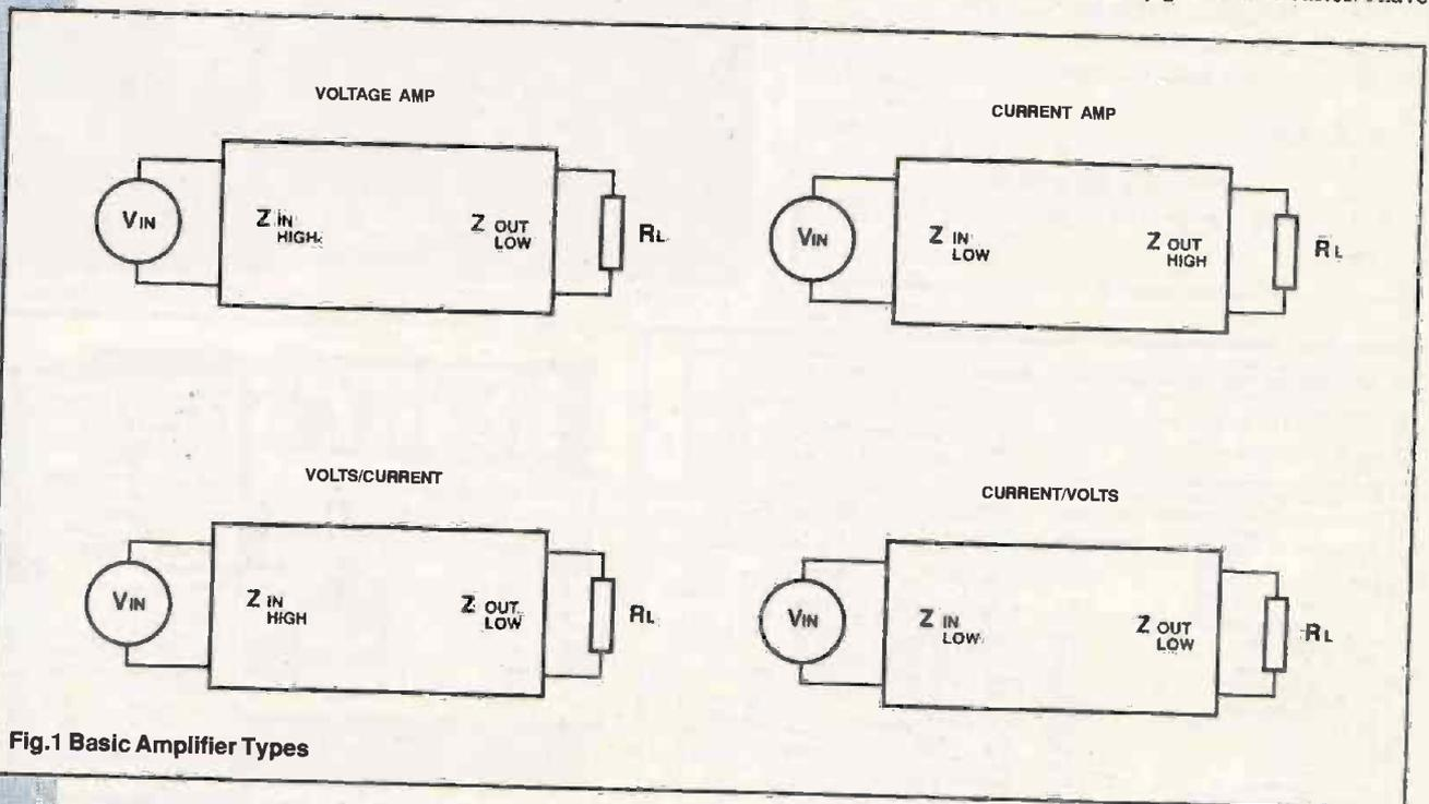
Fig.1 Basic Amplifier Types
