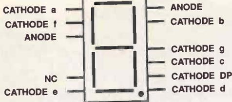
Fig.5 Display Pinouts
