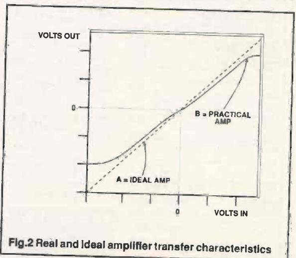
Fig.2 Real and Ideal amplifier transfer characteristics
