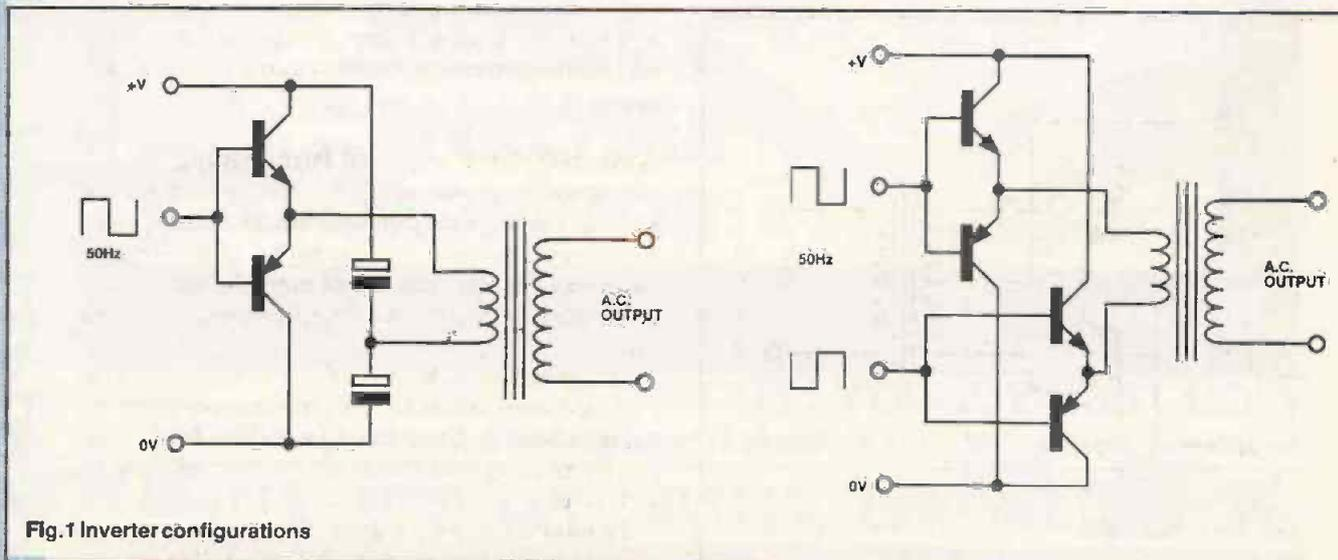
Fig. 1 Inverter configurations
