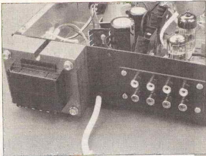
DC blocking capacitor C2. A good quality polypropylene type is used here for its wide frequency response.
