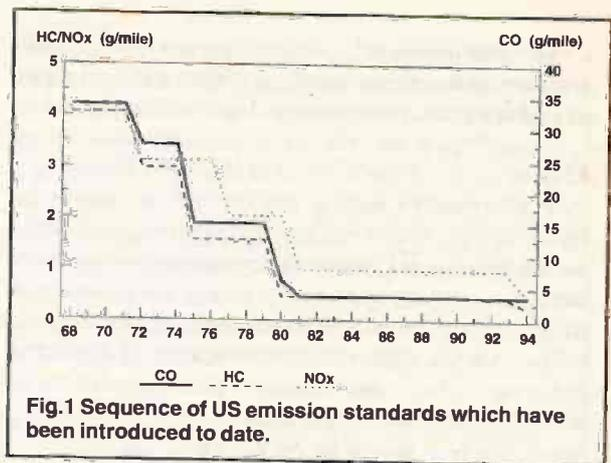
Fig.1 Sequence of US emission standards which have been introduced to date.
