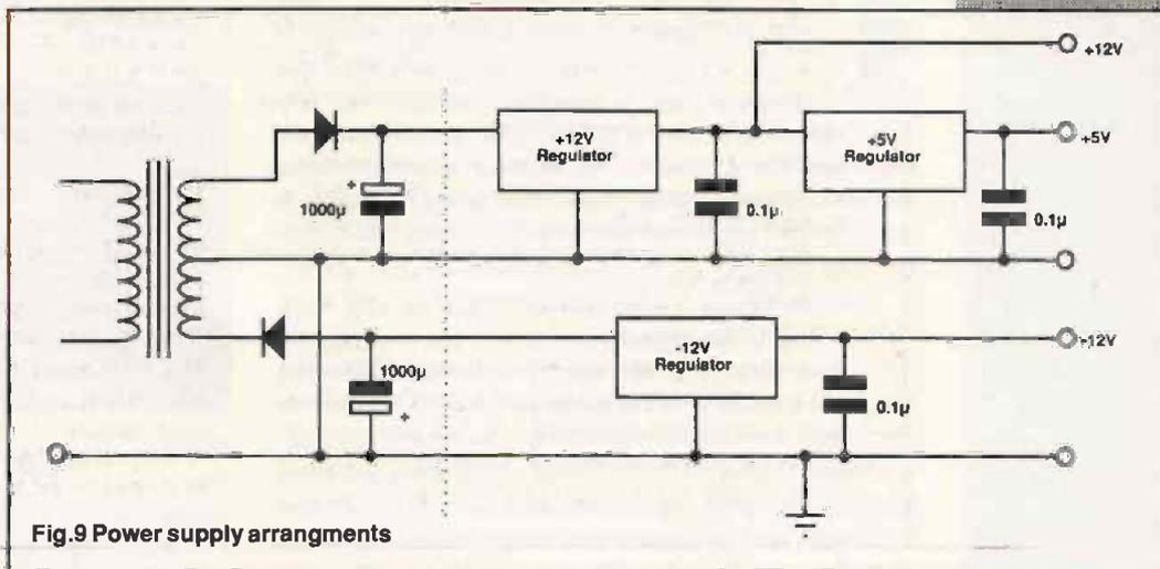
Fig.9 Power supply arrangements
