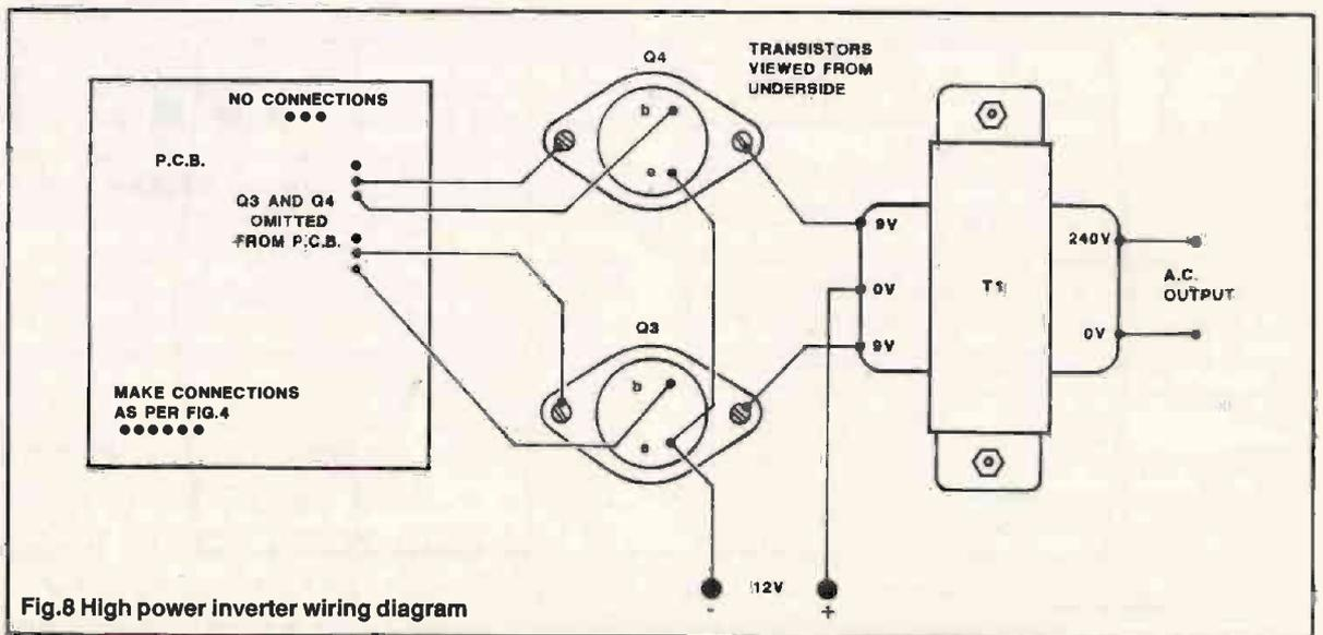
Fig. 8 High power inverter wiring diagram
