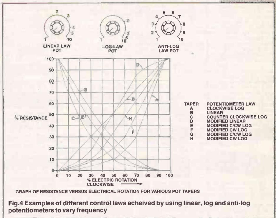
Fig.4 Examples of different control laws achieved by using linear, log and anti-log potentiometers to vary frequency
