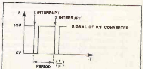
Fig. 9 Input signal as a proportional frequency
