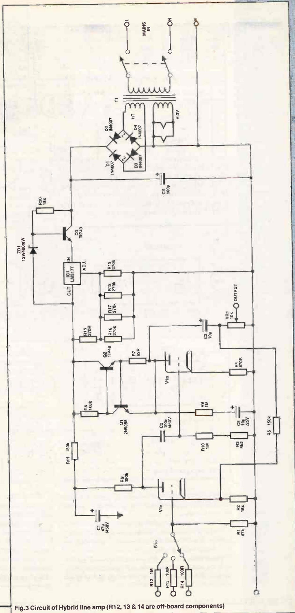
Fig.3 Circuit of Hybrid line amp (R12, 13 & 14 are off-board components)
