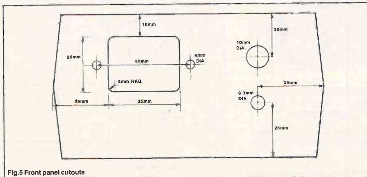
Fig. 5 Front panel cutouts
