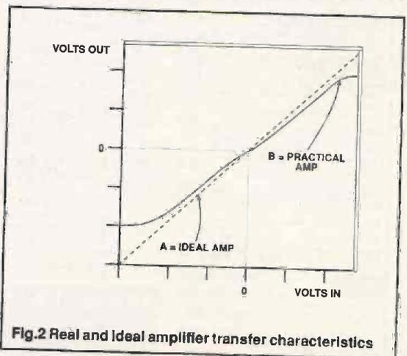
Fig.2 Real and Ideal amplifier transfer characteristics
