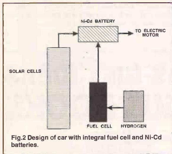
Fig.2 Design of car with integral fuel cell and Ni-Cd batteries.
