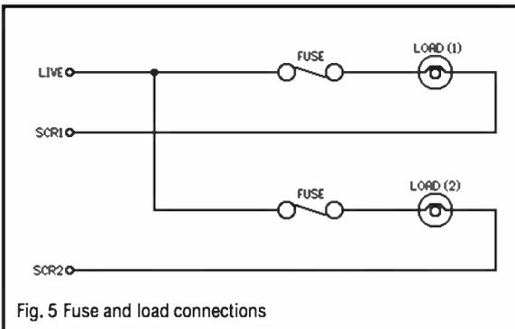
Fig. 5 Fuse and load connections
