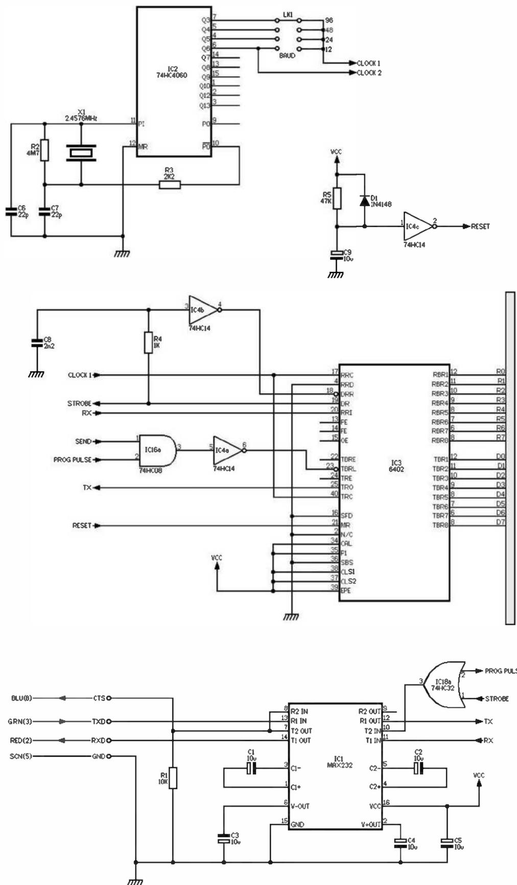
Fig. 1 Serial Interface Circuits
