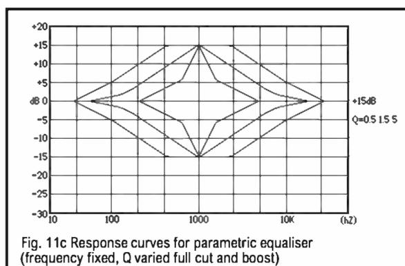
Fig. 11c Response curves for parametric equaliser (frequency fixed, Q varied full cut and boost)
