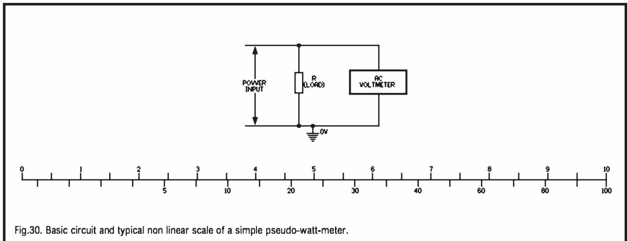
Fig.30. Basic circuit and typical non linear scale of a simple pseudo-watt-meter.
