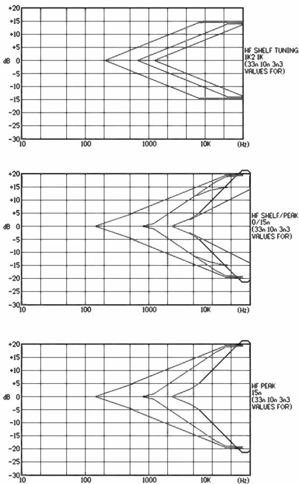
Fig 13a HF Equaliser response curves (Frequency tuning)
