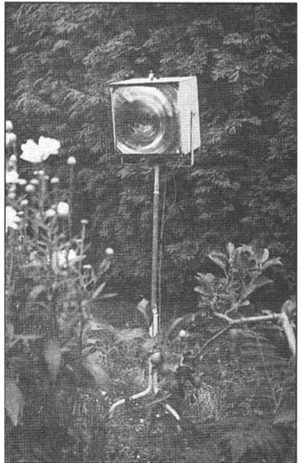
Plop, whine, click, growl, buzz, (deep and high) and other such sounds are the sort of signals that can be heard on the headphones plugged into a Macro Heliography receiver. These signals are the result of sunlight being reflected from the shiny membrane, comprising the wing or wings, of a flying insect, much like the heliography used at sea.
