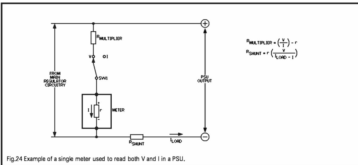
Fig.24 Example of a single meter used to read both V and I in a PSU.
