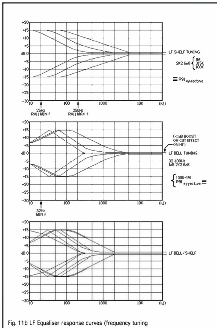
Fig. 11b LF Equaliser response curves (frequency tuning)
