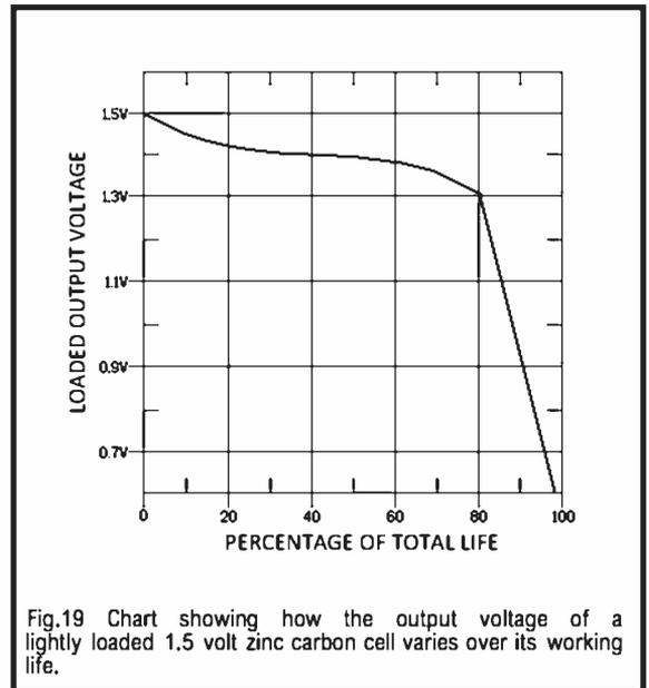
Fig.19 Chart showing how the output voltage of a lightly loaded 1.5 volt zinc carbon cell varies over its working life.
