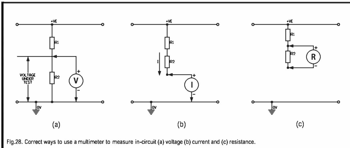
Fig.28. Correct ways to use a multimeter to measure in-circuit (a) voltage (b) current and (c) resistance.
