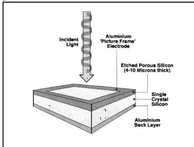
commercially available silicon photo diodes, but without needing an anti-reflection coating.
