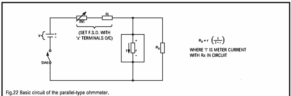
Fig.22 Basic circuit of the parallel-type ohmmeter.
