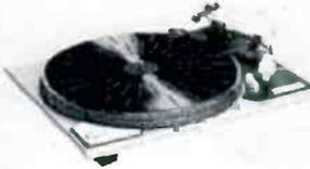
\* Manual arm \* Steel chassis \* Electronic speed control 33 & 45 R.P.M. \* Vari pitch control \* High torque servo driven DC motor \* Transit screws \* 12" die cast platter \* Neon strobe \* Calibrated balance weight \* Removable head shell \* 1/2" cartridge fixings \* Cue lever \* 220/240V 50/60Hz \* 390x305mm \* Supplied with mounting cut-out template.
