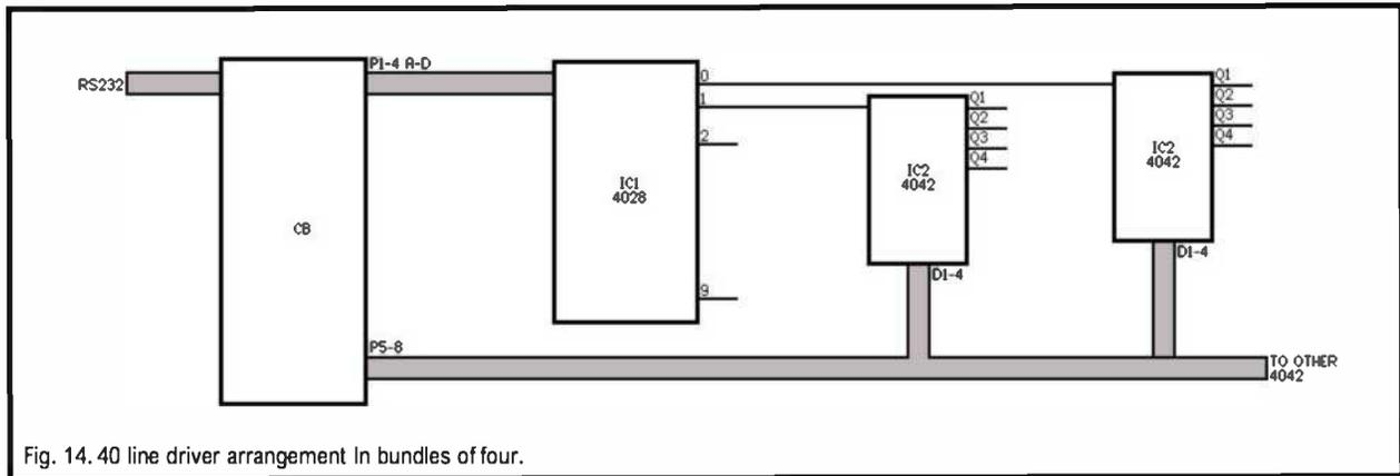
Fig. 14. 40 line driver arrangement in bundles of four.
