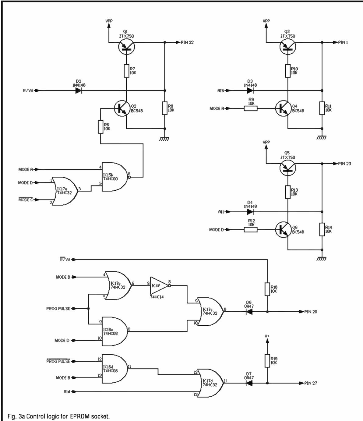
Fig. 3a Control logic for EPROM socket.
