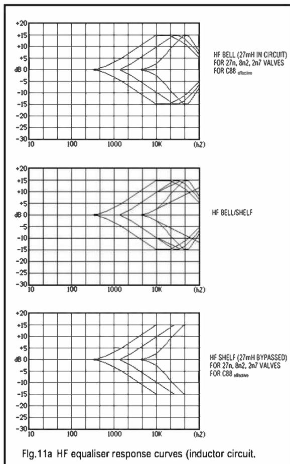
Fig.11a HF equaliser response curves (inductor circuit).
