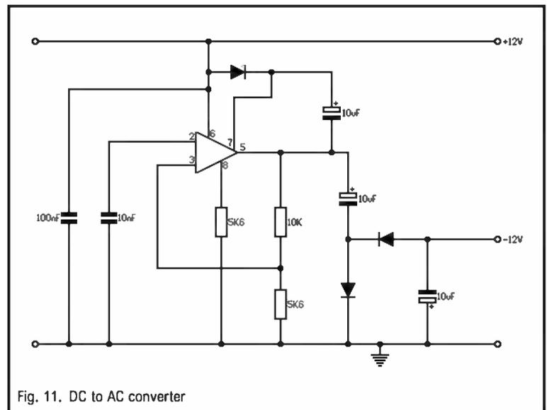
Fig. 11. DC to AC converter
