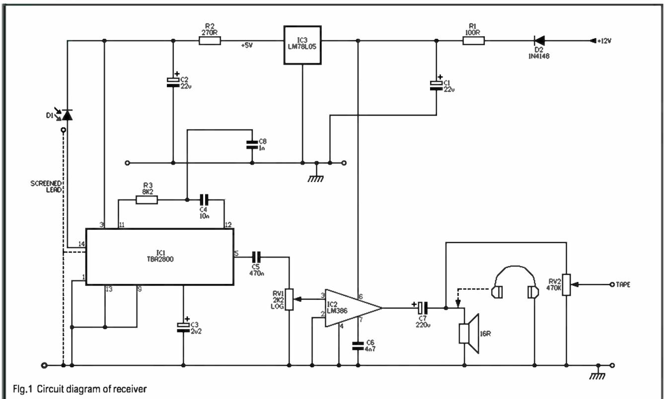
Fig.1 Circuit diagram of receiver
