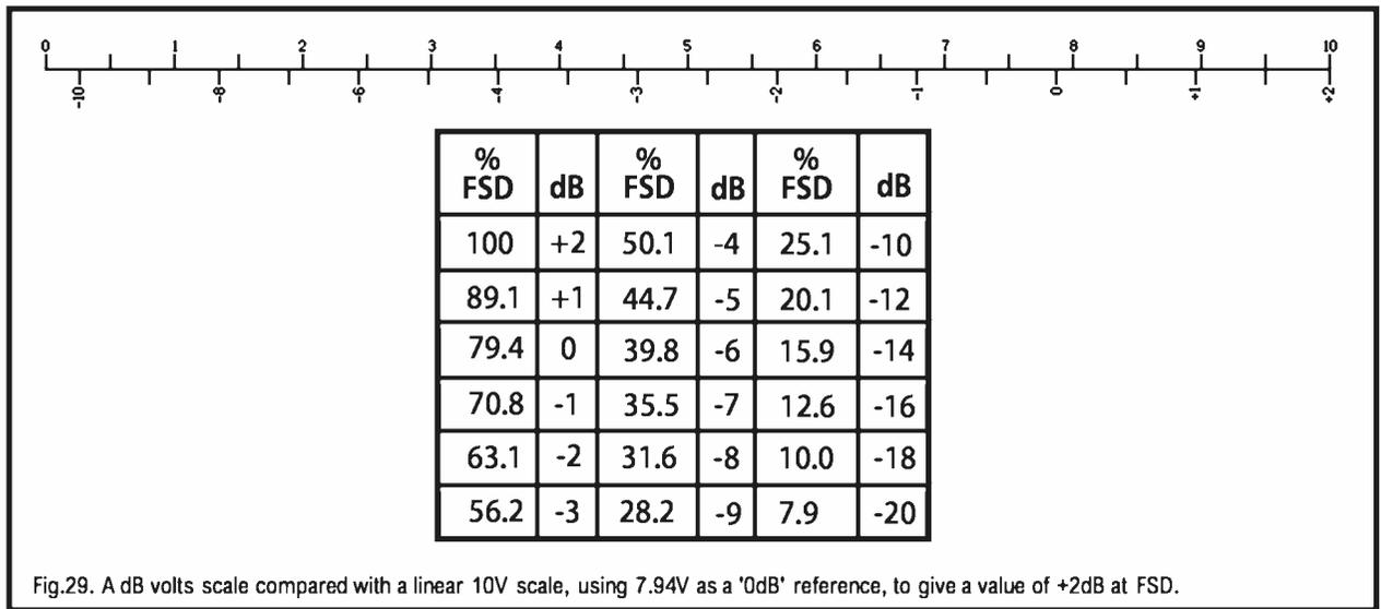
Fig.29. A dB volts scale compared with a linear 10V scale, using 7.94V as a '0dB' reference, to give a value of +2dB at FSD.
