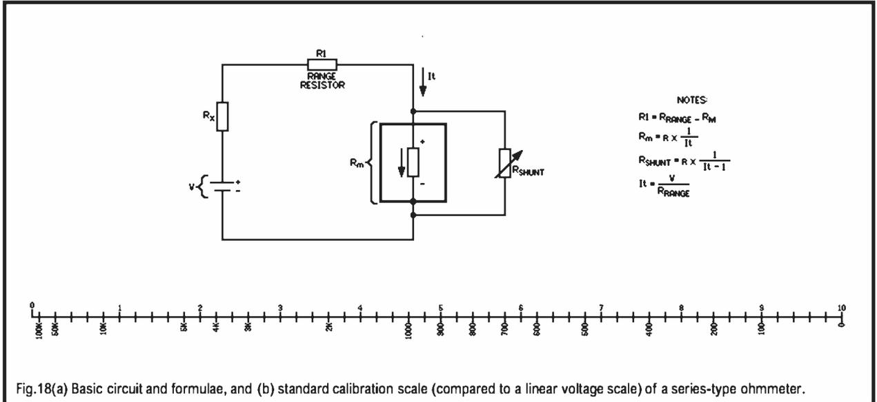
Fig.18(a) Basic circuit and formulae, and (b) standard calibration scale (compared to a linear voltage scale) of a series-type ohmmeter.
