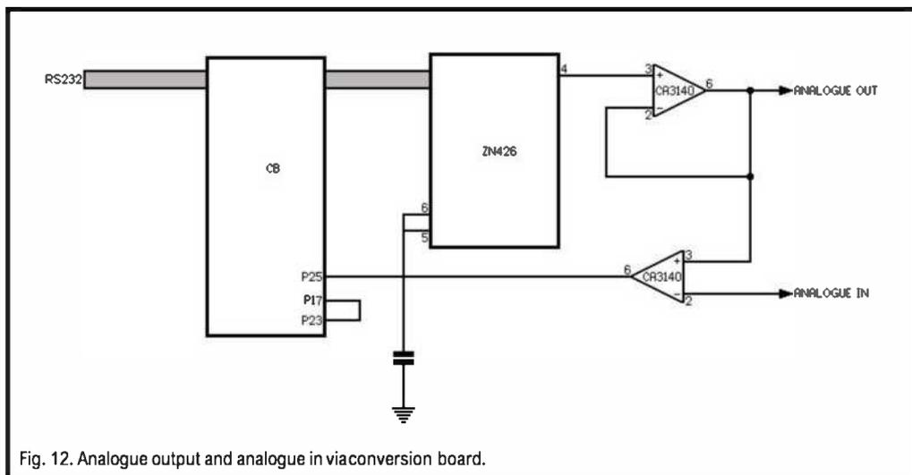
Fig. 12. Analogue output and analogue in via conversion board.
