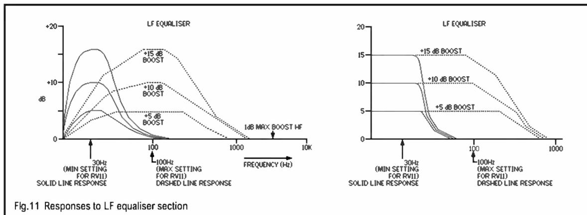
Fig.11 Responses to LF equaliser section
