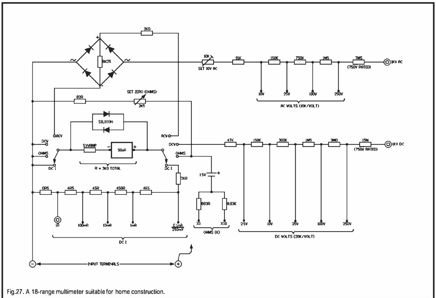
Fig.27. A 18-range multimeter suitable for home construction.
