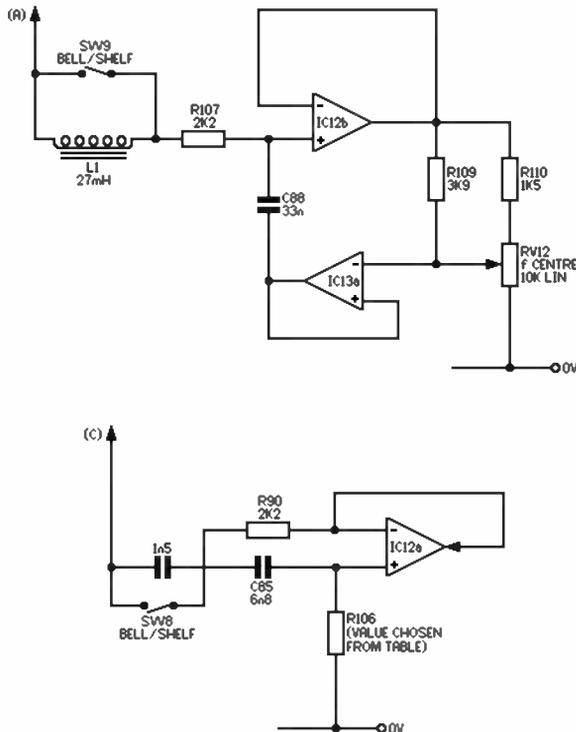
(a) HF EQUALISER WITH C87 OMITTED, R108 ALSO REPLACED BY SINGLE 2K2 RESISTOR AND 27MHz INDUCTOR TO ACHIEVE TRUE BELL TYPE RESPONSE.
