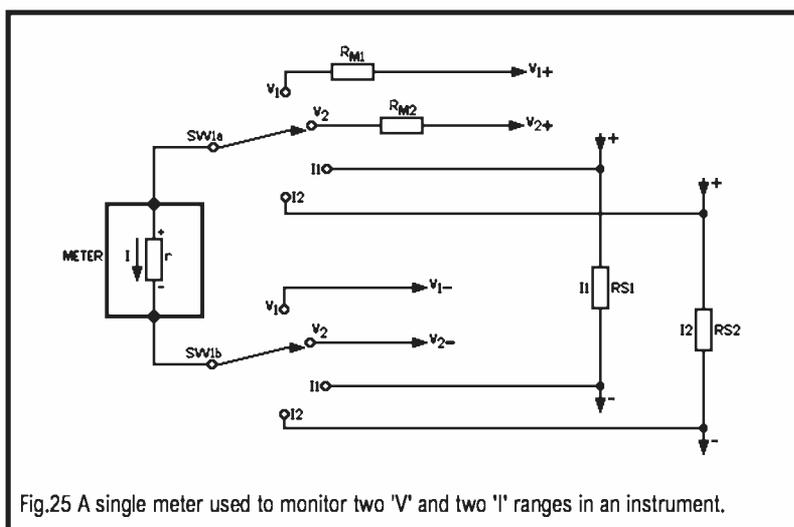
Fig.25 A single meter used to monitor two 'V' and two 'I' ranges in an instrument.
