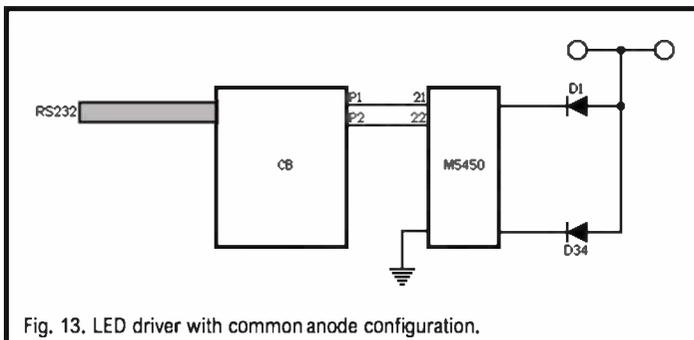
Fig. 13. LED driver with common anode configuration.
