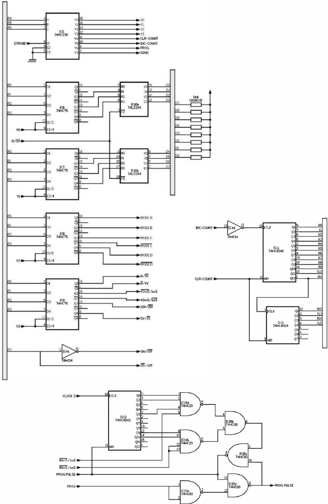
Fig. 2 EPROM Programmer Logic
