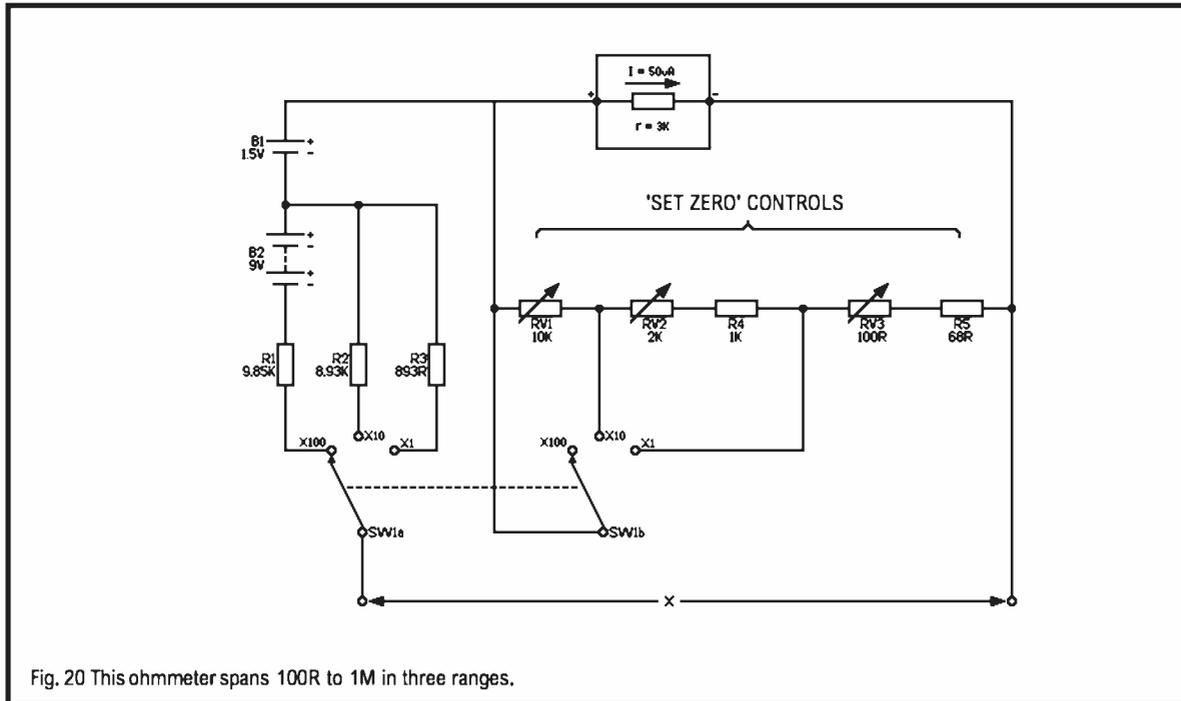
Fig. 20 This ohmmeter spans 100R to 1M in three ranges.
