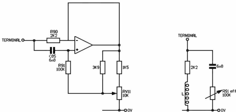
LF SHELF/BELL EQUALISER SHOWN WITH SHELF RESPONSE SELECTED, RV2 FREQUENCY CONTROL SET FOR MAX (100hz)
