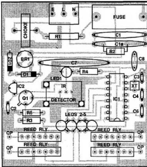
Fig.3 Component Overlay of receiver.
