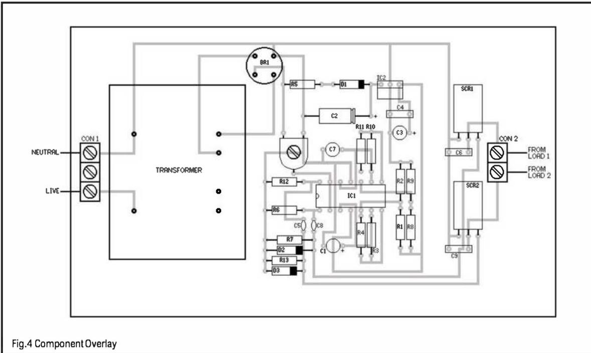
Fig.4 Component Overlay
