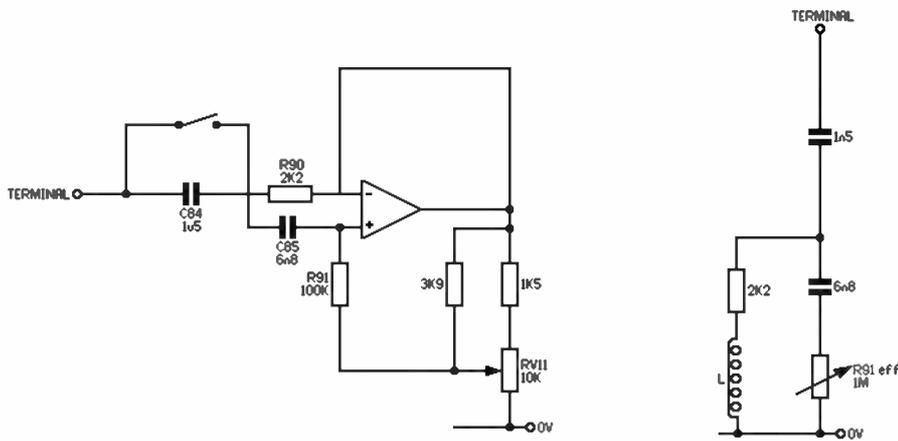
LF SHELF/BELL EQUALISER SHOWN WITH SHELF RESPONSE SELECTED, RV2 FREQUENCY CONTROL SET FOR MAX (30hz)
