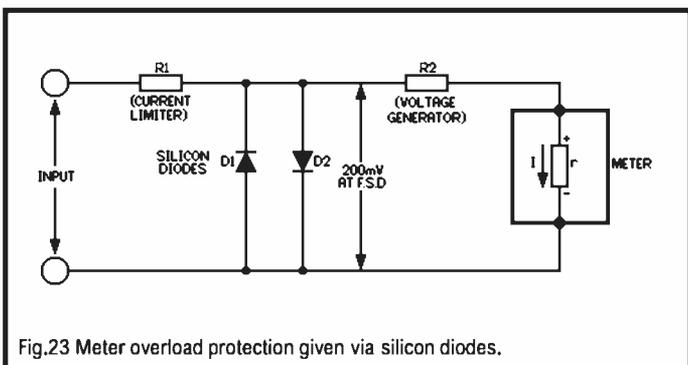
Fig.23 Meter overload protection given via silicon diodes.
