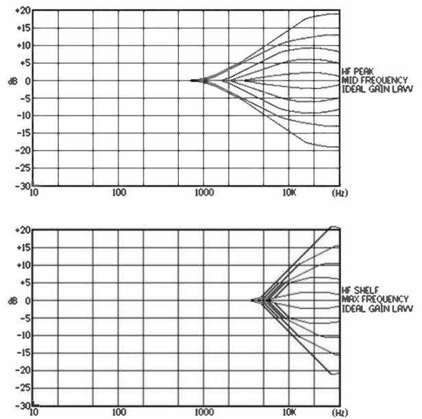
Fig. 13b HF Equaliser response curves (various cut and boost ratios)
