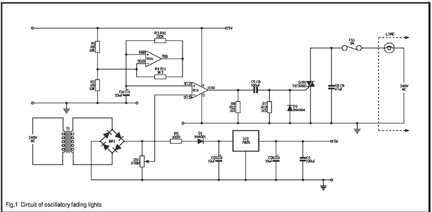
Fig.1 Circuit of oscillatory fading lights
