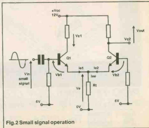
Fig.2 Small signal operation
