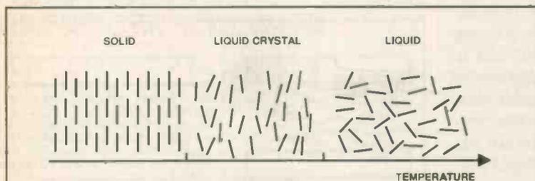
Fig.1 Indication of the solid, liquid crystal and liquid phases where in the solid phase molecules are fixed relative to each other with high level of organisation, in the liquid crystal phase molecules are more loosely associated but still have some collective structure and in the liquid phase the molecules are free to wander around the liquid with no level of order between the molecules.
