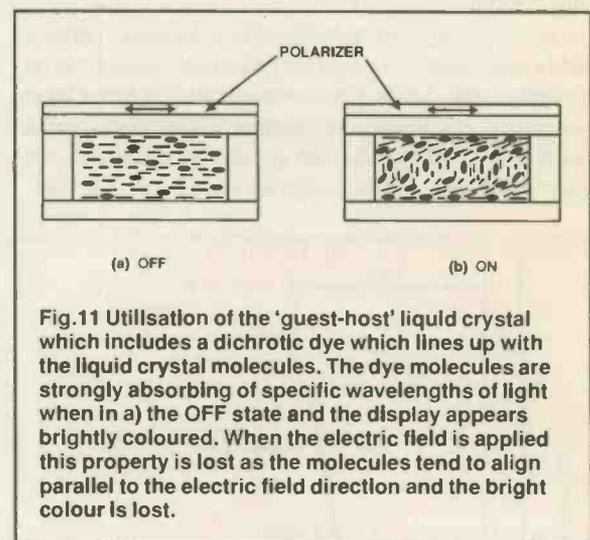
Fig.11 Utilisation of the 'guest-host' liquid crystal which includes a dichotic dye which lines up with the liquid crystal molecules. The dye molecules are strongly absorbing of specific wavelengths of light when in a) the OFF state and the display appears brightly coloured. When the electric field is applied this property is lost as the molecules tend to align parallel to the electric field direction and the bright colour is lost.
