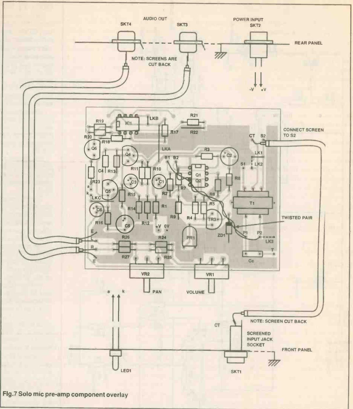
Fig.7 Solo mic pre-amp component overlay
