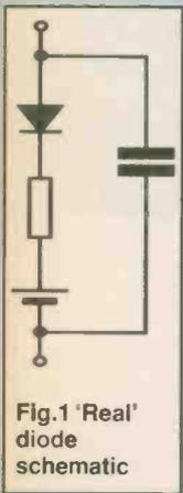
Fig.1 'Real' diode schematic
