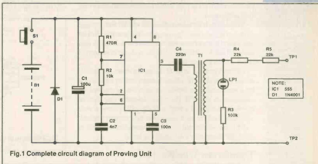
Fig.1 Complete circuit diagram of Proving Unit
