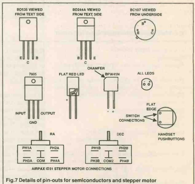
Fig.7 Details of pin-outs for semiconductors and stepper motor
