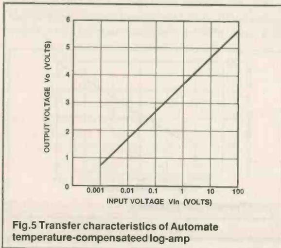
Fig.5 Transfer characteristics of Automate temperature-compensated log-amp
