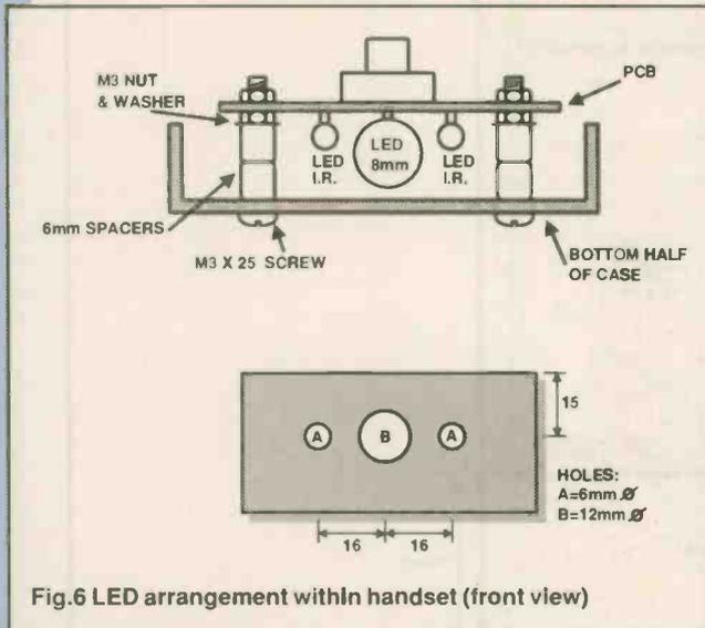
Fig.6 LED arrangement within handset (front view)
