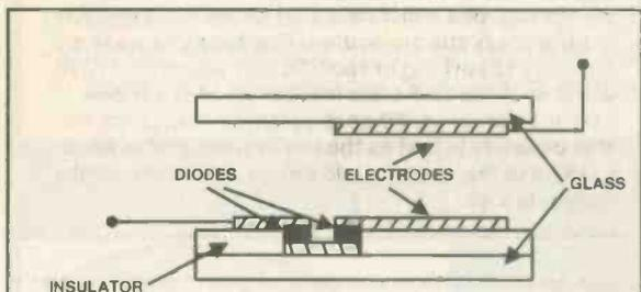
Fig.13 In the active matrix display, the drive signal is modified by a back to back diode. This sharpens the response of the LCD element and allows increases the degree of multiplexing possible. Such technology has been used for pocket colour televisions.
