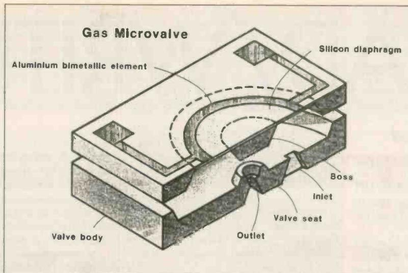
film deposited on the diaphragm forms the other element of the bimetallic structure. Varying the electrical power dissipated by resistors implanted in the diaphragm makes the temperature of the diaphragm change. As temperature increases, the difference in thermal expansion between the sili-
