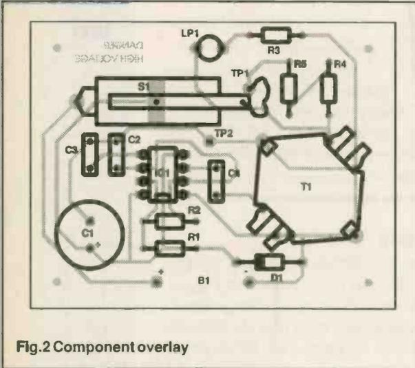
Fig.2 Component overlay
