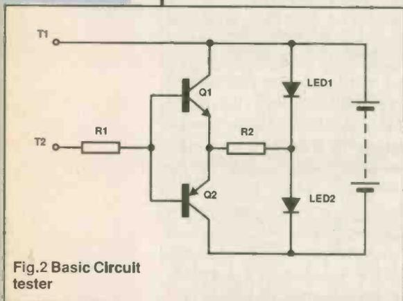
Fig.2 Basic Circuit tester
