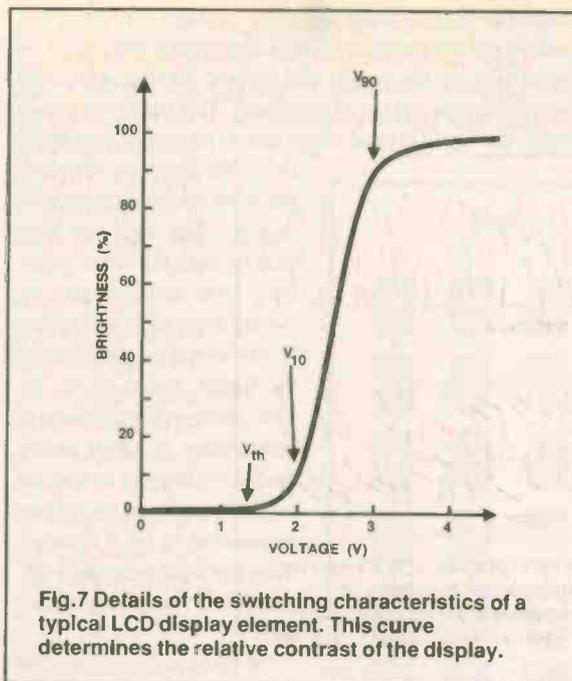
final brightness.  $T_{off}$  is defined as the time taken from switch off to derive 10% brightness. Where  $B_{low}$  and  $B_{high}$  are the brightness values of the two states of the display, the contrast of the display is defined as the ratio of  $B_{high}/B_{low}$ . Values range typically from 10 to 50.
