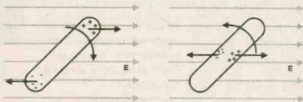
Fig.4 Liquid crystal molecules can exhibit either a permanent dipole as shown in a) or an induced dipole as shown in b) when placed in an electric field. In the case of the permanent dipole the molecule will tend to be aligned in the direction parallel to the field and in the case of the induced dipole at right angles to the field.
