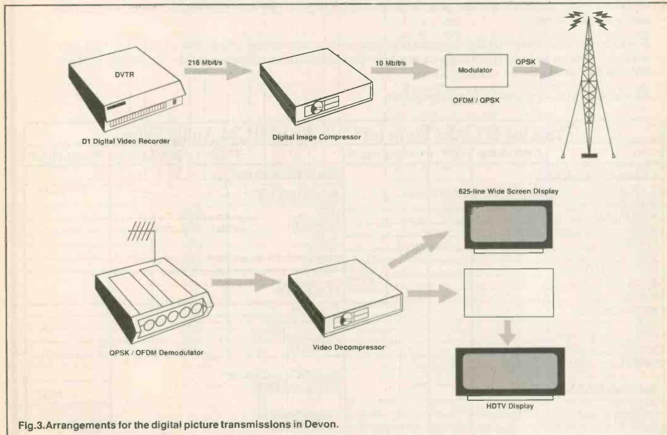
Fig.3. Arrangements for the digital picture transmissions in Devon.
