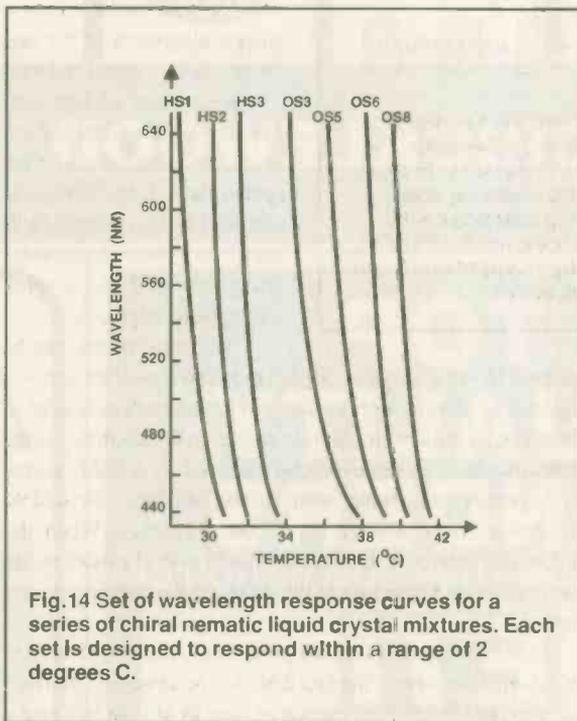
Fig.14 Set of wavelength response curves for a series of chiral nematic liquid crystal mixtures. Each set is designed to respond within a range of 2 degrees C.
