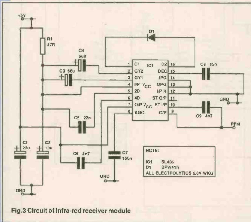
Fig.3 Circuit of Infra-red receiver module
