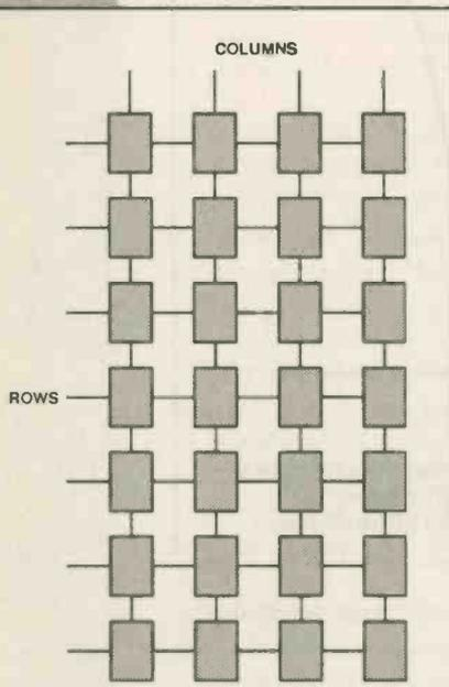
Fig.9 Connection details of multiplex lines to a 4x7 LCD array. Separate connections drive all elements in rows on the upper surface with separate connections driving columns on the lower surface. Only elements activated at the same time by an upper and lower drive signal will be active.
