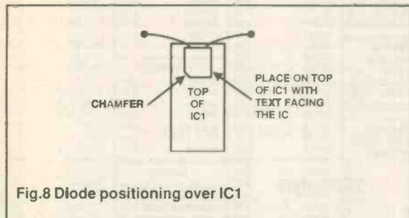
Fig.8 Diode positioning over IC1
