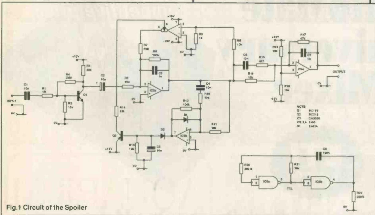
Fig.1 Circuit of the Spoiler
