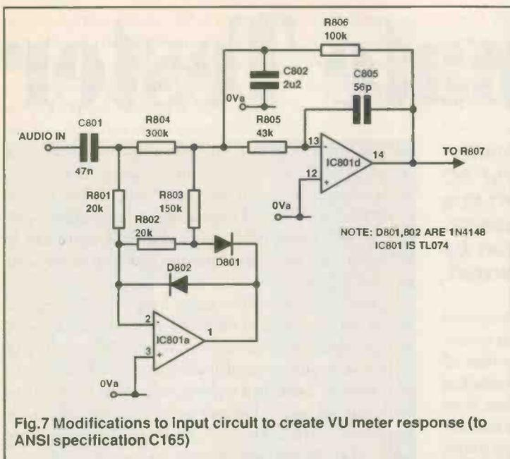
Fig.7 Modifications to Input circuit to create VU meter response (to ANSI specification C165)
