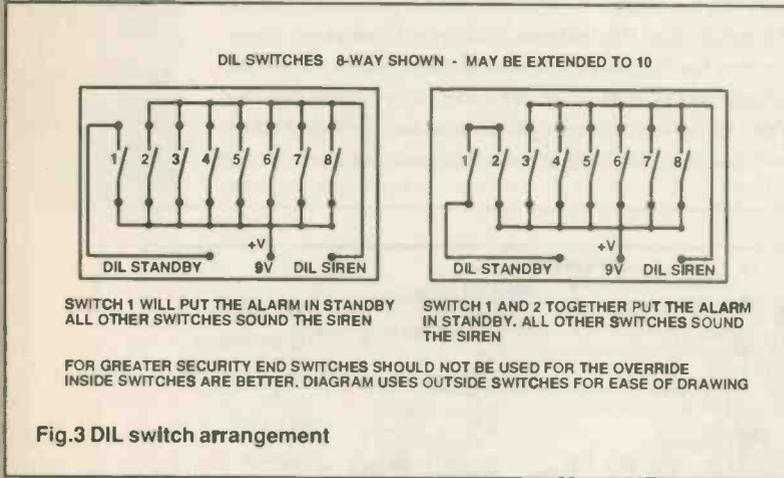
Fig.3 DIL switch arrangement
