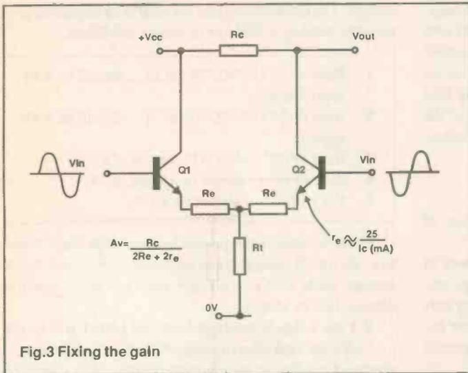
Fig.3 Fixing the gain
