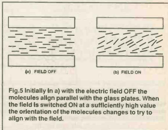
Fig.5 Initially in a) with the electric field OFF the molecules align parallel with the glass plates. When the field is switched ON at a sufficiently high value the orientation of the molecules changes to try to align with the field.
