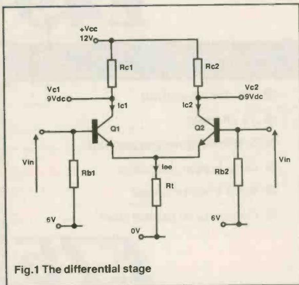
Fig.1 The differential stage
