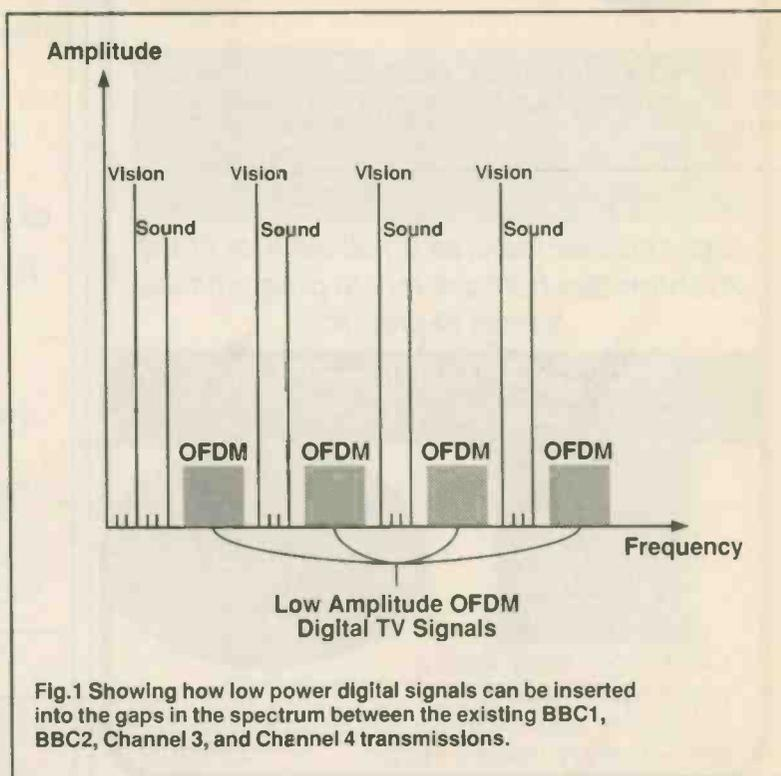
Fig. 1 Showing how low power digital signals can be inserted into the gaps in the spectrum between the existing BBC1, BBC2, Channel 3, and Channel 4 transmissions.
