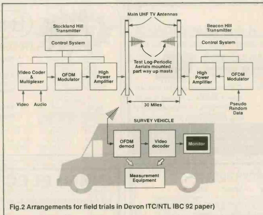
Fig. 2 Arrangements for field trials in Devon ITC/NTL IBC 92 paper)
