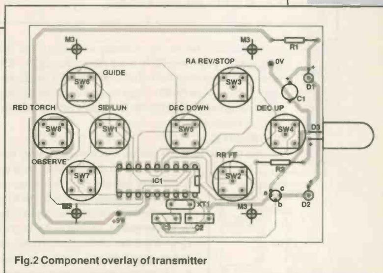
Fig.2 Component overlay of transmitter
