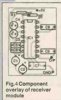
Fig.4 Component overlay of receiver module
