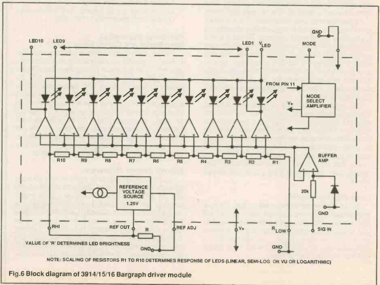
Fig.6 Block diagram of 3914/15/16 Bargraph driver module
