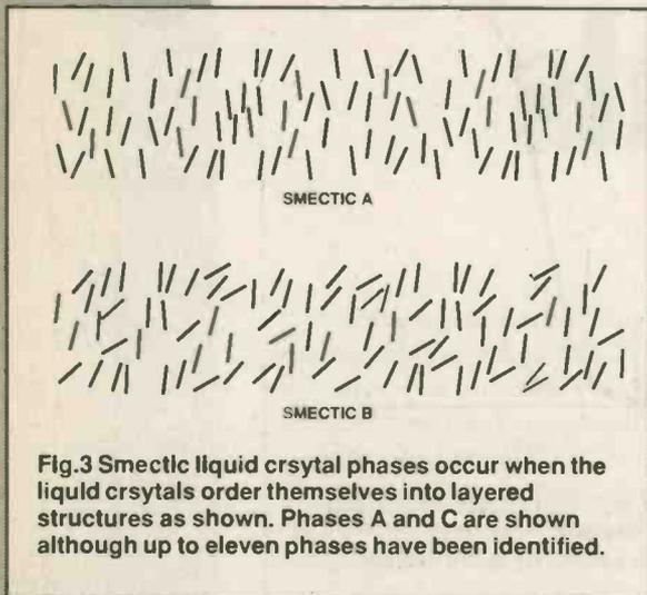
Fig.3 Smectic liquid crystal phases occur when the liquid crystals order themselves into layered structures as shown. Phases A and C are shown although up to eleven phases have been identified.
