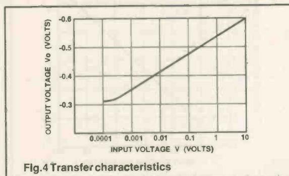
Fig. 4 Transfer characteristics
