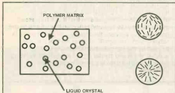
Fig.12 Details of polymer dispersed liquid crystal structures. The liquid crystal is contained in spheres contained with a layer of polymer material. The director of the liquid crystal molecules (line up direction of molecules) can occupy two states as shown in b) - parallel to spherical surfaces or at right angles to spherical surfaces. When the director of the liquid crystal lines up with an applied field, the light which falls directly interacts primarily with these liquid crystals.
