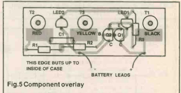
Fig.5 Component overlay
