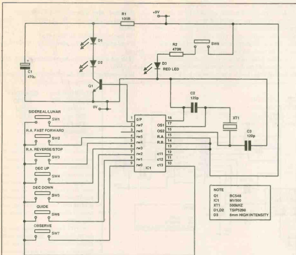
Fig.1 Circuit diagram of Infra-red transmitter
