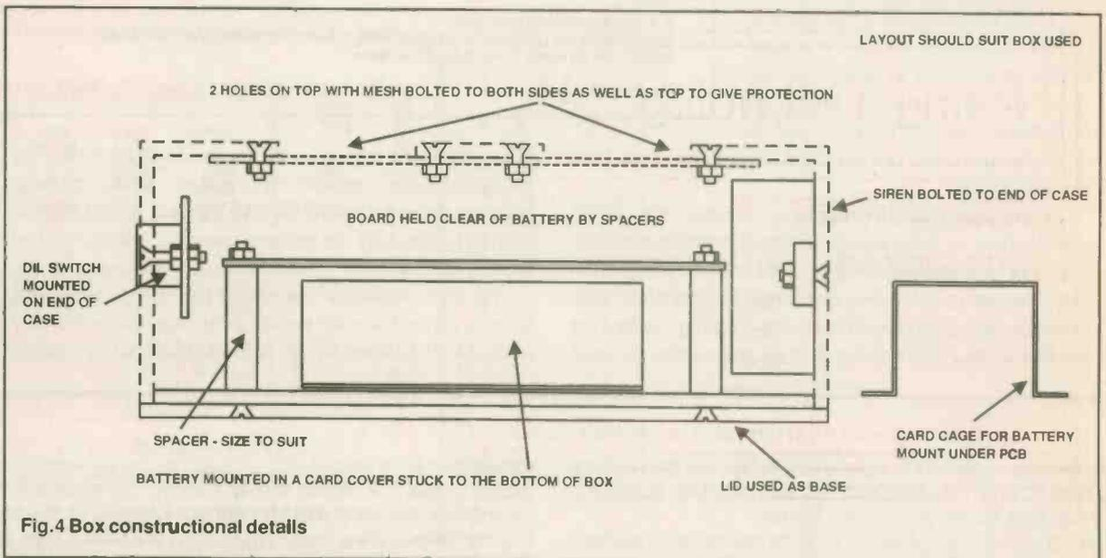
Fig.4 Box constructional details
