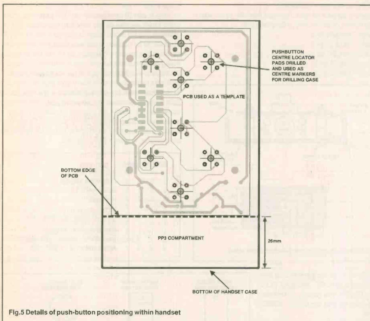
Fig.5 Details of push-button positioning within handset
