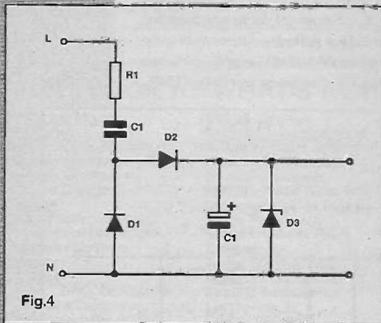
and, in order to calculate the average direct current available it is necessary to average the current in R1 over a whole mains cycle, even though the current is only flowing during positive half-cycles.
