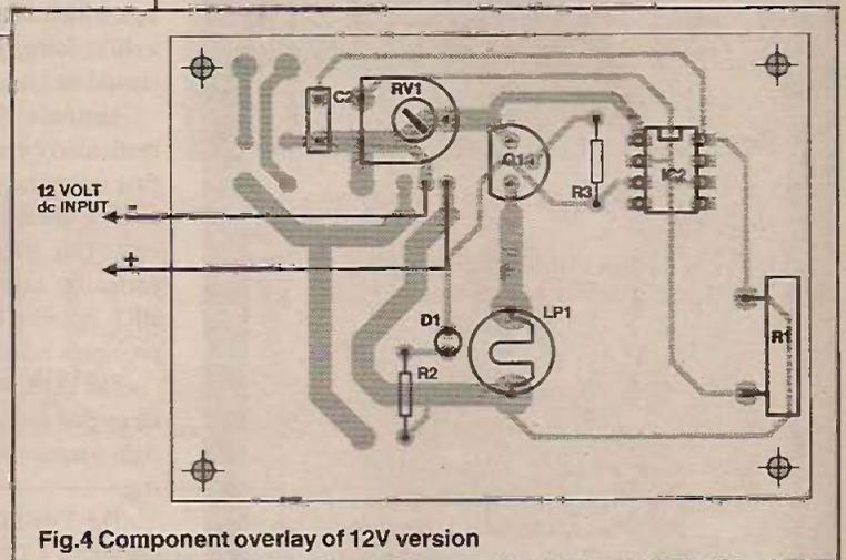
Fig.4 Component overlay of 12V version
