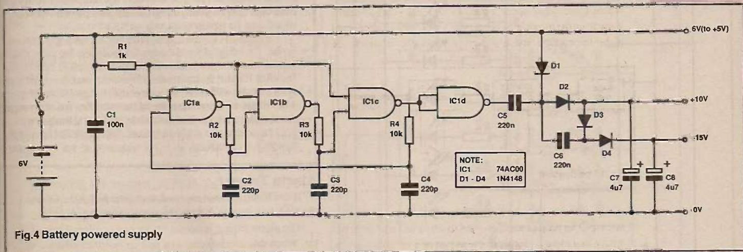
Fig.4 Battery powered supply
