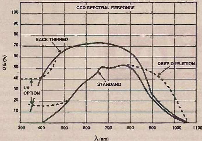
Fig.9 Typical Quantum efficiency of CCD units. Specific options of back thinning, deep depletion or UV enhancement can improve performance as indicated.
