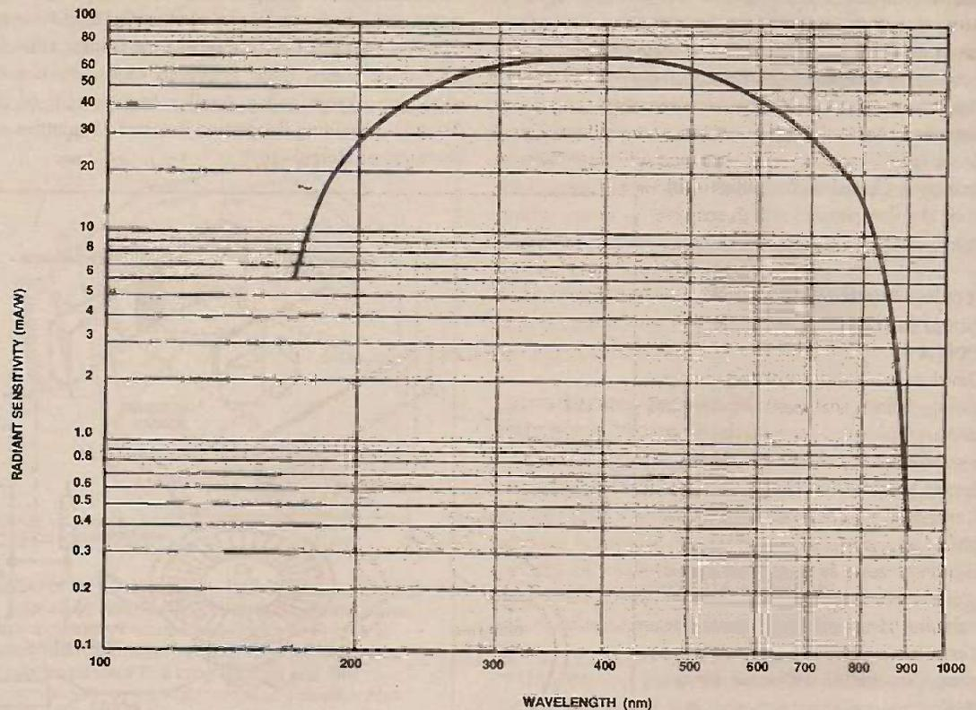
Fig.6 Spectral response of a photomultiplier tube (Rees Instruments 6118/7) which provides significantly greater sensitivity compared with silicon photodiodes
