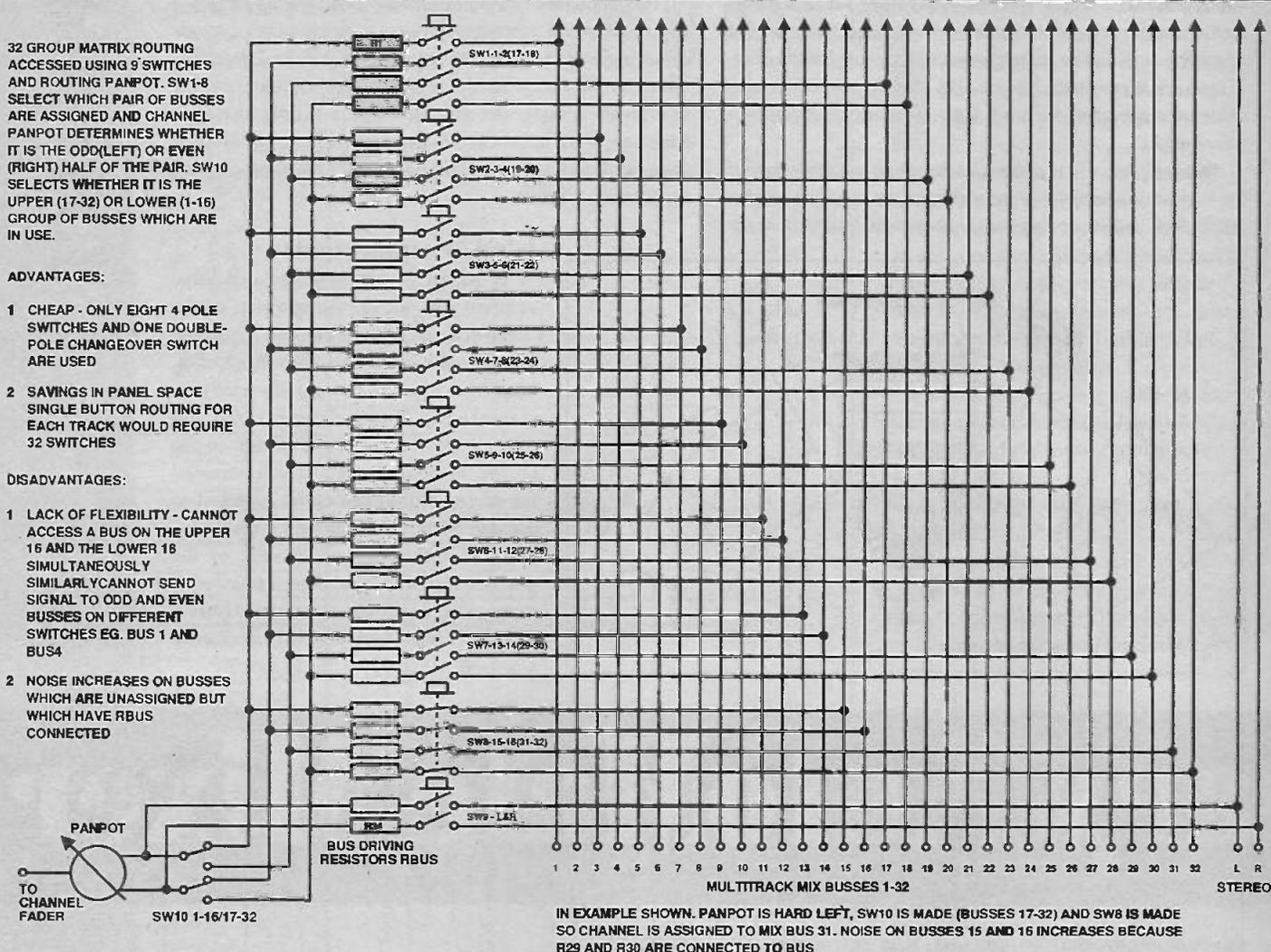
Fig.3a Group routing matrix example (32 bus example - limited access)
