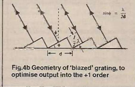
Fig.4b Geometry of 'blazed' grating, to optimise output into the +1 order
