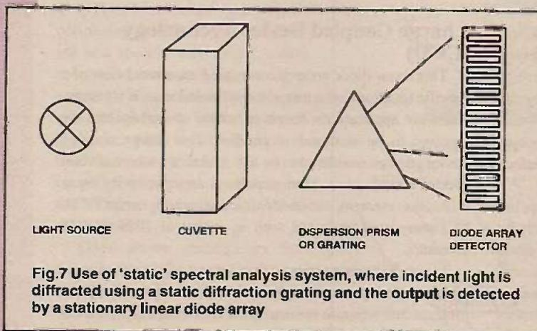
Fig.7 Use of 'static' spectral analysis system, where incident light is diffracted using a static diffraction grating and the output is detected by a stationary linear diode array
