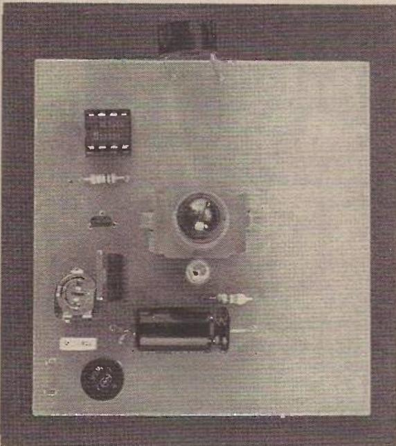
hysteresis for correct operation. Without this hysteresis, the output would fluctuate between the on and off states as the lamp was switched on and the photocell being illuminated by the lamp would experience a fall in resistance, thus turning the lamp off again. This would repeat cyclically until the ambient light level fell sufficiently for the combined effect of daylight and the light from the lamp to be insufficient for repeated triggering.
