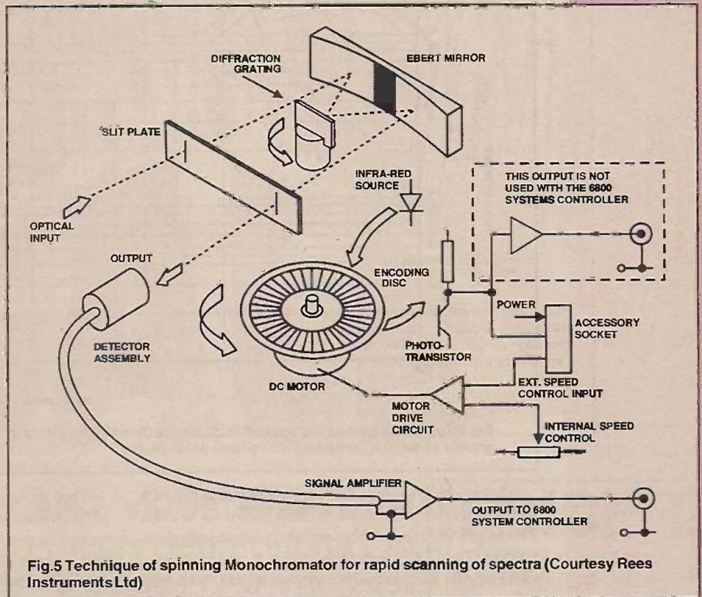
Fig.5 Technique of spinning Monochromator for rapid scanning of spectra (Courtesy Rees Instruments Ltd)
