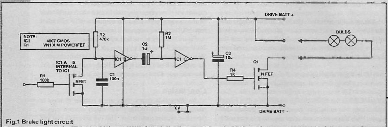
Fig.1 Brake light circuit
