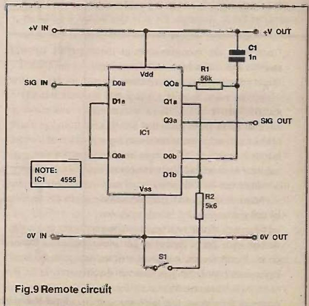
Fig.9 Remote circuit
