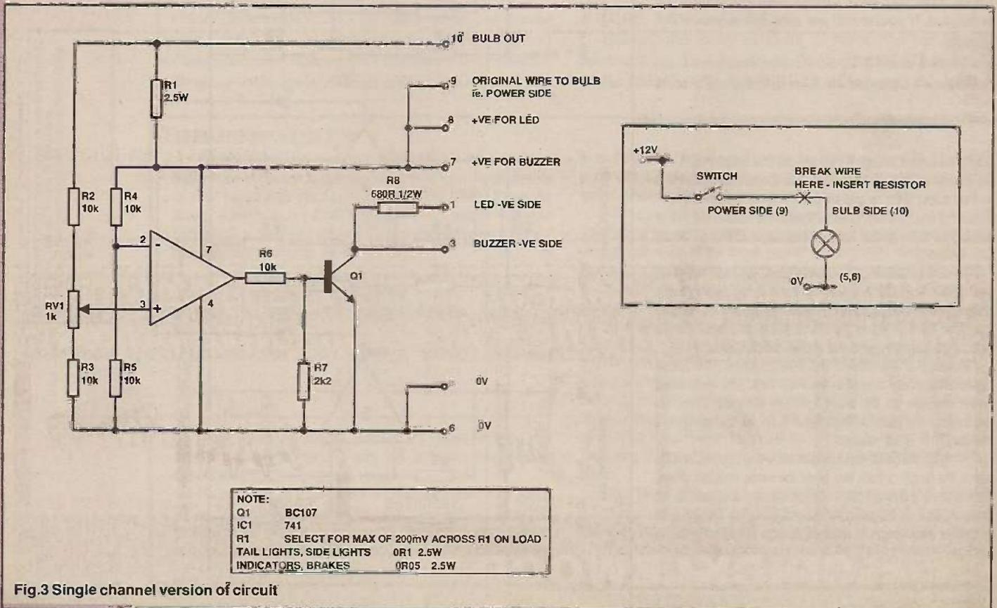
Fig.3 Single channel version of circuit
