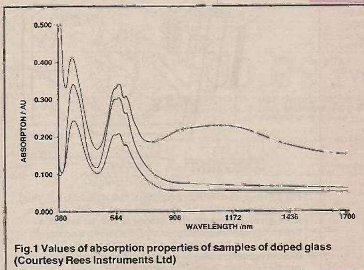
Fig.1 Values of absorption properties of samples of doped glass (Courtesy Rees Instruments Ltd)
