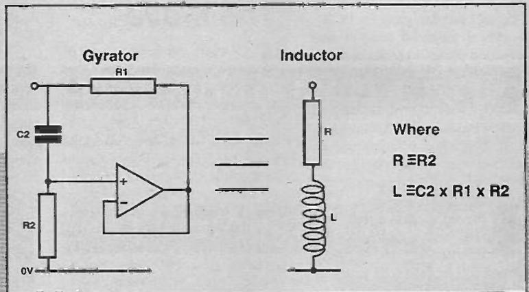
The answer comparing the gyrator with an inductor and a series resistor, is shown in the diagram.
