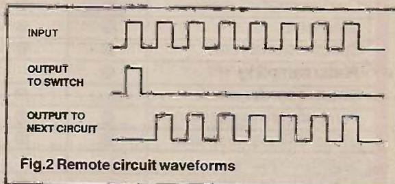
Fig.2 Remote circuit waveforms
