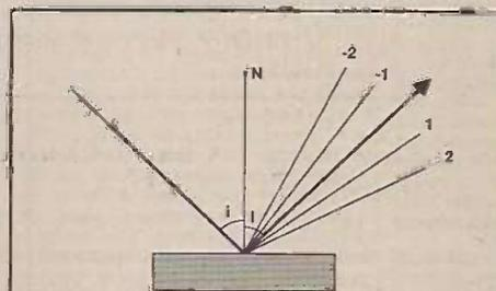
Fig.4a Process of diffraction of light by a reflection grating into different orders +2, +1, 0, -1 and -2
