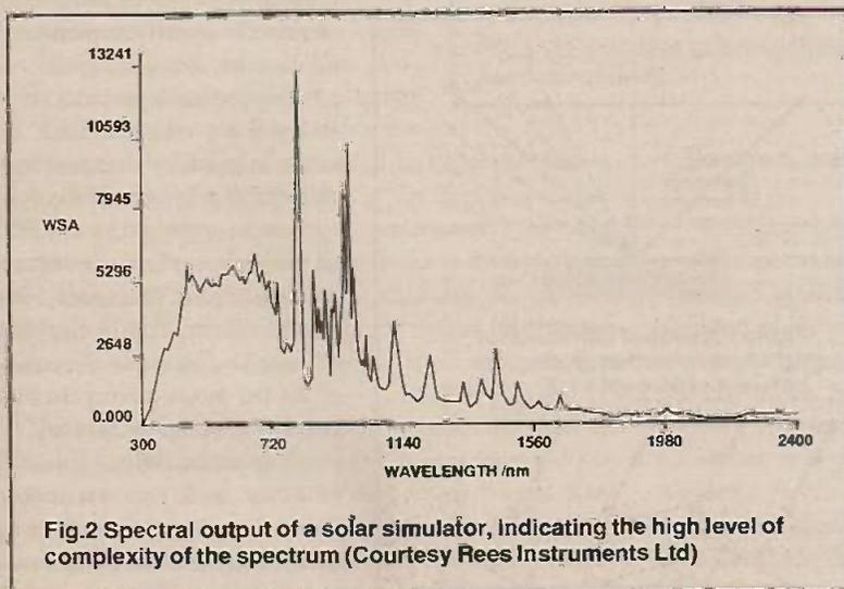
Fig.2 Spectral output of a solar simulator, indicating the high level of complexity of the spectrum (Courtesy Rees Instruments Ltd)
