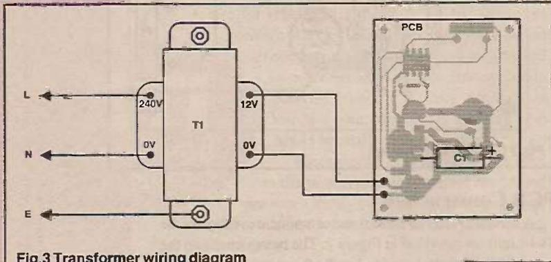
Fig.3 Transformer wiring diagram
