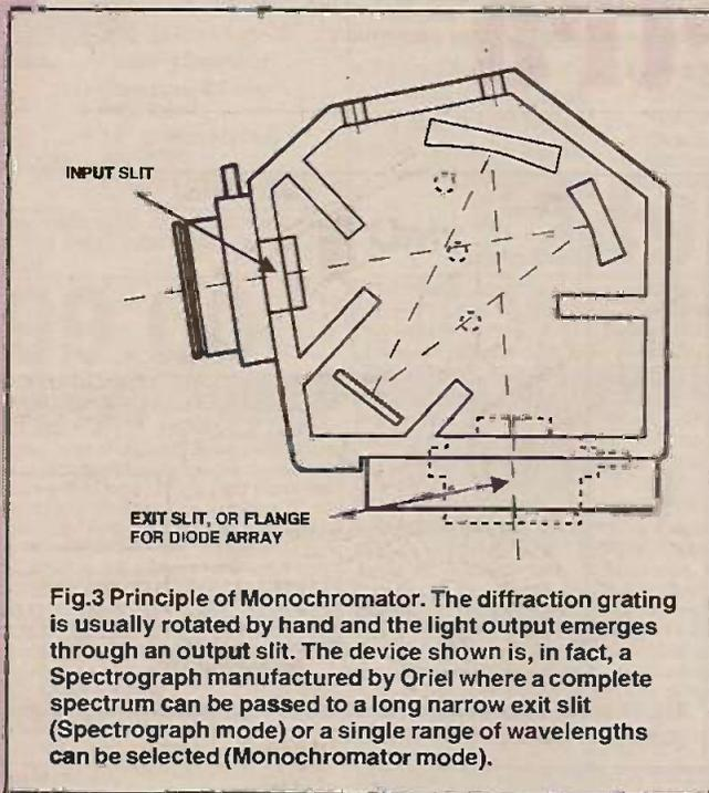
Fig.3 Principle of Monochromator. The diffraction grating is usually rotated by hand and the light output emerges through an output slit. The device shown is, in fact, a Spectrograph manufactured by Oriel where a complete spectrum can be passed to a long narrow exit slit (Spectrograph mode) or a single range of wavelengths can be selected (Monochromator mode).
