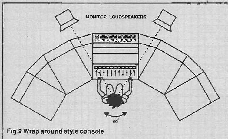
Fig.2 Wrap around style console
